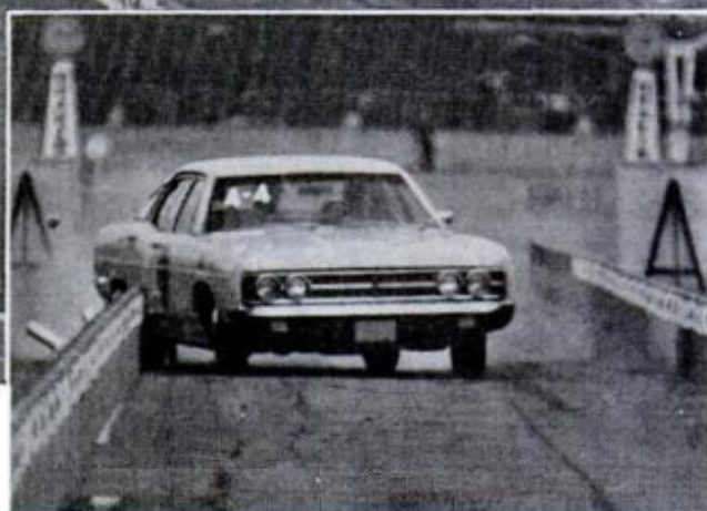
EMERGENCY STOPPING LANE is 500 feet long marked with pylons. If brakes lock unevenly, car will not stop straight. Penalty imposed is 2 feet per pylon
