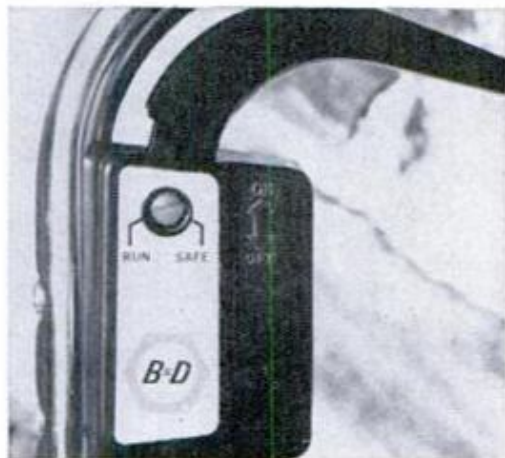
CONTACT SWITCH is quick-release type. Safety lock prevents accidental starting
