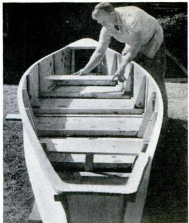
TO MAKE SPONSON, rest foam block beside hull, use a block of wood and pencil to scribe the curve
