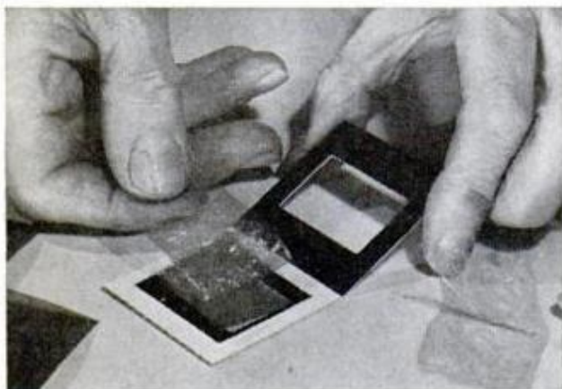
CRUMPLED CELLOPHANE combined with polarizing filter produces striking patterns of changing color. Bind a small piece of each together in a slide mount and insert with filter toward the projector lamp
