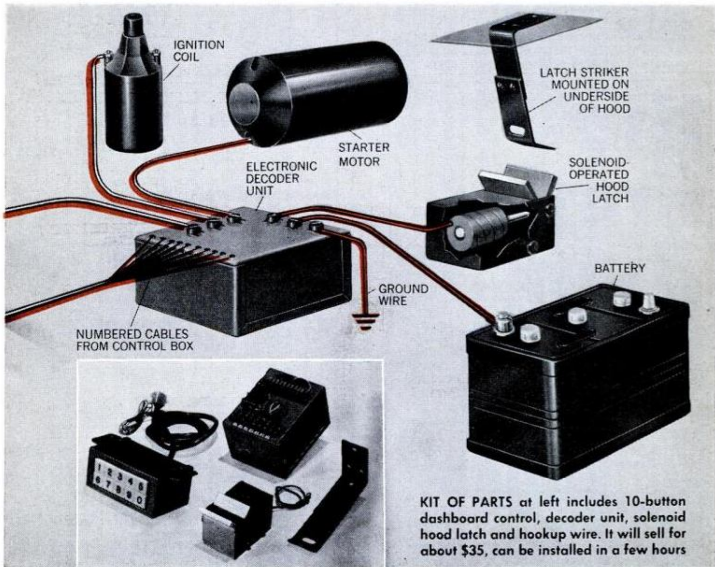
DECODER UNIT and hood latch can mount anywhere in engine compartment, against a side wall or on engine itself with brackets. The code can be changed merely by rearranging connections on the decoder
