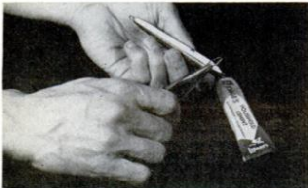
9. PLASTIC MAY BE CUT with soldering gun attachment or by scoring with a sharp knife and breaking along score line. Set in slot with waterproof glue
