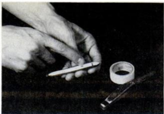
8. CUT WATERPROOF TAPE 4 inches long and \frac{1}{4} inch wide; make slit where wire insert protrudes. Fasten to lure bottom and cut slot for plastic lip
