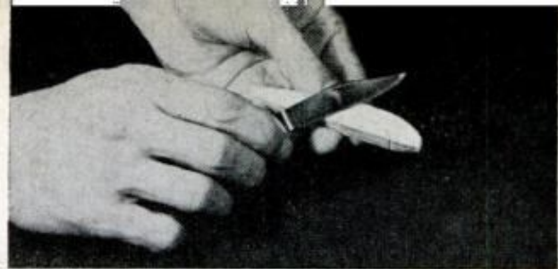
2. CUT BALSAWOOD to basic minnow shape, removing an even amount of the material from each side
