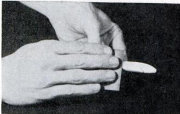
3. TRIM AND SAND SMOOTH — \frac{1}{4} -inch lengthwise cut is to hold wire prepared per color diagram below
