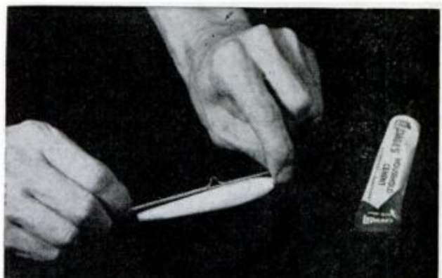
4. SHAPE AND SOLDER wire insert; with waterproof glue, fix it in slot. Diagonal cut is for plastic lip
