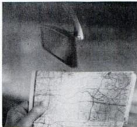
SEVERAL OWNERS didn't like the rearview mirror—too big (12 in. wide), blocks their forward vision
