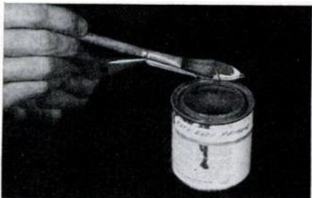
5. COAT ALL SURFACES and crevices with red oxide primer. When dry, smooth with No. 400 wet paper
