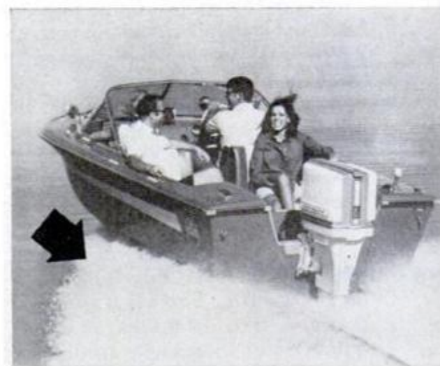
DEEP VEE HULL is a good rough-water design which plows groove in the water, sending it out to sides with much spray
