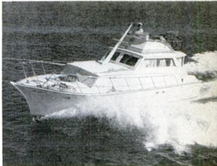
POWER IS LOST in overcoming water resistance with a heavy boat; it may not lift much from water
