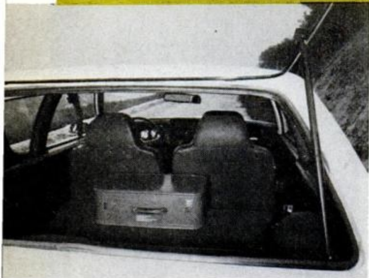
HINGED REAR WINDOW in the four-passenger model raises to gain cargo-area access. Back seat folds flat
