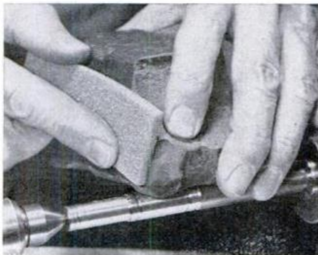
RIGID PLASTIC-FOAM BLOCK , rubbed over a cake of buffing compound, provides an adequate sheen, too
