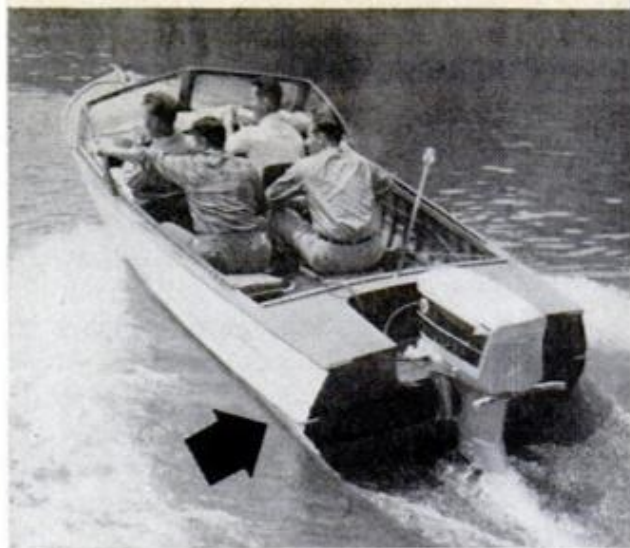
WATER FLOWS UP SIDES of round bilge boat causing skin friction without adding to hull's lifting ability when on a plane
