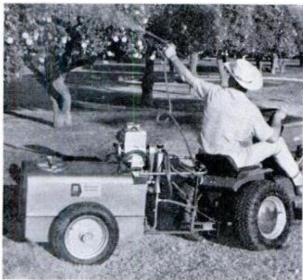
50-GALLON POWER SPRAYER for orchard work can be run from driver's seat. Sprayer, $440; hitch, $16
