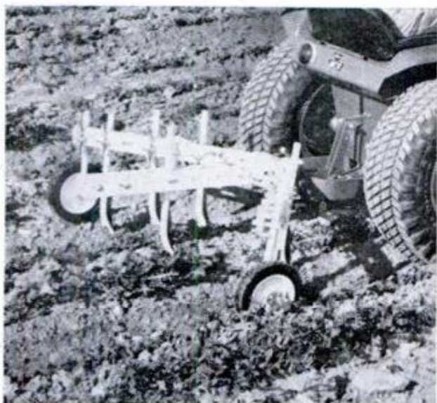
ROW CROP CULTIVATOR eliminates hand weeding. It adjusts for 6 to 42-inch rows, $50; hitch is $30
