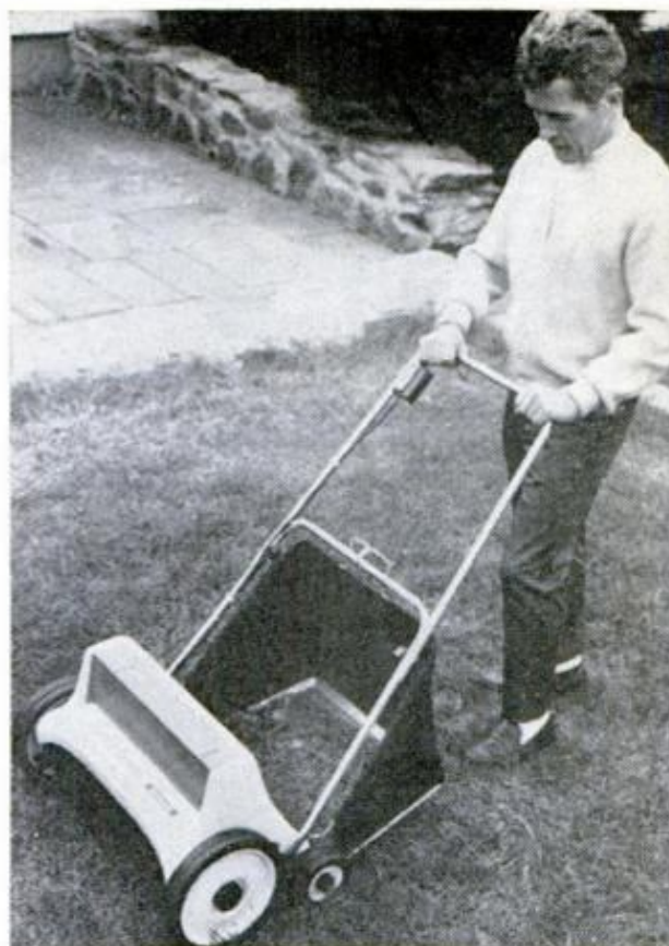
CLEAN-LINED PLASTIC SHROUD conceals motor, battery. Rear wheels replace the conventional roller bar
