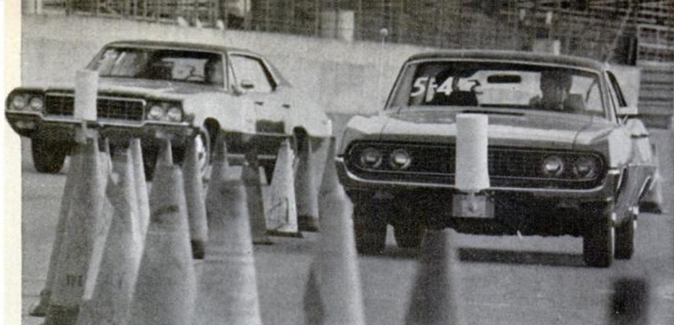
ECONOMY TEST in the Union 76 Performance Trials uses a separate fuel supply mounted on front of the car
