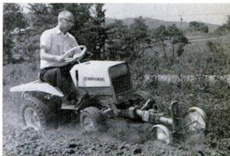
ROTARY PLOW (on Gravely 430) prepares seedbed without other preparation; it's $128, plus adapter kit
