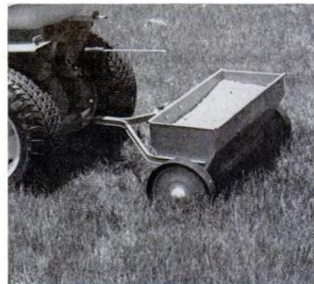
LAWN-SEEDER-FERTILIZER , 30 inches wide, has 85-pound hopper. Lever at seat starts, stops flow. $102
