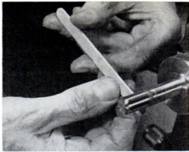
TIGHT GROOVES ARE POLISHED with flat stick charged with abrasive grit mixed with a light oil
