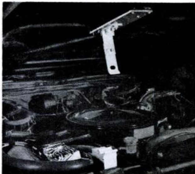
LATCH STRIKER PLATE is bolted to underside of hood so it slips into a slot in the solenoid-operated latch when the hood is closed. Latch bolt engages hole in the striker plate to lock hood securely
