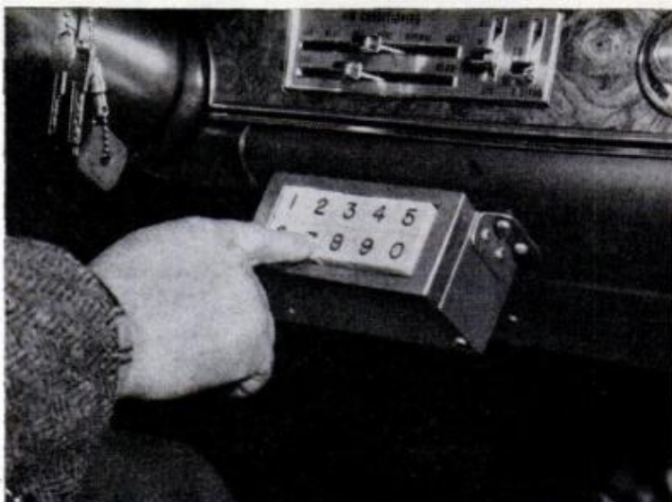
KEYBOARD CONTROL mounts under the dash, has 10 numbered pushbutton switches. To start the car, you must press four of the 10 buttons in a coded sequence. Possible number of different codes: 5024
