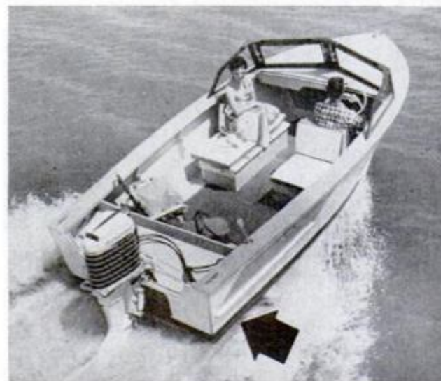
WATER DOES NOT TOUCH SIDES and shoots clear of hard chine hull's bottom, giving exceptionally dry ride, greater lift
