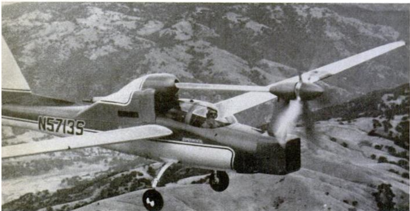
MONGREL CONFIGURATION of Q-Star resulted from center-of-gravity problem. Engine is behind cockpit
