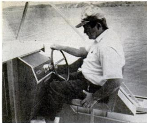
MANY DASHBOARDS are set so low as to cause bottom edge to press uncomfortably on driver's knees
