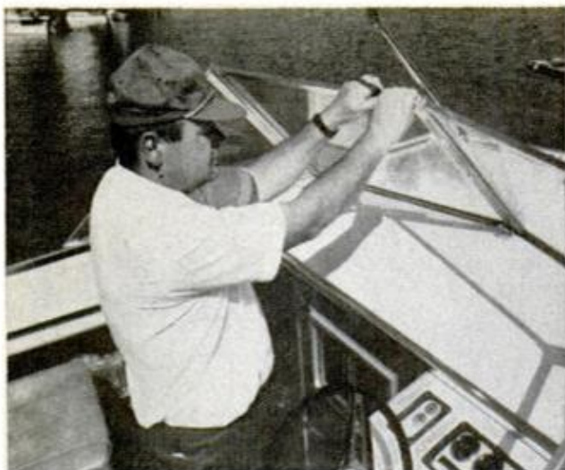
THIS WINDSHIELD HAS NO BRACING to resist strain caused by people grasping top or leaning against it
