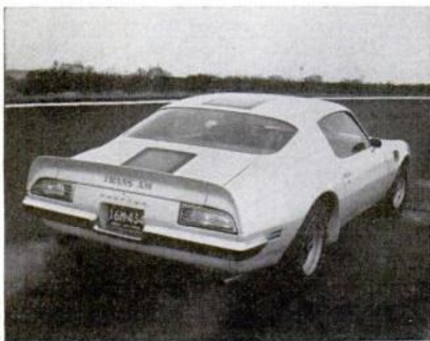
AIR SPOILER is featured on rear deck of Trans Am version of Firebird. Note "airdams" on wheel openings
