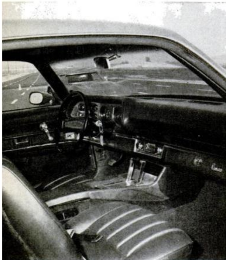
CAMARO DASHBOARD has been completely redesigned with a wraparound theme. Mirror bonded to windshield glass is new. Hidden wipers are optional
