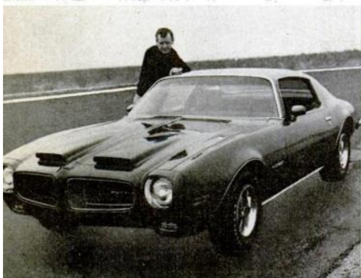
HOOD SCOOPS mark Formula 400 version, force cool air to carburetor. Car's only 50.4 in. high overall
