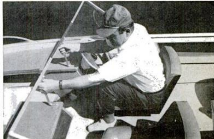
PAIR OF STURDY BRACES reinforcing this windshield helps it to withstand inevitably rough handling
