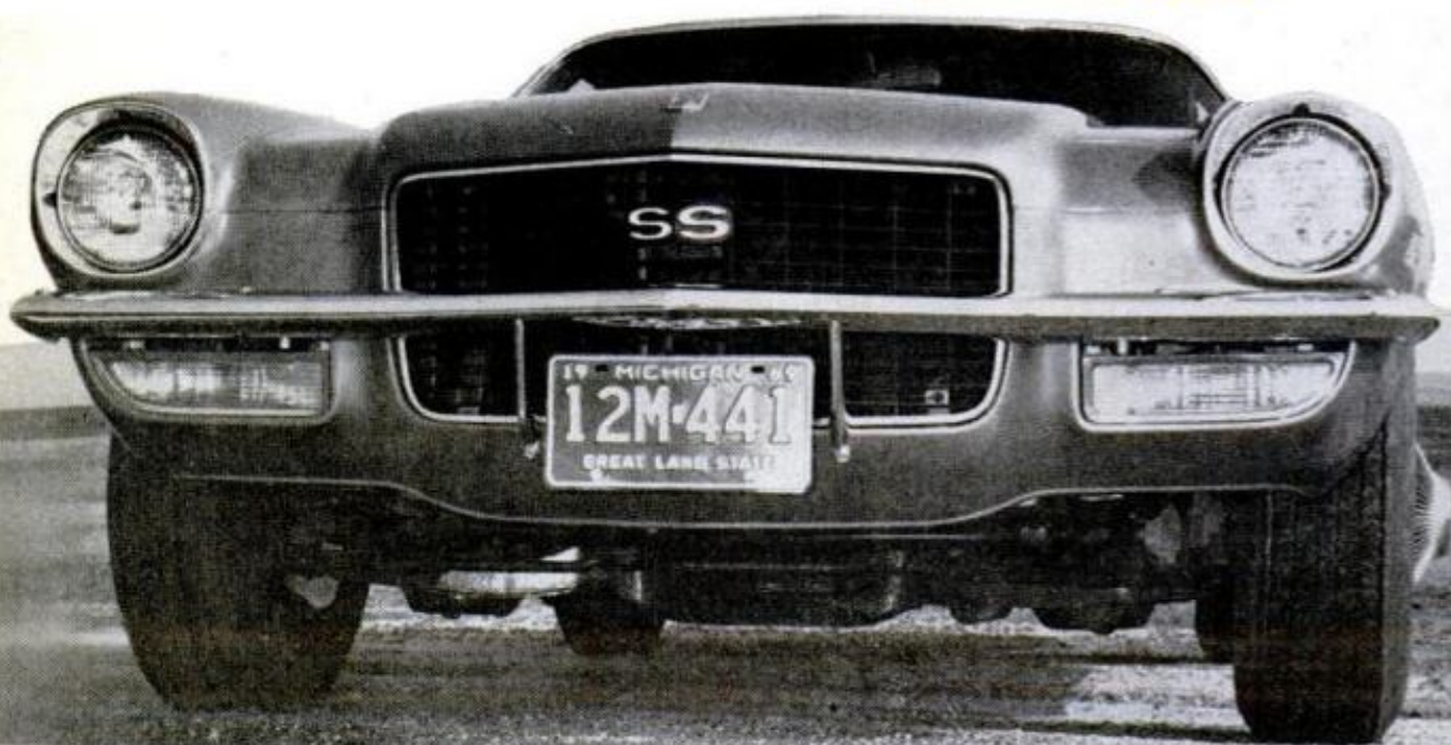
CAMARO SS front-end treatment features a full-width front bumper which divides the grille. Turn-signal/parking lights are below the bumper. Standard on all Camaro models for 1970 are front-wheel disc brakes
