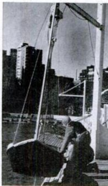
WELL-FURNISHED MARINA will provide little extras like an electric hoist, to make easy work of launching small sailboats, and locking gate to the gas dock
