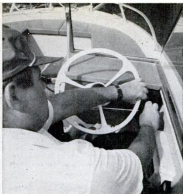
HERE'S A STEERING WHEEL that's installed too close to cockpit side, causing interference between steering hand and motor-control hand when maneuvering
