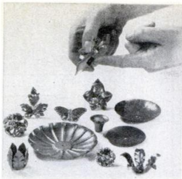
ORNAMENTS CAN BE INSERTED in scrollwork's riveted joints. Most have spot-welded angle brackets
