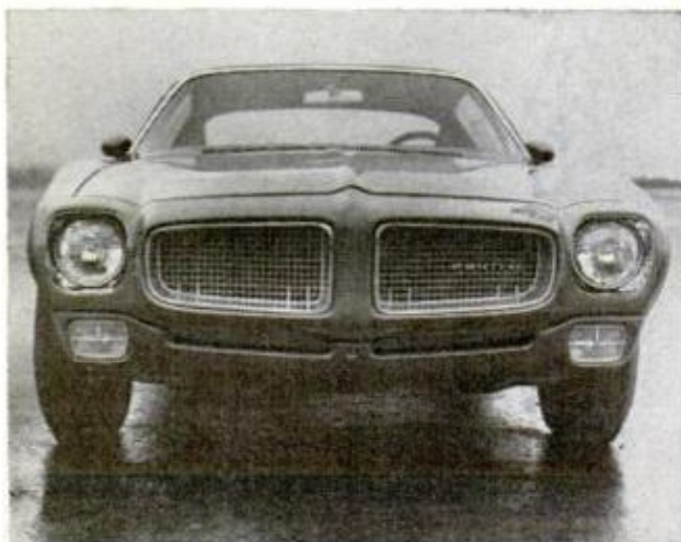
FRONT BUMPER of rubberized plastic wraps around single headlamps, blends smoothly into hood, fenders
