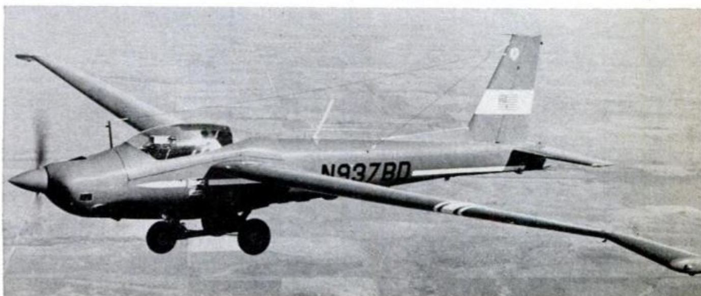
"BEDE'S "ROUND THE WORLD" PLANE has a 210-hp engine, wingtip extension for stability and fuel storage
