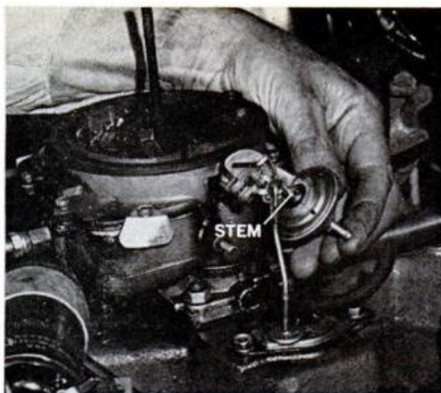
IF VACUUM IS GOOD check diaphragm by depressing stem, then covering vacuum opening (see text)
