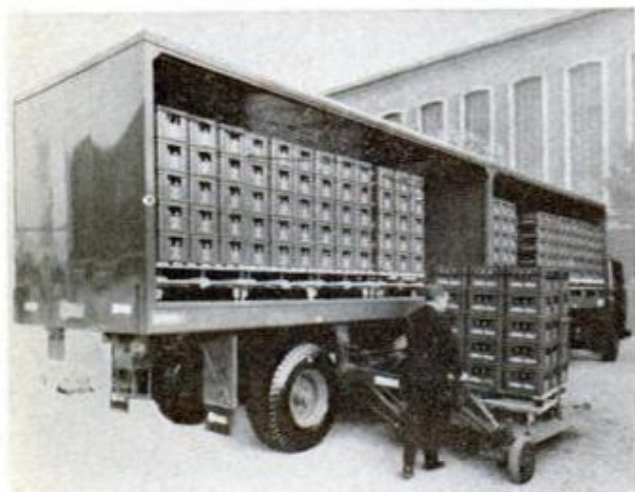
ELEVATING LOADER , shown here on big beer trailer, moves up and down electrically at push of a button, full length of the trailer bed on a suspended track. When you're through using the loader, you park and tote it in the "kneehole" located underneath the floor of the trailer. Loader was exhibited by Rationorm
