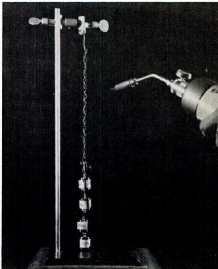
HEATED, titanium alloy "remembers" original coiled shape, as shown through time-lapse photography
