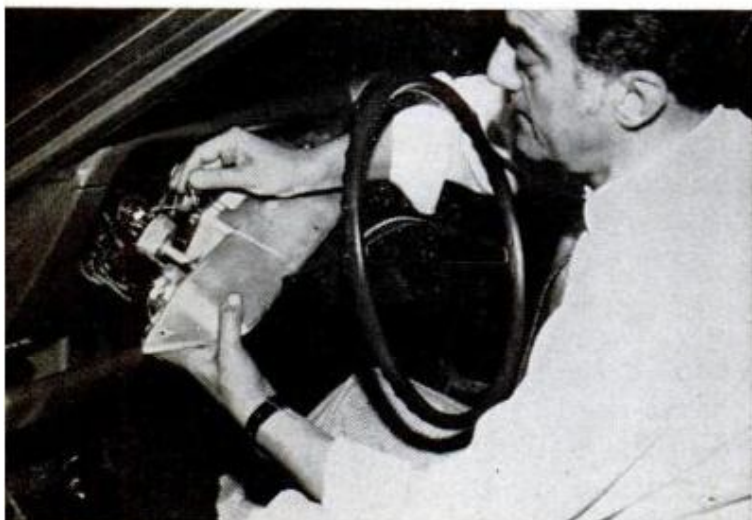
INSTRUMENT PANELS on new Hornet (left) and Maverick are easily removed, providing quick access for check-out of wiring, instrument repair, bulb replacement. Note foolproof printed circuit on Maverick
