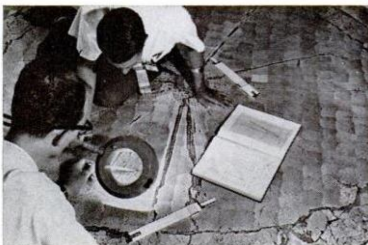
MAGNIFIED PHOTOMOSAIC of cross section of a half-inch-diameter fuel element is studied for possible improvement
