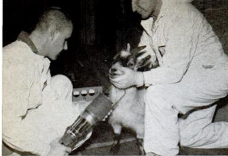
RADIOIODINE IN THYROID of miniature goat is monitored by staff members at Battelle-Northwest lab
