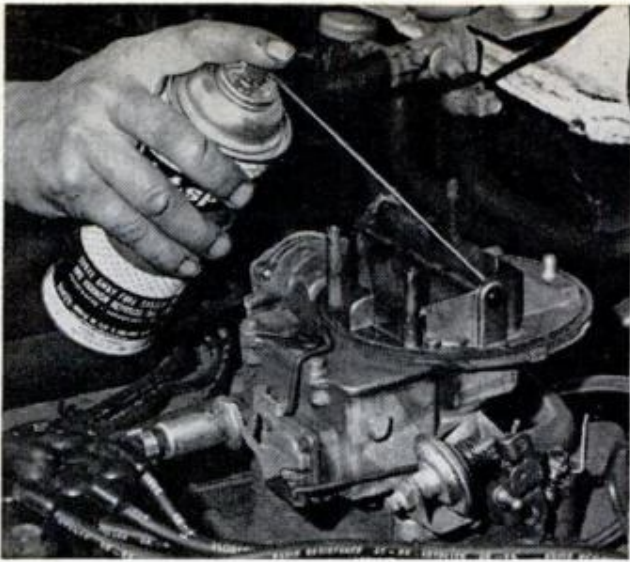
CHOKE VALVE sticking because of buildup of deposits is troublemaker. Clean as routine maintenance
