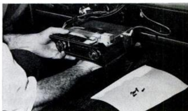
RADIO of Maverick can be removed via four screws in fraction of time required for most installations
