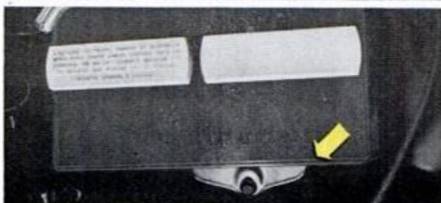
BATTERY OF AMC Rambler is held in place by means of two bolts. Same job is done by one on the Hornet
