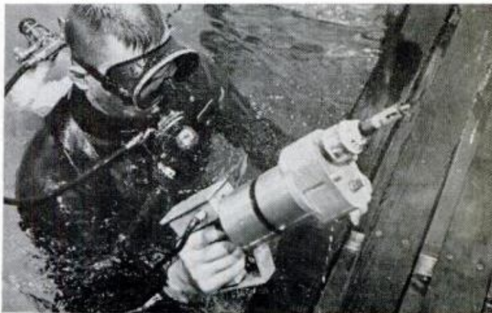
UNDERWATER TOOL can drill through quarter-inch steel in 20 seconds. It was developed for the Navy
