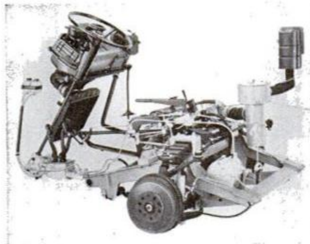
FRONT-WHEEL-DRIVE gives Fiat 238 trucks and vans great capacity, low loading height (16 inches). Engine-transmission unit mounted transversely ahead of cab puts load on front wheels to give maximum traction, even when van is empty. Four-cylinder engine has 1438 cc, all four wheels independent suspension
