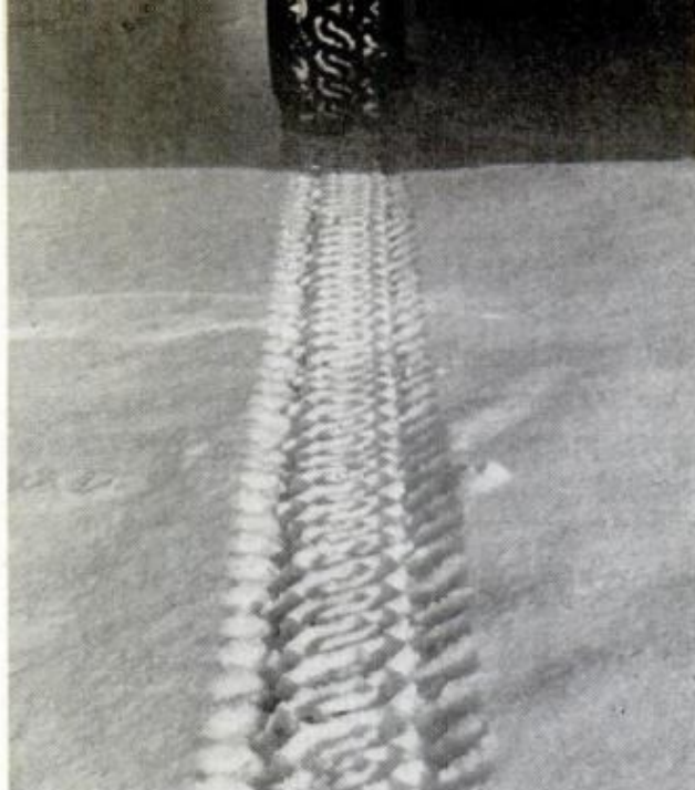
WINTER TREAD with studs bites clean on snow. Studs are mounted only on shoulder of the tire tread
