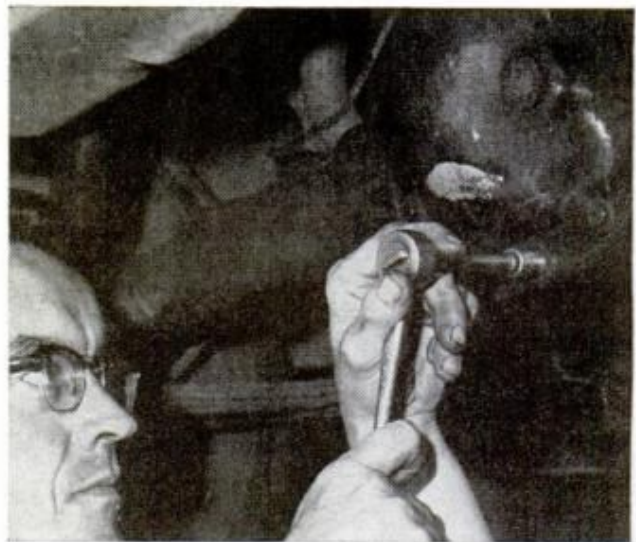
LUBRICANT LEAK caused by a faulty gasket is easily repaired. First step is to remove all the differential cover bolts. Catch remaining lubricant in a pan
