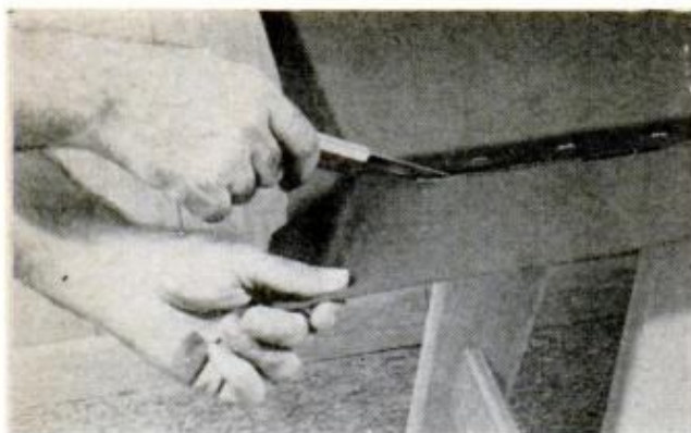
BED CLOTH IS STAPLED around perimeter every inch or so. Knife for trimming should be razor sharp
