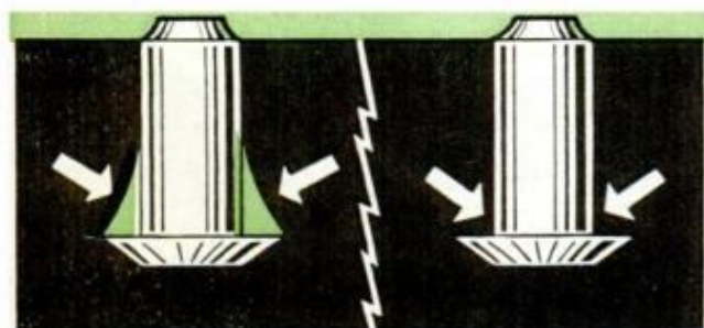
SHOULDER OF STUD SHELL is firmly clenched by rubber when tire is broken in during first 50 miles
