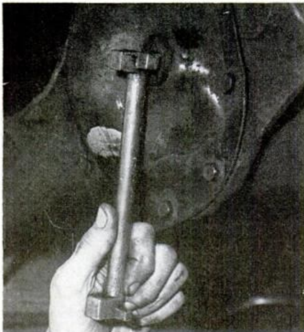
DIFFERENTIAL CASE has a plug in the rear half that may require a special tool for opening. Hole is for checking lubricant, adding when necessary
