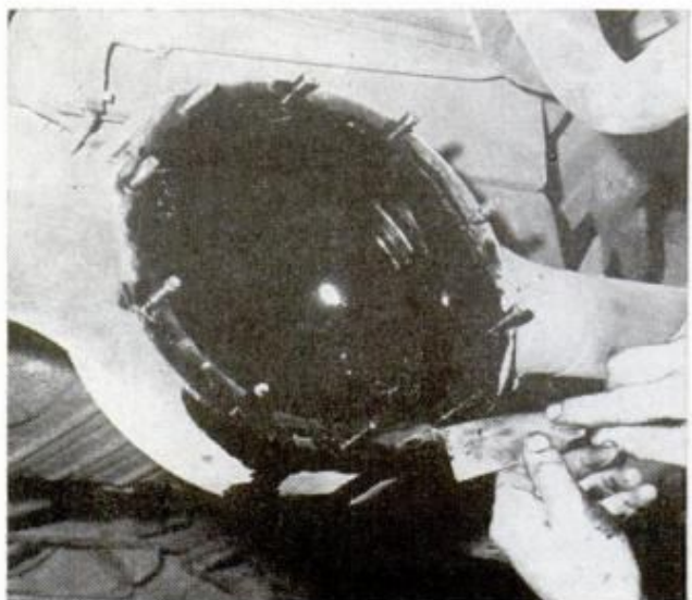
FLANGES of both the differential case and cover are scraped and cleaned thoroughly of pieces of gasket and sealer. Use solvent if necessary; wipe dry
