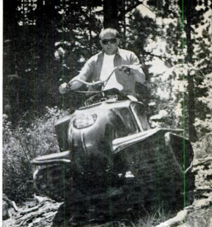
THE EAGLE SKITTERS over rough woods road at better than 30 mph. Battery headlight is for night driving
