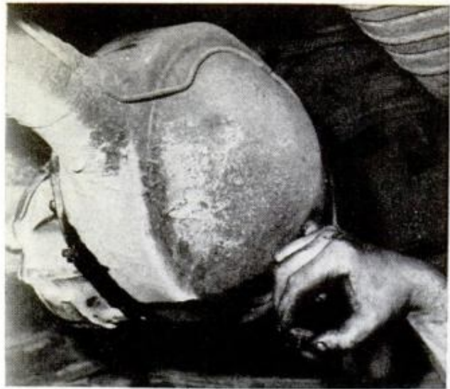
PINKY TEST is used to check lubricant level. The level hole can be used to drain and fill differential case if you have a goosenecked suction gun
