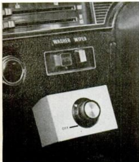
MOUNTED UNDER DASHBOARD, speed control turns wipers on and off and varies the sweep rate with a
