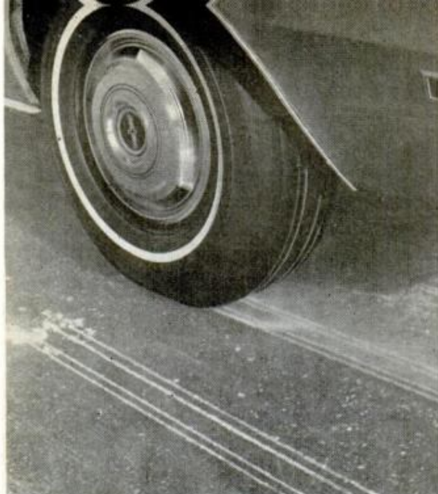
BITE OF STUDS in acceleration gives straight-line start. Bottom tracks were left on ice after stop
