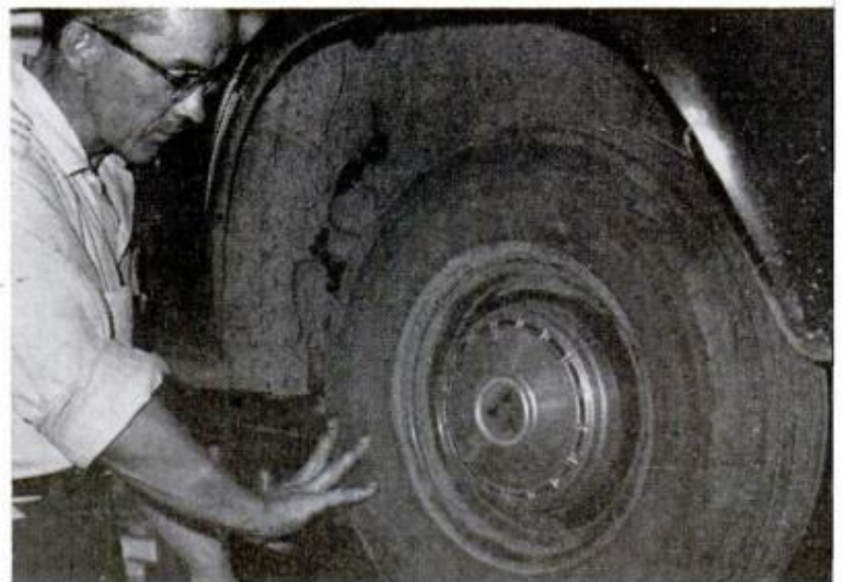
SPIN WHEELS by hand and listen when you suspect that a front-wheel bearing or axle-shaft bearing is causing noise. You may be able to pinpoint trouble
