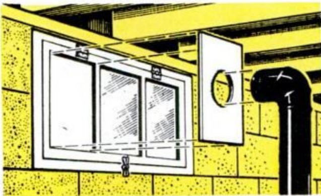
CUTTING A PIPE HOLE through "pane" of asbestos cement when venting a dryer through a basement window is a cinch by making plunge cut in material
