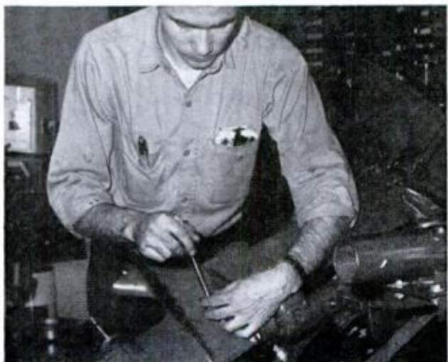
5. REMOVE FASTENERS that hold gearcase to the exhaust housing; place in handy place for reassembly
