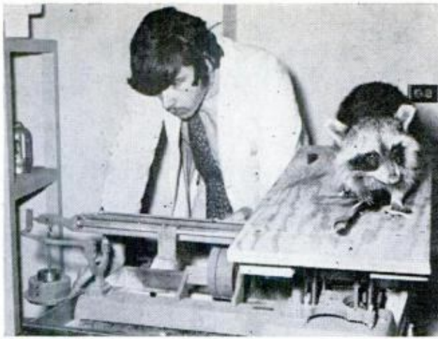
WEIGHT LOSS indicates evaporation of body fluids. Freeze-drying is completed when weight loss stops
