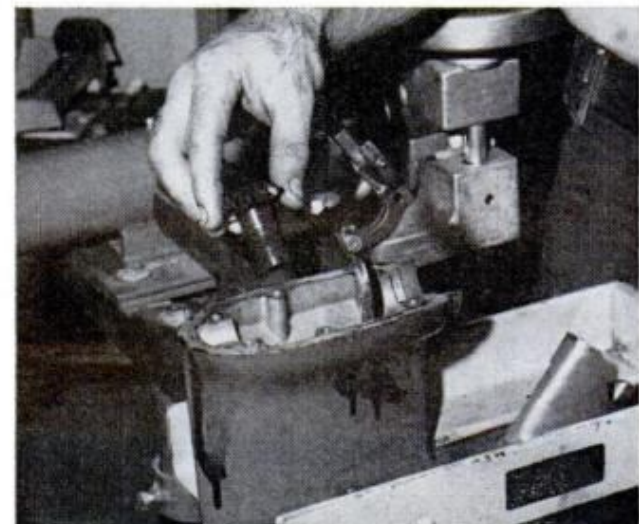
10. EXPOSED GEAR TRAIN , after removal of the skeg
