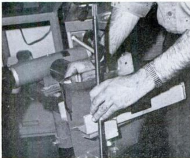
13. REMOVE DRIVESHAFT and, if bent, replace it
