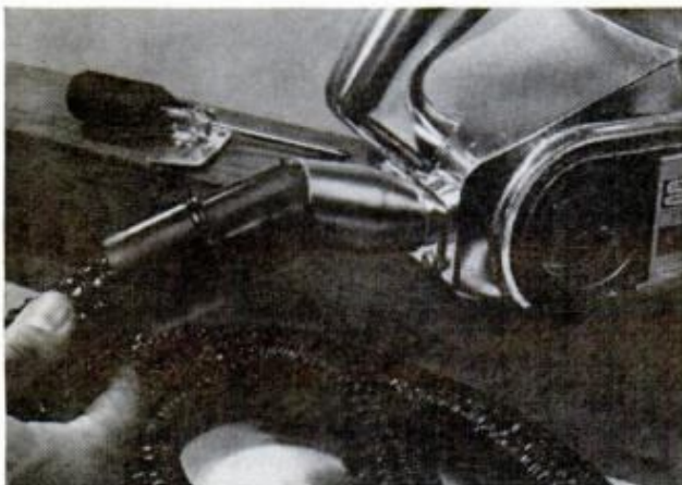
HOSE AND NOZZLE serve as dust collector on the Stanley sander—they're attached to vacuum cleaner
