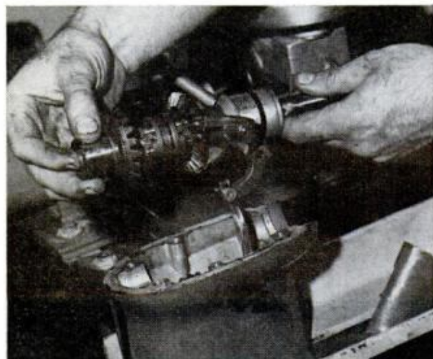
9. REMOVE PIVOT PIN and screws to free the skeg
