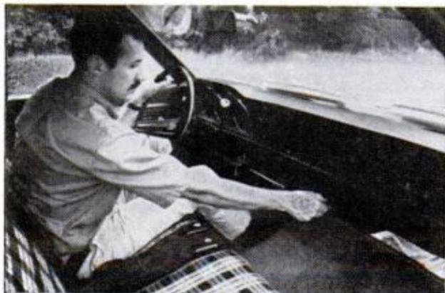
FULL-WIDTH SHELF is no substitute for real glove box which is sorely missed by many Maverick owners
