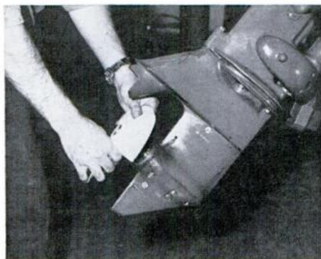
3. BEGIN LOWER-UNIT REPAIR WORK by removing the propeller and draining the gearcase of lubricant
