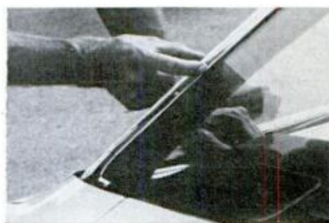
FLUSH-MOUNTED WINDSHIELD is one of several wind-cheaters on the Challenger
