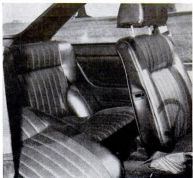
BOTH FRONT SEATS recline and move on long tracks. Legroom is comfortable for driver of any size. Rear seat is well padded but cramped for adults
