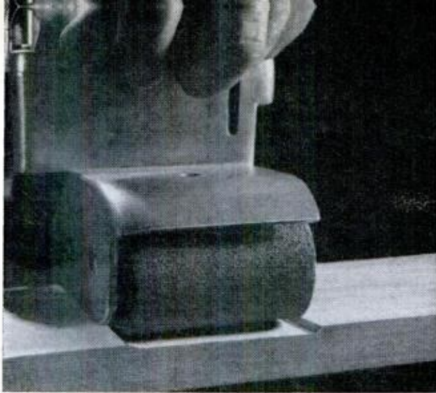
LEFT IN ONE SPOT TOO LONG , belt sander will plow a deep groove (shown across the grain here)
