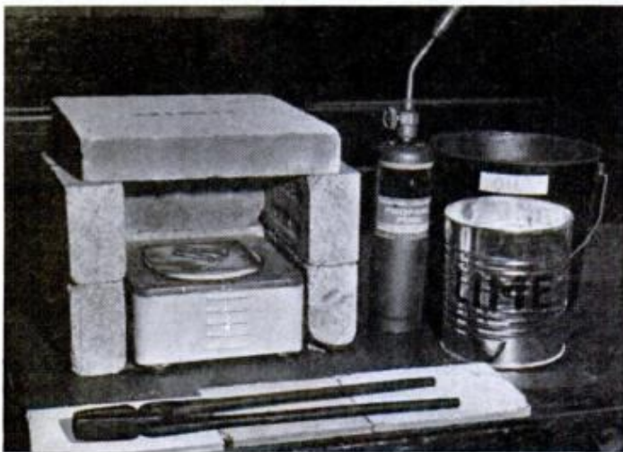
ANNEALING AND HARDENING TOOLS are furnace, torch, oil, dehydrated lime and pair of tongs. Asbestos can be substituted for the oven bricks if necessary
