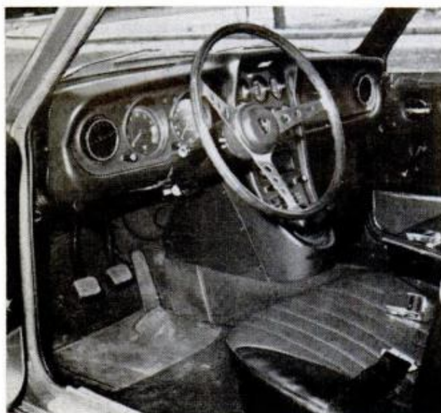
COCKPIT LAYOUT has 8000-rpm tachometer left of speedometer. All other gauges, switches, radio and shift lever are in central pod. Wheel is real wood
