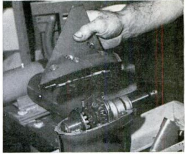
12. REMOVE PINION GEAR , then the thrust washer
