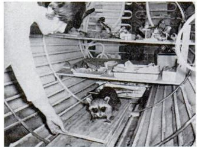
SPECIMENS DRY OUT in chilled vacuum chamber, a key step in process. Drying takes about two weeks
