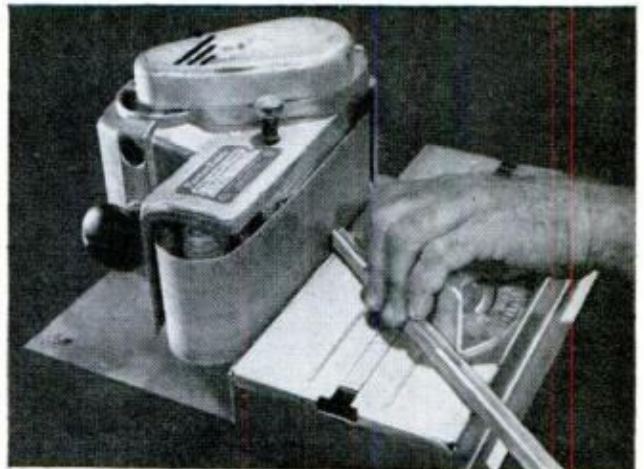
WORKBENCH STAND comes with accurate miter gauge, secures sander. The one shown is by Rockwell
