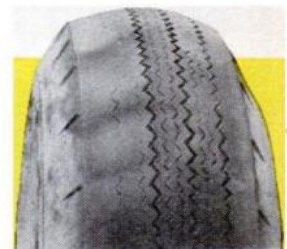
FIG. 9. This tire was ruined in 3000 miles of driving. A combination of worn upper control-arm bushings, loose ball joints and a loose idler arm caused the wear
