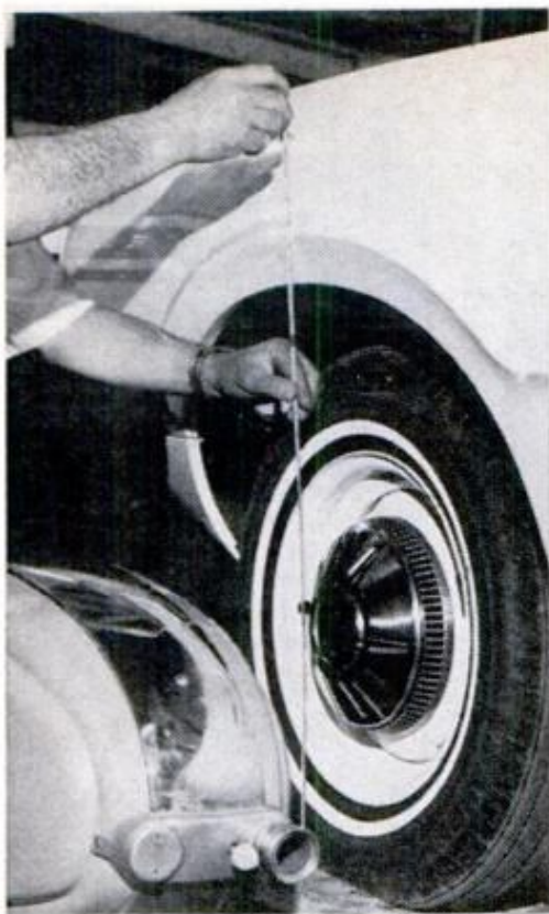
CHECK FOR SAGGING SPRINGS by measuring height to fender well on both sides of car. Check for equal tire pressure first
