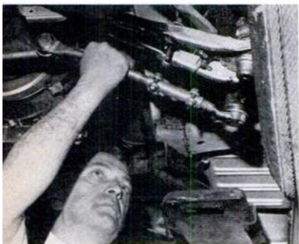
TIE RODS should be checked for play and replaced if any is present. Tie rods are usually split for easier replacement
