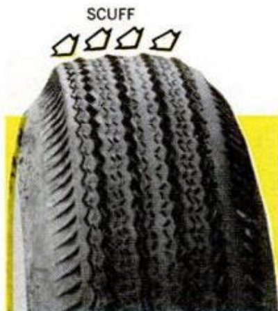
FIG. 4. Scuffing over the entire width of the tire indicates incorrect toe alignment—a constant toe-wear condition. Tread pattern gets a ragged appearance
