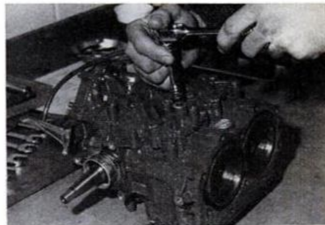
4. TAKE OFF the bypass covers. Once they are removed, you can get an idea of block's condition
