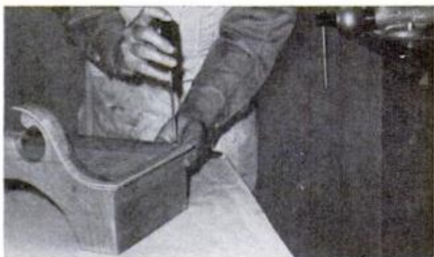
USE SCREWS to fasten top. Moldings along sides are mitered to mate with curved moldings at front
