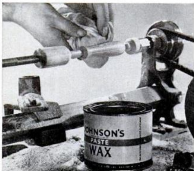
PASTE WAX FINISH is adequate for small turnings. Wipe-on a half-dozen coats and buff each with a rag
