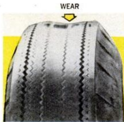
FIG. 2. Excessive wear of the center tread indicates running with tires overinflated. Always check and inflate your tires before driving, while they're cold
