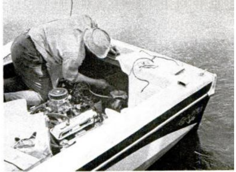
CLEANING OUT THE IMPELLER is easy once you know how—even when pieces of vine wrap around shaft
