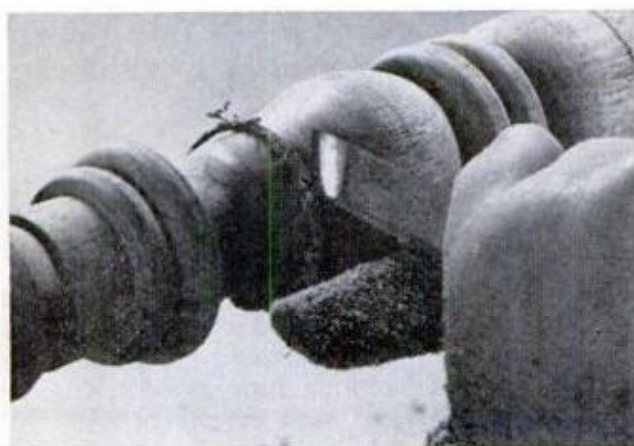
PARING CUTS are made with a skew chisel or gouge angled in such a way that bevel rides on the work
