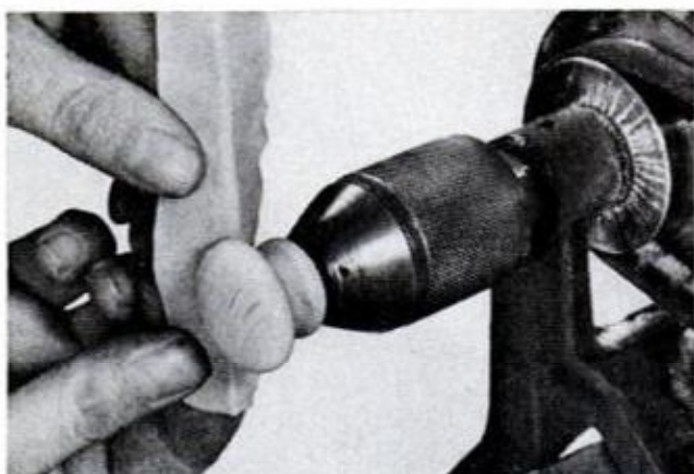
SMALL-DIAMETER WORK can be turned in chuck. Spindle nose on AMT 6-in.-swing lathe has \frac{1}{2} -20 threads
