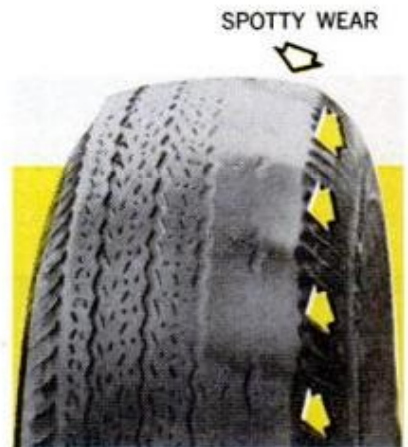
FIG. 6. Tread wear, on the inside or outside edge, that is spotty indicates intermittent camber wear. The characteristic "knotty" wear pattern is very noticeable
