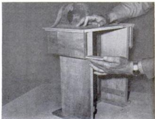
CLOSURE STRIPS slide in and close openings between pediment and hood. Hood is now fixed in place
