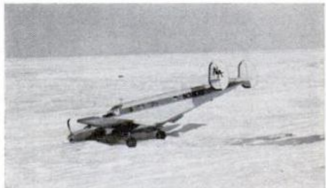
COLLAPSED NOSE WHEEL made this plane a casualty on landing at Slope. Landing is risky part of trip
