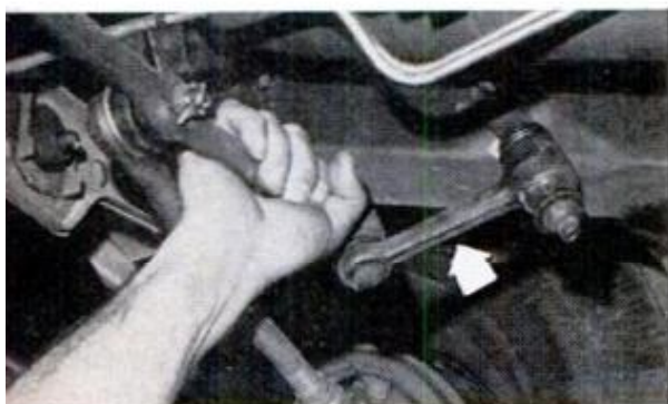
STEERING IDLER ARM (arrow) can be tested for play by twisting it and adjacent rods
