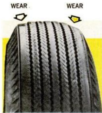
FIG. 1. Excessive wear on the outside edges of any of your four tires indicates they've been running with insufficient air pressure. Check the pressure every week
