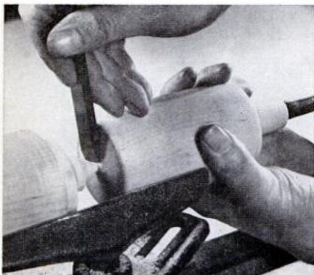
TO CUT OFF finished turning, make deep V-cuts to leave but \frac{1}{8} in., stop lathe, finish with handsaw
