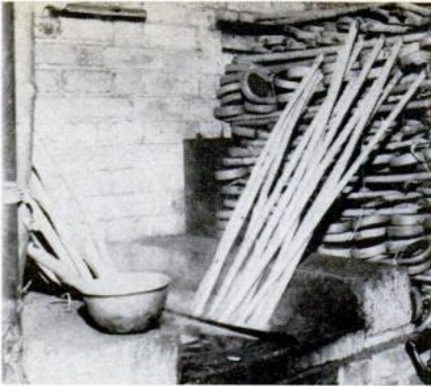
1. STICKS ARE BOILED , then soaked in preservative
