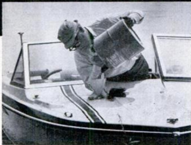
FILLING from reserve gas cans aboard is quite easy. The bow tank holds 18 gallons, which last for a day
