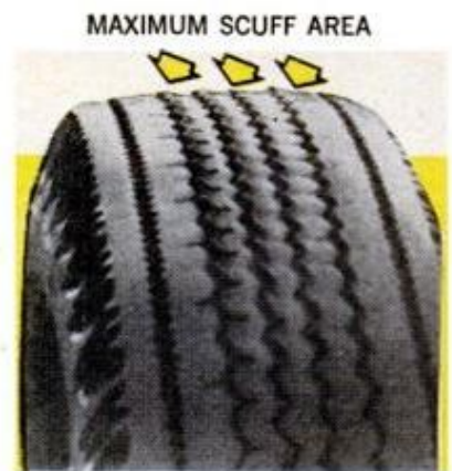
FIG. 3. Center tread scuffed, as opposed to evenly worn as with overinflation, is a sure indication of intermittent toe wear. Cause is damaged front-end part
