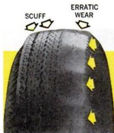
FIG. 8. Erratic wear on one side and sharp, feather edges worn on the other indicate loose suspension part (here, a control arm) and excessive toe-out condition
