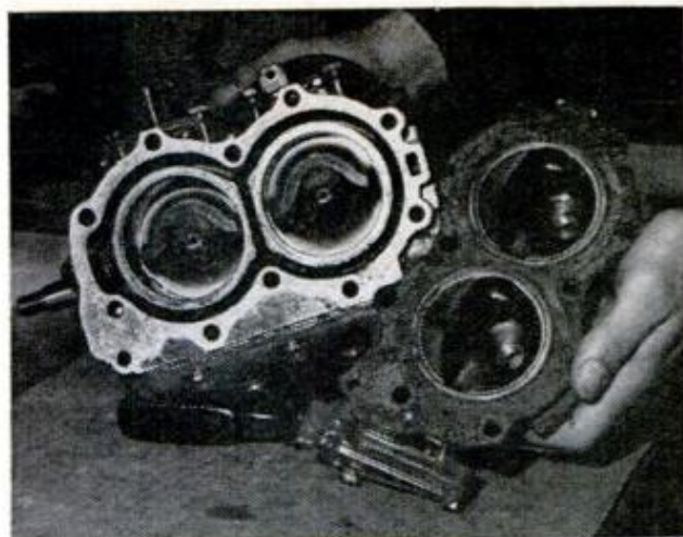
6. WITH CYLINDER HEAD removed, examine tops of pistons, part of cylinder wall and all of cylinder head
