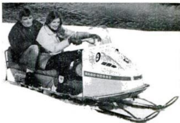
JOHNSON'S SKEE-HORSE comes in two basic 25-hp models. This Light-Trac model sports a 15½-in. track while the Wide-Trac model has one of 20½-in.
