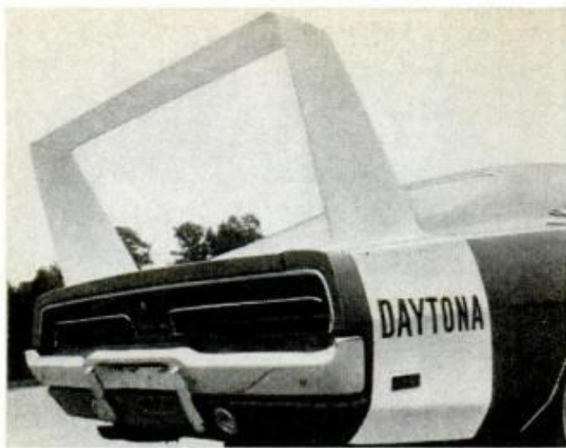
SPOILER on Dodge Charger Daytona is engineered to help hold car's rear end down at 200-plus mph racing speeds. It's also great for drying wet bathing suits
