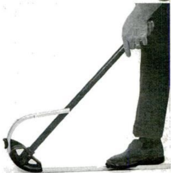
HICKEY IS PLACED on bend-start mark (top), and pressure applied. At finish mark bend is 90°. To bend 180°, pipe passes handle, must be straightened
