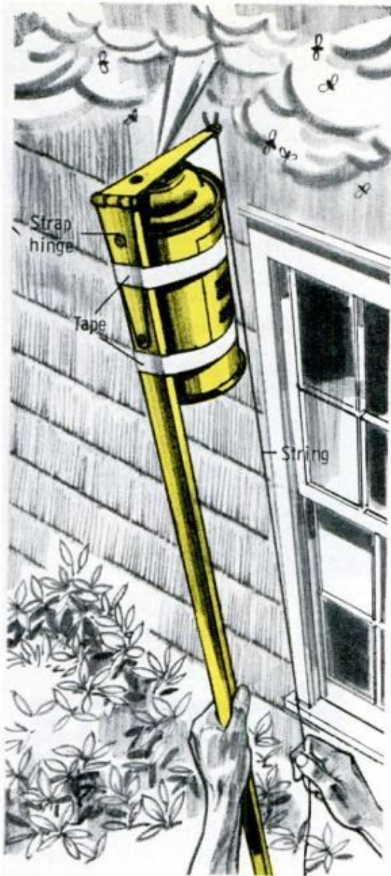
TO REACH HORNET'S NEST under eave attach strap hinge and spray can to pole. String to hinge runs spray.— B. R. Alexander
