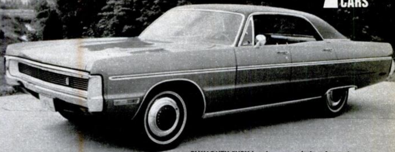
PLYMOUTH FURY has been restyled up front via new bumper, grille. Car's longer, the rear track wider
