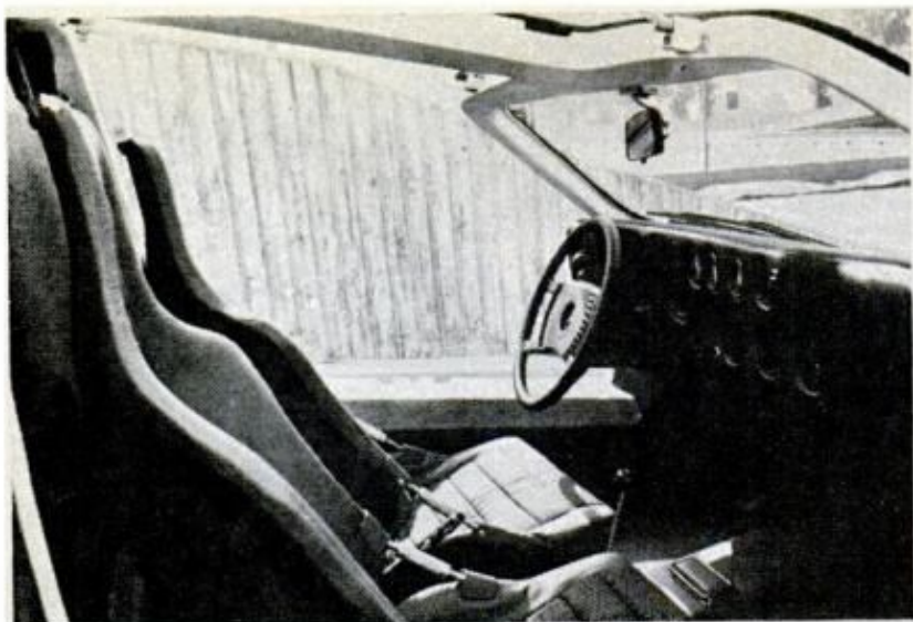
STRIKING INTERIOR is at once all function and all luxury. The seats have turnbuckle adjustable rake and extraordinary lateral support
