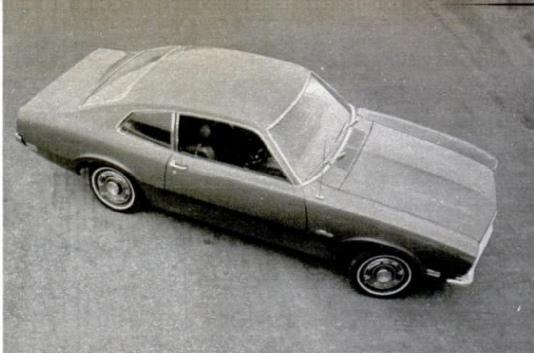
FORD MAVERICK remains the same as when introduced last spring—a two-door fastback powered by either the standard 170-CID Six or optional 200-CID Six
