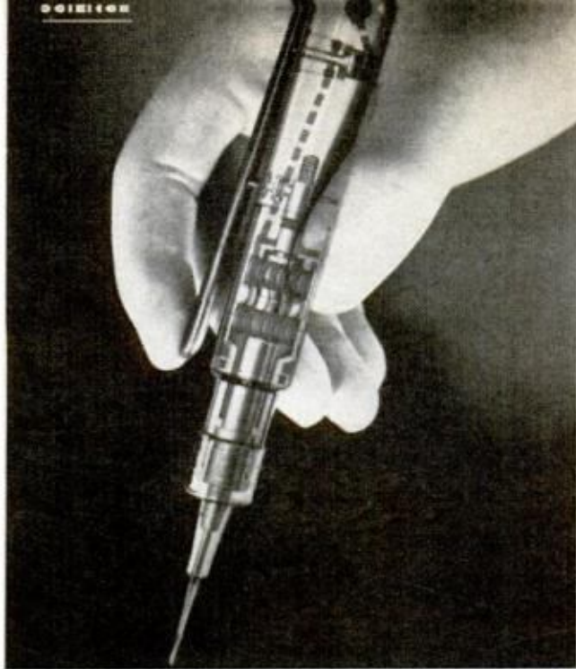
FINGER-TIP THROTTLE (left) gives surgeon precise control. Brake stops drill in two seconds
