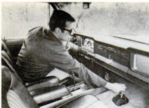
4WD CONTROL LEVER has shift pattern outlined on knob; some find it hard to shift to 4wd low range
