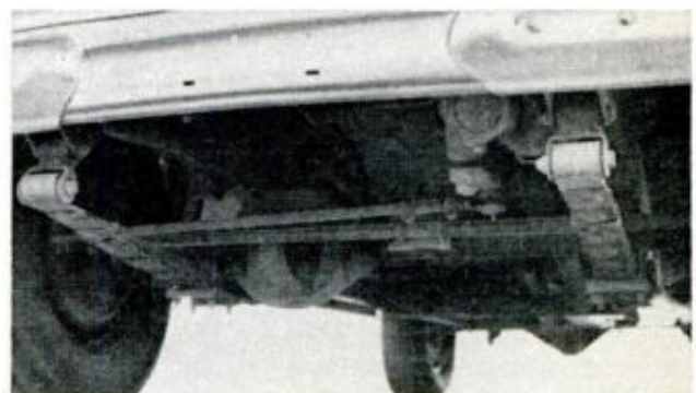
TRANSFER CASE between leaf-spring suspension puts power to front wheels at 1:1 and 2.03:1 ratios
