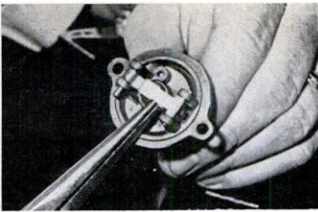
7. BEND the lower float-arm lever to make any adjustments to the float level on fixed-jet carbs
