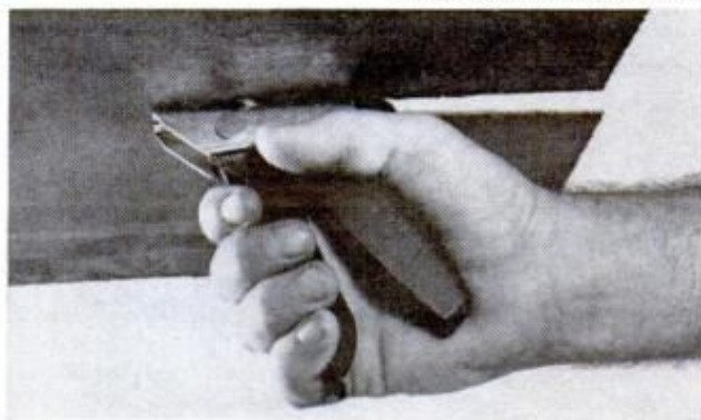
CUTTER STAYS BELOW WORK (Formica used here). Aluminum anvils must remain parallel to the work
