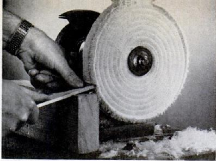
RAKING A NEW BUFF with a sharp-edged steel bar cleans the cloth and frays the wheel's periphery. Rerake the wheel thoroughly whenever you switch from coarse to fine compounds
