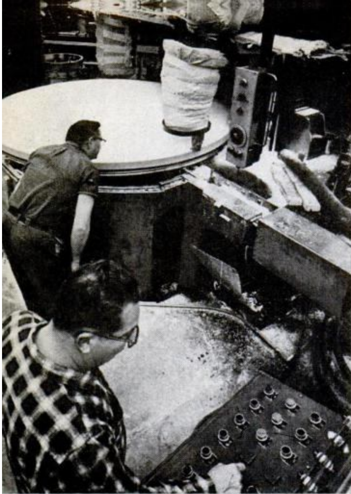
SUPER-SMOOTH FINISH is required for heat shield of Gemini space vehicle, shown (left) being machined with diamond tool. Photo above shows copper wire for electronic watches drawn through battery of diamond dies to reduce it to required fineness. Die holes are measured in millionths of an inch
