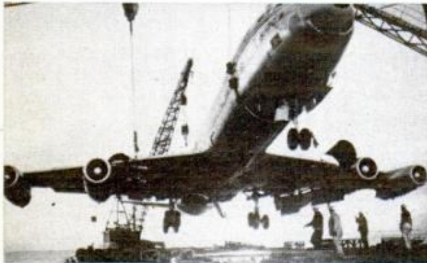
NOSE HARNESS and lifting beams carry full weight of plane as it is swung by cranes to waiting barge
