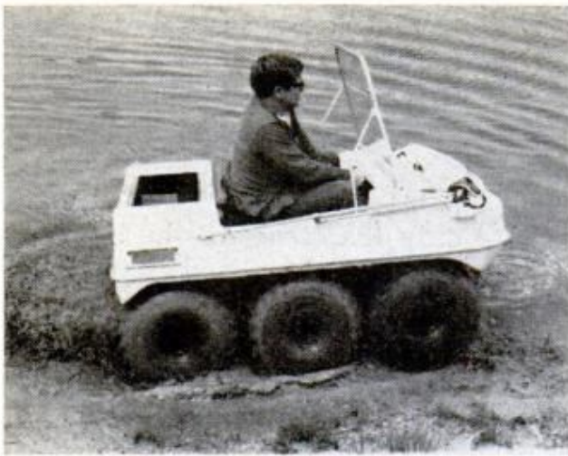
AT WATER'S EDGE , this machine moves well, depending on how muddy the terrain and how steep the bank
