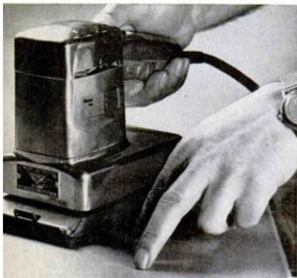
ALUMINUM OR FLAT-BRASS STOCK can be polished ready for buffing with well-worn, fine-grit cloth in orbital sander
