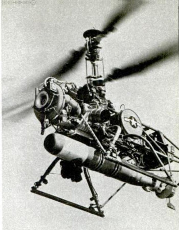
NAVY'S NEW MK 46, a solid-rocket-propellant torpedo, is carried by a drone helicopter in test at sea
