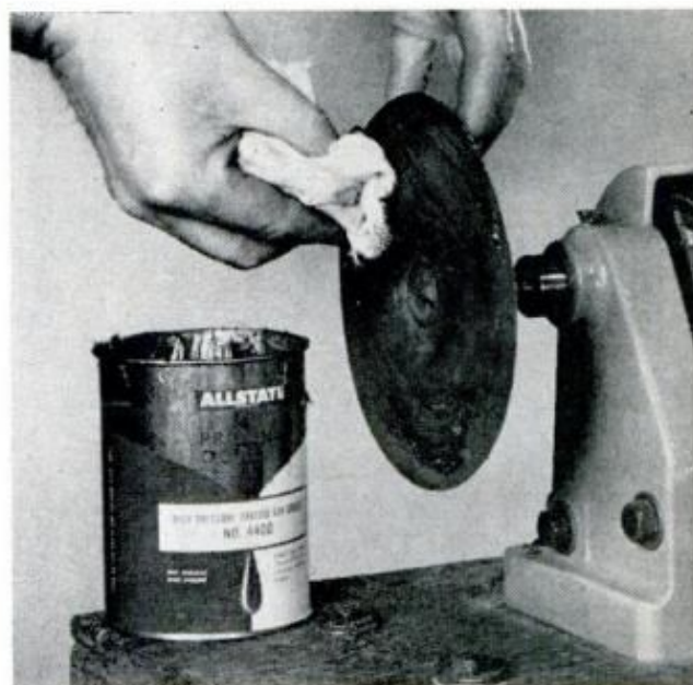
GREASED ABRASIVE CLOTH gives metal a much higher shine than same cloth used dry. Apply grease stick or chassis grease, regreasing wheel frequently
