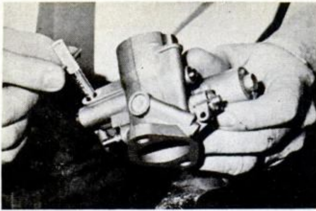
5. REMOVE fixed-jet by uncovering and unscrewing with a fixed-jet tool or an exact-size screwdriver
