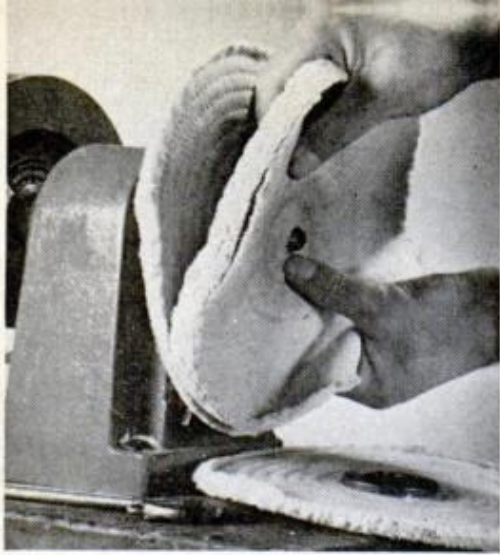
MUSLIN BUFFS come spiral sewed or unstitched. Loose buff sandwiched between sewed buffs makes wheel for heavy work
