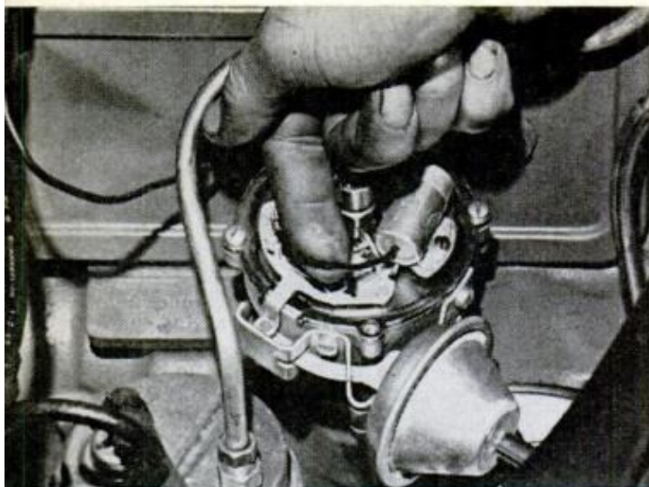
CHECK PIGTAIL of the condenser for solid insulation. If bare wire grounds against the distributor body, you won't start. See text for another really hidden no-start condition due to "cold condenser"
