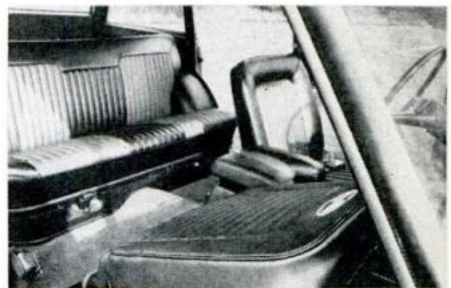
REAR SEAT in the upright position is held by two spring-loaded pins which rattle and are hard to use
