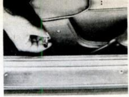
MONEY-SAVING DESIGN places seat-back release at floor level. Owners would pay to raise it
