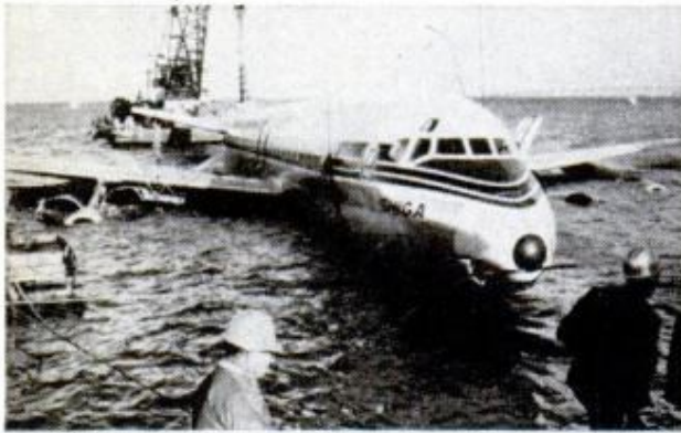
LIFTING BEAMS under the wings are in place and barge-mounted cranes start to lift Shiga from water
