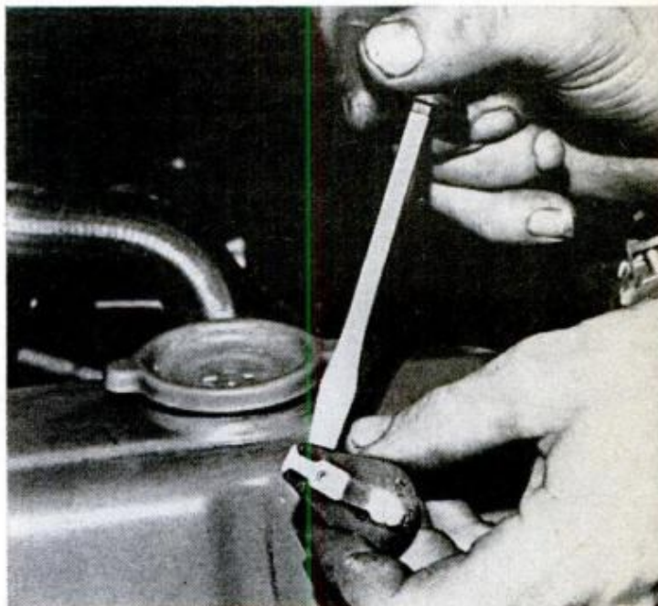
ROTOR should be pulled and inspected carefully, especially to check that metal contact is not misaligned, loose or damaged. Also, on either side of the top inspect flanges which sometimes break off
