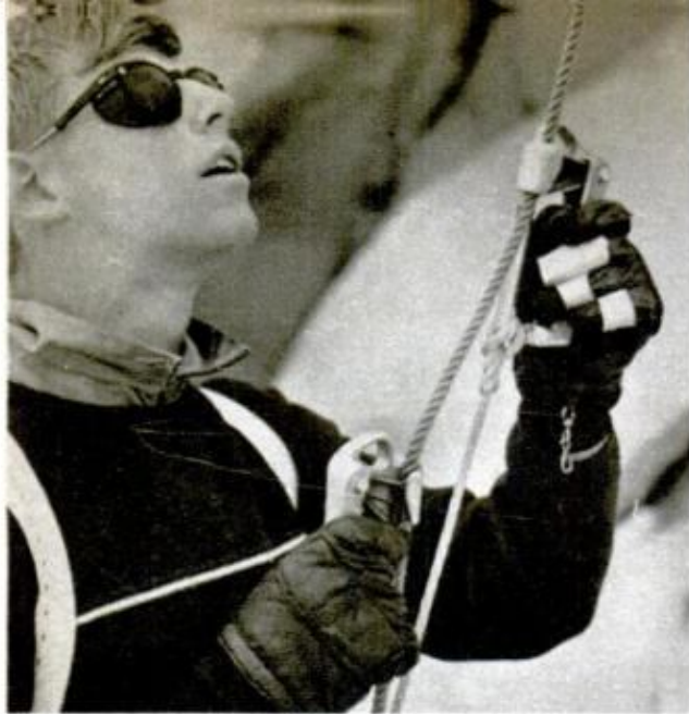
THE JUMAR ASCENDER is an important new device used by mountain climbers to get up and down guide ropes more easily. It was developed in Switzerland
