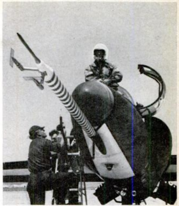
SENSITIVE VANES at end of 8-foot boom register wind velocities in this high-flying CAT-hunting U-2
