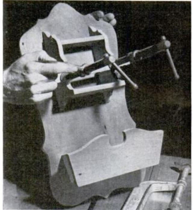
POSITION THE CLOCK SHELF 3\frac{3}{4} in. down from the top and attach it to plaque with flat-headed screws
