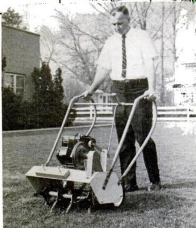
THIS AERIFYING MACHINE has "spoons" that scoop out cores of soil in manner shown in diagram above
