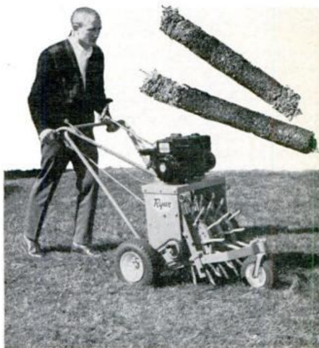
AERIFYING MACHINE penetrates up to 2½ in. on 5-in. centers, to cut out soil plugs like those above
