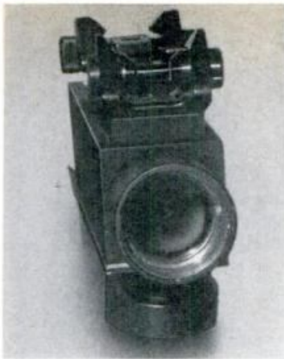
FRONT (lens) end of transmitter. Case contains battery power pack
