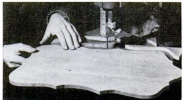
BAND OR JIGSAW makes quick work of sawing out plaque and the three other scroll-cut parts required
