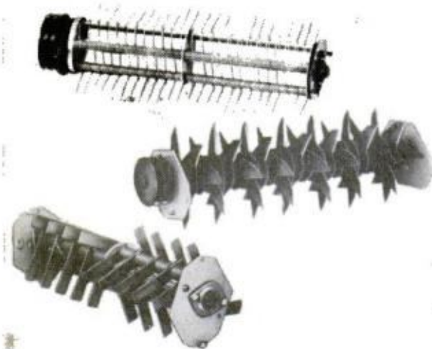
THIS DE-THATCHING MACHINE comes equipped with three interchangeable reels: tine, knife and flail, which are pictured in that order below the machine
