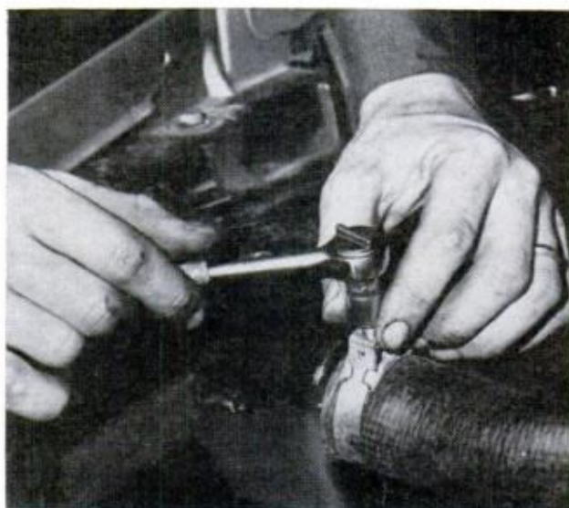
HOSE CLAMPS , if they are the screw-down type, should be tight for a good connection. Using a ratchet wrench is easier than using a screwdriver
