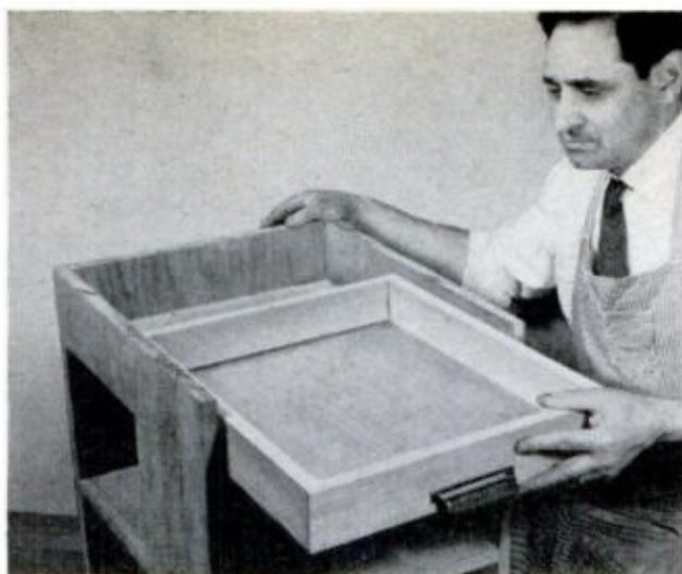
SHALLOW DRAWER is made to fit compartment. Side clearance, plus wax, will make drawer slide freely
