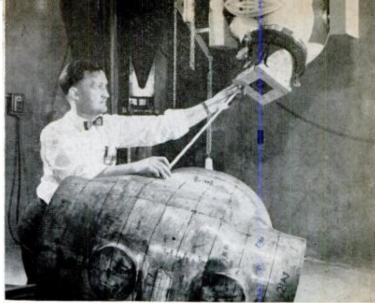
A GIANT VALVE for a high-pressure pipeline is X-rayed in same way as a dentist X-rays your teeth. Defects appear as dark spots on film—just like cavities
