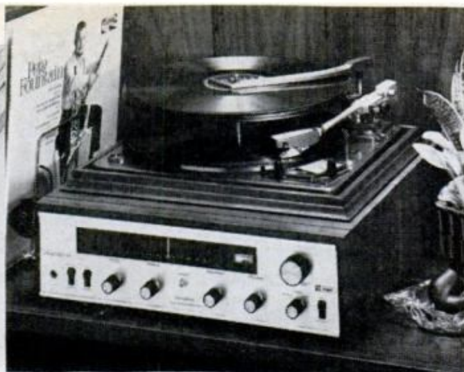
RECORD CHANGER and FM/FM-stereo receiver are stacked together in a space-saving piggyback design in this Knight-Kit compact by Allied. Wiring is simplified by printed-circuit boards and easily joined subassemblies (upper left)
