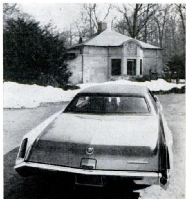
KNEE-KNOCKER bumper and taillight protrusions and the limited rear visibility are accentuated here
