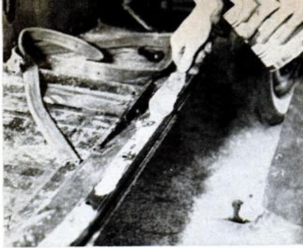
WEATHERPROOF RUBBER STRIP should be renewed, if necessary, to insure dry and comfortable rides
