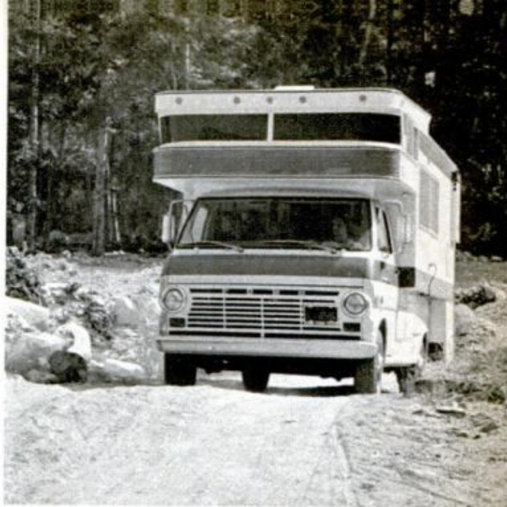
GROUND CLEARANCE is important. It can vary from 4 inches on sedans to 11 inches on pickups and vans
