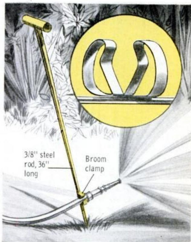
GROUND SPIKE HANDLE lets you move hose without stooping when watering flowerbeds. Consists of 3-ft. pointed rod with a broom clamp riveted 8 in. from end. Hose snaps securely in clamp.—William Waggoner
