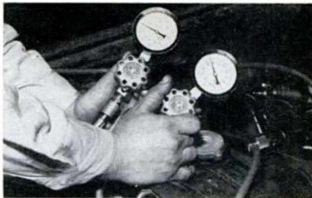
SYSTEM IS DISCHARGED by opening high and low-pressure valves of gauge set; gauges drop to zero
