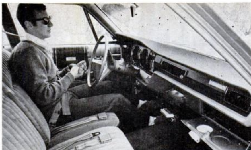
SPLIT FRONT SEAT combines advantage of bench, comfort and convenience of individually adjustable buckets. Ashtray is hard to use for some owners
