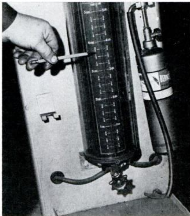
PROFESSIONAL EQUIPMENT , above, makes recharging easy. Right amount of refrigerant is measured out
