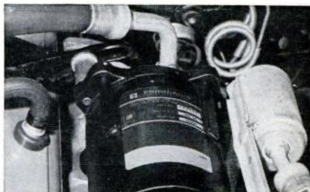
COMPRESSOR NAMEPLATE identifies manufacturer, gives amount of refrigerant charge, test pressures
