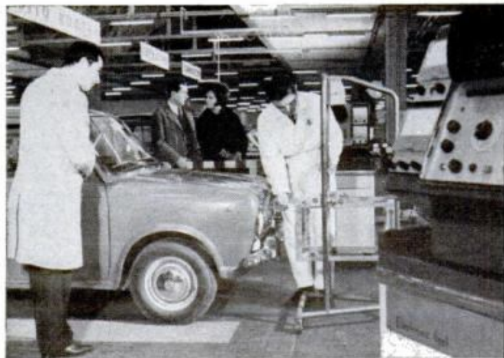
HEADLIGHT ALIGNMENT is set while customer looks on. Most of service is while-you-wait or one-day
