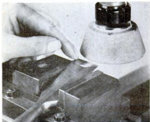
TO GRIND CUTTING EDGES with a cup wheel, use 1700-2500-rpm speed, take light cuts to avoid burning
