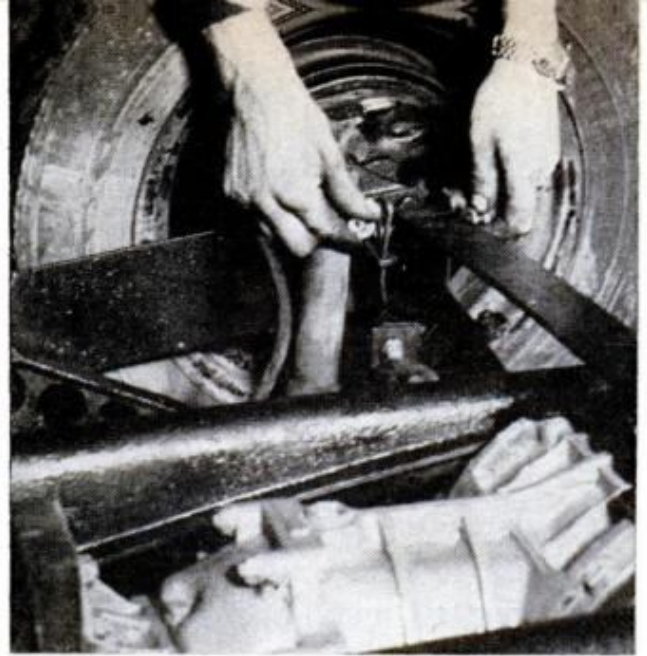
REAR CAMBER COMPENSATOR is bolted to the transmission housing, and then to independent axles
