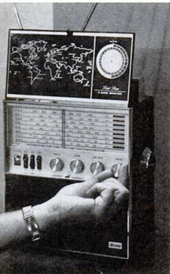
LARGE DIAL on Allied's new wide-range portable makes it easy to tune any of eight separate receiving bands. On flip-up lid is a world map and time-zone indicator. For portable use, the set runs on four flashlight batteries in a handy clip (below)
