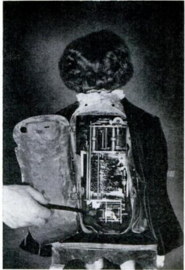
"SPINAL COLUMN" of the writer consists of cams and pegs controlling wrist motions to form letters
