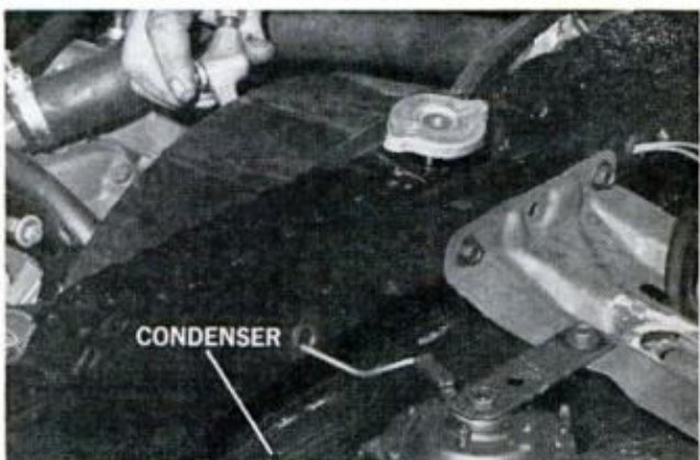
CONDENSER is ahead of radiator. Clean out debris by blowing compressed air through both from rear
