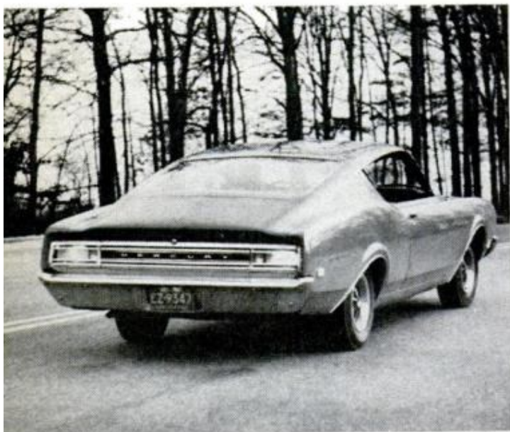
FASTBACK STYLE of Cyclone poses difficulties for owners. Rear visibility is limited, rear seat puts passengers up tight physically and headroom is scant
