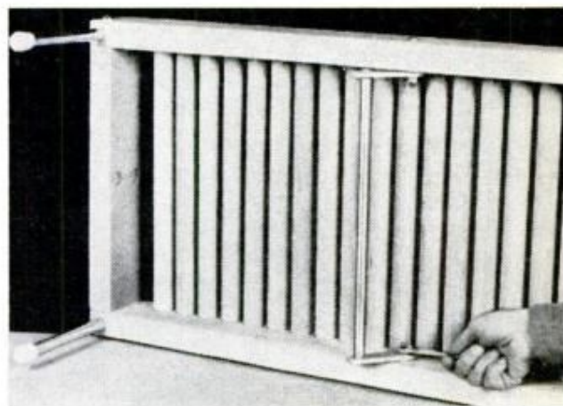
BELT TENSION IS REGULATED by moving bar toward or away from rollers and locking by tightening bolts
