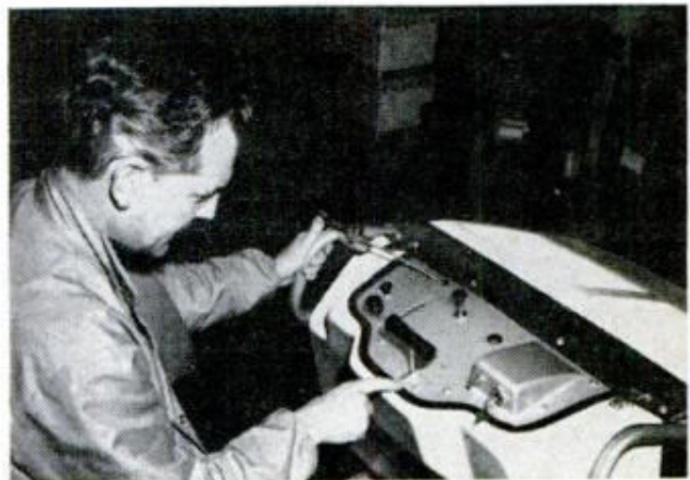
OPERATIONAL CONTROL of ATV is via single T-handle mounted on dash directly in front of driver
