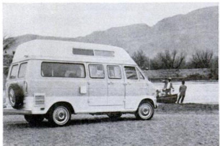
FIBERGLASS TOP has sliding, screened windows both sides. Water heater is at lower left; space heater next to door
