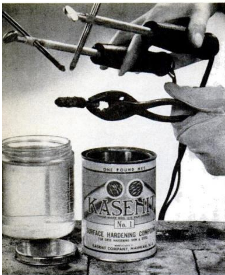
CASE-HARDEN MILD STEEL by heating it until red hot, then fuse on carburizing compound and quench
