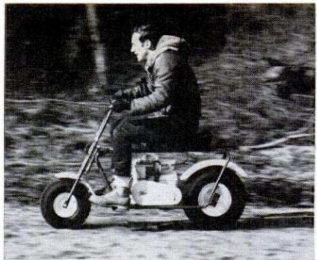
BIKE MOVES at 30 mph in high gear; 15 mph in low. A five-inch internal expanding rear brake stops it
