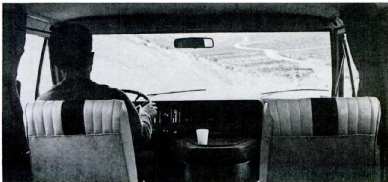
STABLE RIDE is demonstrated by cup on engine shroud. Insulation against engine heat and noise is excellent
