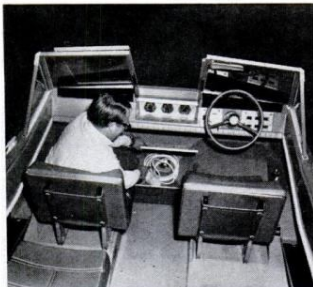
STORAGE COMPARTMENT between seats is good for a small anchor, line and other nautical items. Note positioning of gauges to the left of the driver's seat
