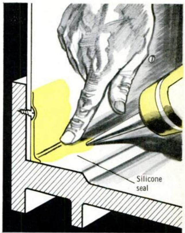
TO STOP RUST FORMING on bottom edge of metal shower stall, wipe joint dry where sides meet plastic base and apply 1/4-in. layer of GE's silicone. Run a bead all around base with finger.— John Goffin
