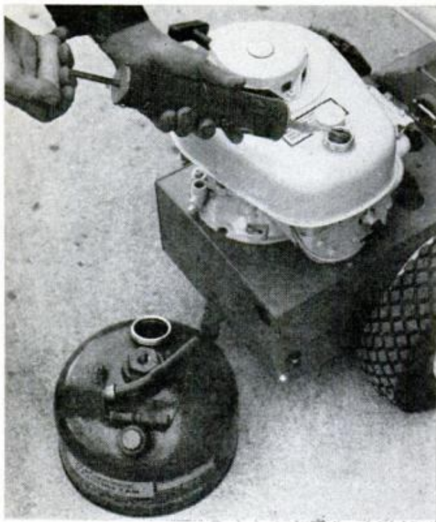
DRAWING UP ON PUMP HANDLE will suck leftover gas from power mower when storing it for winter
