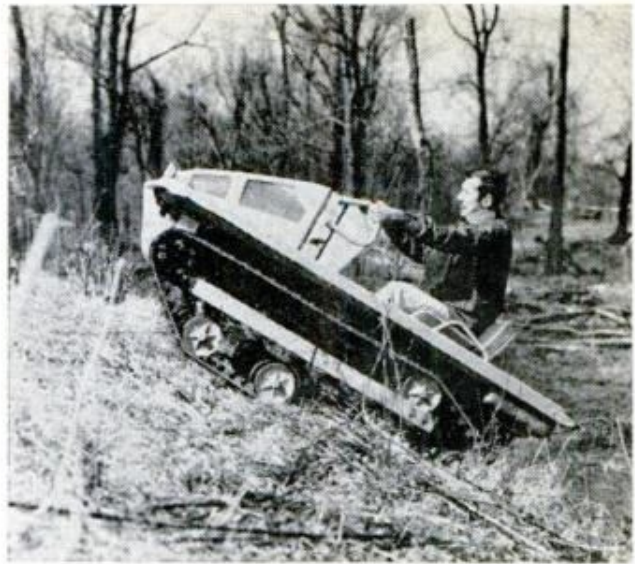
OMC ATV goes uphill through stumps, over brush. If bottom is cleared, rubber tracks will climb stumps
