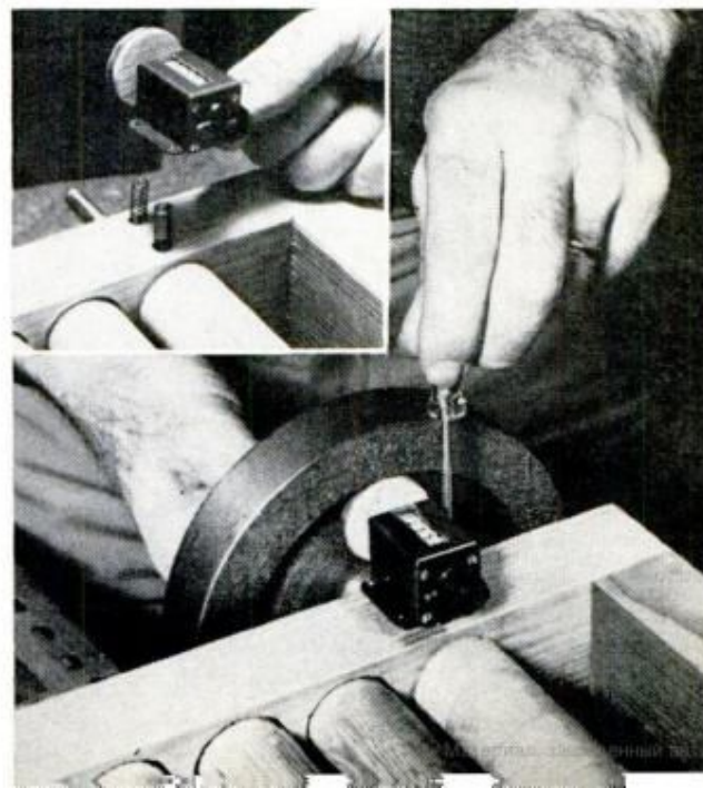
SPRINGS UNDER PEDIOMETER keep rubber-faced pulley riding against recessed rim of cast-iron flywheel
