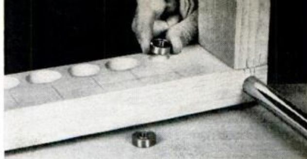
SHAFTS OF END ROLLERS turn in ball bearings seated flush in counterbored holes drilled ½ in. deep
