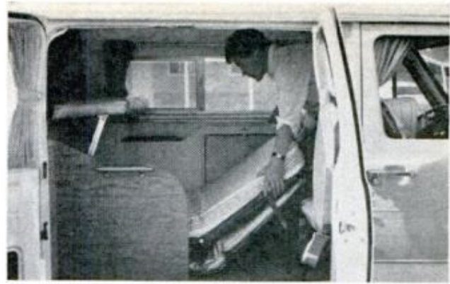
REAL BED WITH FOAM MATTRESS folds out of lounge. Seatback locks in position to serve as night table
