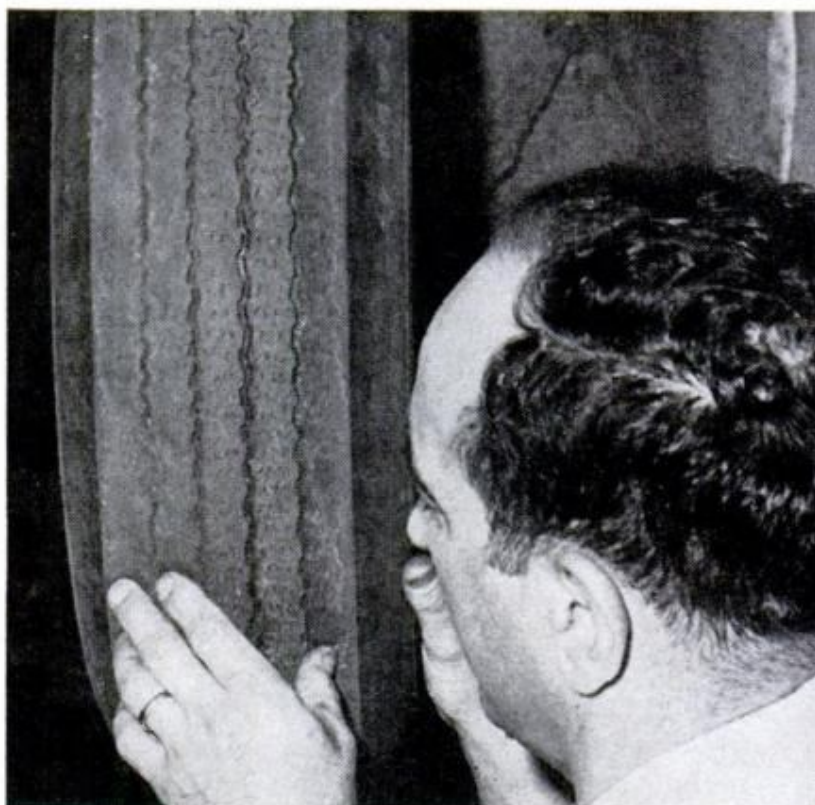
TIRES are the obvious rubber on your automobile and most likely to get your regular attention. Keep an eye out for cuts, gouges, depth of tread and uneven wear as shown above. The greater rate of wear on the inside of this tire indicates a problem of faulty camber which needs correcting
