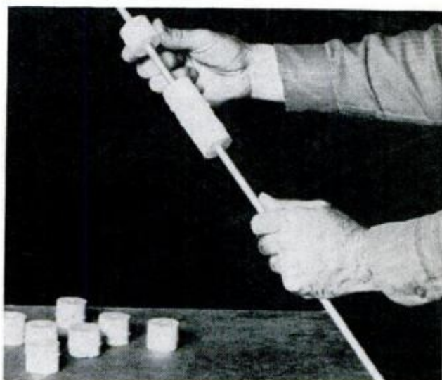
EACH END ROLLER is made by slipping 21 wooden plugs (cut with a hole saw) on a \frac{3}{8} -in. steel shaft
