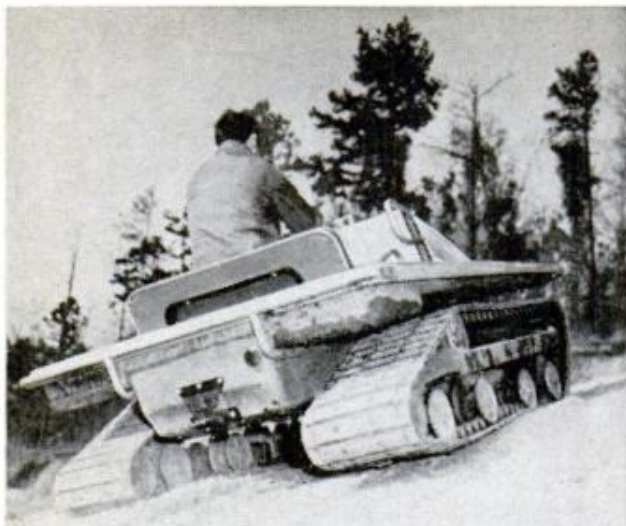
GREEN MACHINE will run on top of deep snow. Its tracks also have outstanding traction on icy glaze
