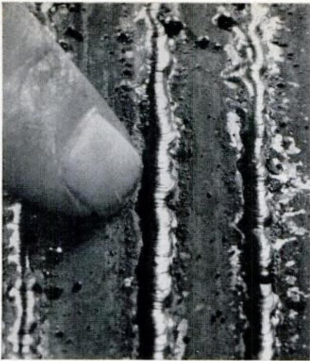
RUN PRACTICE BEADS on 1/16-in.-thick steel to learn knack of welding with flux-coated electrodes
