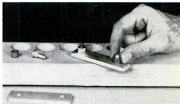
BELT-TENSION BAR (which is tubing) spins on two bronze bearings slipped over ends of splined bolts
