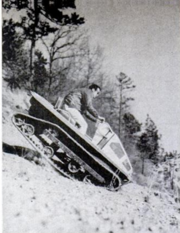
GREEN MACHINE will run on top of deep snow. Its tracks also have outstanding traction on icy glaze
