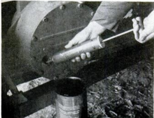
PUMP BECOMES GREASE GUN by filling cartridge with lubricant and squirting it out tapered nozzle
