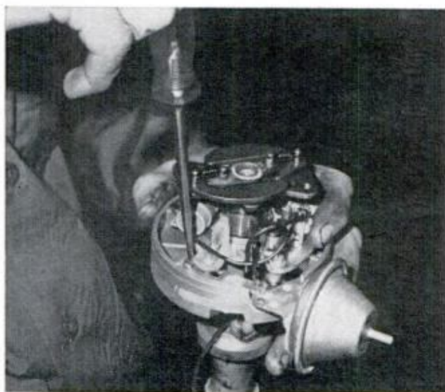
FAULTY VACUUM ADVANCE UNIT is easily removed from distributor body after body is taken off engine. Replace only with a new unit specified for your car
