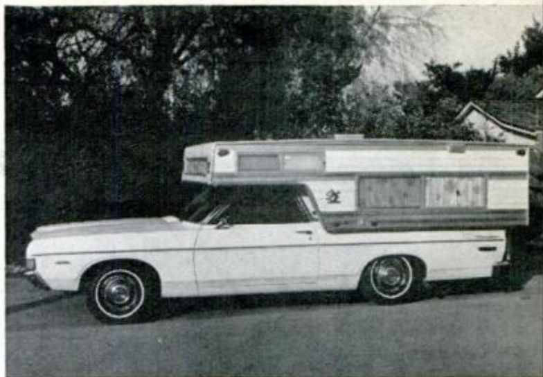
SIESTA'S TELESCOPING CAB-OVER is for the sleek Ranchero pickup. Roof of the unit is 6 ft. from ground in the lowered position, offers 6-ft. headroom when it's raised. A single hand crank is used to operate the roof
