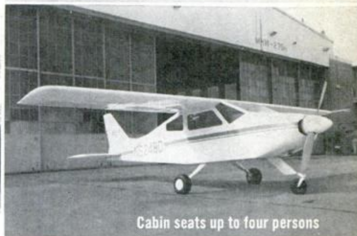
BD-4 with 150-hp engine cruises at 166 mph
