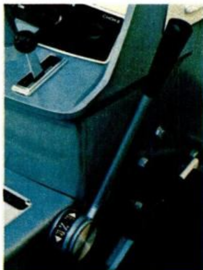
Cockpit has grouped instrument panel: Single Lever Control for no-effort tractoring, visual gas gauge, and cigarette lighter.
