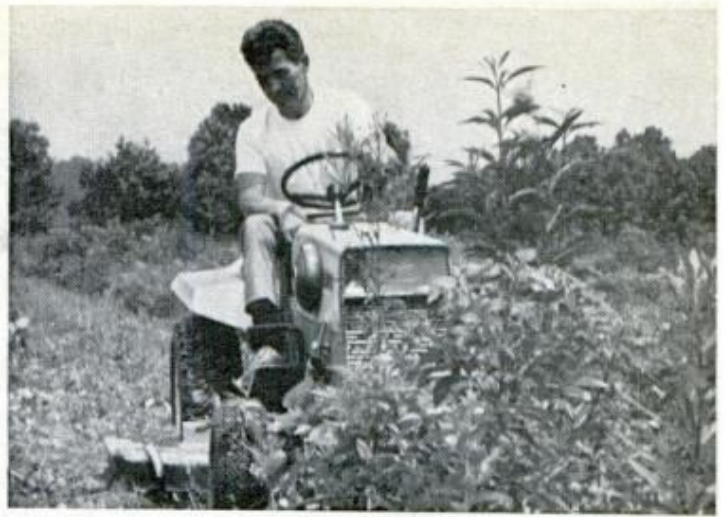
ABANDONED RAILROAD SIDING next to Case plant (left) is used to bump-test tractors. A Gravely 424 with standard mower chews its way through tall weeds in test of shock loads expected when customers mow overgrown vacant lots
