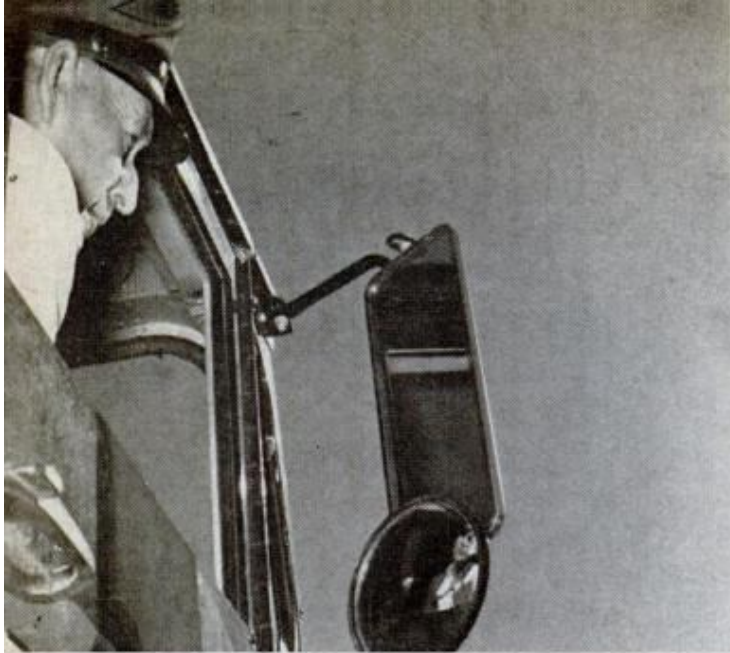
DOUBLE MIRROR ARRANGEMENT on right side of Carolina Line tractor minimizes blind spots—standard and convex mirrors give close, distant vision
