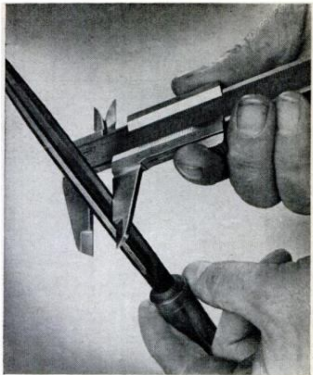
USE SPECIAL CARE when measuring hardened-steel cutting tools to prevent damage to the caliper's jaws
