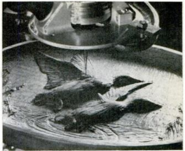
FINAL FINE-LINE CARVING is done with a pointed cutter after roughing-down blank with large cutter
