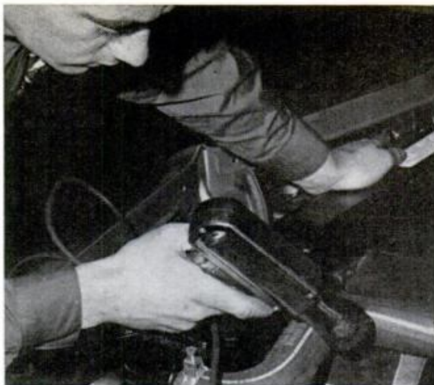
TIMING LIGHT is aimed at timing mark on pulley; if adjustment is necessary, turn distributor body to advance or retard the ignition timing (see text)
