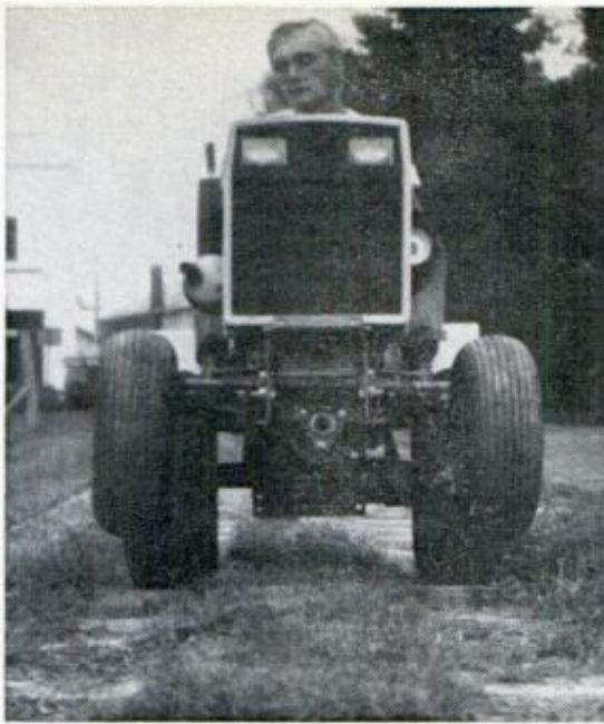
ABANDONED RAILROAD SIDING next to Case plant (left) is used to bump-test tractors. A Gravely 424 with standard mower chews its way through tall weeds in test of shock loads expected when customers mow overgrown vacant lots
