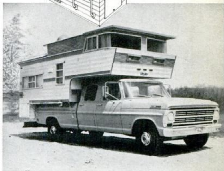
DEL REY'S IMPERIAL SKYLOUNGE is a cab-over coach designed to match crew-cab pickup trucks. The Skylounge (photo above and cutaway) comes in three different interior layouts. It's planned for big-family use
