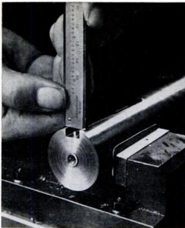
DEPTHS CAN BE MEASURED with the sliding jaw or rod on end of caliper beam. Vernier indicates reading
