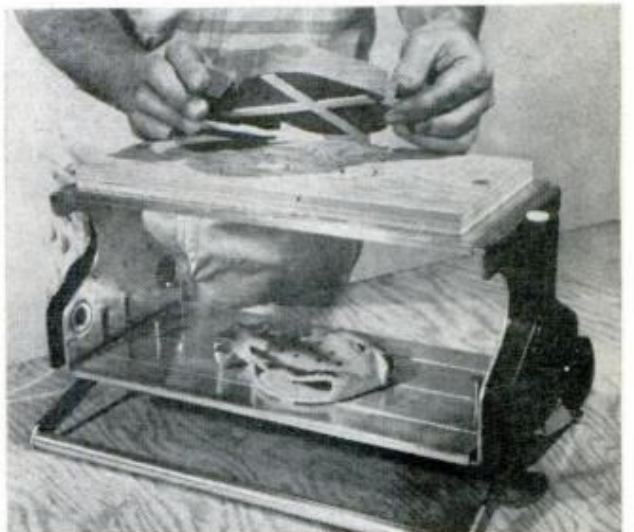
BLANK IS STUCK to top of table, pattern to bottom. Protective wood carving surface is added to top
