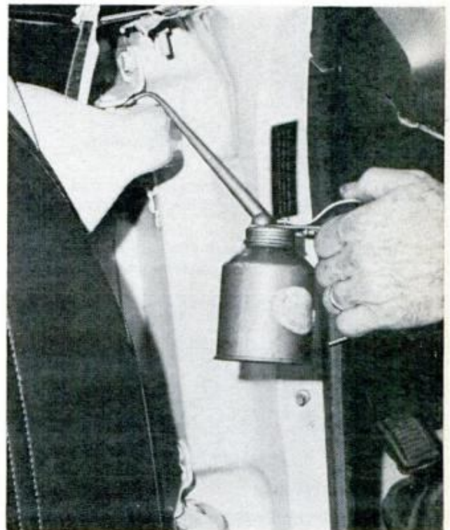
OIL CAN with long, curved, needle-nosed spout puts oil right where you want it. SAE 20 is best viscosity to use in places where complete penetration is needed for lubrication, as with hinge pins
