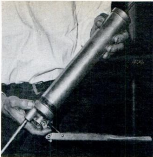
GREASE GUN CAP is screwed on after cartridge is inserted. Plunger forces grease out of gun under high pressure—approximately 10,000 p.s.i. is required
