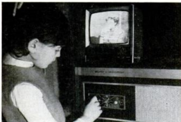
BUILT-IN MONITOR is an added feature on this compact Sony VTR. Below screen is automatic timer
