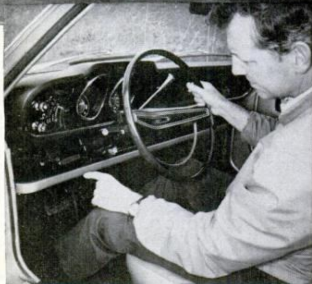
A PACKAGE TRAY is slung beneath the Maverick's dash panel in lieu of standard glove compartment
