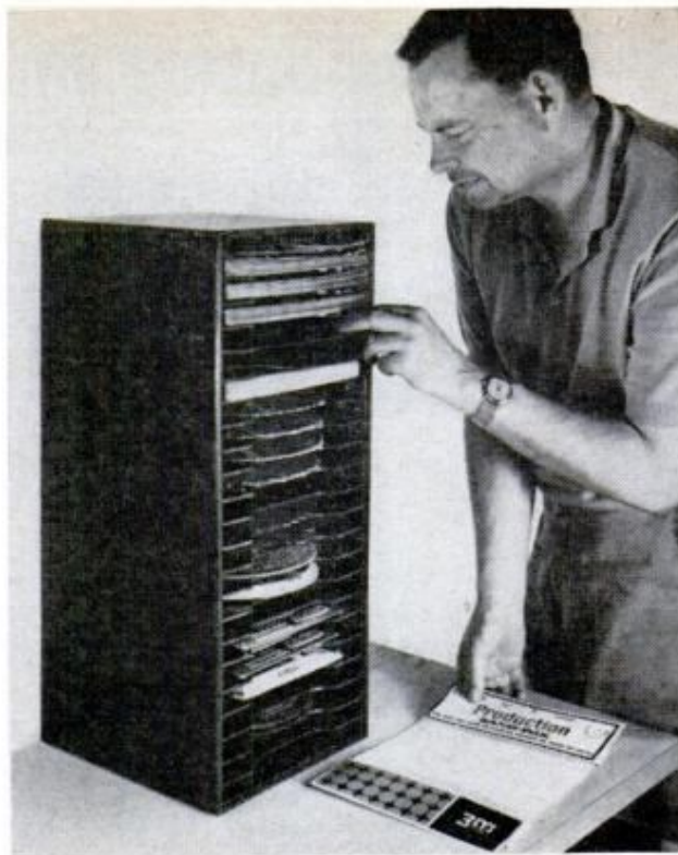
PAPER STORAGE "INCH" RACK has \frac{1}{8} -in. hardboard shelves 1 in. apart. Compartments of 9\frac{1}{4} \times 11 in. hold standard 9 \times 11 -in. sheets. Shelves fit grooves in sides of \frac{3}{8} -in. plywood box.—John Burroughs
