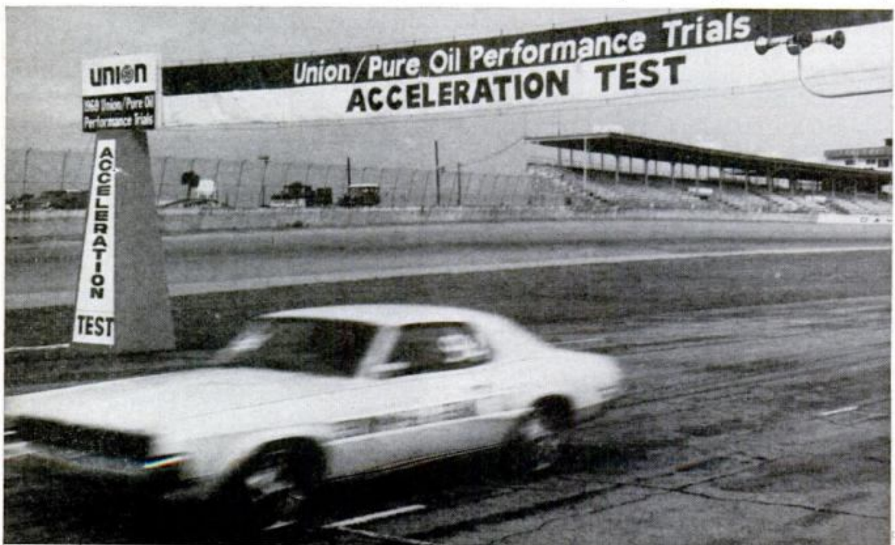
ACCELERATION TEST simulates a typical passing situation, checks how long it takes to go from 25 to 70 mph
