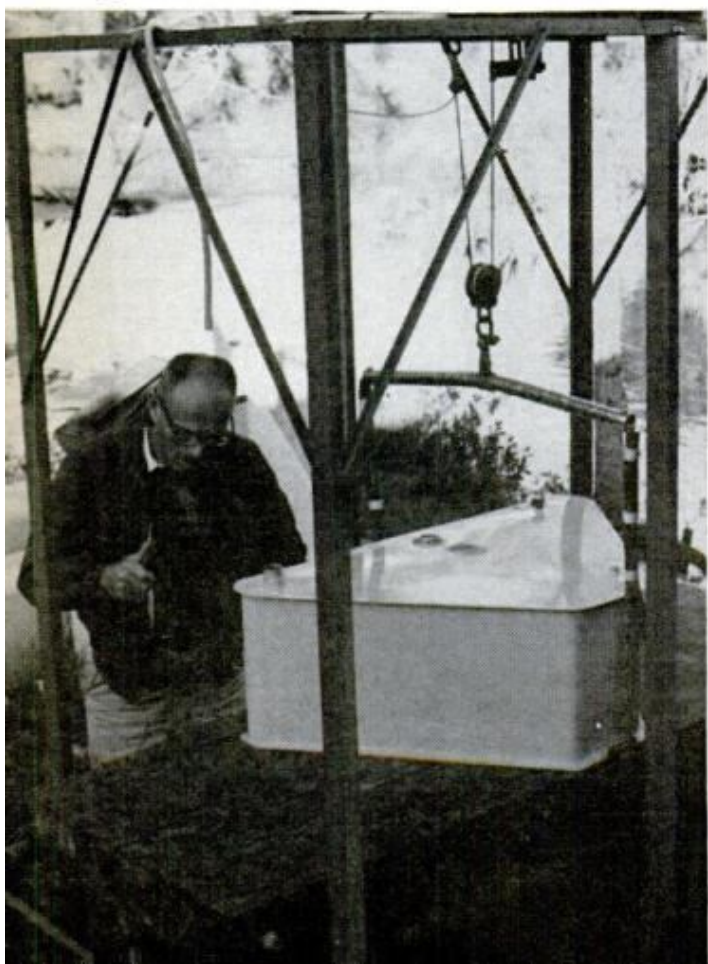
GAS-TANK FIRE TEST subjects gasoline-filled tanks to 1000°F. for 2½ minutes. Tanks must withstand this tremendous heat to pass. Marshall Eldredge Jr., holds a stopwatch waiting for temperature, registered on wall meter, to reach the proper figure
