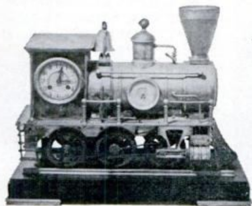
LARGE WHEELS of railroad engine revolve as piston moves in and out
