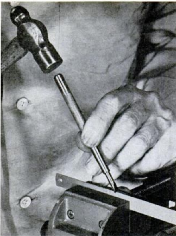
NEAT MODELMAKER'S SAW can be made by using a sharp chisel to notch a strip of carton-binding steel
