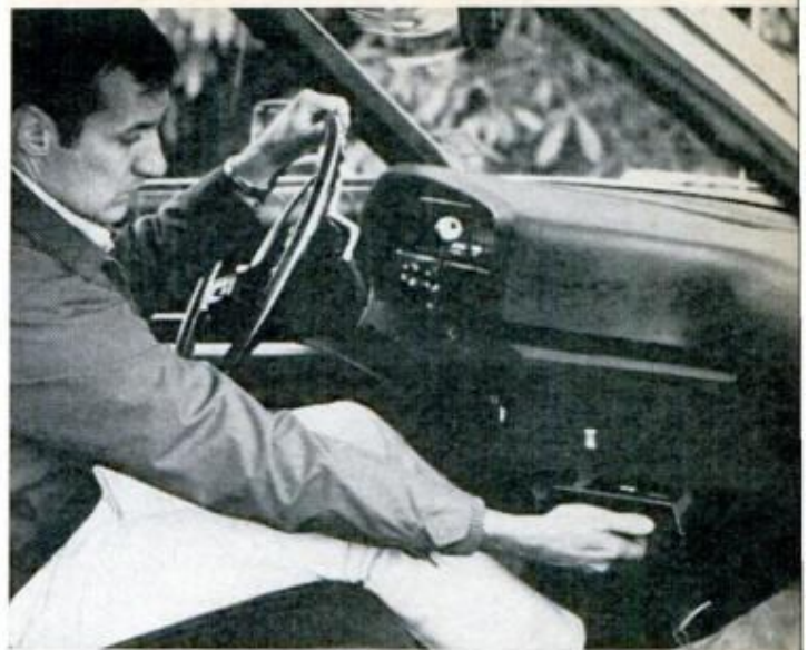
DRIVER'S ASHTRAY , believe it or not, is around the corner of the semi-wraparound instrument panel. Puzzled owners criticized this clumsy arrangement
