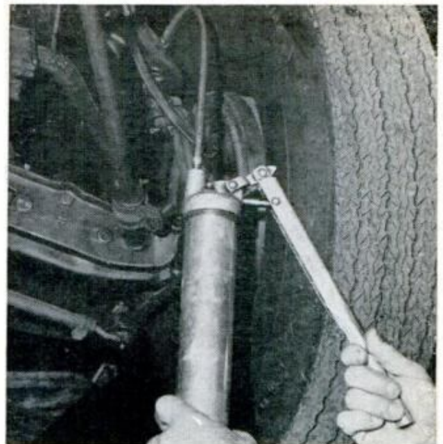
FLEXIBLE ADAPTER on nozzle of grease gun is sometimes needed to reach fittings hidden among suspension components. Upper ball joints are one example
