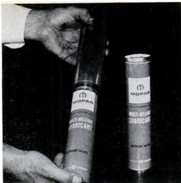
GREASE CARTRIDGES do away with old method of packing your gun with bulk grease. Cartridge slides in, grease is dispensed and cartridge is discarded
