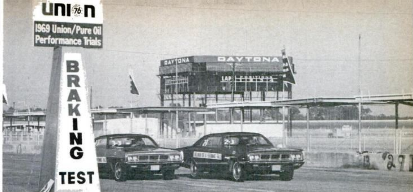
318-CU.-IN. POLARA (left) got more mpg, stopped quicker, accelerated slightly slower than 383 cu.-in. Monaco
