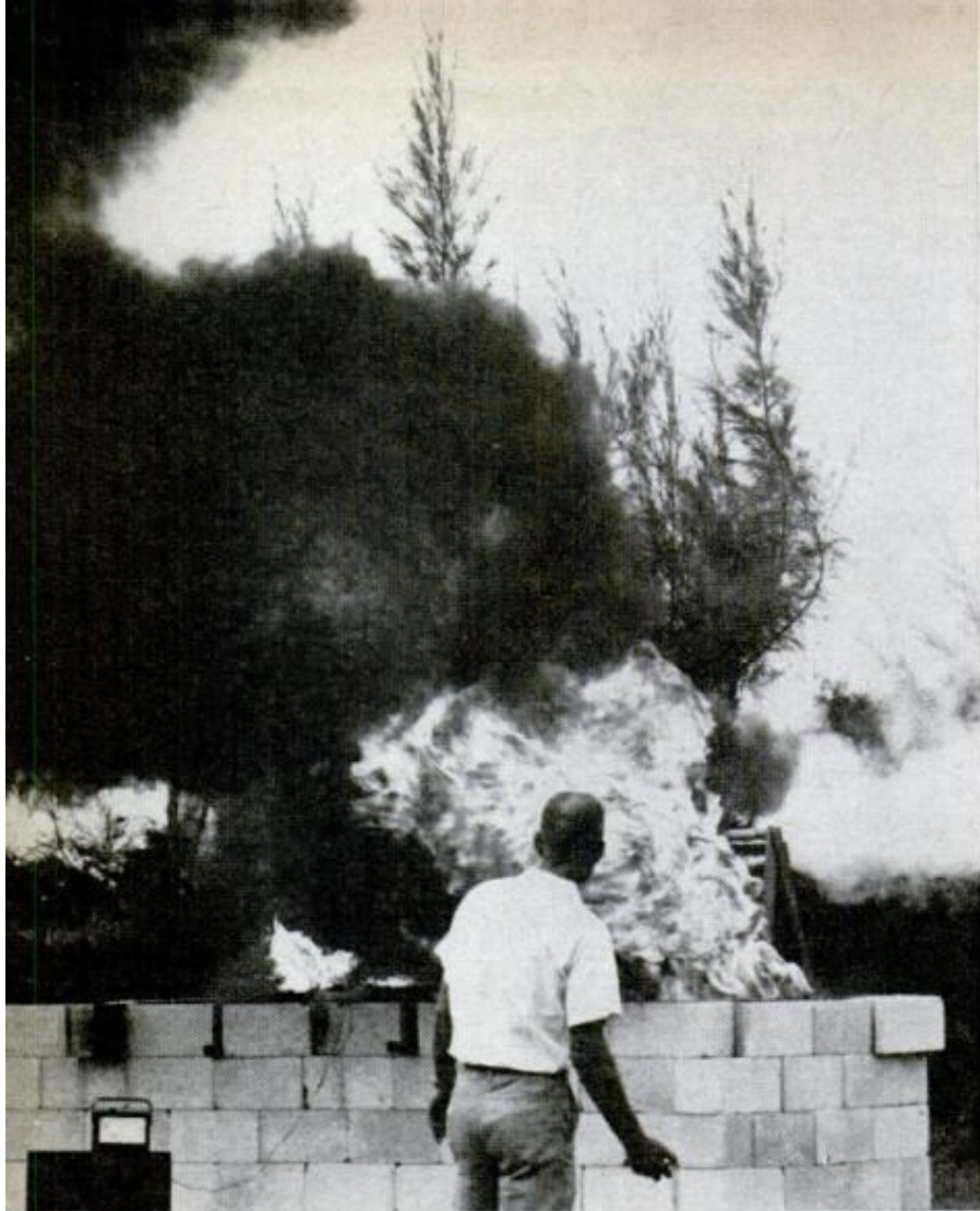
GAS-TANK FIRE TEST subjects gasoline-filled tanks to 1000°F. for 2½ minutes. Tanks must withstand this tremendous heat to pass. Marshall Eldredge Jr., holds a stopwatch waiting for temperature, registered on wall meter, to reach the proper figure
