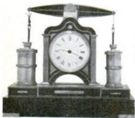
WALKING BEAM. As beam moves up and down, it controls rate of clock
