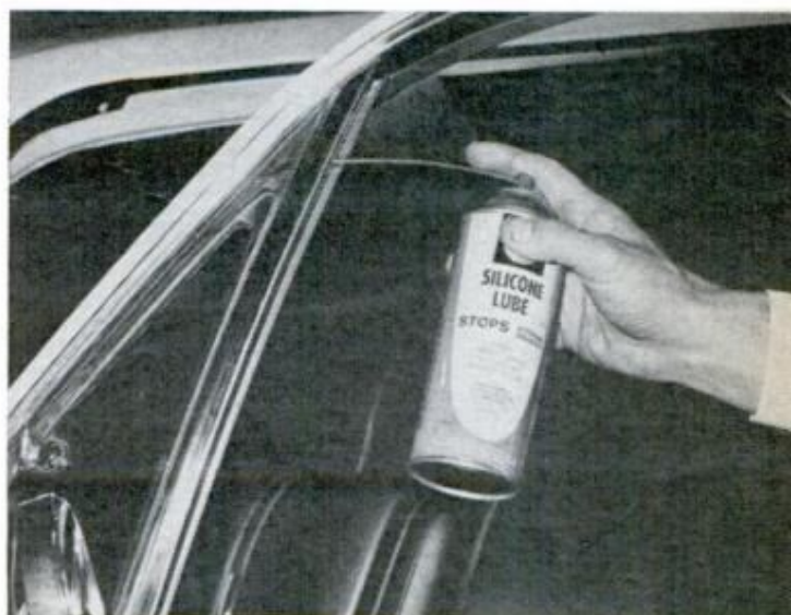
SILICONE SPRAY has dozens of applications in house and garage; lube of car-window channels is one
