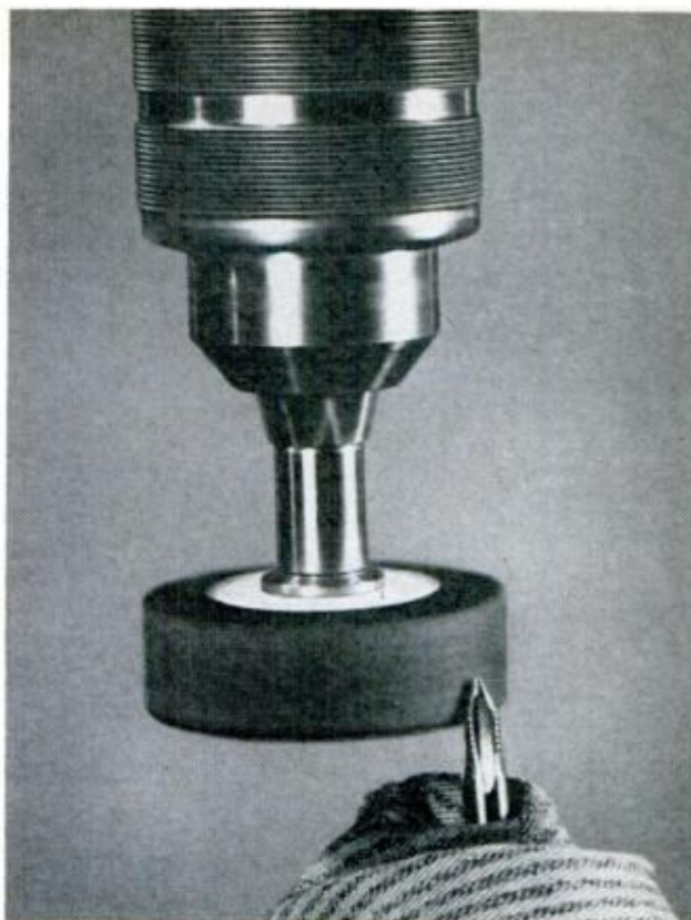
GRINDING WHEEL chucked into drill press offers easy method of grinding taps. Cloth protects the vise
