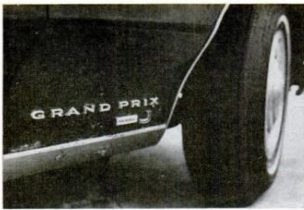
INWARD CURVE of rocker panel styling is catchall for dirt, road debris tossed up by both front tires
