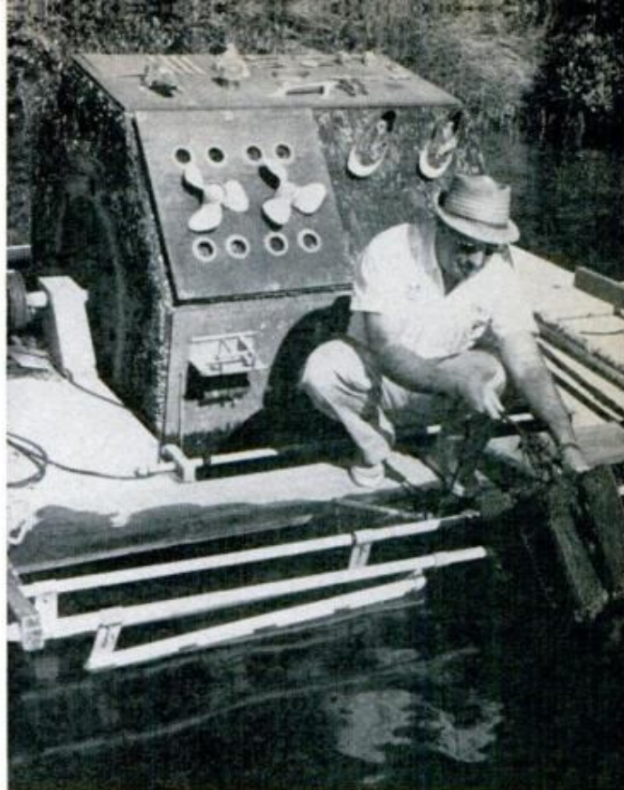
DIP-DRY is the test wheel that rotates once every six hours, submerging items for two hours, exposing them to sun for four. Bob Parker checks paint test
