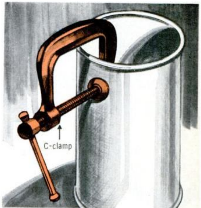
TEMPORARY BUT RIGID HANDLE for an empty can or similar container can be improvised by tightening a 2 or 3-in. C-clamp over the edge as shown above
