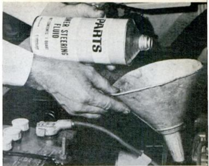
POWER-STEERING RESERVOIR should be checked regularly. Stock power-steering fluid for topping off
