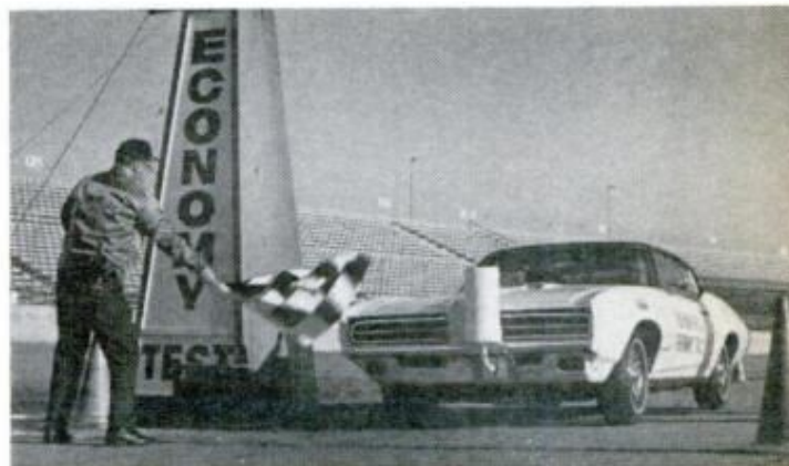
ALL CARS get precise measure of gas for economy test. Insulation keeps fuel at uniform temperature
