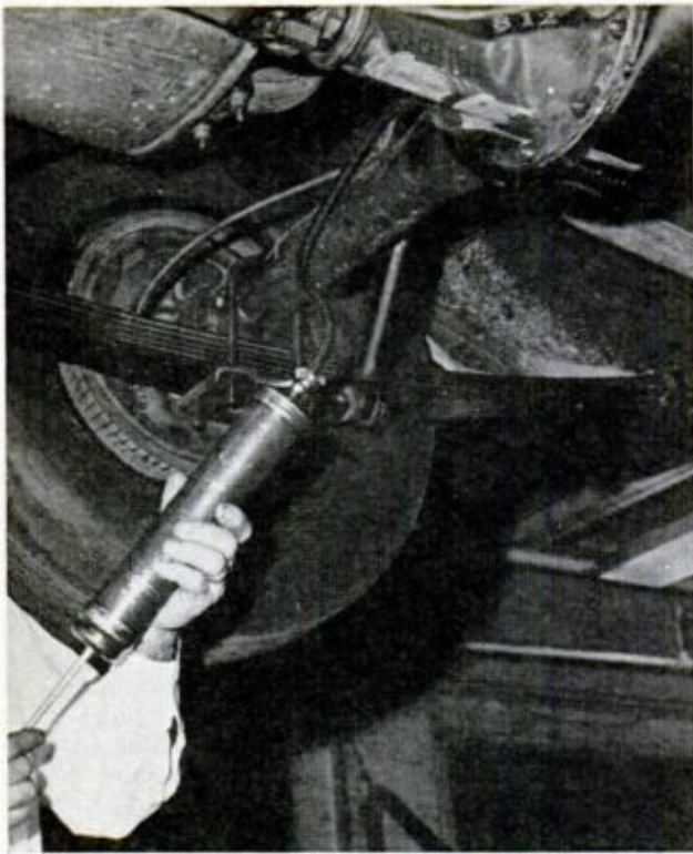
SUCTION GUN tops off lubricant in gear boxes and rear axles, removes it when flushing is necessary
