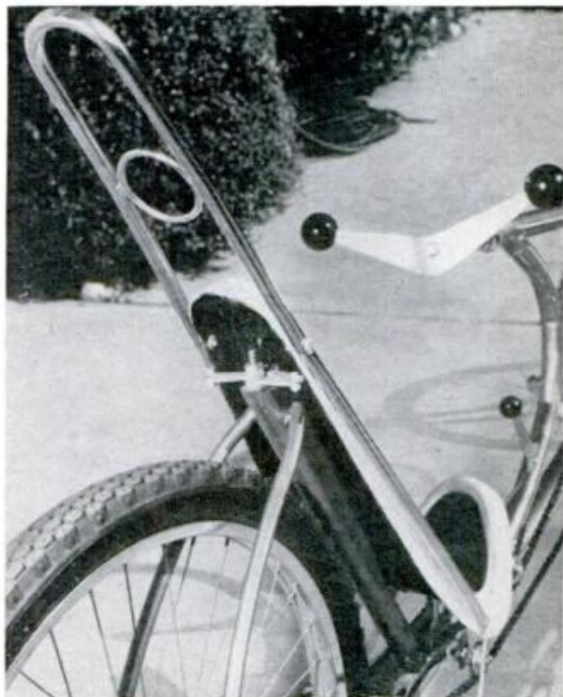
BUCKET SEAT is anchored at top to threaded stud in frame's post. High back bar bolts to sides of seat
