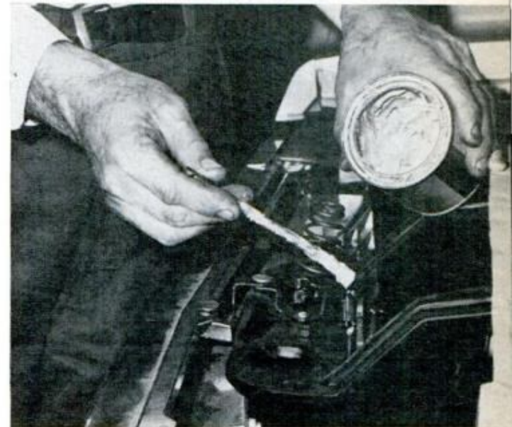
ALL-PURPOSE WHITE GREASE is used on rubbing metal parts such as hood latch, doesn't run like oil
