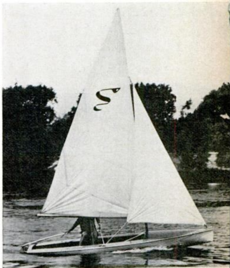
MFG'S SIDEWINDER is a 15½-foot planing-hull sailboat that comes rigged as either cat or sloop. Fiberglass hull is self-bailing; weight is under 200 pounds
