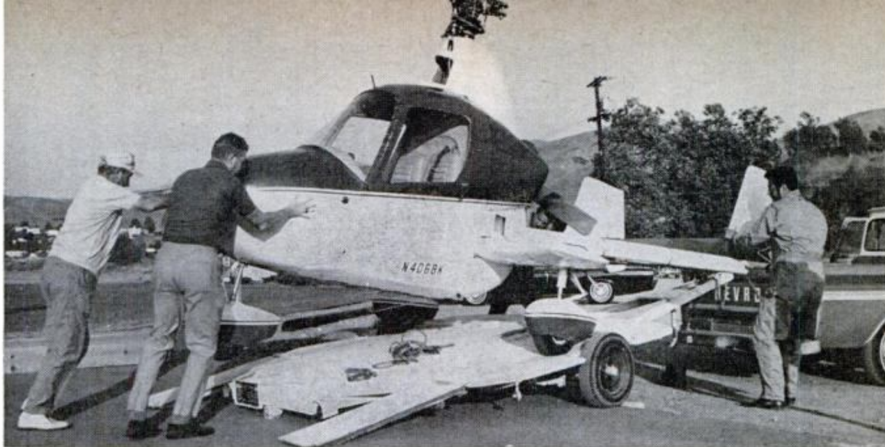
EASILY TRAILERABLE by removing the rotor, the J-2 weighs only 900 pounds, can be loaded by two men
