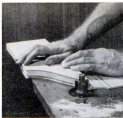
TEMPLATE TACKED to sidewall permits curve to be trimmed with straight shaper cutter
