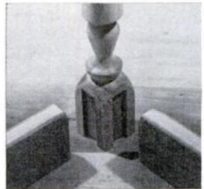
SNUG-FITTING DADO makes a strong glued joint. Apron ends are rounded to conform to blind dado
