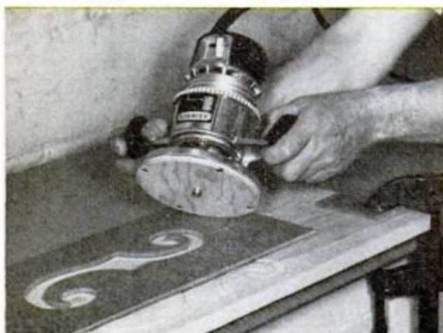
SLEEVE THROUGH PLYWOOD DISC guides router bit around inside, outside of template tacked to the work
