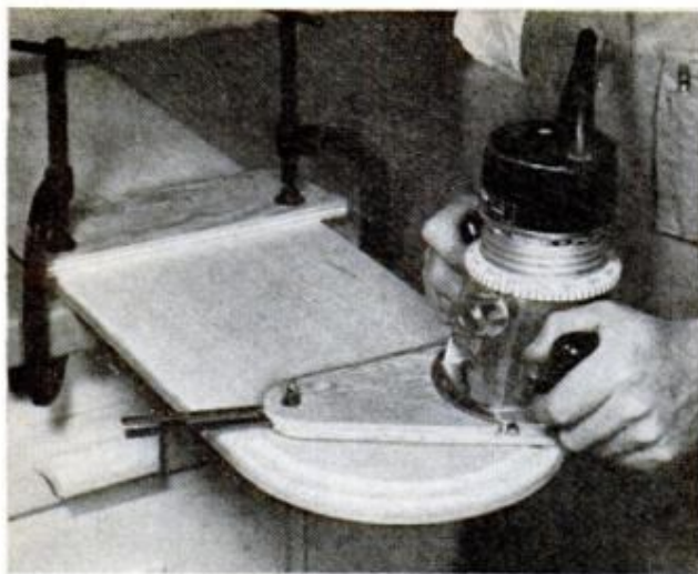
WITH THIS ATTACHMENT, the router can be swung around to rout perfect circles, rabbet edge of work
