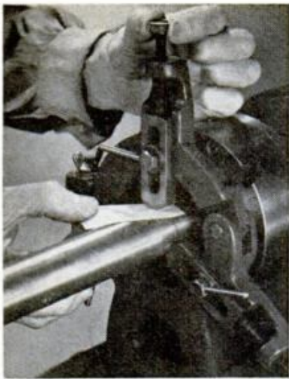
A SLIP OF PAPER inserted between jaws and workpiece will help you set proper jaw clearance
