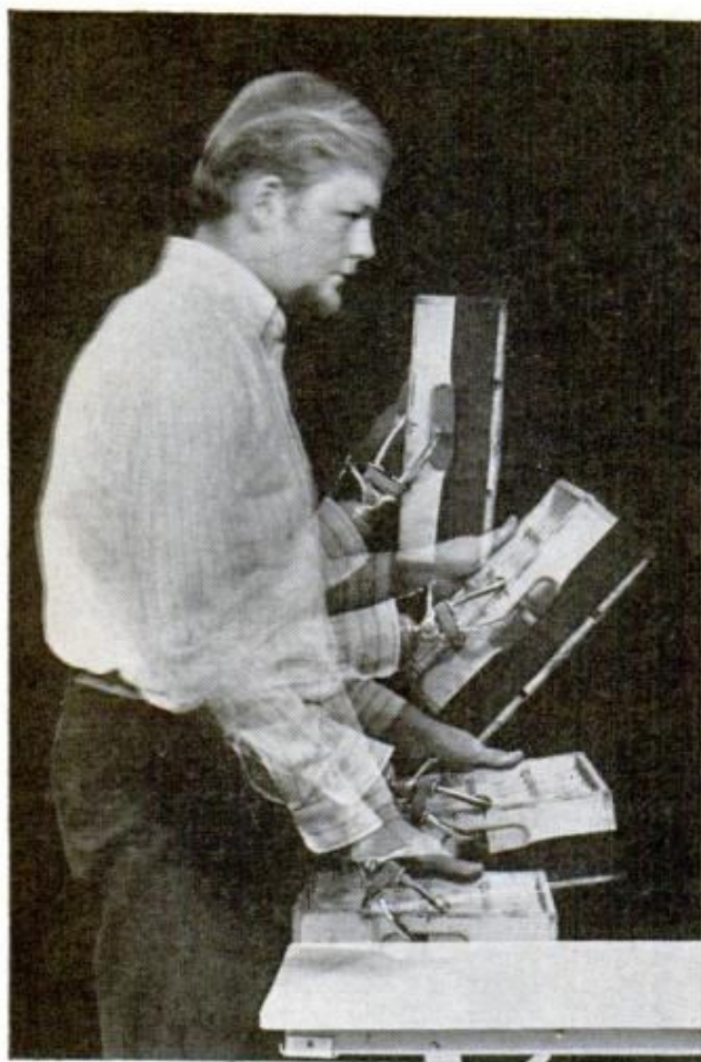
PICKING UP A BOX with two hands, one real and one artificial, an amputee shows how the mechanical device is so sensitive he can easily balance the weight between the two to keep the box level. The amount of muscle tension required to lift the box is determined by strain gauges inside the device
