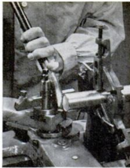
SPINNING THE EDGE of a brass pipe over a wood disc to form a cylinder calls for the use of a rest
