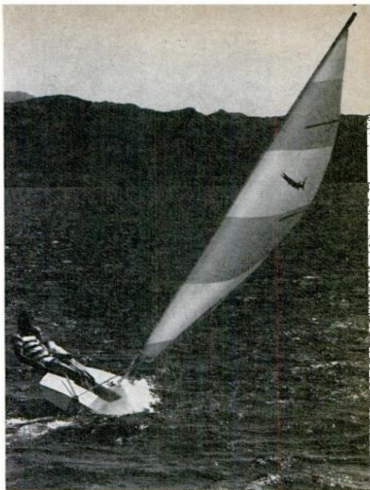
CHRYSLER'S BARRACUDA is a 13-foot, fiberglass-hull sailboat with planing hull. This 180-pound boat comes with either lateen or high aspect ratio cat rigs
