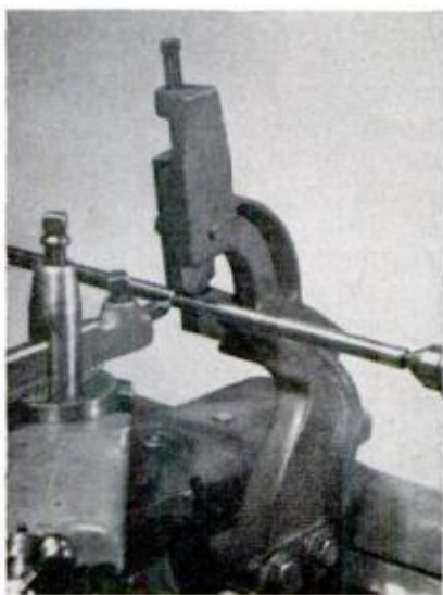
FOLLOWER REST can be attached to the carriage to travel directly in line with tool to support work
