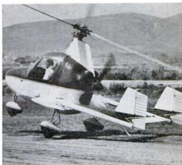
GYROPLANE LEAPS OFF at 30 mph when blade is tilted 5°. Stubby craft is virtually spin-and-stallproof
