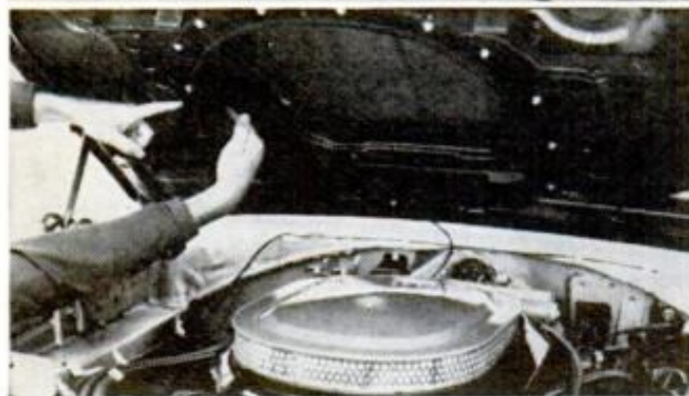
AIR GRABBER hood scoops duct-cool air to carb when engine compartment breathing is closed off. Some thought power boost would be more noticeable
