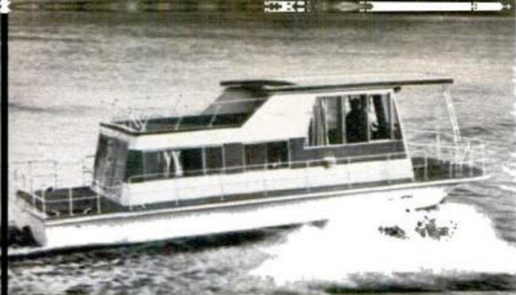
BOATEL'S 35-FT. HOUSEBOAT has new roomy interior design. Fiberglass boat did 32 mph during trials
