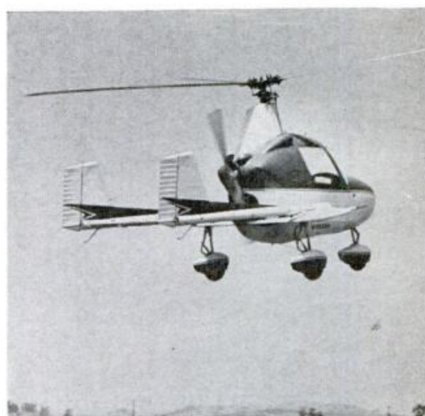
PUSHER PROP provides forward motion that keeps rotor spinning. J-2 then flies like fixed-wing craft
