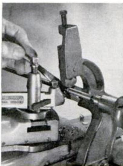
WHEN THREADING slender piece of work, set the follower rest so that it travels in front of the bit
