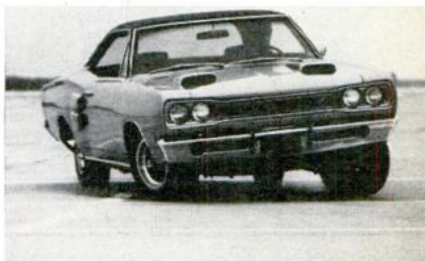
HANDLING impresses owners most. As on all Chrysler cars, wishbones and torsion bars suspend front end. Ram air scoops are detailed on the next page
