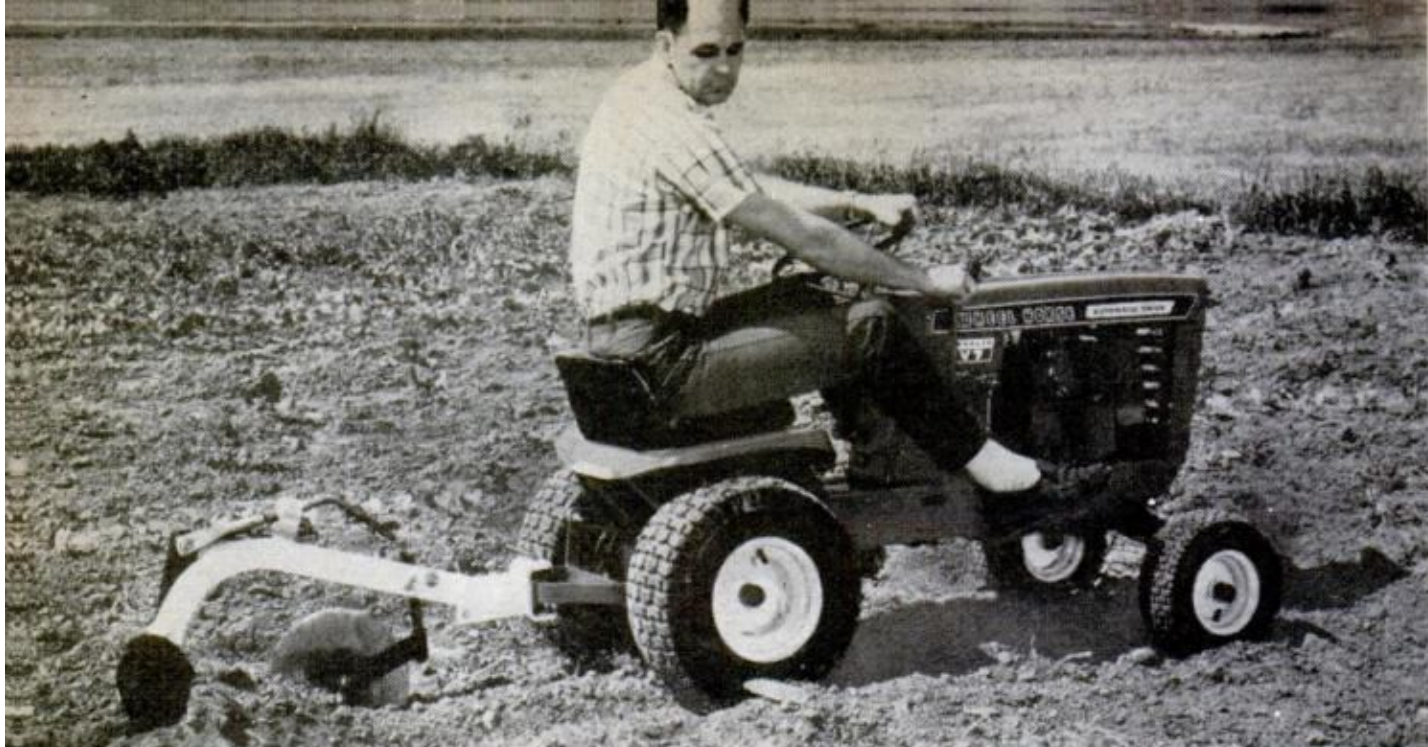
WHEELHORSE CHARGER V7 (electric-starting standard) takes 36-inch mower, pulls 8-inch plow, costs $780
