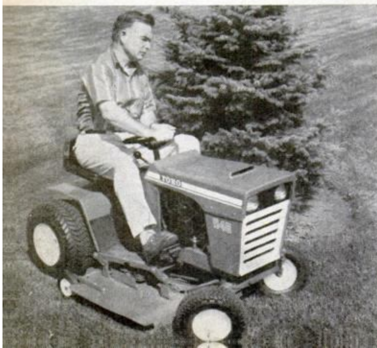
TORO'S 25-INCH TURNING RADIUS makes it highly maneuverable. The $800 price includes as standard a 36-inch mower, headlights, electric starting
