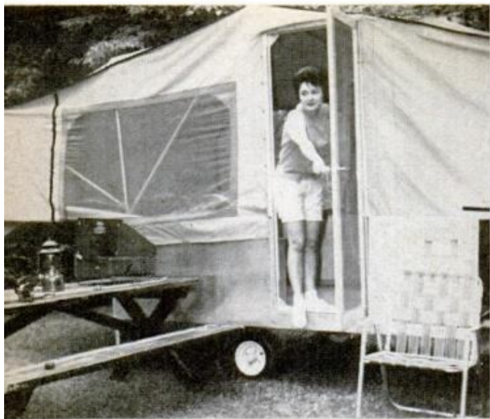
SCREEN DOOR can be mounted. This door is removed and laid on the floor when you collapse the trailer
