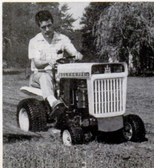
BOLENS HUSKY 775 has foot-pedal control for hydrostatic: toe down for forward, heel down for reverse. Standard: electric starting, headlights at $750
