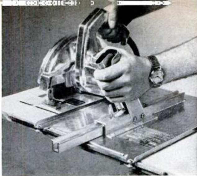
CLAMP-ON CUTOFF GUIDE won't sideslip; squeeze-type handle will clamp lumber up to 12-in. wide
