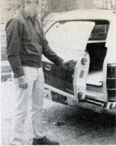
TWO-WAY TAILGATE hinging at side or bottom is standard on many wagons. Ford's Magic Doorgate, shown here, is the only "fifth door" that is operable with the rear window fully up
