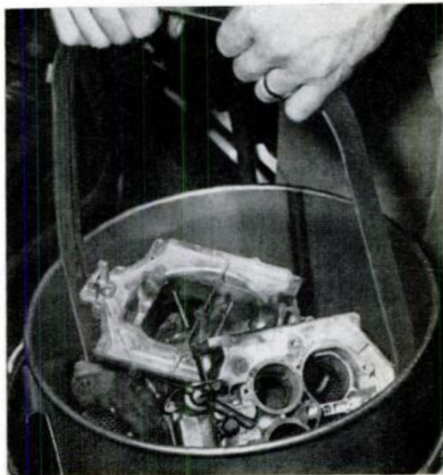
BEST CLEANING is by placing parts in solvent for couple of hours, then blasting with compressed air
