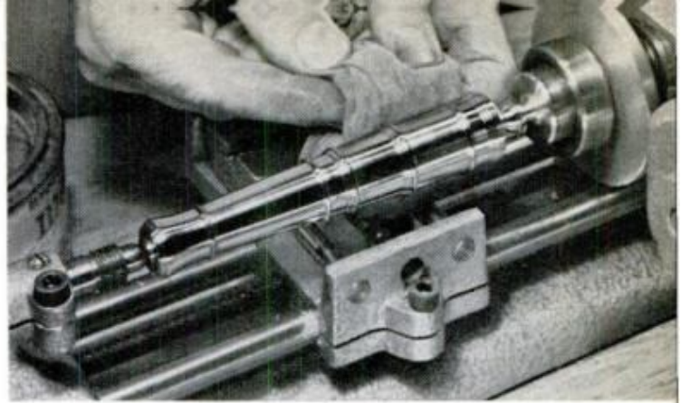
COMPLETED BARREL is polished in the lathe with a brass polish; the ball end is hand-finished later
