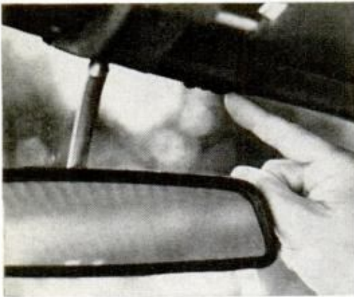
WINDSHIELD SEALER , squeezed out and not trimmed smartly, is minor complaint
