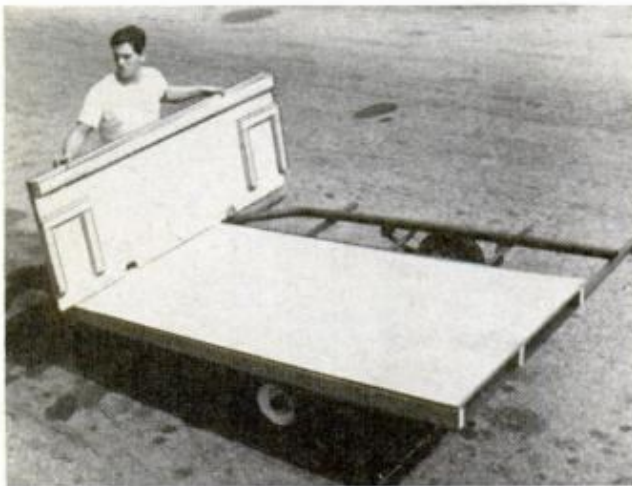
PREFABING SIDES is a good idea. Note position of the structural supports for cabinets at box ends
