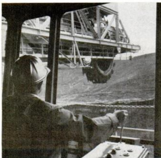
OPERATOR can swing, raise or lower the wheel. Wheel works in semicircle as entire machine moves
