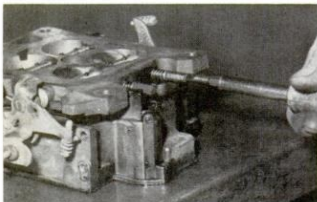
IDLE SCREWS are removed and checked. If damaged, and rebuild kit has no replacements, buy separately
