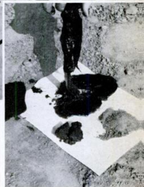
OILY SAND (left) yields a tar substance called bitumen (center) and clean sand (right). The bitumen is treated to produce crude oil, coke, sulphur. Crude oil is pumped 250 miles to refinery, while clean sand is used to fill the excavation
