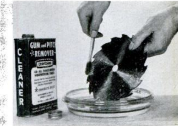
BLADE CLEANING SOLVENT makes it easy to remove pitch from saw blades, carbide-grit sanding wheels
