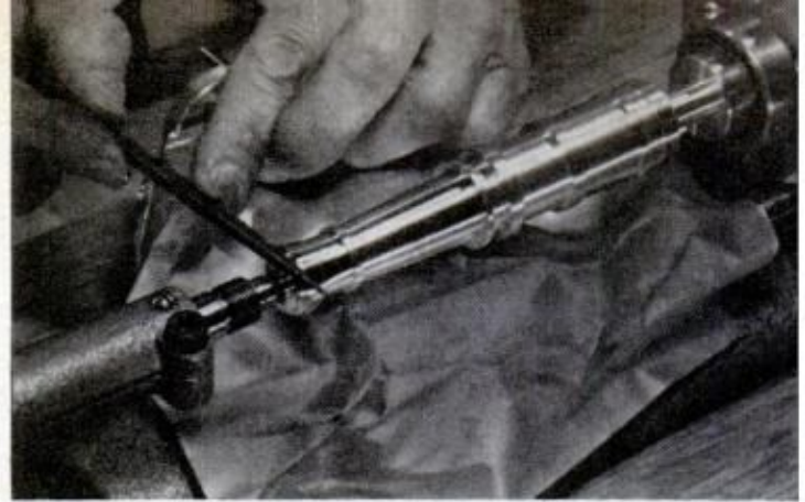
AFTER RIDGES are machined square they're rounded with Swiss-type file as done here at gun's muzzle end
