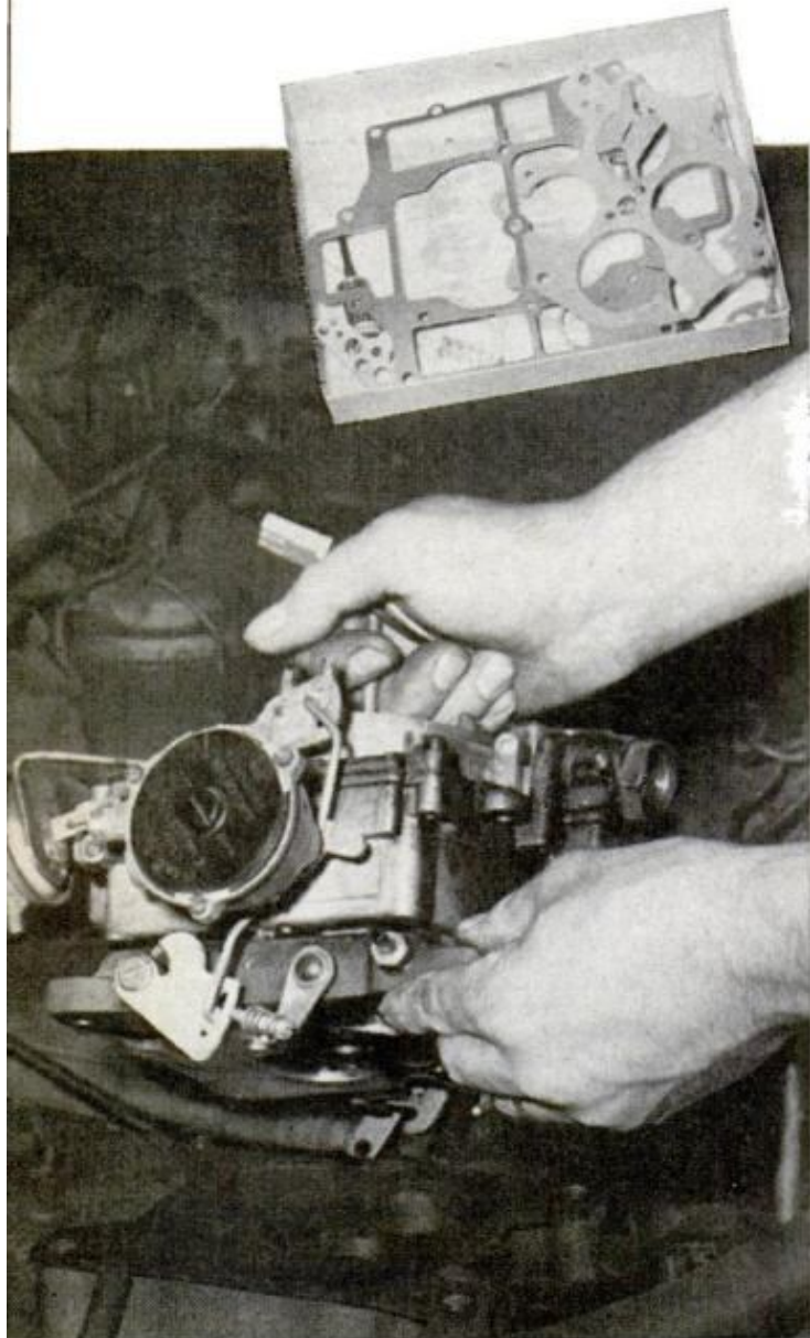
REBUILD KIT for major overhaul has everything from a manifold gasket to a rubber idle vent (above)
