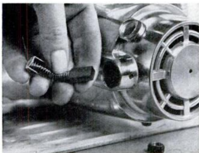
CHECK CARBON BRUSHES REGULARLY. When they wear to half their original length, install replacements
