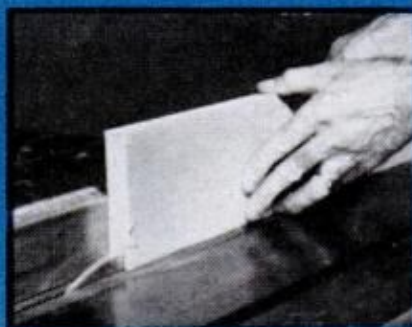
CUT BOTH RABBETS in one 30-in. board. Then cut the sides and top to length from this board.
