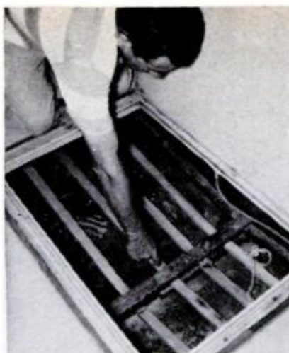
STRINGERS protect bottom when heavy gear is stored in the bow
