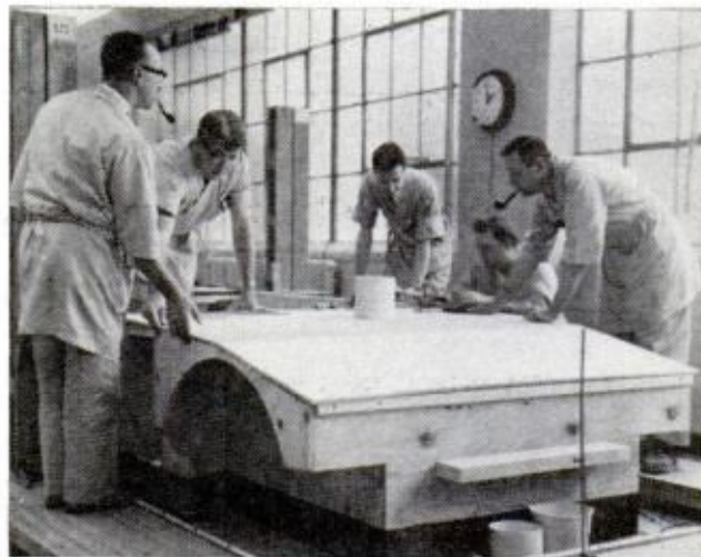
WOOD CHASSIS are built to hold full-size models for final changes in detail before making die molds
