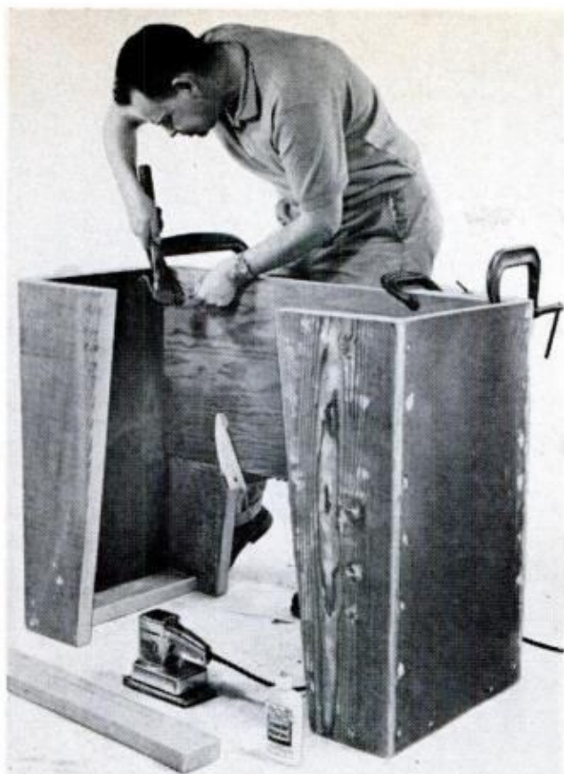
JOIN BOX LEGS with a 2x4 rail in front and a plywood panel in rear. Glue and nail all joints securely
