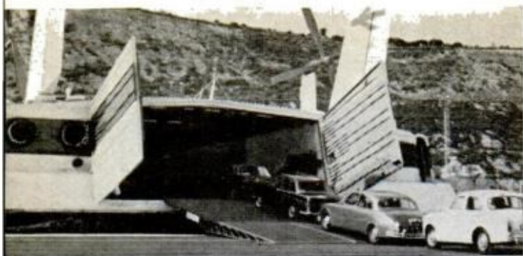
CARS, TOO, are loaded aboard 100-ton Hovercraft. Huge ship can carry 30 of them for each crossing
