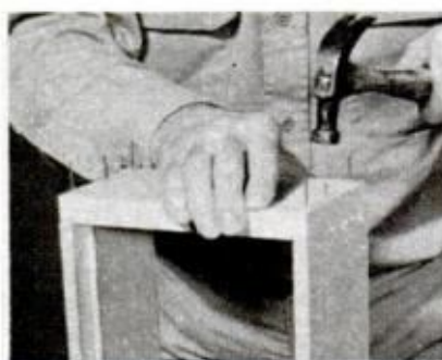
GLUE AND NAIL the mitered joints with 6d finishing nails. I blunted the nail points to avoid splitting
