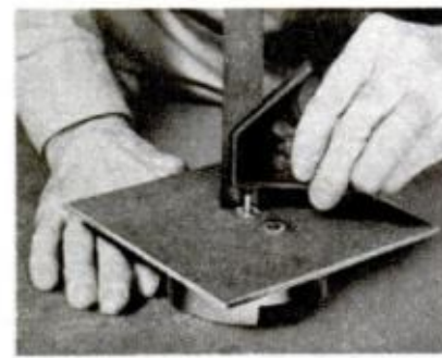
MOVEMENT IS MOUNTED on dial backing plate, then used to determine location of support cleats
