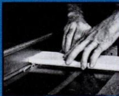
RABBET MITER used to join sides and top is begun by making \frac{3}{8} -inch cut \frac{1}{4} inch from the end.
