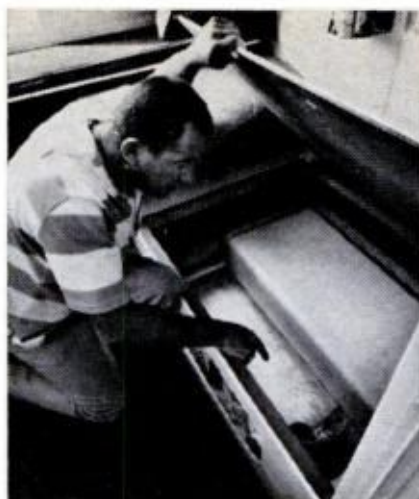
UNDER LOWER BUNK are water tank, pump, good storage space
