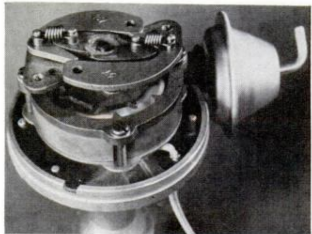
PULSE DISTRIBUTOR triggers spark magnetically; no points and rotor to wear out, timing stays set
