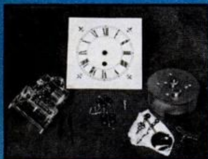
CLOCK MOVEMENT is a standard eight-day short-pendulum type which has a roman-numeral dial.
