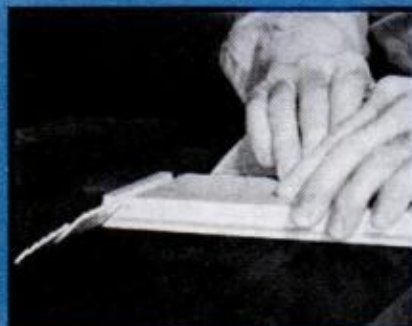
MITER CUT at 45^\circ should just reach the root of the first cut. Sides are then cut to length.
