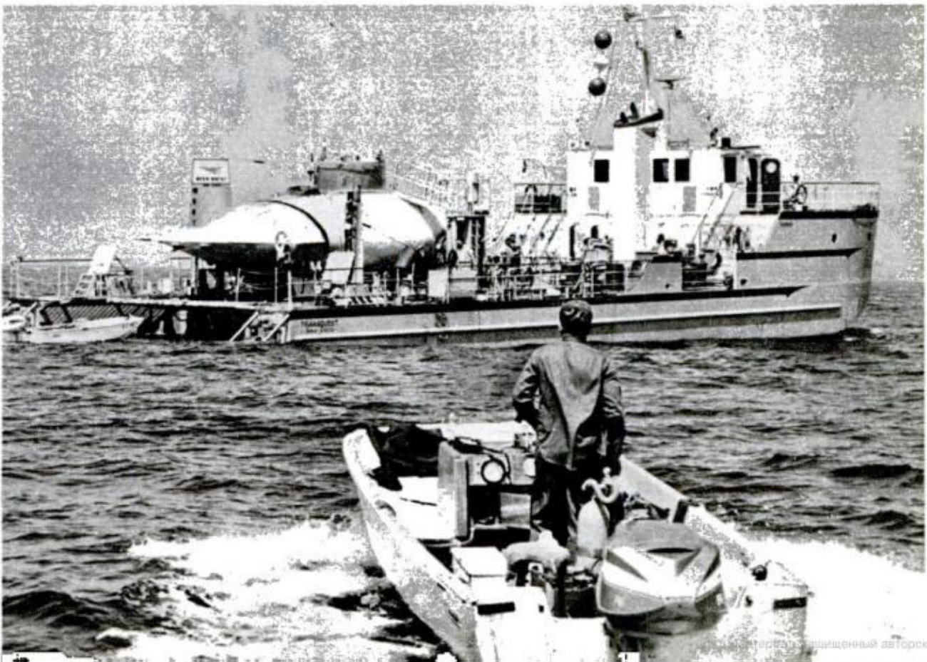
TRANSQUEST carries Deep Quest out to diving site where it will lower sub to water level on its elevator
