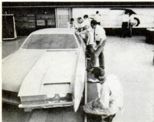
CLAY MODELS are made when Styling and Engineering agree; then fiberglass molds are made from them
