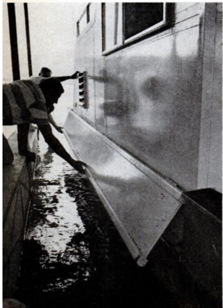
CATWALKS CAN BE DROPPED when entering a tight mooring slip or preparing the boat for trailering
