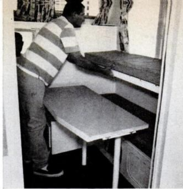
BUNKS FOR TWO are located in the deckhouse. The back of the settee swings in to serve as upper bunk
