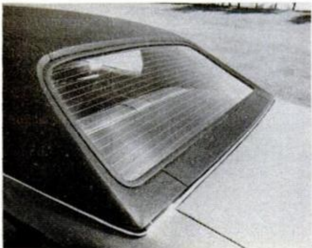
PONTIAC GRAND PRIX options include a wired rear window that provides quick defogging, ice removal
