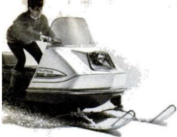
POLARIS Mustang is a family-size machine. The track has been widened to 20 inches for more stability. Mustang is available with any of six engine sizes
