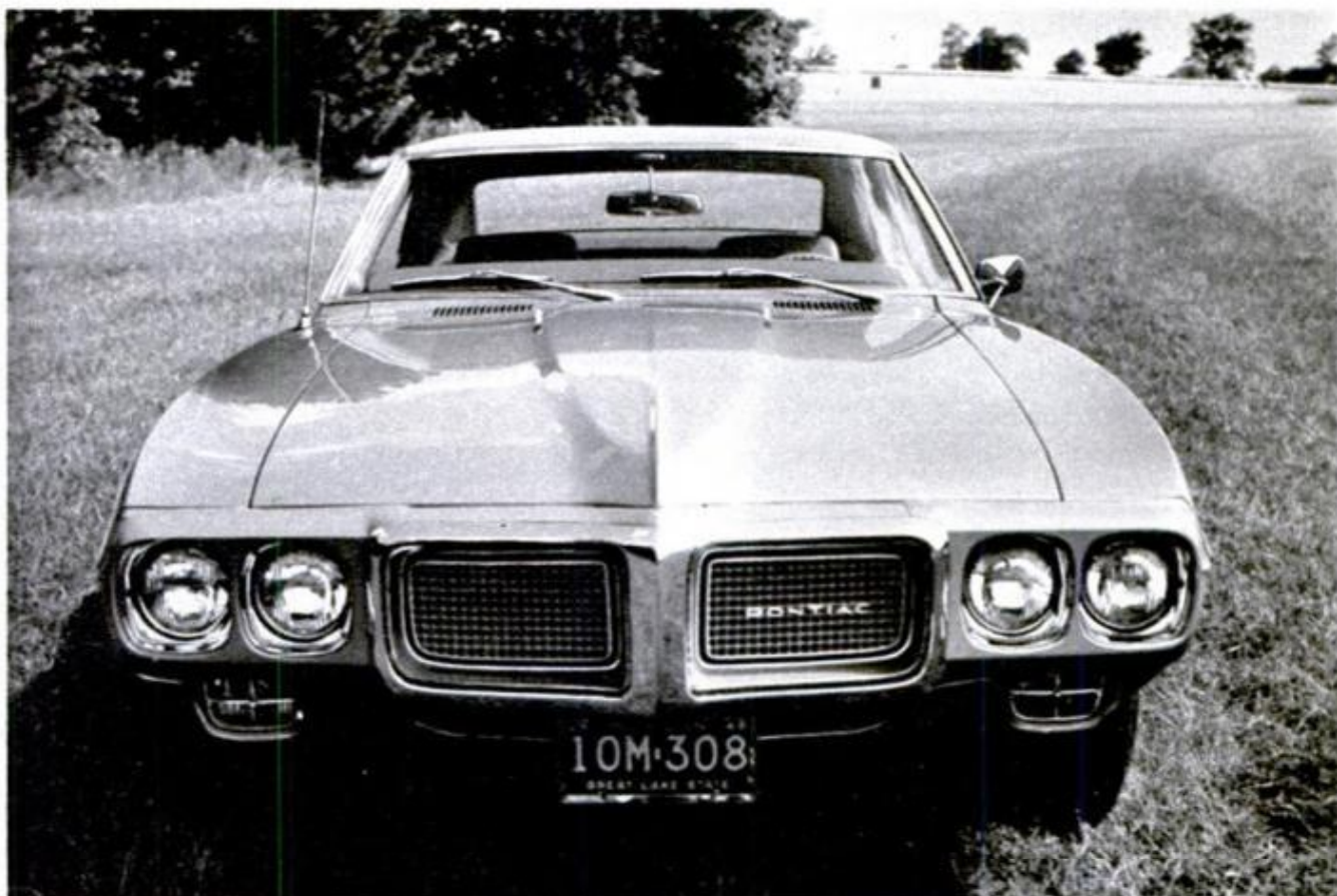
PONTIAC FIREBIRD features a new grille, front bumper extensions made of energy-absorbing polymeric plastic
