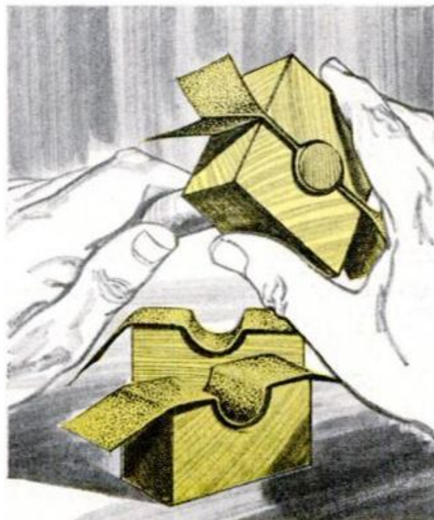
WHEN REGLUING CHAIRS , you can do a fast and neat job of removing old glue with a split sanding jig. Clamp two blocks together and drill a hole 1/16 in. larger than spindles, then line jig with sandpaper
