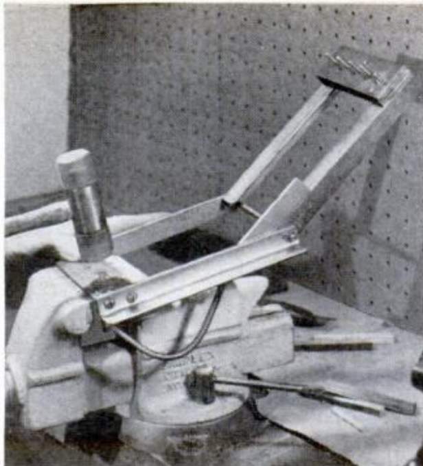
FOR SMALLER DOWELS , blank is then driven through a succession of smaller holes until it is desired size
