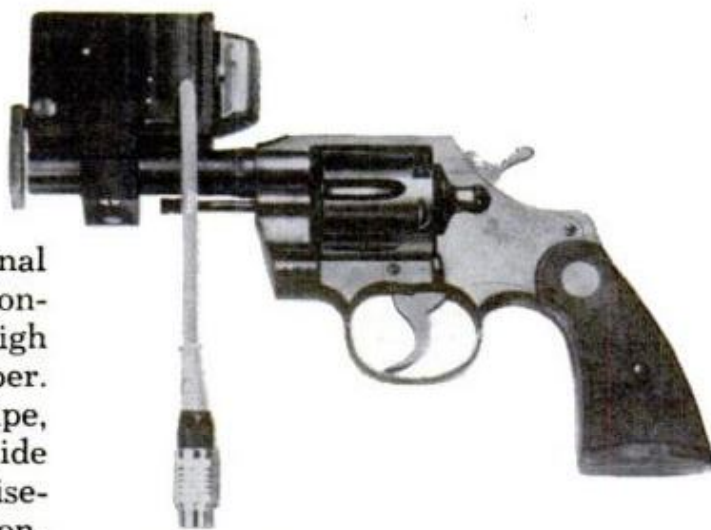
NEW STARTING GUN has microphone on muzzle to relay sound to a loudspeaker in each contestant's lane. Each hears signal at same instant, eliminating delay caused by sound's slow travel through air
