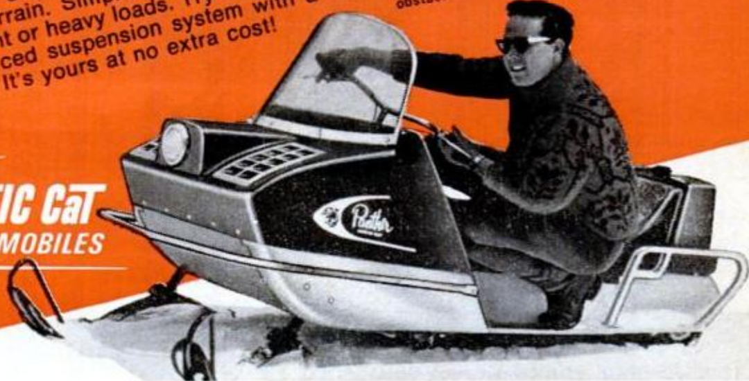
Front end of track absorbs obstacle shocks Track "rides the top" to span ridges and bumps Floating action cushions sudden rear end drops
