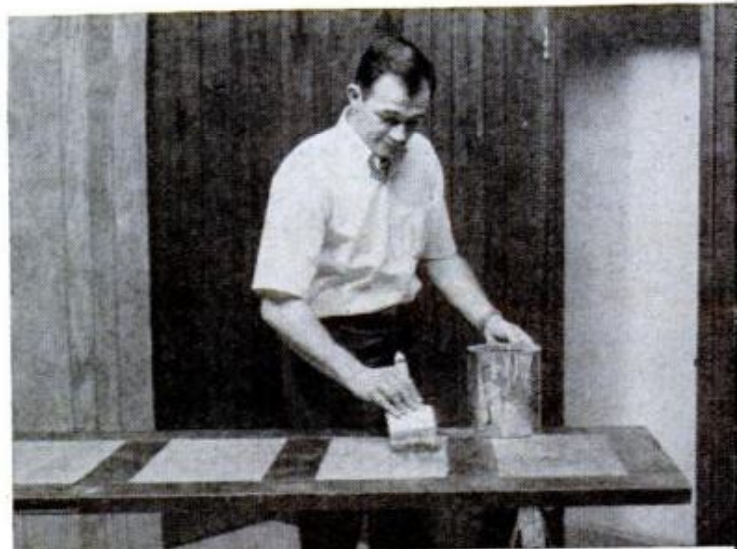
APPLY A LIBERAL COATING of contact cement to both the door and \frac{1}{8} -in. panel and allow to dry
