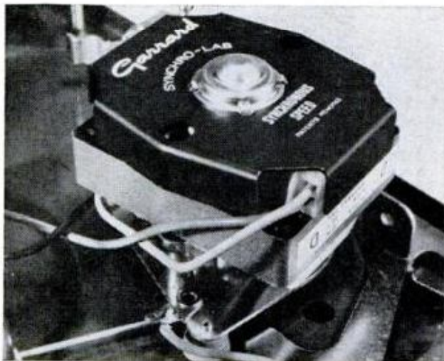
INGENIOUS MOTOR on this Garrard is one of many turntable refinements. Though basically an induc-
