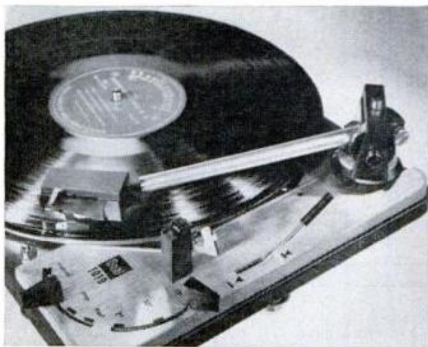
ANTI-SKATING CONTROL on the Dual 1019 puts arm under slight spring tension to offset tendency to
