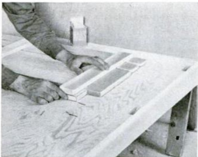
POSITION SIDEBOARD POSTS accurately by the use of a block of wood as a vertical placement guide SEPTEMBER 1968
