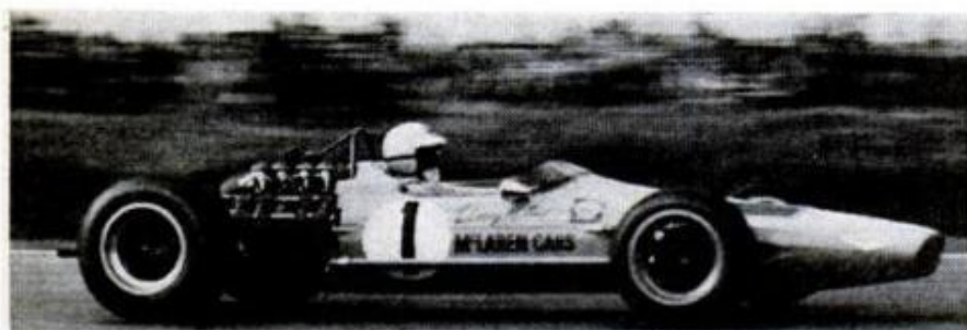
BRUCE McLAREN of New Zealand drives cars of his own design and make, powered by the Ford-Cosworth 408-hp V8. Note the fiberglass cone
