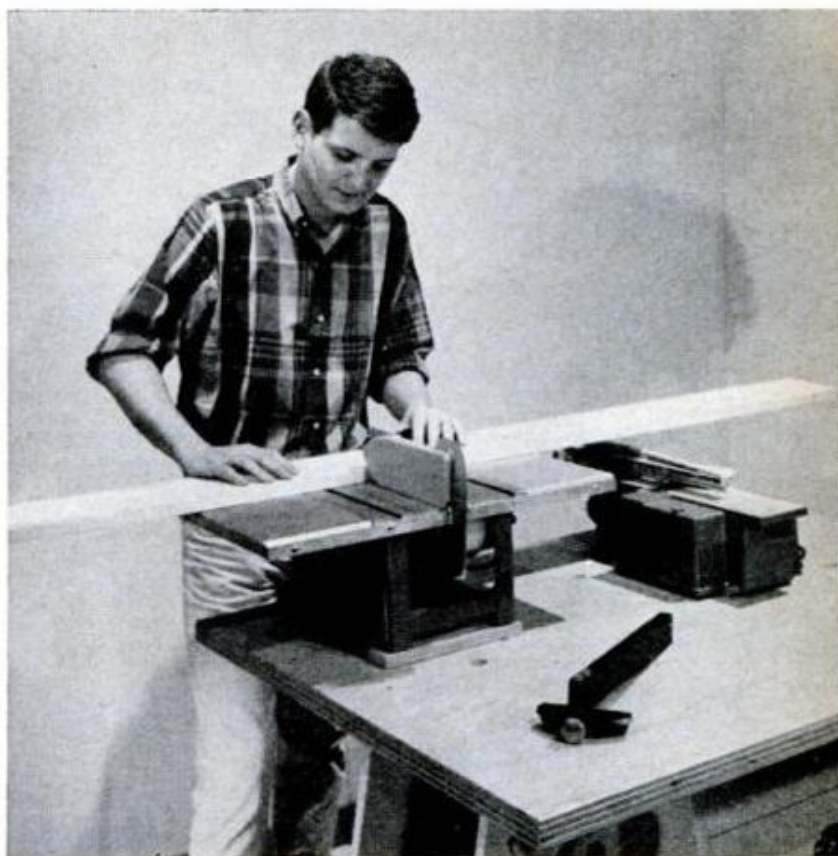
POSITIONING SAW on bench with relation to room's size lets you rip and crosscut long boards easily and without hindrance
