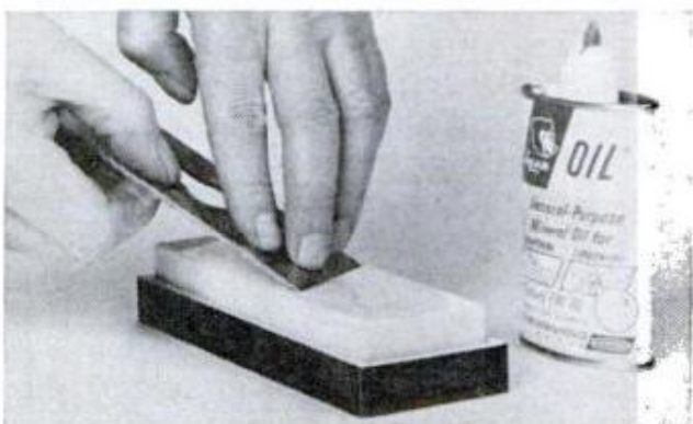
WITH A BENCH-SIZE STONE , keep the bevel flat on stone surface to avoid rounding the cutting edge
