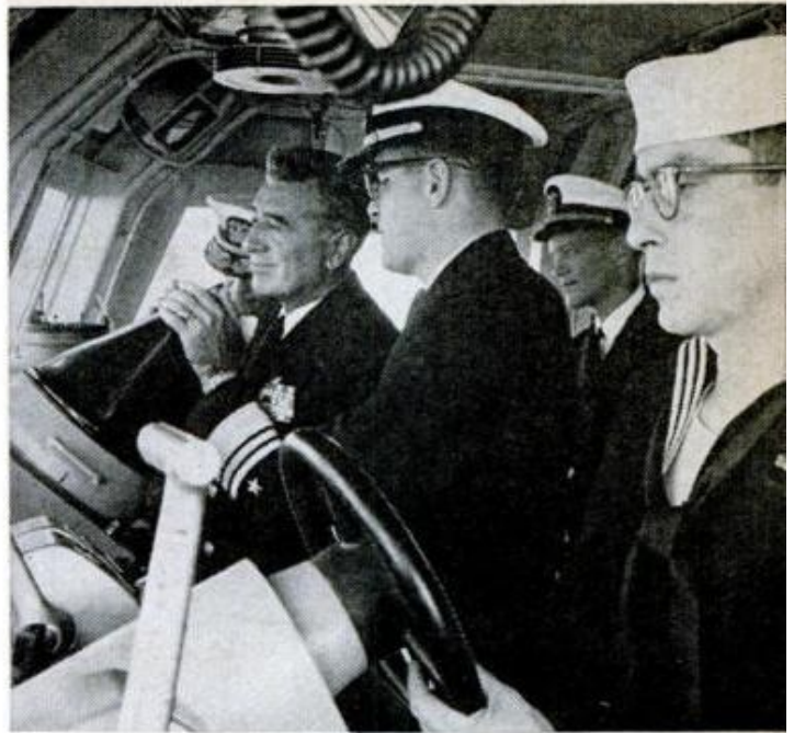
ON PG BRIDGE, helmsman (right) holds relatively small wheel. Jet-engine throttle is in foreground
