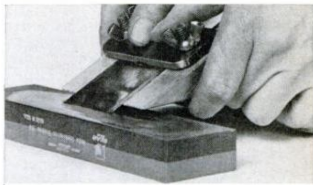
SWIRL BLADE on coarse side of stone to true bevel and grind out nicks. Then finish-whet on fine side
