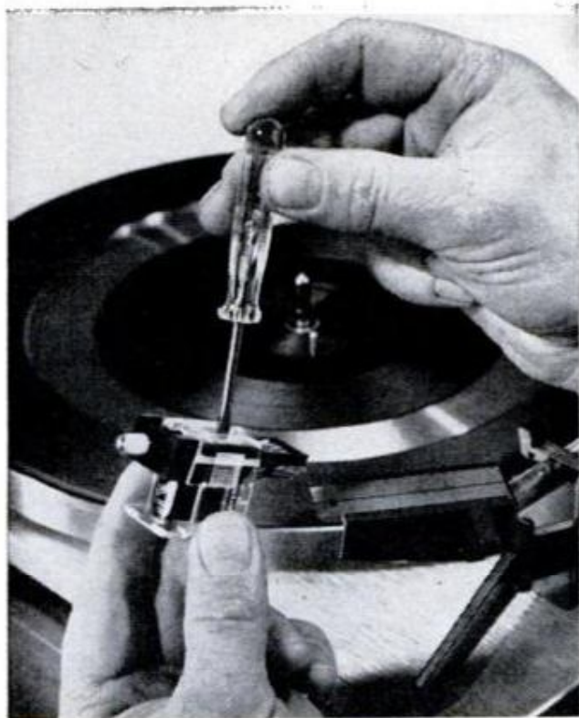
PRECISE PICKUP MOUNTING is aided by this plastic jig supplied with Perpetuum-Ebner models. Jig
