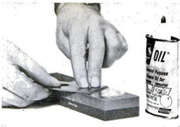
TRUE THE FLAT FACE of the blade on the fine-grit side of combination stone. Oil is necessary
