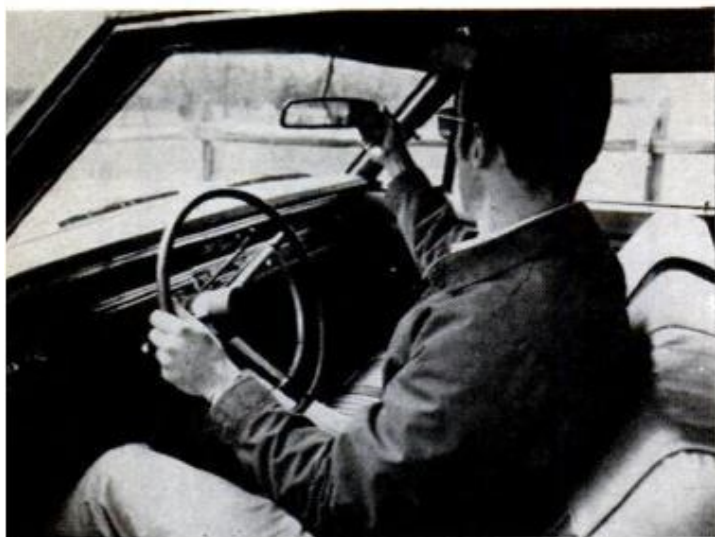
POSITION OF REAR-VIEW MIRROR blocks vision in right-hand turns, but where else can it be located?
