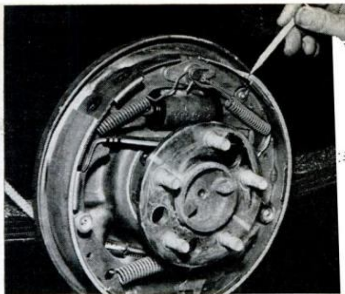
BRAKE LININGS should be checked over their entire surface so uneven wear does not go undetected
