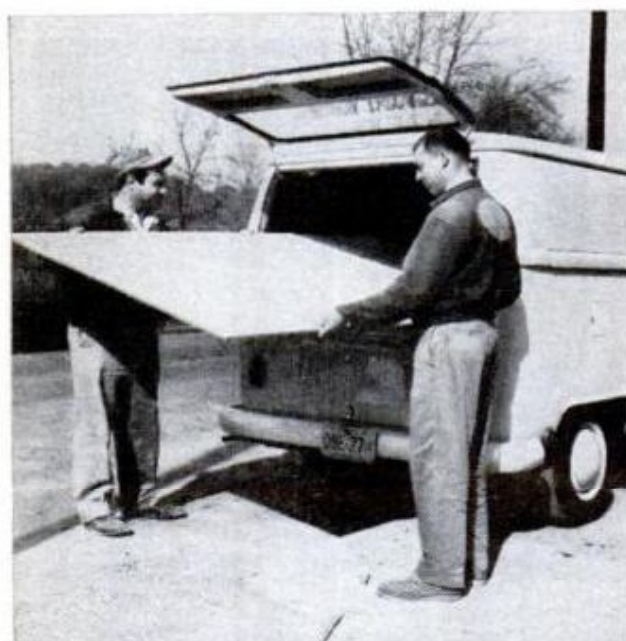
WOOD PANEL IS TILTED to clear spare wheel in VW. Spare could be remounted behind one of the seats
