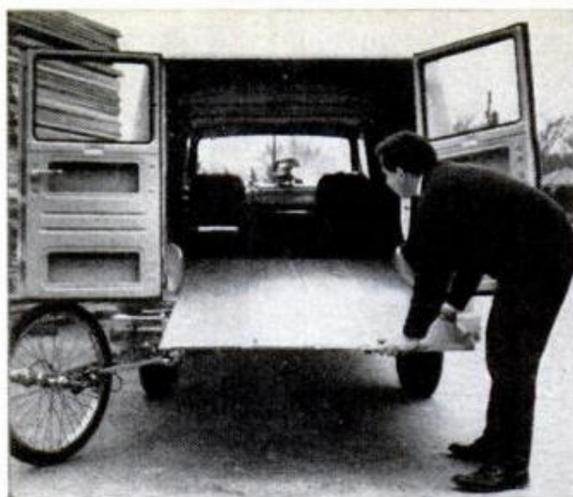
IT'S A TIGHT SQUEEZE between those wheel wells, but 4x8 panel lies flat in cargo area of Dodge van
