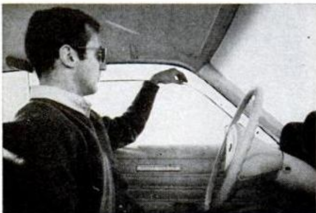
VENTLESS SIDE WINDOW on Torino, unlike that of most cars, has cap of chrome molding for snug fit
