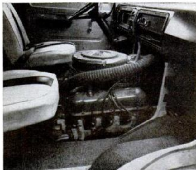
COVER UNBOLTS EASILY to expose entire Ford engine. When you need to check oil, radiator, wipers...
