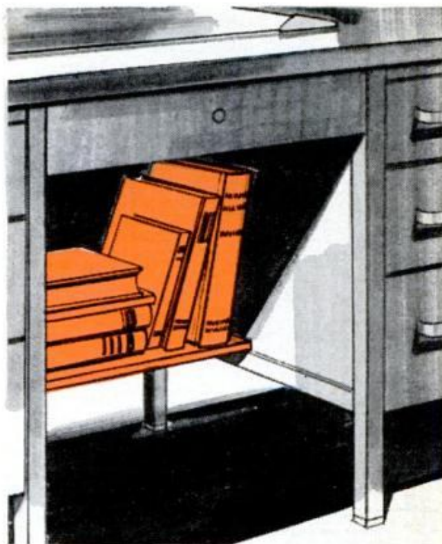
HIDDEN SHELF in your kneehole desk holds seldom used books or files neatly out of sight. Make it about 10 in. deep, notching corners to fit around the desk framing. It rests on well molding without nailing
