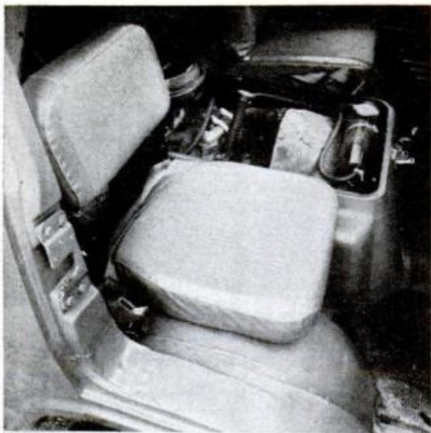
TOP OF ENGINE COVER lifts for quick inspection of Chevy V8. Passenger seat is small but comfortable
