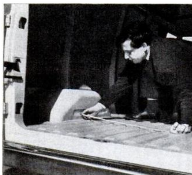
DISTANCE BETWEEN WHEEL WELLS is greater than rear-door width in the Ford. A 4x8 panel fits easily
