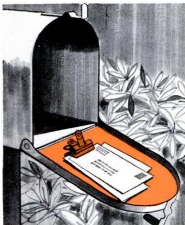
LETTER HOLDER for a rural mailbox prevents outgoing mail from blowing away when the box is opened. A spring paper clamp bolted to inside of door not only holds mail but eliminates the long reach into the box
