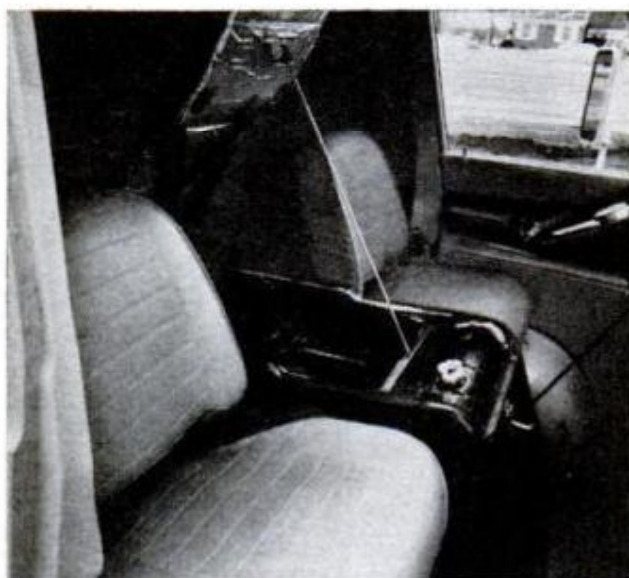
PROP HOLDS UP ENGINE COVER in Dodge. Good insulation keeps engine heat from escaping to cockpit
