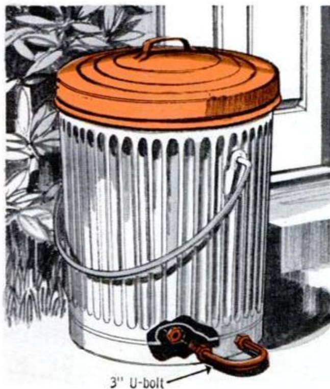
HANDY HOLD-DOWN on your garbage can lets you steady can with your foot when pulling off a tight lid. Make it by attaching 3-in. U-bolt to bottom edge with four nuts, two on the inside and two on outside
