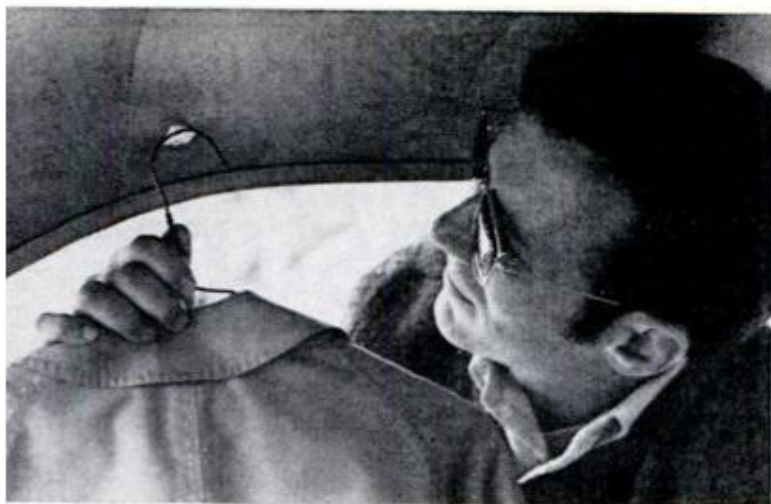
COAT HOOK is mounted too high in this single instance, making it horizontal and totally useless
