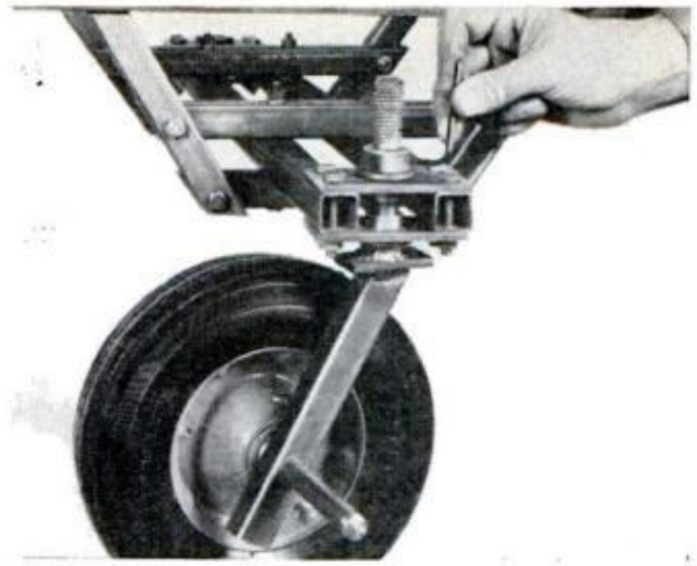
8. DOUBLE-WHEEL CASTERS move almost effortlessly, are the only parts of vehicle that require welding
