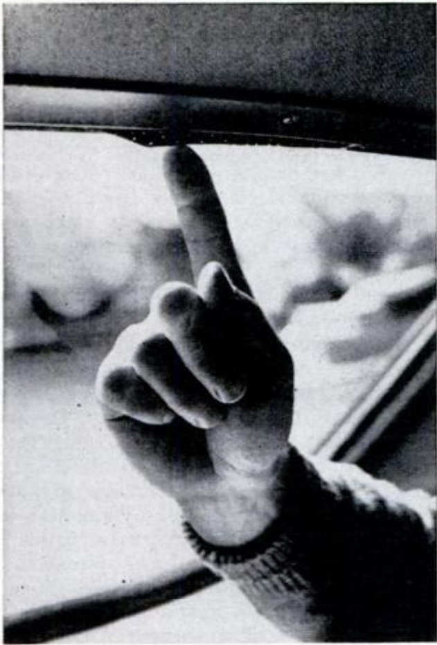
SLIPSHOD HANDIWORK inside Dart includes such things as careless headliner trimming, shown here
