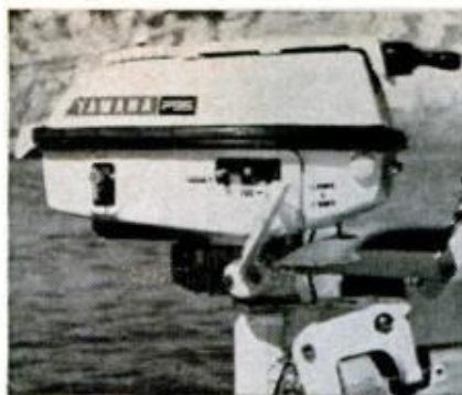
SHIFT LEVER (forward and neutral) is easy to reach on 5-hp motor's right side. Clean design is typical
