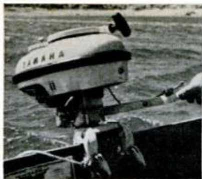
EXCEPTIONAL POWER for such a small unit is key feature of 3.5 hp. Note stop button on front
