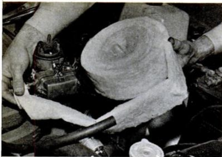
FIBERGLASS INSULATION is very compressible for use around fuel lines near block or other parts
