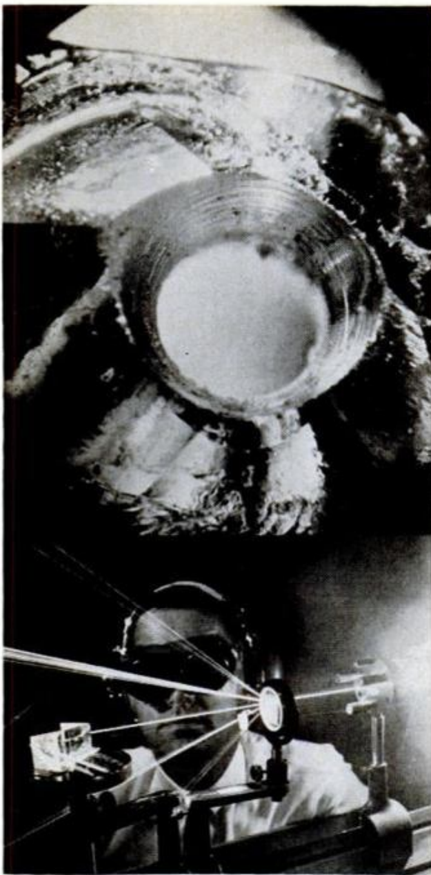
MAGNIFIED HUNDREDS OF TIMES , the circle you see at the top of the page is actually a hair-size hole drilled in a diamond by a laser beam. The diamond die is used to draw rod into fine wire. In lower photo, a continuous-wave argon laser is split into different wavelengths by use of a grating and prisms.
