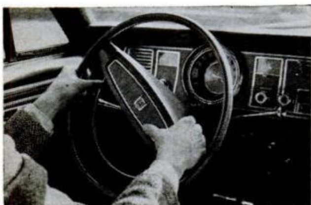
THUMBSTRETCHER horn ring, on all Ford cars, is consistently complained about. So is bulky crossbar
