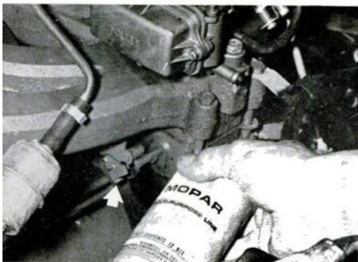
MANIFOLD HEAT-CONTROL VALVE should be checked periodically and kept free with a squirt of solvent
