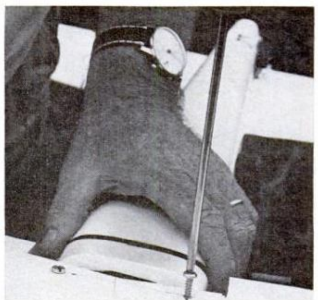
WING CAN BE HELD by thick rubber bands over posts in fuselage or by wood block and sheet metal screws
