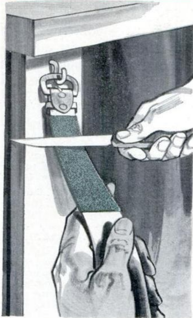
TO KEEP A GOOD EDGE on shop knives and other workshop tools, cement a strip of fine emery cloth to an old leather belt and hang it on your workbench. Use the other side of the belt to strop the knives
