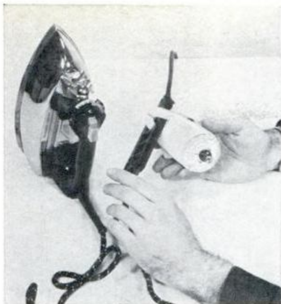
APPLIANCE CURRENT DRAW is checked without breaking circuit using snap-jawed Amprobe meter
