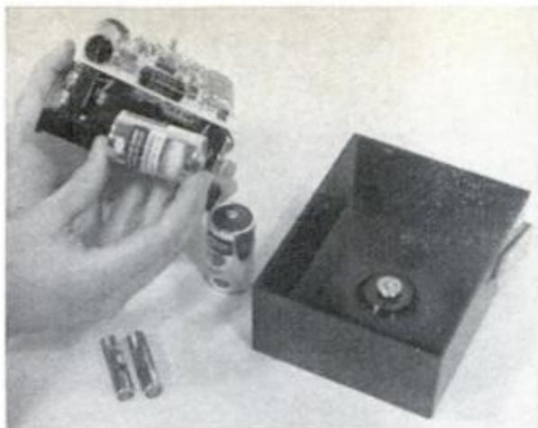
PERIODIC BATTERY REPLACEMENT in a v.o.m. or v.t.v.m. is a must. Keep record of dates on the case
