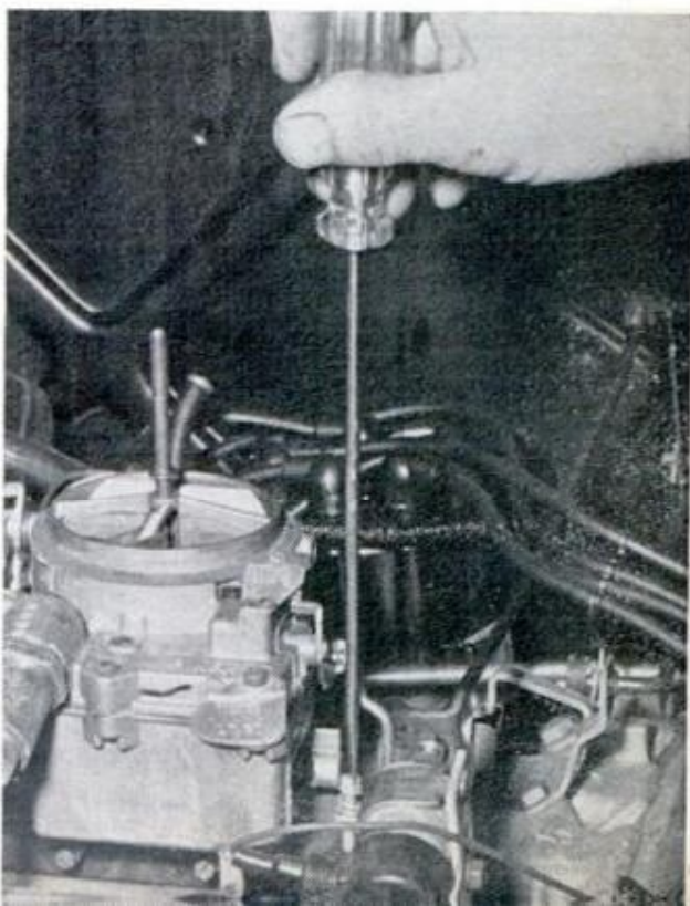
HIGH, STEADY READING during idle adjustment (above) shows carb is clean. Back out throttle stop screw (below) to shut throttle valve for cranking test
