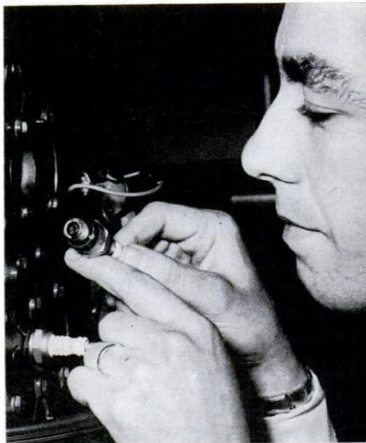
CHECKING PLUGS in problem motors can answer many questions. If plug is dry, as above, there's trouble in fuel system—if wet, recheck ignition system
