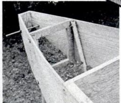
SPORT SUBMARINE , shown in art cutaway and photos, is basically plywood construction with metal tubing. Plastic bubble is vital. Sealed with copper tubing, it contains air pocket
