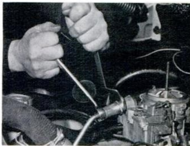
FUEL-PUMP PRESSURE can easily be checked by inserting gauge in fuel line between line and carb
