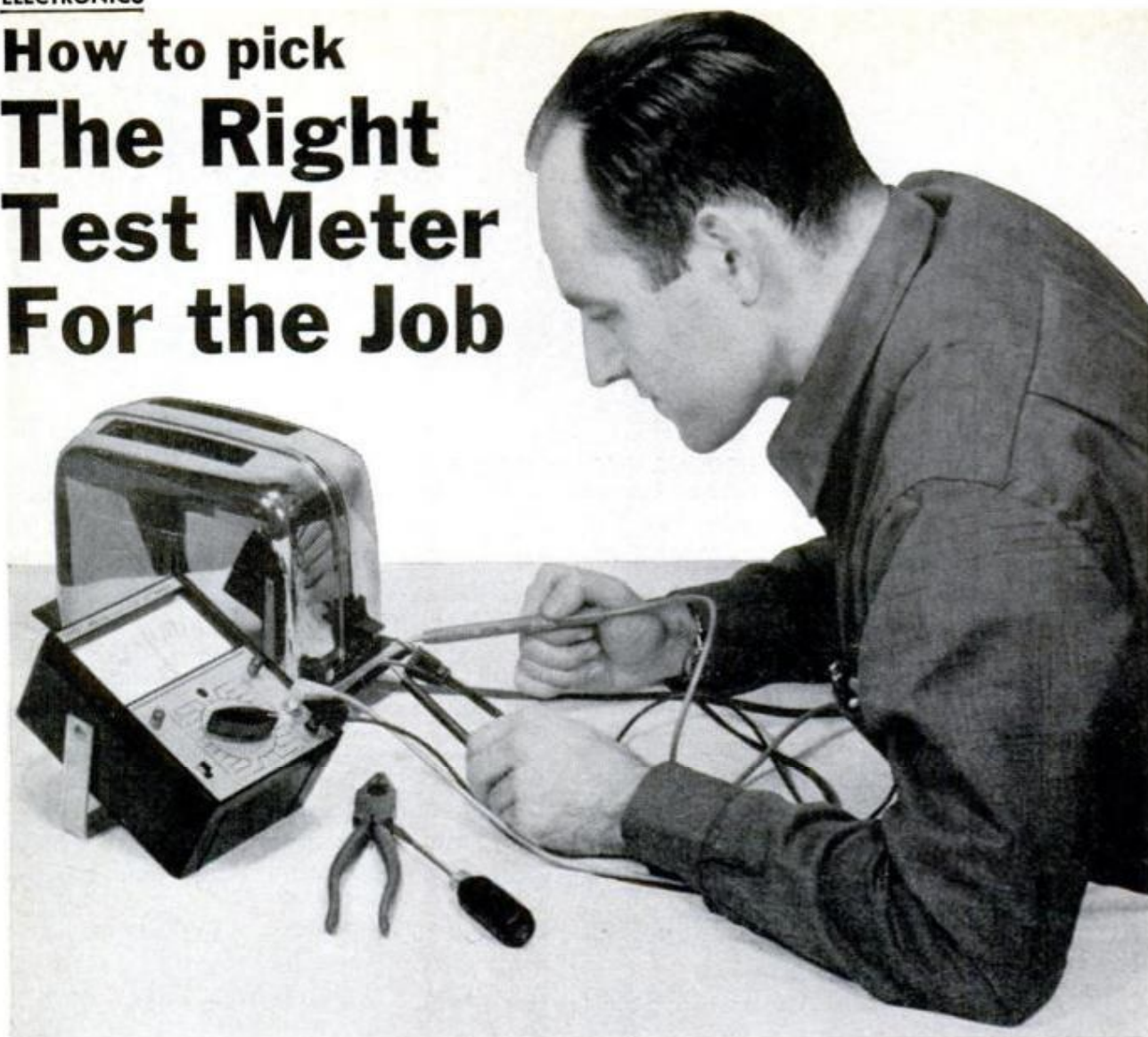
TOASTER HEATING ELEMENT is checked with ohmmeter scale of Triplett Model 600 transistorized volt-ohmmeter
