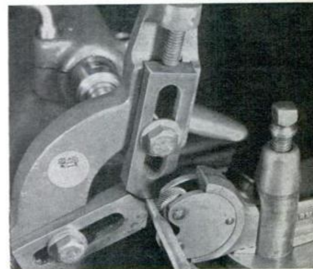
SPRINGY ALUMINUM ROD is held against knurls by a follower rest bolted to lathe carriage. In such cases, use plenty of oil
