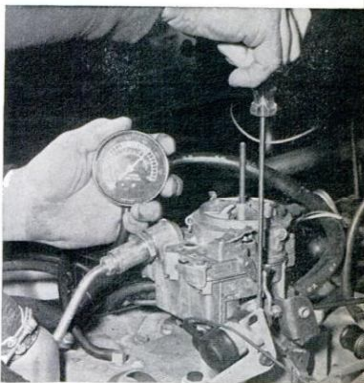
HIGH, STEADY READING during idle adjustment (above) shows carb is clean. Back out throttle stop screw (below) to shut throttle valve for cranking test
