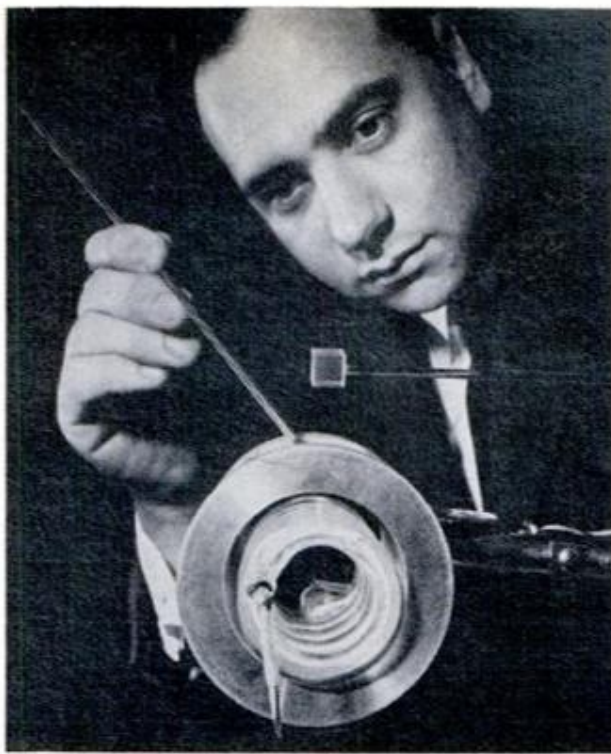
SYNTHETIC RUBY CRYSTAL , the tiny cube at center above, is the heart of this laser setup at Hughes
