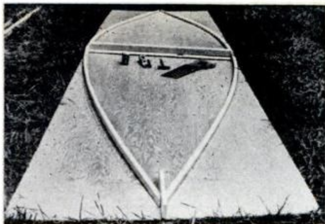
CUTTING PATTERN for the bottom panel is arrived at by bending the chines around beam-width crosspiece
