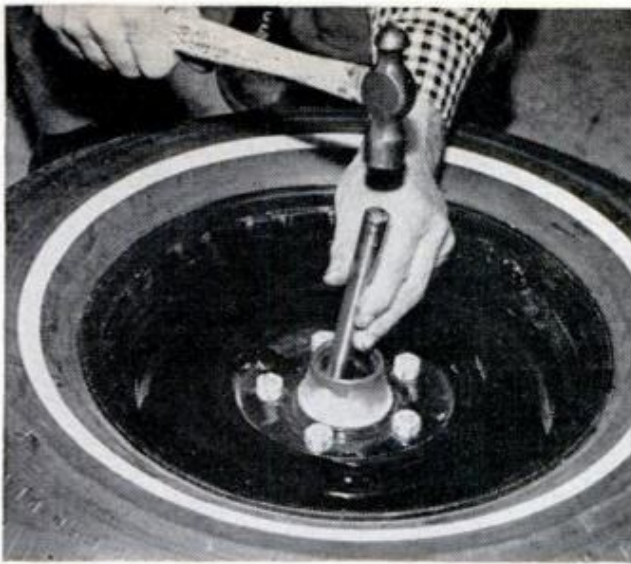
INNER BEARING can be popped from the wheel hub by tapping it with a drift. Remove cups the same way
