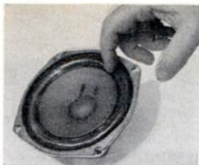
SPEAKER CONE of acoustic suspension design has flexible mounting for good bass, plastic-coated center area for tweeter action
