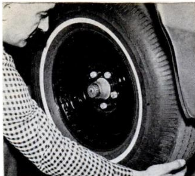
OUTER BEARING can be popped from its seat by pulling the wheel toward you and then pushing it back
