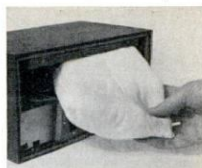
SOUND DAMPENING action in KLH tabletop is provided by fiberglass pillow. No hot tubes will burn it with solid-state design
