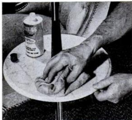
PLASTIC COATING SEALS pores in marble and other porous surfaces so stains can't enter
