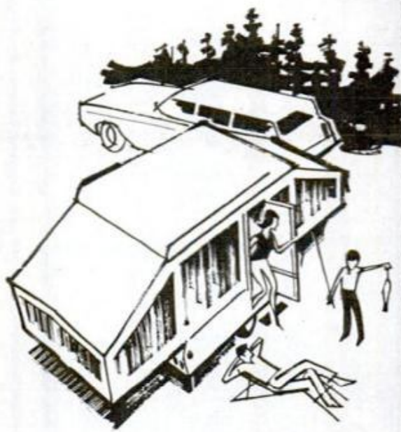
Hard-top goes up, bed wings slide out simultaneously with easy cranking motion.
