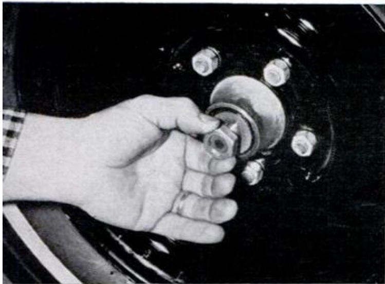
WHEEL BEARING ASSEMBLY , removed from spindle, is shown in exploded view at top. Photo above shows lock-adjust nut being removed, revealing thrust washer which guards outer bearing. Clean the spindle thoroughly, as shown below, before popping bearing
