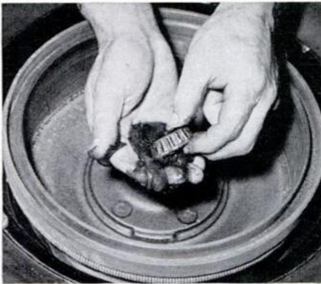
ALWAYS HANDLE BEARING by its race and don't skimp in working grease between bearing's needles
