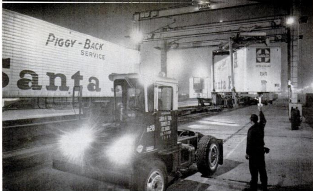
AT LOS ANGELES YARD, Super C is straddled by giant cranes that start to remove the first piggyback trailer one minute after the train came to a halt. The entire 11-car train was unloaded within 30 minutes
