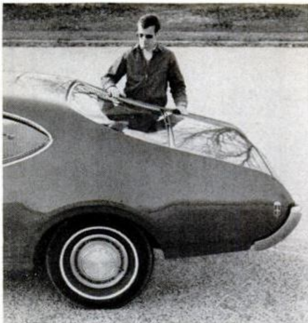
REAR END TREATMENT , while a style success, is controversial for its visibility and snow problems
