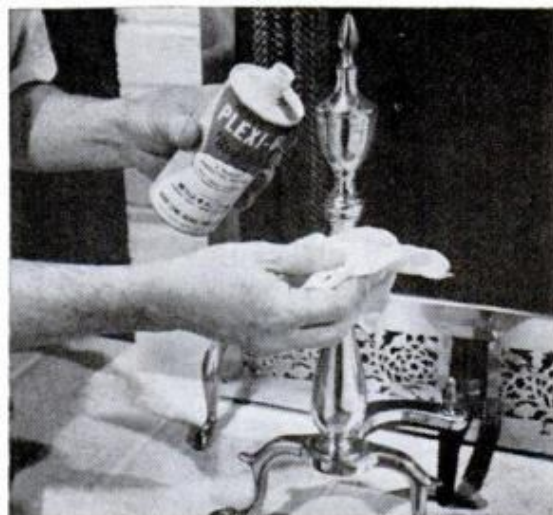
REGULAR BRASS POLISH won't stop tarnish for very long, but a coat of liquid plastic will
