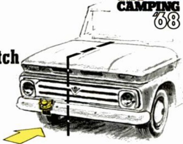
Mount front bumper hitch off center so driver can see.
