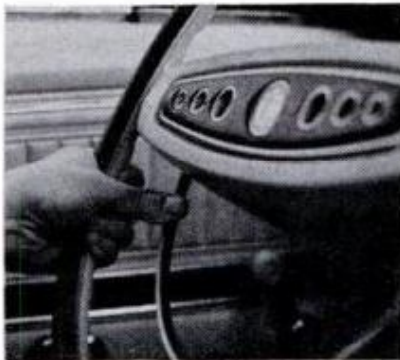
HORN RING is set too far below wheel for quick reach with thumb
