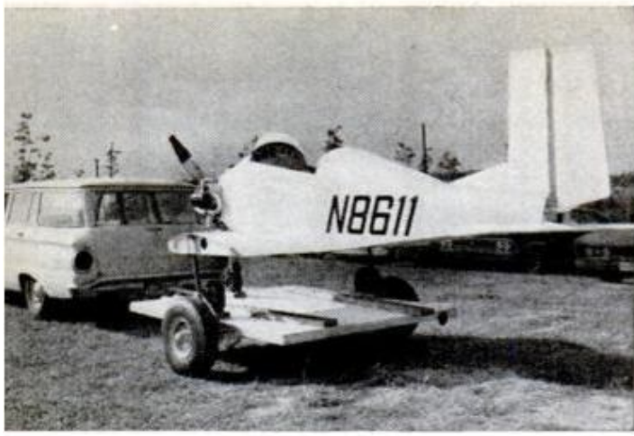
JEANIE'S TEENIE has removable wings which can be stowed in station wagon while the plane is towed
