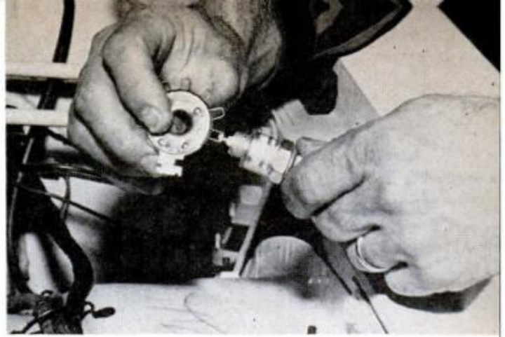
SPARKPLUG ELECTRODE GAP is set to specification when you feel a slight resistance on the wire gauge
