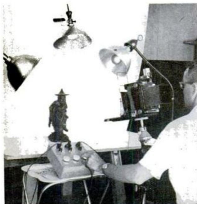
ADJUSTING FLOODS in multiple-light setups like this is easy with dimmer control alongside camera
