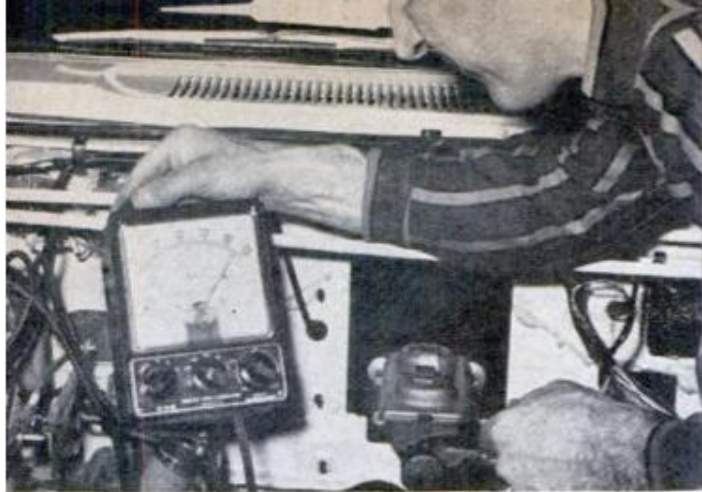
DWELL ANGLE IS READ directly in degrees on tach/dwell meter after points are set to specification
