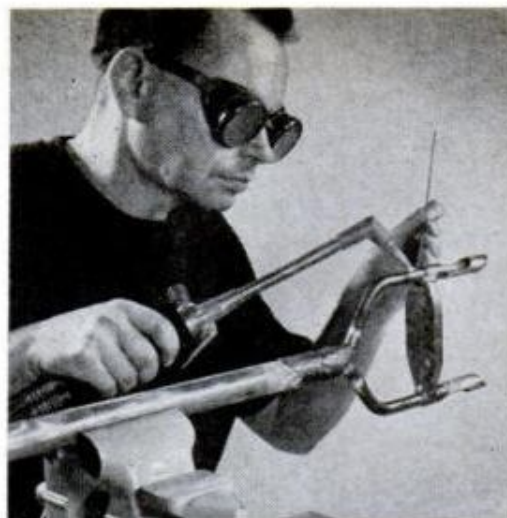
PLUG CUTTERS are lengths of steel pipe with side channels to release the plugs
