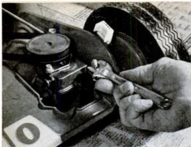
ADJUST BELT TENSION through idler or by tilting drive box, as on the Toro Pow-R-Drive shown above
