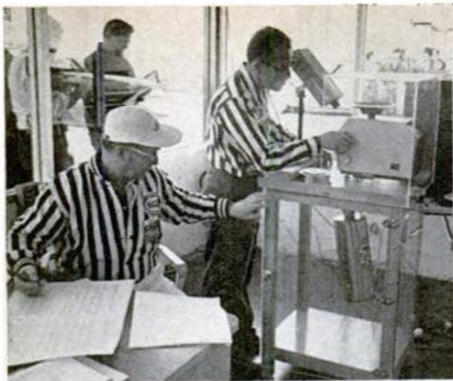
PRECISELY MEASURED FUEL supply powers car during economy run. All cars run over the same distance
