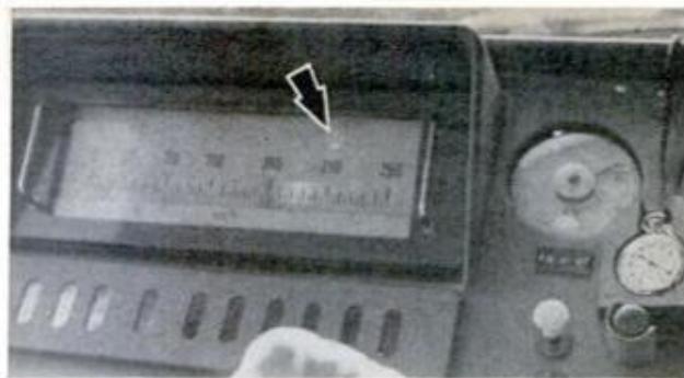
CIRCLE (arrow) lights up to show top speed allowed on any part of run; speed is controlled by Tokyo
