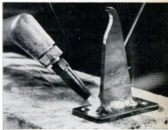
FOR SMALL PIECES that won't be hardened, use low-carbon steel. It's the cheapest and is easy to braze
