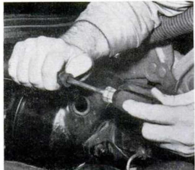
CHECK VACUUM HOSE for hydraulic fluid, presence of which indicates defective master cylinder seals
