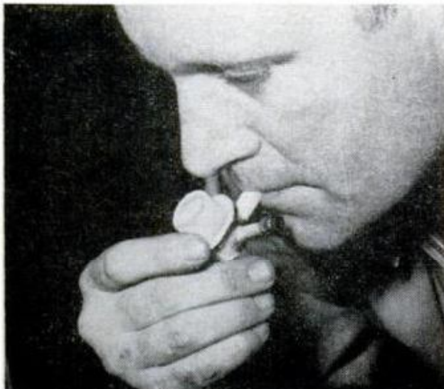
TEST CHECK VALVE simply by blowing into each end. Valve should only allow air to exit from the booster
