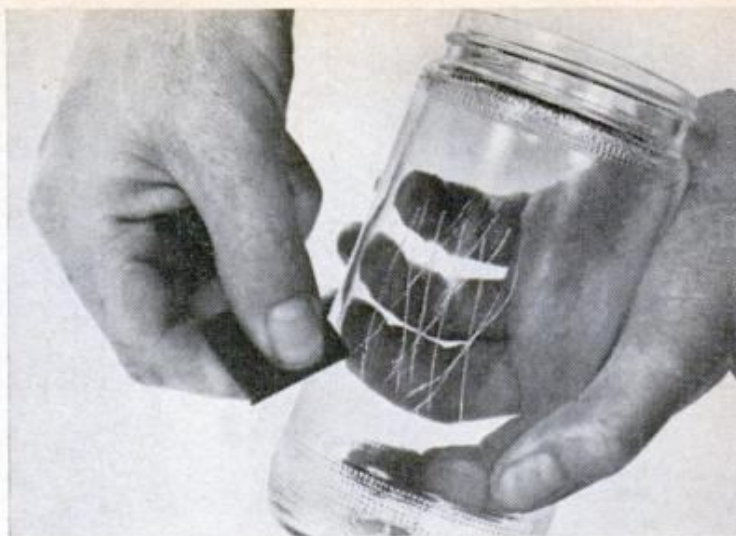
QUENCHED TOOL STEEL will scratch glass and is very brittle. Relieve brittleness by tempering in oven
