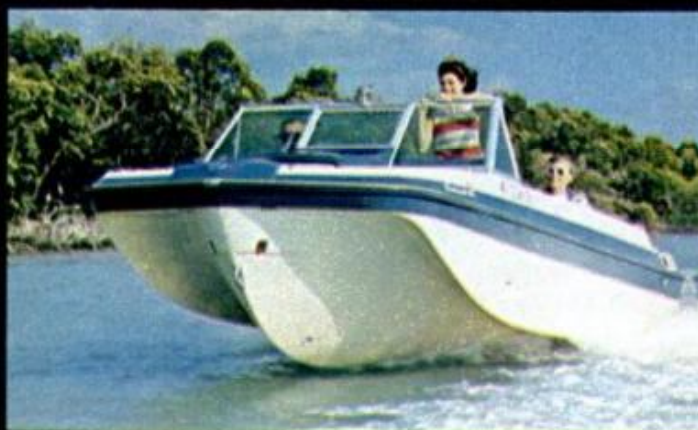
EVINRUDE ROGUE II , new gull wing for '68, is a 19-ft., 210-hp I-O runabout with walk-through windshield and sliding hatch for easy mooring
