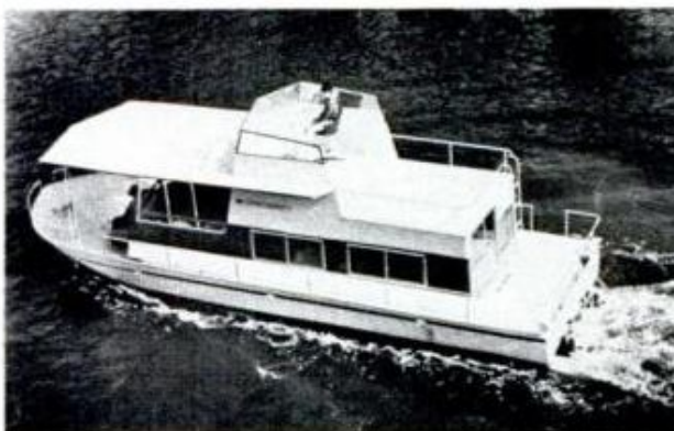
40-FT. RIVER QUEEN sleeps six and comes with twin Chrysler 210-hp I-Os which will push it to 30 mph. Almost everything is included in the purchase price of $19,750 f.o.b. the plant in Gary, Ind. 46403
