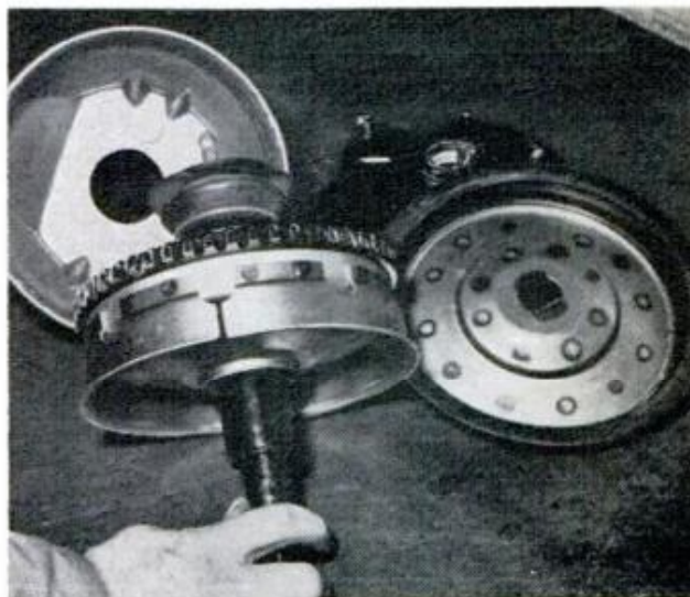
DISASSEMBLED BOOSTER reveals diaphragm, at right, and control hub assembly that houses the push rod
