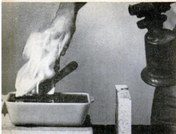
TOOL STEEL CAN BE HARDENED by heating red hot, then quenching it in a container of warm light oil
