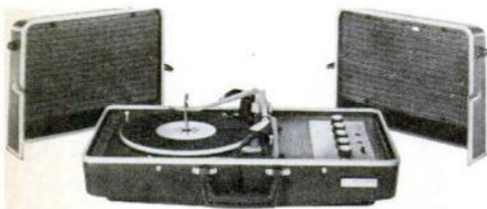
FISHER 50-B weighs 35 pounds and has detachable speakers that snap on to form the portable's cover
