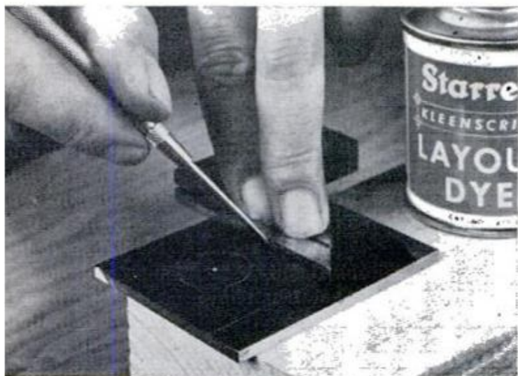
COATING STOCK WITH BLUE DYE makes scribed lines easy to see and helps simplify complex layout work
