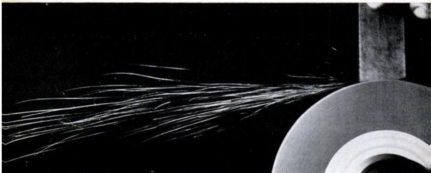
TO IDENTIFY UNMARKED SCRAP , touch it to a grinder and compare the sparks with those from known metal
