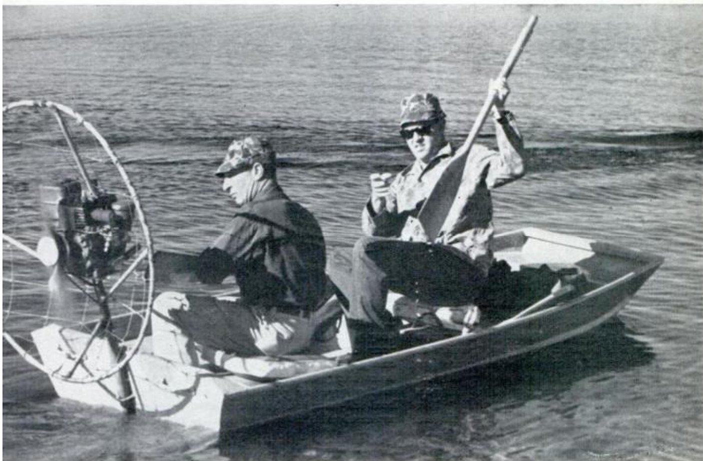
SMALL AIRBOATS are now appearing frequently. This skiff is driven by a small Briggs & Stratton motor that you can easily detach just by removing pipe attached to stern. This is slow-and-easy rig, but adequate
