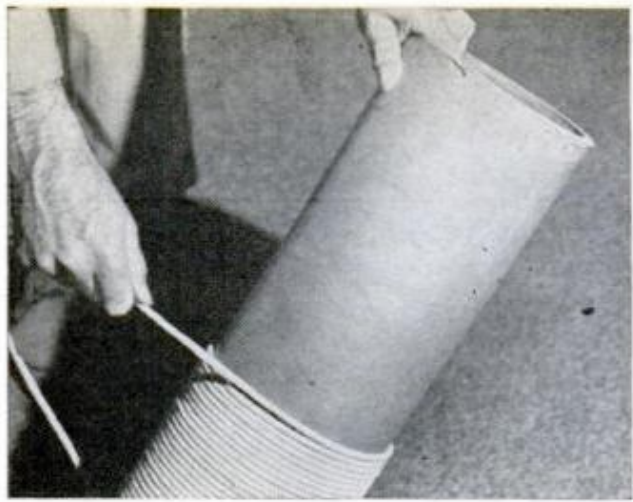
WIND RIP CORD around tube. When pulled out later, cord leaves space enough to remove cardboard core
