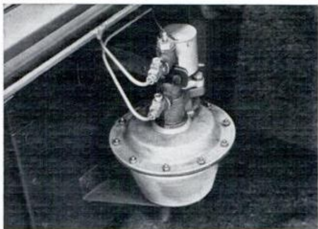
BRAKE CONTROL UNIT of Kelsey-Hayes system gives on-off braking automatically 'til skidding car stops
