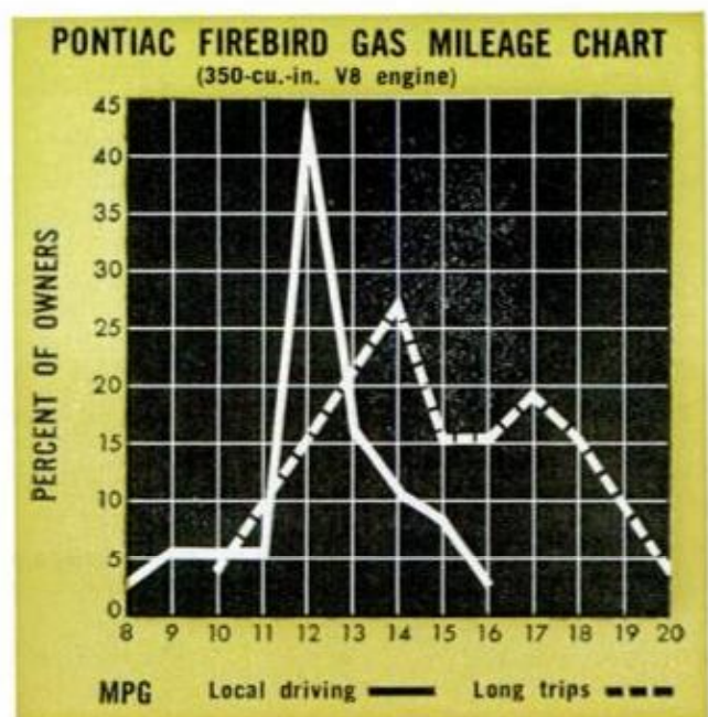
FUEL CONSUMPTION for most popular 350-cu.-in. V8 averages 12.3 mpg on short trips, 15.7 on long ones
