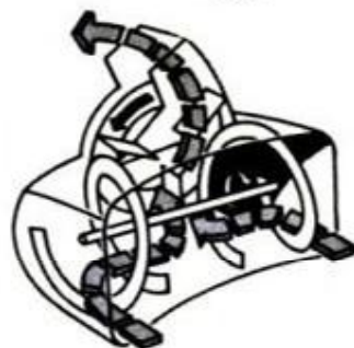
Single-stage thrower: auger whirls snow out chute in a single motion. Two-stage: auger feeds to an impeller at base of discharge chute.
