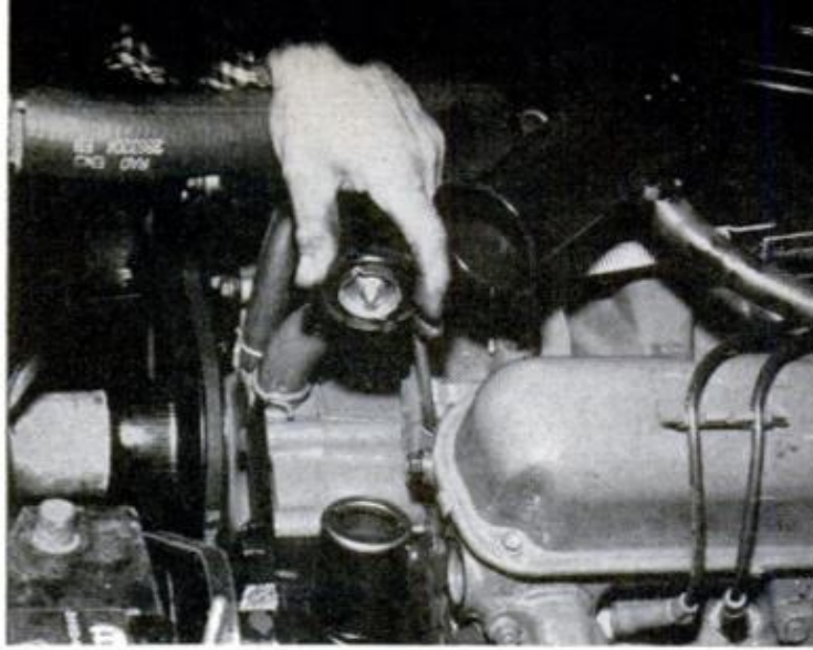
FLUID RESERVOIR CAP may not have dipstick attached. If it hasn't, fluid level is checked visually
