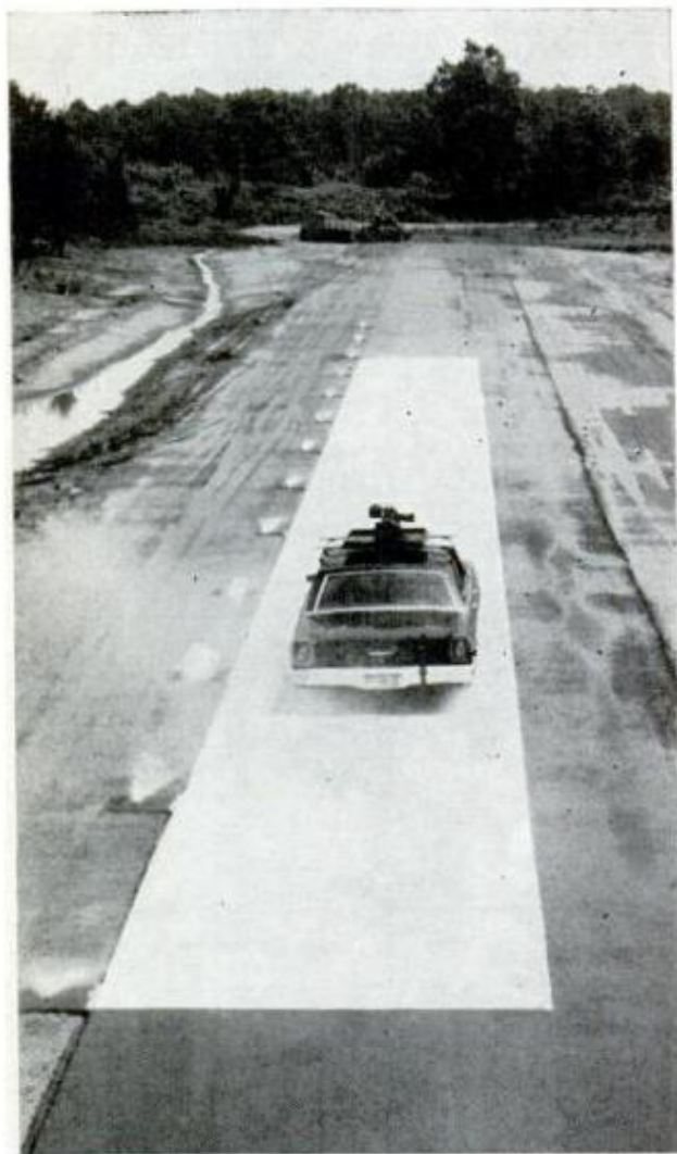
PLASTIC SHEET covers antiskid test pad. Wet down, sheet simulates extremely icy road conditions. Rest of strip is surfaced with various types of asphalt, providing the different coefficients of skid friction
