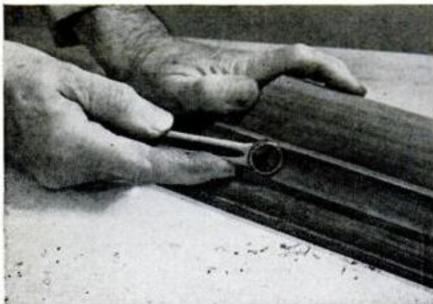
SHAVING RING made from 12-point box-end wrench makes neat work of smoothing out curves in hardwood
