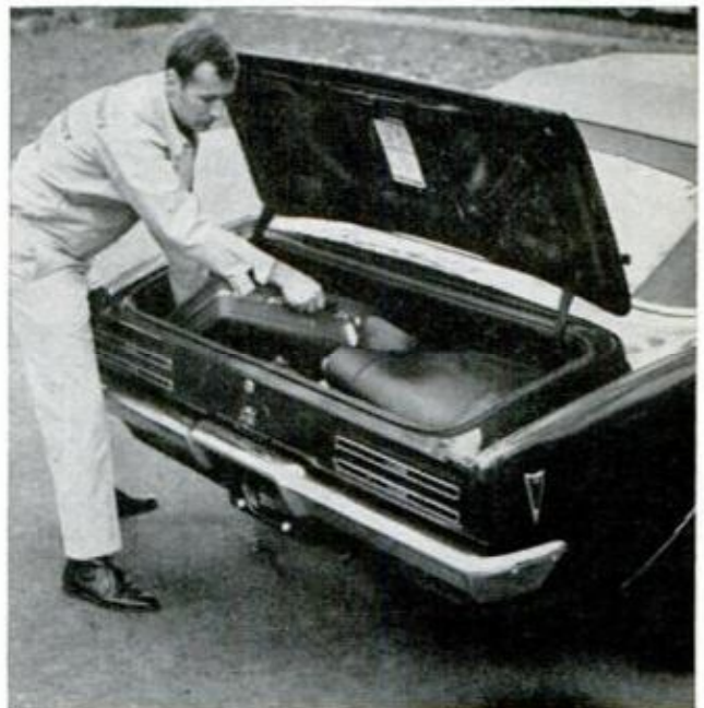
TRUNK ROOM is cut in half with conventional spare, present here, but collapsible-type is standard
