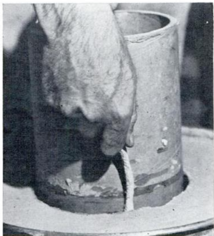
PULL THE RIP CORD and allow it to unwind from around the tube. Then remove core and clean out wax, other debris
