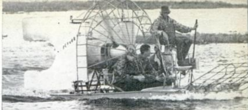
A PULLING MOTOR instead of the usual pushing arrangement makes this 220-hp, big-single-rudder machine unique
