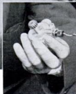
SMALL SENSOR is key to new antiskid system proposed by Bendix Corp.
