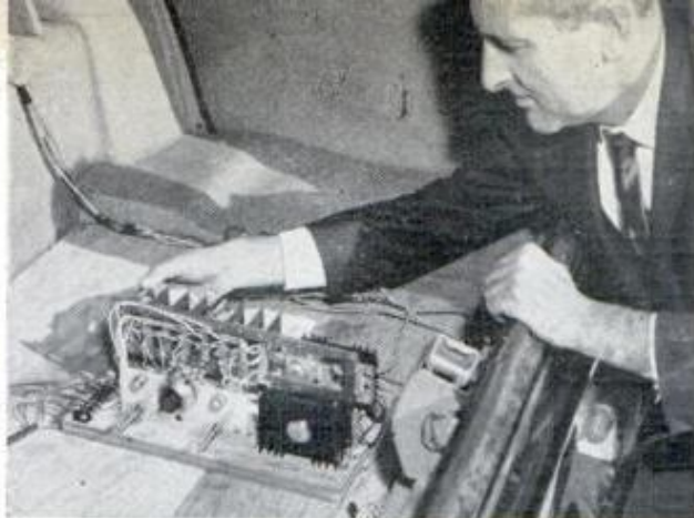
ELECTRONIC CIRCUITRY is the "brain" of new Bendix antiskid system. Production version will be smaller
