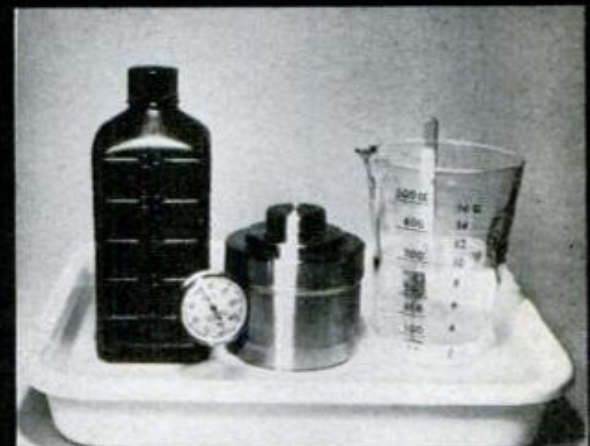
TO KEEP EVERYTHING at the same temperature, put tank and beakers in a tray of water that's been brought to the correct temperature first
