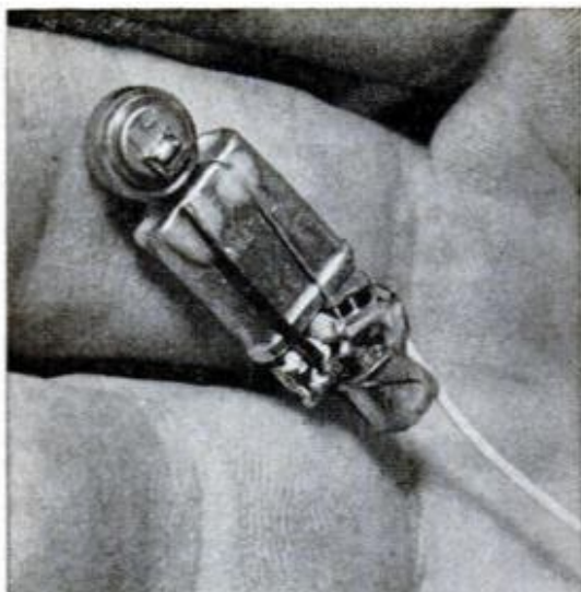
TRANSMITTER (left) with antenna and battery weighs just over 1/10th oz. It's attached to birds (right) so they can be tracked on migrations. The system was designed by Bill Cochran of the University of Illinois
