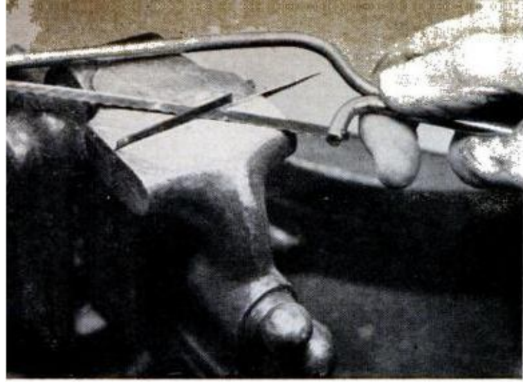
DRILL LEVERS as shown in drawings, then rough out shape by making saw cuts flush with vise jaws
