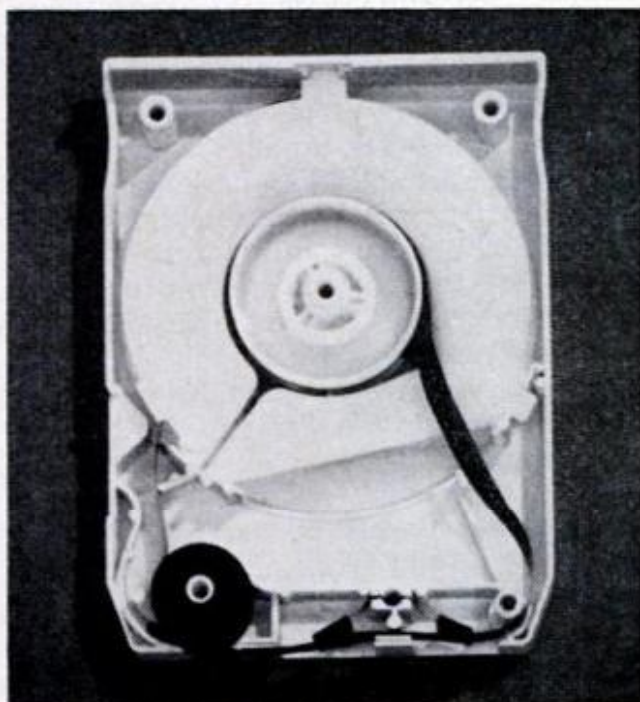
TAPE CASSETTE , above, is shown in relative size with 8-track cartridge at left. Cutaways show how tape in continuous-loop cartridge feeds in one direction only—from center of the reel past tape heads (in machine) and onto outside of reel. In the cassette, tape moves from reel to reel in either direction
