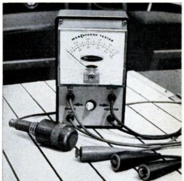
TEST METER which measures corrosion potential of the water demonstrates protection from MerCathode
