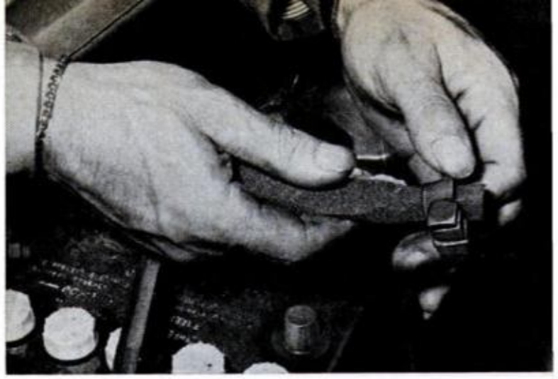
BATTERY TERMINALS and cable connections should be kept clean to give good low-resistance contact
