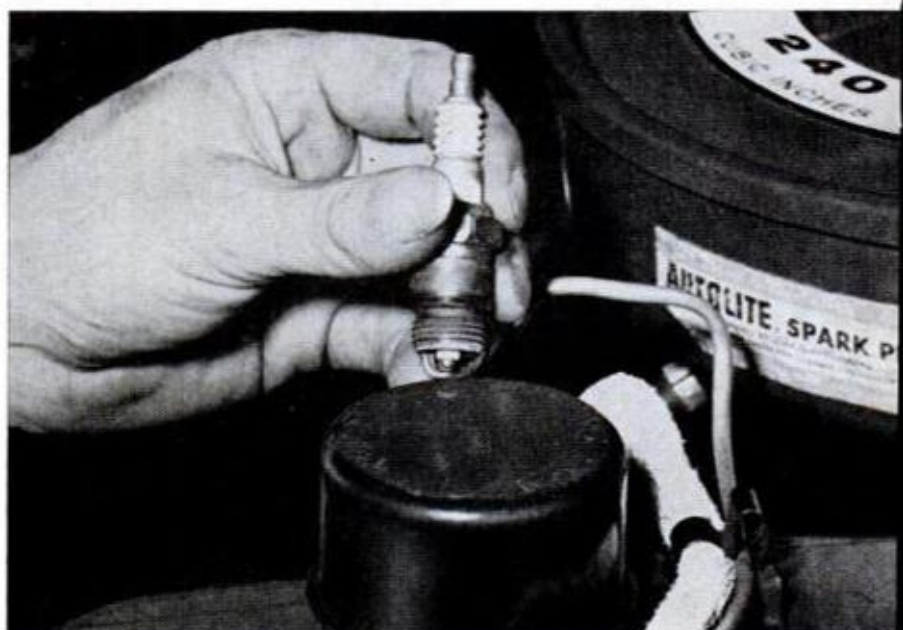
IGNITION SYSTEM must produce hot spark for cold-weather starting. Tapping plugs to close gap slightly helps in emergency
