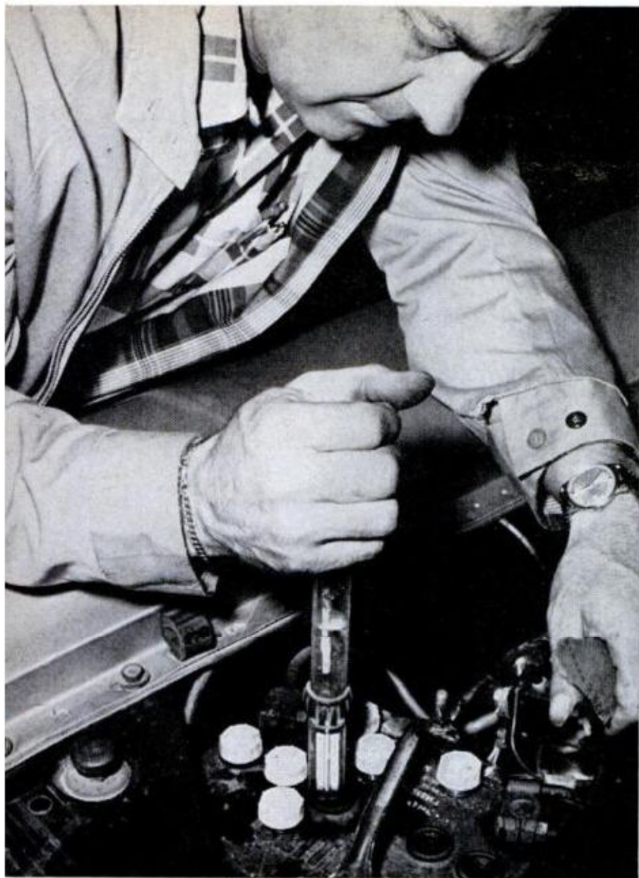
ELECTRICAL SYSTEM must provide high current for starting. Hydrometer checks battery charge, but you need cell tester, too
