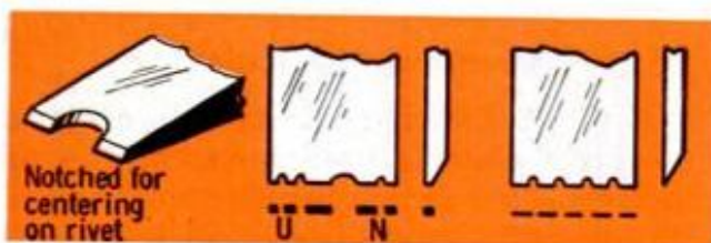
SERIES OF NOTCHES uniformly spaced and ground in edge of wood chisel makes it a perforating tool
