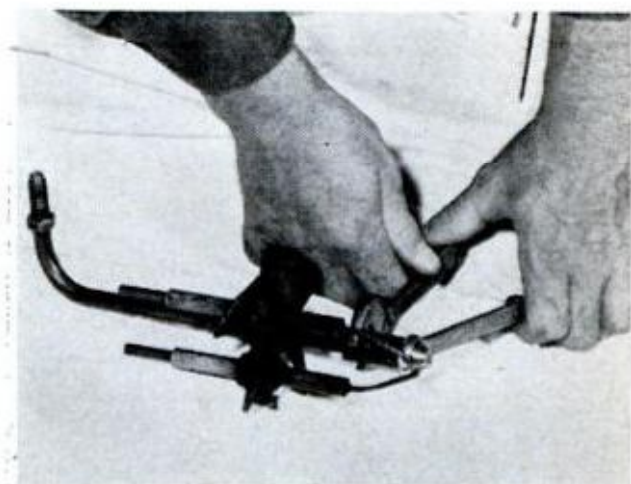
REMOVE NOZZLE with two wrenches. Clean the filter and setscrew, test nozzle and then reassemble
