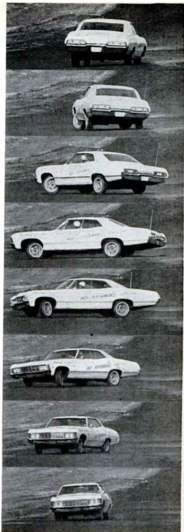
FORWARD SPIN , resulting in car doing a 180° turn-about, is a basic maneuver taught at the school. Technique involves simultaneously hitting brakes, flipping the steering wheel over fast and hard to break rear end loose and swing car around. As nose comes around, power is applied, car straightens out
