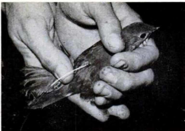
TRANSMITTER (left) with antenna and battery weighs just over 1/10th oz. It's attached to birds (right) so they can be tracked on migrations. The system was designed by Bill Cochran of the University of Illinois
