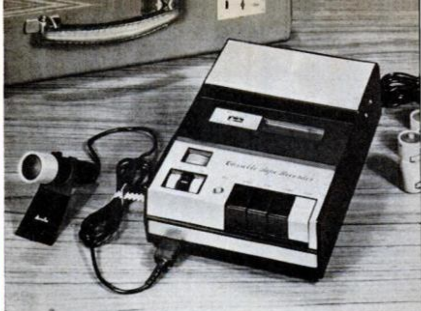
ARVIN PORTABLE , above, features combination record-level (VU) meter and battery strength meter. The $70 recorder comes with a.c. cord and mike with remote on/off switch. Sony portable, left, is smallest you can get. Price is $100
