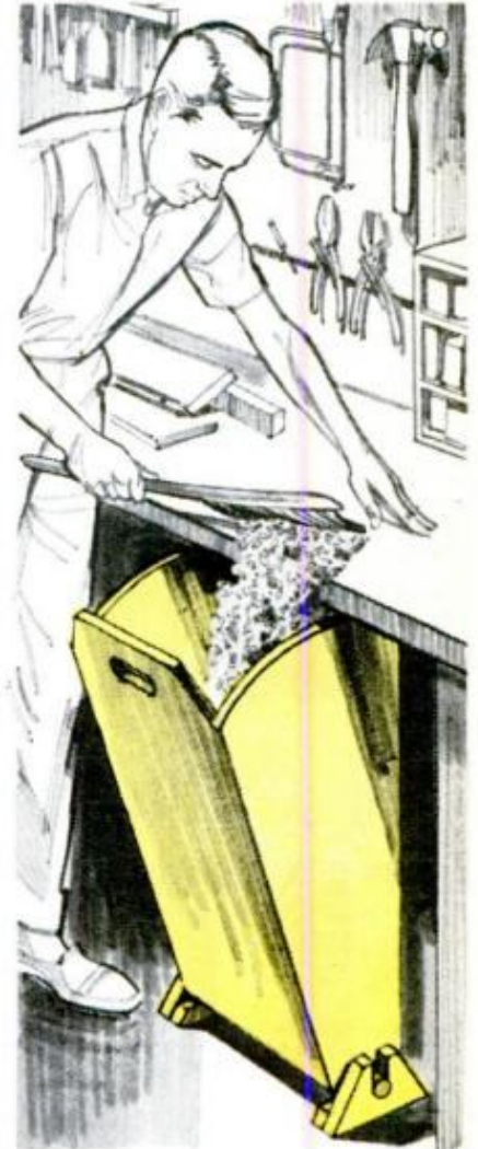
TRASH BIN swings out from under your workbench, pivoting on a 1-in. supporting dowel which passes through box at the bottom. Ends of dowel rest in notched blocks anchored to floor, permitting bin to be lifted out easily for emptying when it becomes full
