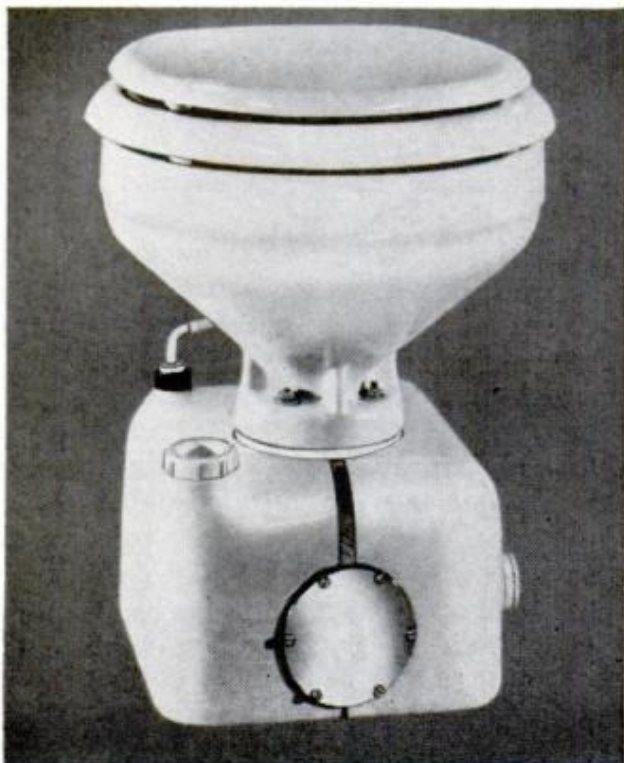
RARITAN CROWN HEAD grinds waste, galley garbage, adds chlorine from tank, discharges overboard
