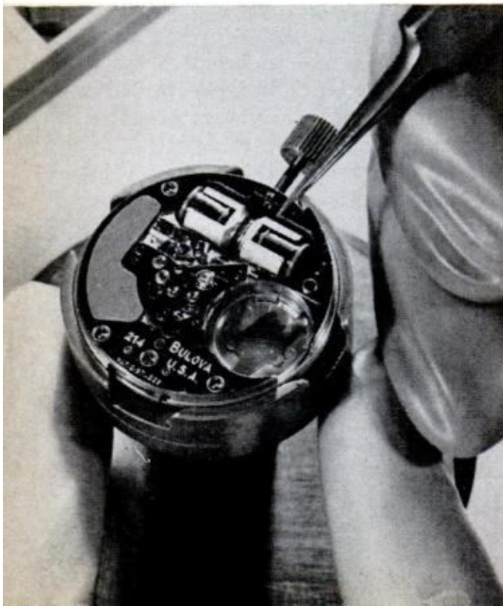
TRICKY WORK: A Swiss watchmaker painstakingly assembles a row of Eterna watches held in a shallow tray above. Below, a technician wears gloves while adjusting a Bulova Accutron to keep the parts clean
