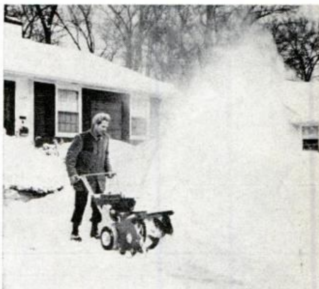
DUAL-STAGE WHEELHORSE 26-in., 7 hp ($360) shows advantage of blowing: Snow can be lofted over bank
