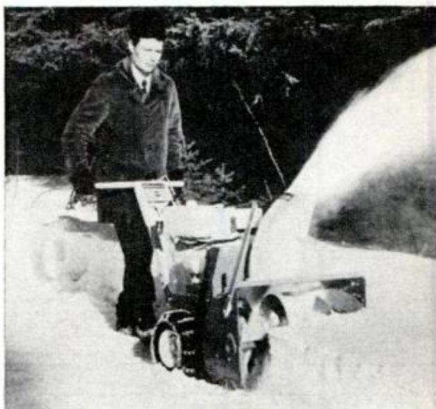
GILSON'S DUAL-STAGE 7-hp model costs $375. Under ideal conditions, it throws snow up to 40 feet
