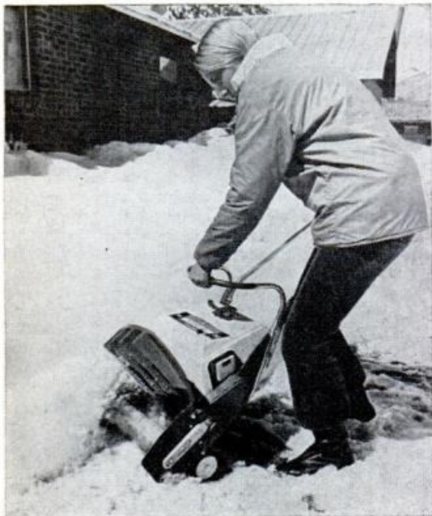
AMF HUSKY, JUNIOR cuts 14-in. swath, has polyethylene rotor. Gas-powered, it sells for $100
