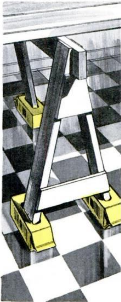
SAWHORSE SHOES will protect highly polished tile or hardwood floors during remodeling work. Just cut narrow slots in front panels of four cardboard milk cartons and slip these on feet of sawhorse. Angled tops act as runners to ride over any irregularities
