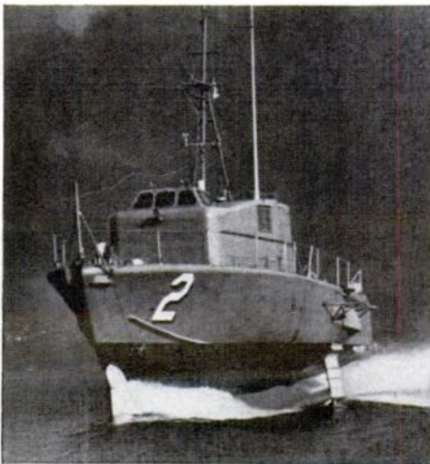
GUNBOAT TUCUMCARI , built by Boeing, features canard configuration, with one foil forward, two aft
