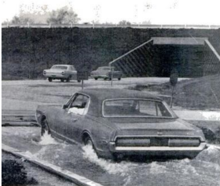
SALTWATER BATH gives Cougar an hourly dunking on its 25,000-mile durability cycle at Lincoln-Mercury
