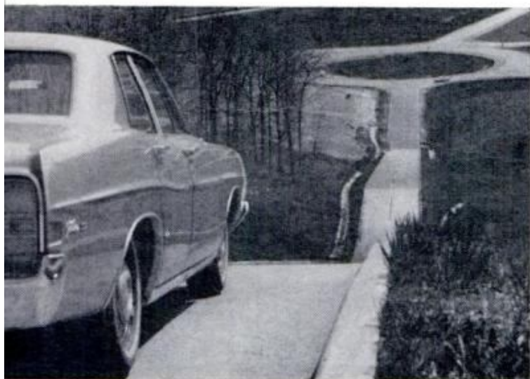
STEEP GRADE , one of several at Ford's Romeo, Mich., proving grounds, tests drivetrain under load
