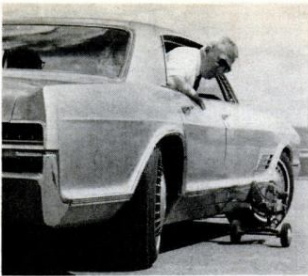
STEERABLE REAR WHEELS are part of GM research car which simulates various handling characteristics
