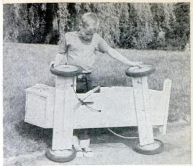
CHASSIS VIEW shows how speedometer cable goes out bottom and back to rear wheel. Rear axle board is nailed to chassis, front one bolts to plywood
