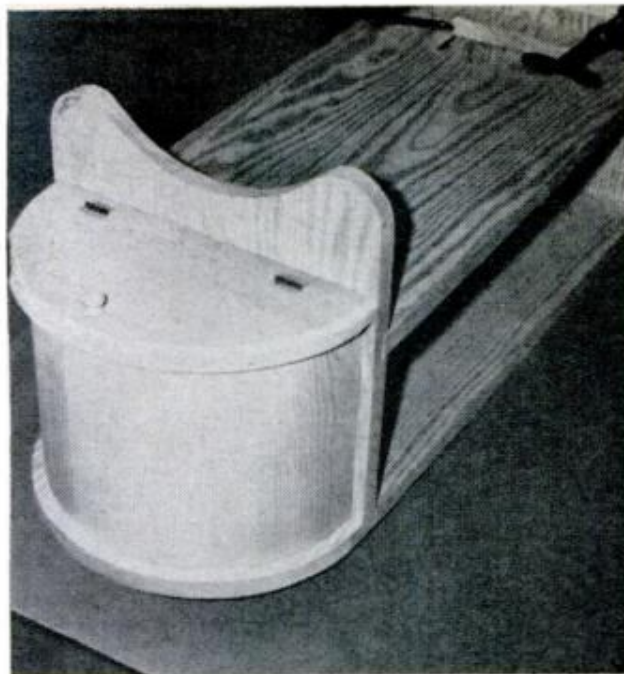
BUCKET ENDS are turned as a single drum, then are cut in half. Lid overlaps drum as does table bottom
