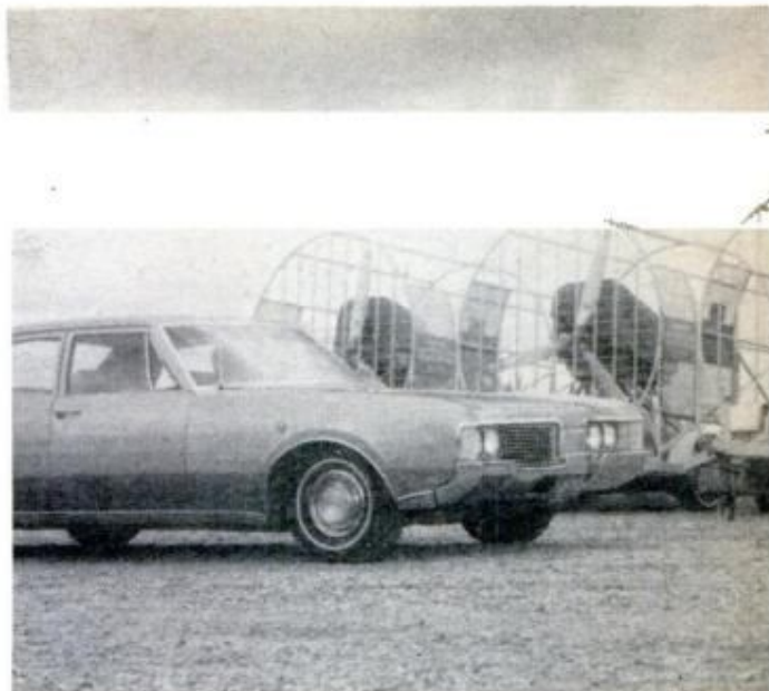
CROSSWINDS of controlled magnitude are generated by huge aircraft engines at General Motors facility
