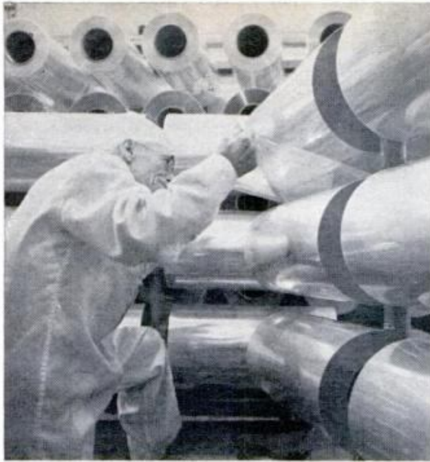
TAPE BASE MATERIAL is inspected before being coated with magnetic oxide particles and slit to ¼ in.
