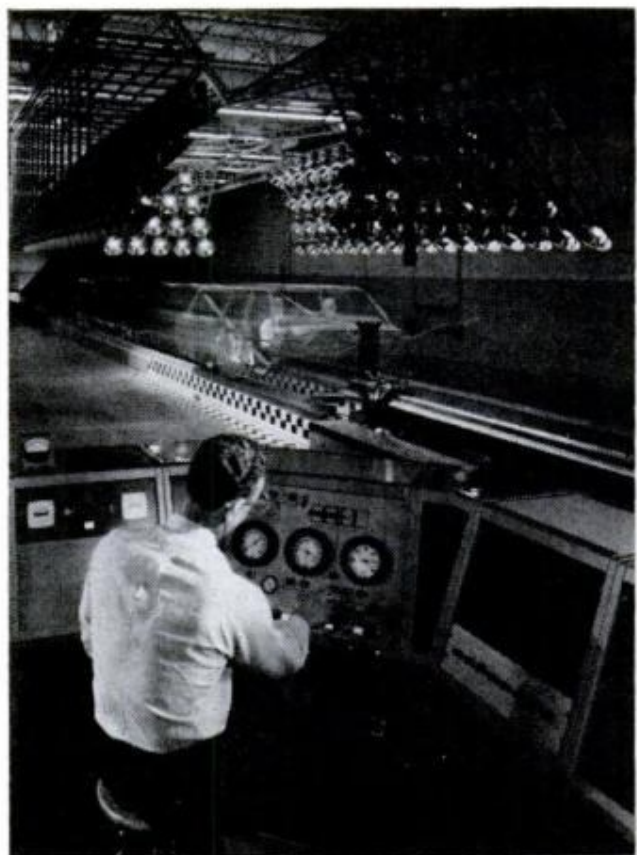
IMPACT-SIMULATOR SLED uses vertical post to ram car down track. Impact occurs at beginning of run
