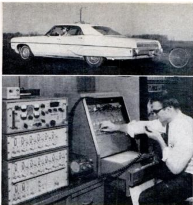
COMMUNICATIONS HOOKUP from car to computer transmits design data which is analyzed in seconds
