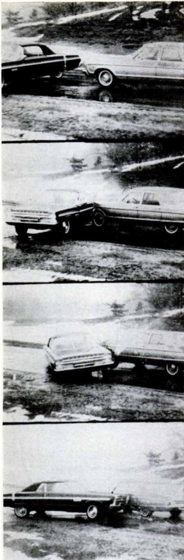
SAFETY RESEARCH takes a large toll of cars on the proving grounds. Remotely steered car is coasted down a grade at a speed of 40 mph in this sequence of photos of a broadside collision. Instruments in the cars, and often in dummy passengers, record forces
