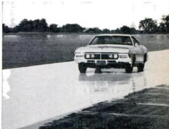
SLICK SURFACE at GM's Milford, Mich., proving ground is used to research four-wheel antilock brakes
