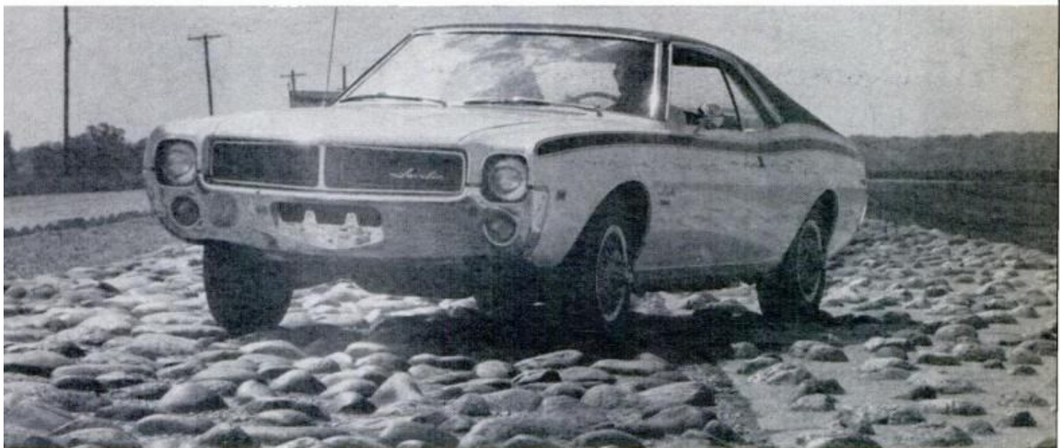
ROCKY TEST BED at American Motors' Burlington, Wis., facility can take a car apart at the seams
