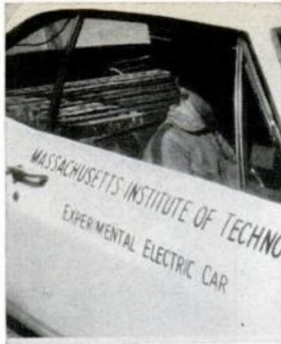
BACK SEAT AND FRONT BOOT contain 320 cells arranged in four, 80-cell, 100-volt packs. Headlight cutouts are also cooling-air scoops
