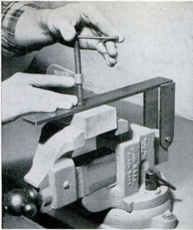
CLAMP THE ARM of the bracket to the legs and weld. Make arm longer if a counterbalance is needed
