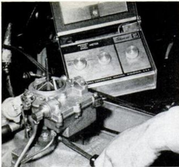
FUEL-AIR RATIO or "richness" mixture is adjusted at idling speed when engine is hot to cure stalling problem. Richness is adjusted for specified idle rpm
