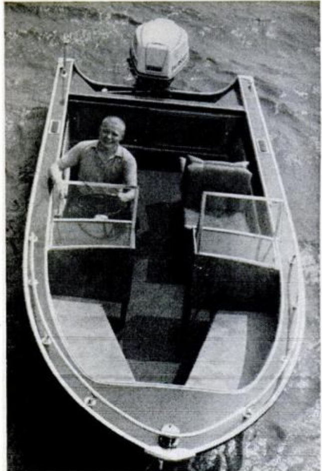
CONCAVE-V HULL features a basic V shape to smooth out chop but curves down at chines for extra lift
