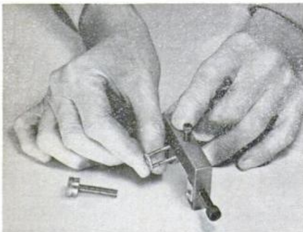
MICROMETER STOP provides control of travel in sideways direction, is calibrated to 1/1000 in.
