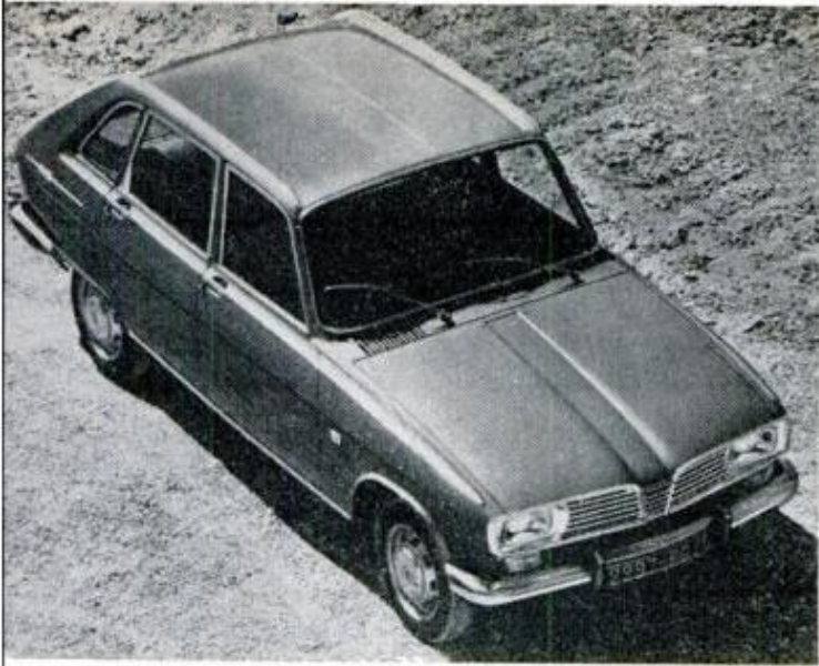
RENAULT 16 , bigger, more advanced than models sold here, has front drive, 4-wheel independent suspension
