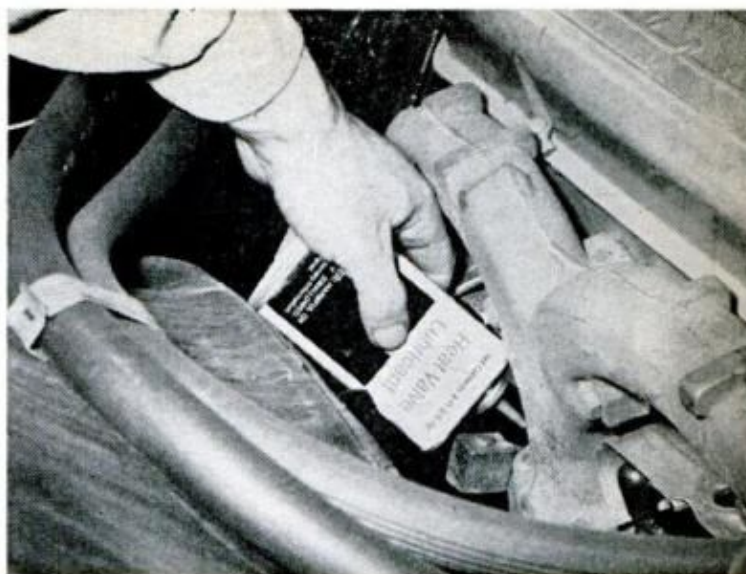
MANIFOLD HEAT-CONTROL VALVE that is stuck open prevents engine from coming up to temperature quickly. Apply lubricant if it doesn't move freely
