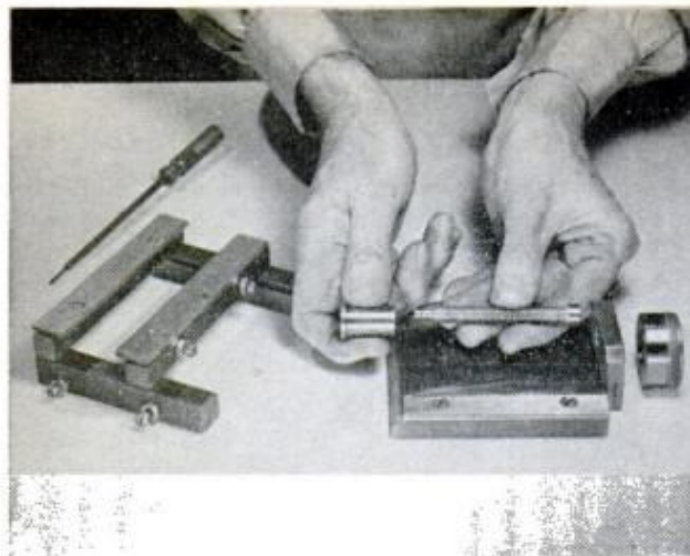
FEED SCREW is secured to frame member C with setscrew. Knob and sleeve ride screw, control slide
