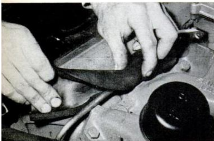
VAPOR LOCK , a sure cause of stalling, can be permanently remedied by wrapping fuel lines with a plastic foam or similar type of insulating material
