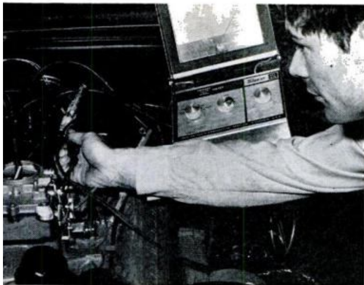
FAST IDLE ADJUSTMENT ensures that enough fuel reaches cylinders of a cold engine to prevent stalling. Screw, which rests on cam, is turned to adjust
