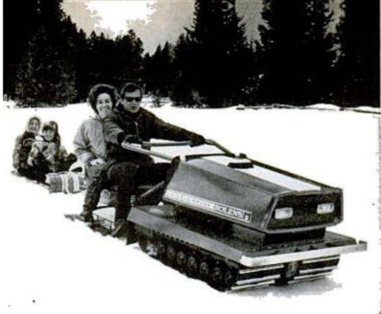
DIABLO ROUGE is the most unusual-looking machine of all the snowmobiles on the market today. You sit on a sled and steer "tractor" by moving handlebar
