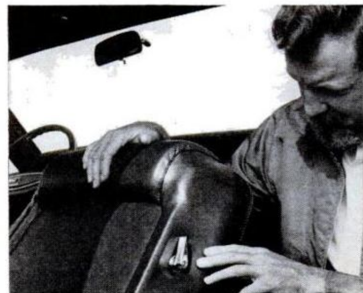
COUGAR'S FRONT-SEAT BACKREST LOCK is easily accessible. All 1968 two-door models have them
