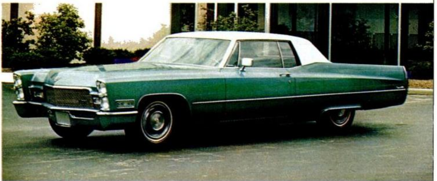
CADILLAC has new grille, elongated hood to accommodate recessed windshield wipers, is slightly longer
