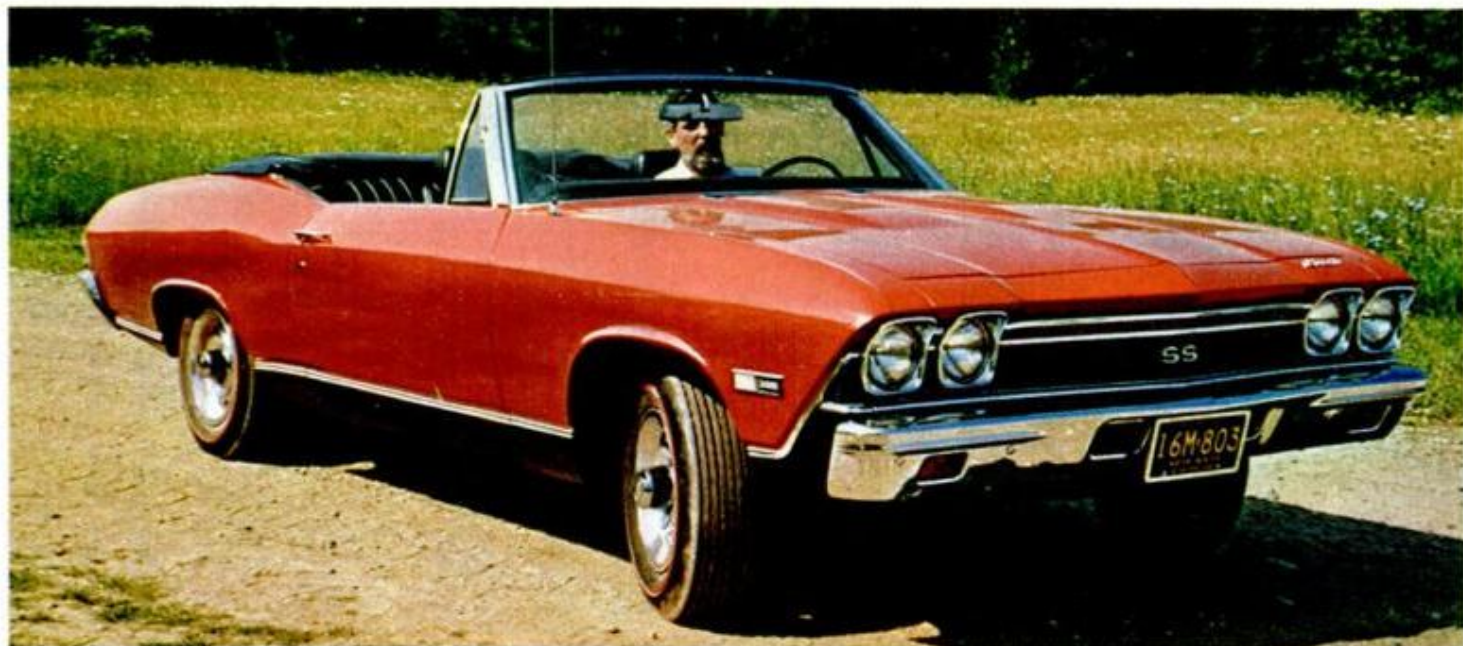
CHEVROLET CHEVELLE SS tops newly styled line. Coupes, convertibles have 112-in. wheelbase; others 116
