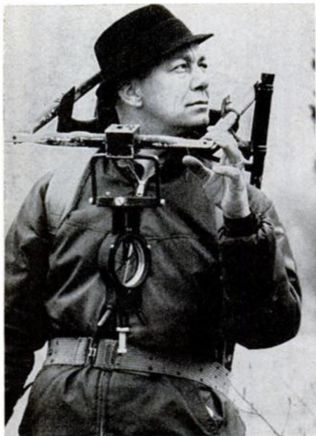
"HAP" JAMIESON uses gear of tubing to hold magnetometer in search for variations in magnetic field
