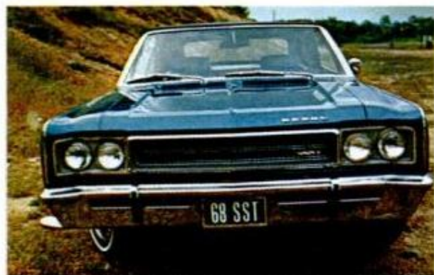
AMC REBEL SST tops series, has new hood lines, new injection-molded plastic grille
