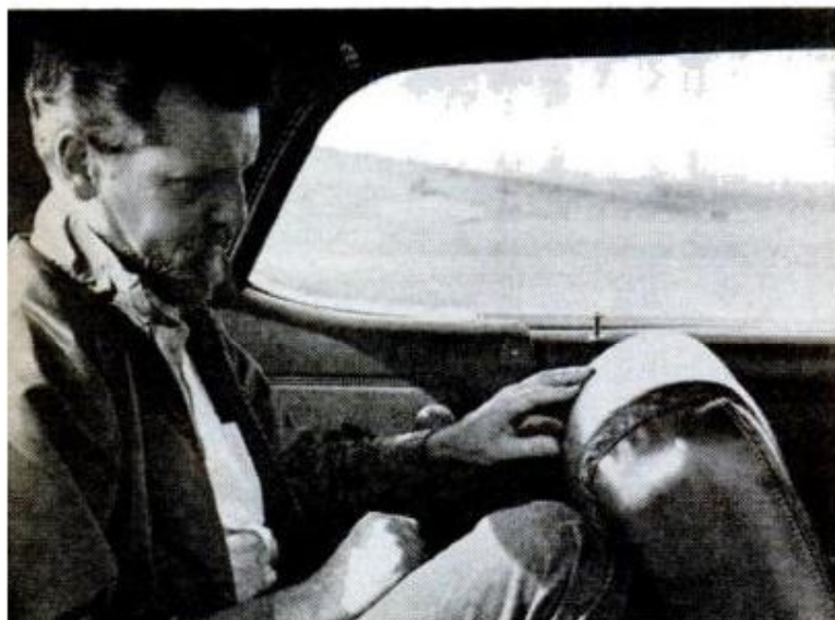
PADDING ON REAR OF FRONT SEAT of Cougar protects knees and heads. All cars have it this year
