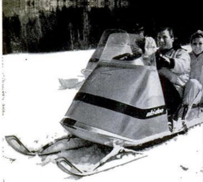
SKI-DOO is a smooth-looking machine this year, with a retractable headlight in the hood. This cuts down on wind resistance during high-speed races
