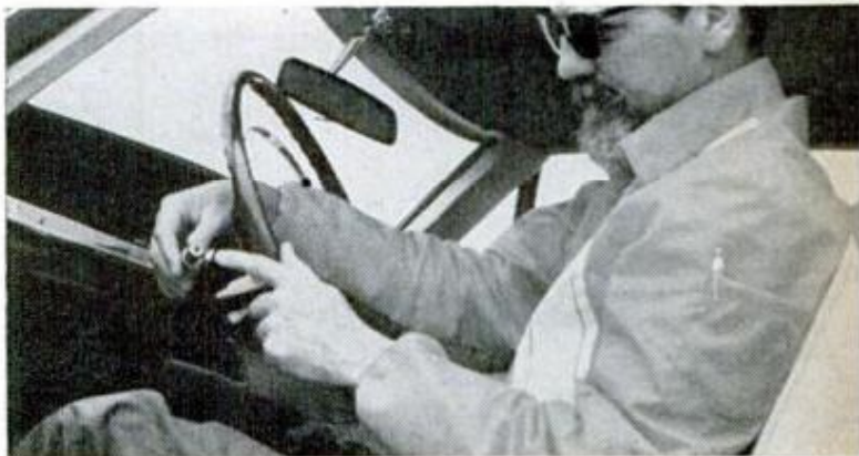
SPEED CONTROL on Chrysler cars is set using the actuator located on the end of the directionals lever
