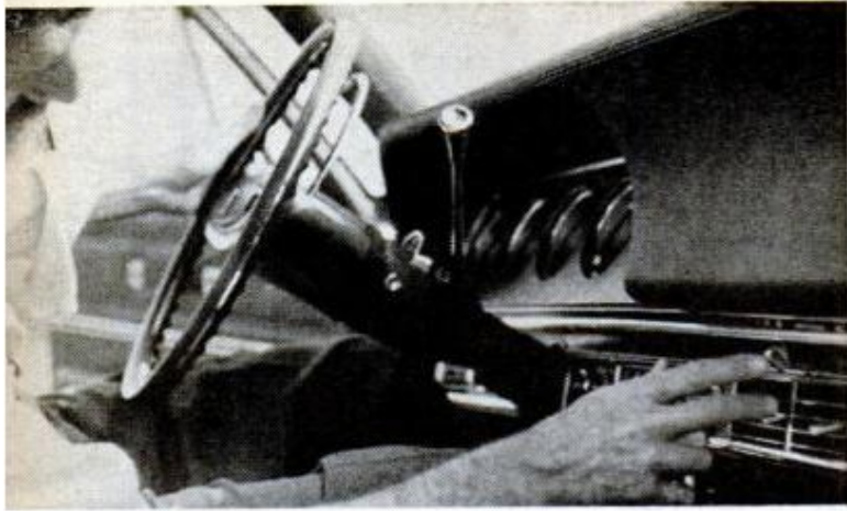
PEEK-A-BOO HEATER-CONTROL MARKINGS on new Mercurys are rough to see around corner on dash
