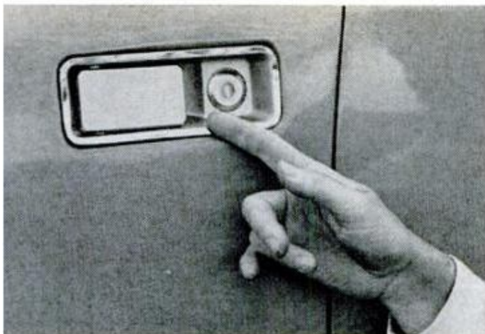
SLICK RECESSED DOOR HANDLE is American Motors' design. Fingertips go between lock and the catch
