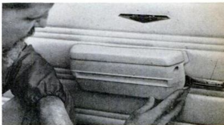
"OLD-FASHIONED" DOOR HANDLE is placed forward of and partly enclosed by armrest on GTO Pontiac
