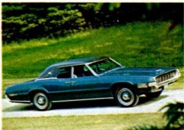
FORD THUNDERBIRD has latticed, recessed grille, slotted, two-piece bumper to improve engine cooling
