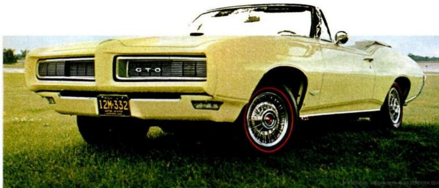
PONTIAC GTO tops Tempest line, features new nonmetal, impact-absorbing bumper as part of hood styling
