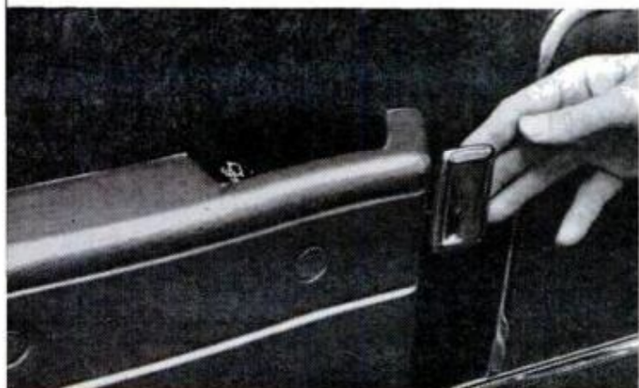
AMERICAN MOTORS DOOR RELEASE is on forward end of armrest. Locking lever is also in the armrest
