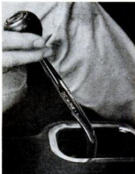
BOOT AT BOTTOM of Pontiac gear shift lever forms a debris-collecting hole
