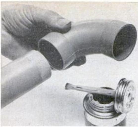
ELBOWS, TEES AND OTHER FITTINGS are "fused" to tubing with PVC cement which produces airtight joints in system. Cement is potent; avoid breathing
