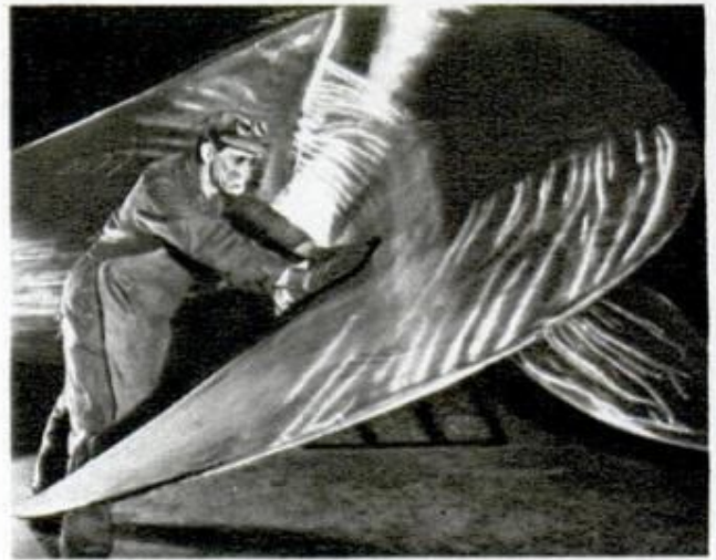
SIX-BLADED PROPELLERS for the new liner are 19 feet in diameter—the largest on any twin-screw ship
