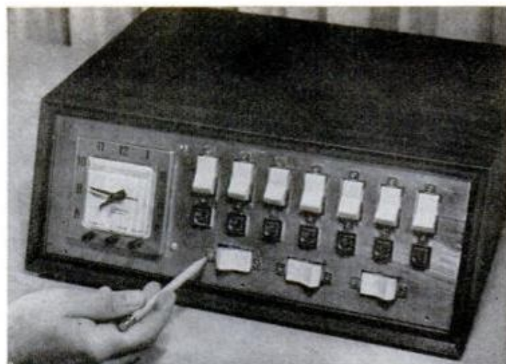
SWITCHES ARE MOUNTED using washers to adjust distance from front panel. Second panel slips over switches, lamps and clock to hide hardware
