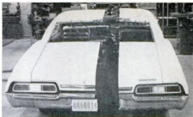
THE FORE AND AFT CUT was actually made to the right of the center line to leave the drive train intact. The left side can do 40 mph on its own
