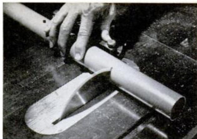
PLASTIC TUBING saws easily. If you don't have a power saw, a miterbox will assure squarely cut ends to obtain perfect fit inside the plastic fittings
