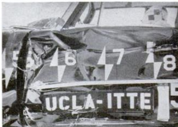
20-MPH CRASH. Photos above by Automotive Collision Research Laboratory at UCLA show effects of side-impact crash with both cars going 20 mph. Sketch shows forces acting on drivers and passengers
