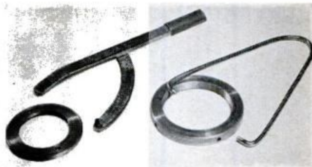
SPARTAN-LOOKING wrenches will fit most rings and perform as well as their chromed counterparts
