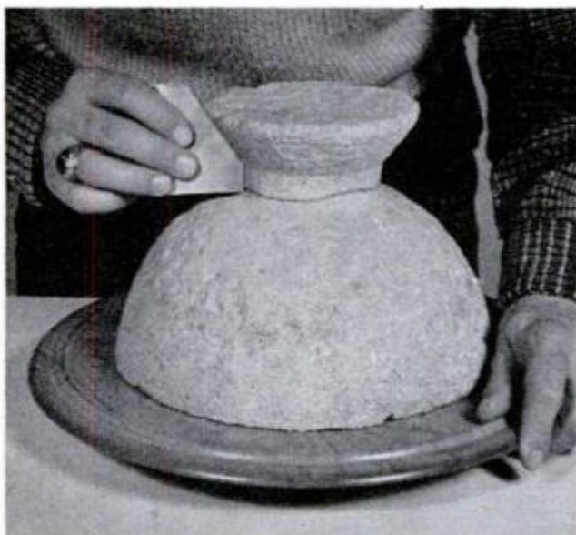
ALUMINUM TEMPLATE is applied to spinning form until the desired configuration has been reached
