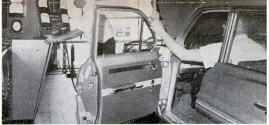
ON THE MOBIL ANALYSIS LANE , Bob Borst's Pontiac is tested with wheels turning at 60 mph. One technician operates control while a second reads meter
