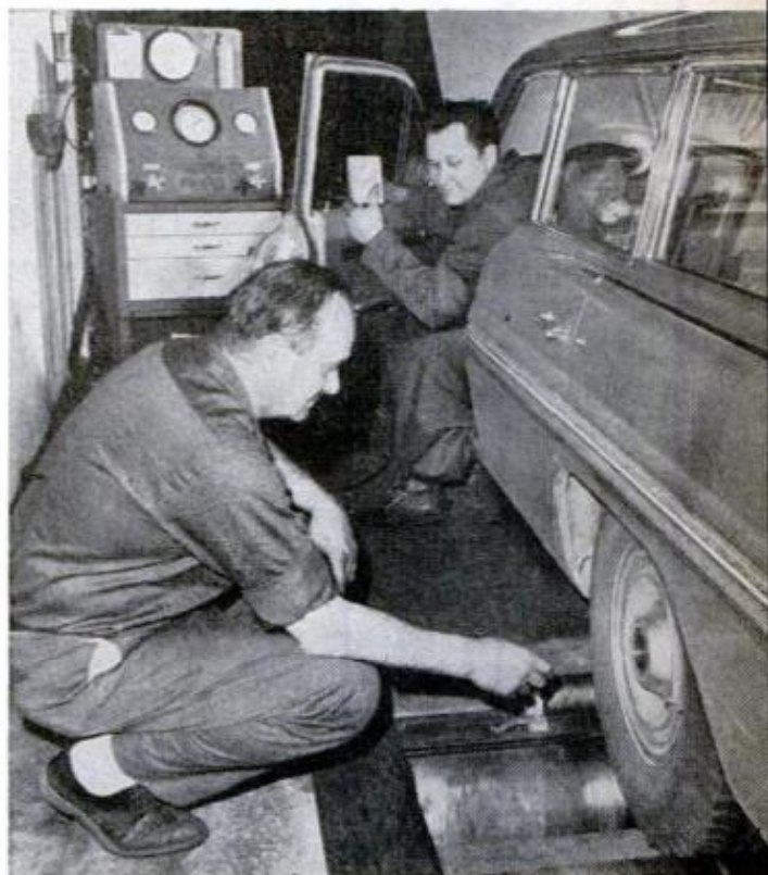
REAR WHEELS are brought up to rpm equivalent of 60 mph on the road, and the rear hub is "felt" for excessive vibration at the Polce garage
