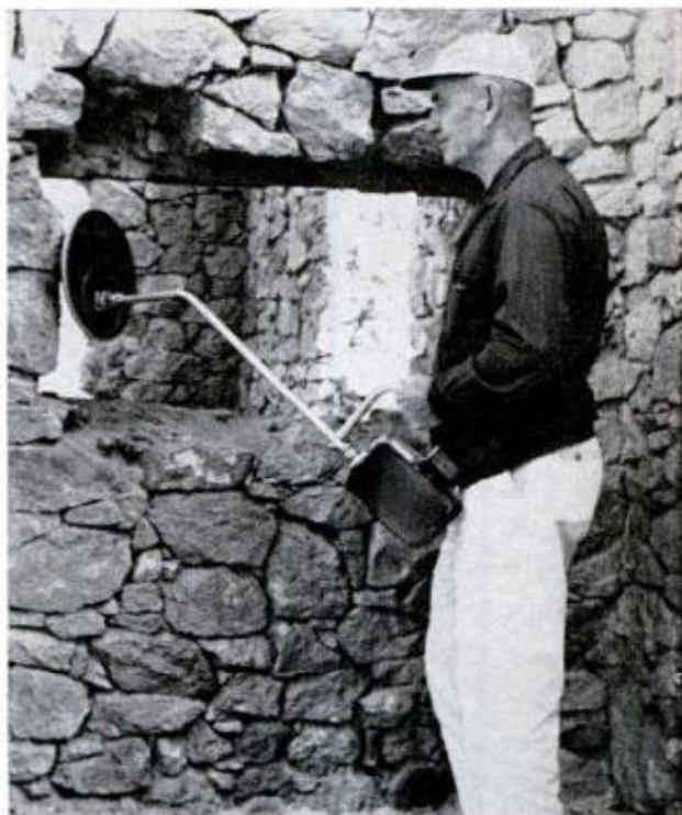
BEAT-FREQUENCY DETECTOR has a single loop at the end of a pole. It sets up an electromagnetic field that indicates the presence of metallic objects
