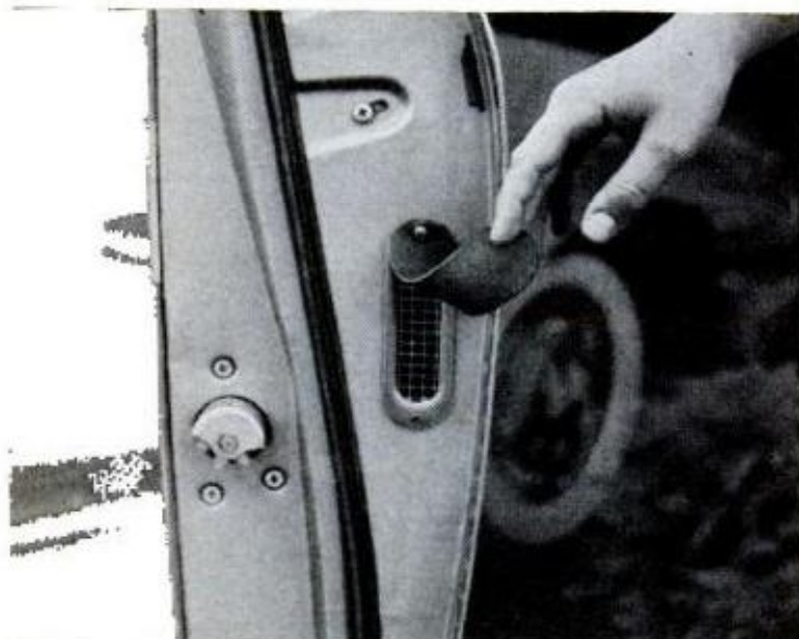
ONE-WAY VALVE cut from inner tubing can be added to exhaust if you live in an especially cold climate
