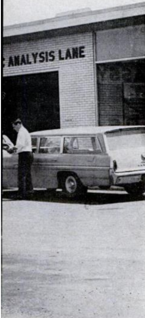
ON THE MOBIL ANALYSIS LANE , Bob Borst's Pontiac is tested with wheels turning at 60 mph. One technician operates control while a second reads meter
