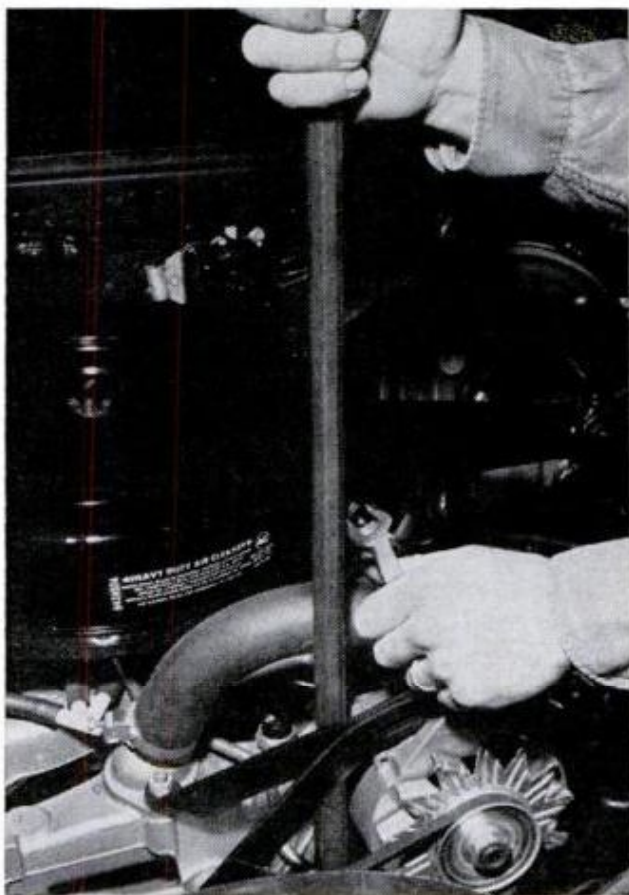
ALTERNATOR DRIVE BELT is tightened by bringing leverage to bear on center of alternator housing. Tighten bolts while holding alternator in position
