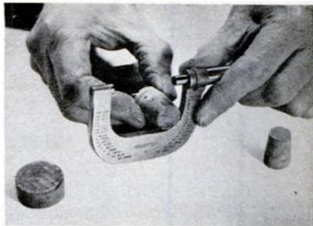
REMOVING TARNISH from a curved metal surface is a cinch if you use the curved section of a cork with approximately the same diameter. To brighten the flat surfaces, apply the widest face of the cork
