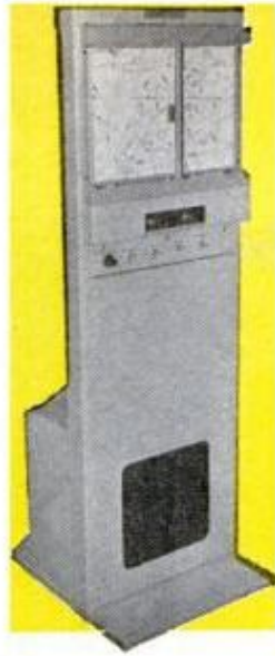
AT THE CONTROLS OF THE GAT-1 (right) is the author. Instrument panel is a direct copy of those in standard single-engine plane. Engine and prop sounds add to realism. Dials at left of cockpit door are used by instructor to adjust normal flight or instrument characteristics, or feed in abnormal ones to test student's reaction to emergencies. Stand-up recorder (left) traces flight path on realistic air map
