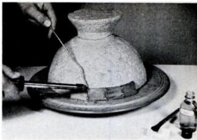
GLASS PIECES, framed in copper foil, are tacked to each other until one entire row is completed
