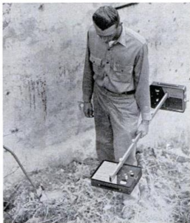
RADIO-TYPE DETECTOR has a loop at each end of a pole. Signal broadcast from one loop bounces off metal objects and is received by the second loop
