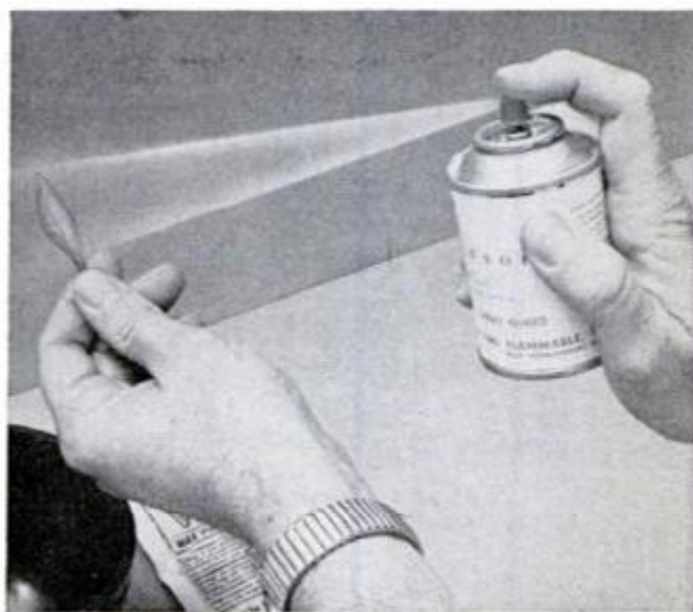
SPRAY THE PATTERN —in this case a small leaf—with a wetting agent before embedding it. This lets the mold mix flow smoothly over the entire surface
