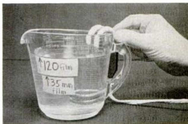
A KITCHEN MEASURING CUP of ovenproof glass is ideal for mixing photo-processing solutions since it can be subjected to heat and cold for critical control of temperature. Mark levels for various film sizes with taped-on labels.—Robert Hertzberg
