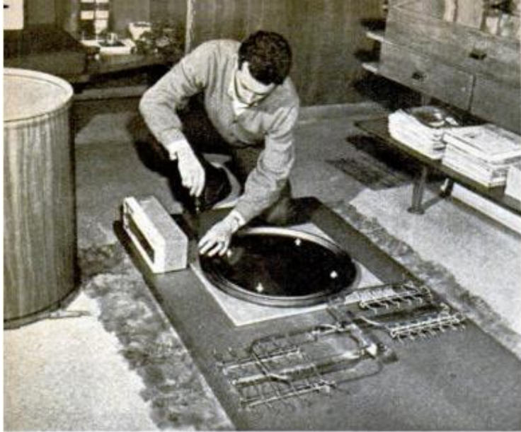
FIBER DRUMS form king-size "legs" for the hobby table. The metal lids are first bolted to plywood squares, then the squares are screwed to the underside of the top, as at left above. Plywood discs,
