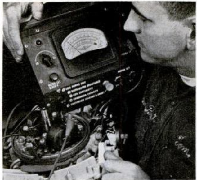
MAGNETO TESTER helps to determine whether a full spark occurs at just the right time. Ignition system and compression are critical factors for speed
