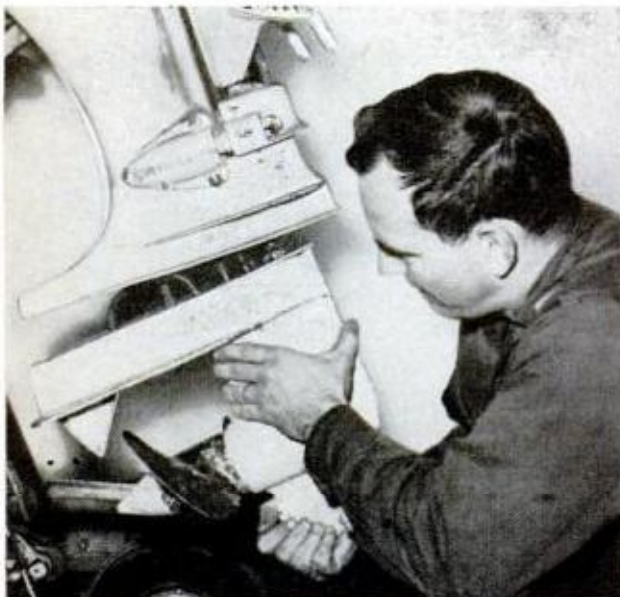
HIGH SPEEDS make efficient cooling even more important than normal, so drop the lower unit and check cooling system, especially pump and impeller
