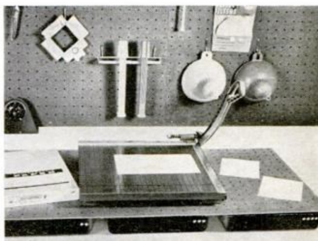
LAY A STRIP OF HARDBOARD over your developing trays and you'll have a temporary work counter without disturbing your chemicals. The trick comes in handy for jobs like cutting more paper halfway through a session of printing.—D. E. Anderson
