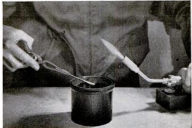
AFTER HEATING A WIRE to reharden it, quench it quickly in water before it has time to air-cool
