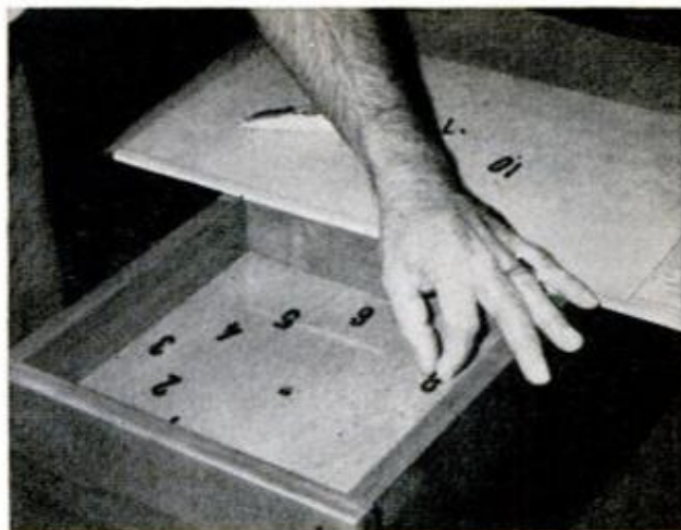
BLACK PLASTIC NUMERALS, 1\frac{1}{4} in. high, are cemented to clockface with spot of model plane cement
