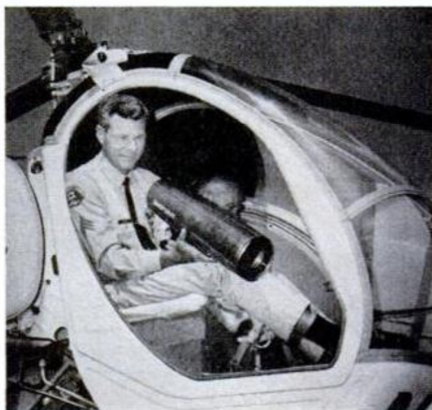
TROUBLE AT NIGHT is quickly detected with this high-intensity searchlight that can illuminate an area as big as a football field from up in the sky
