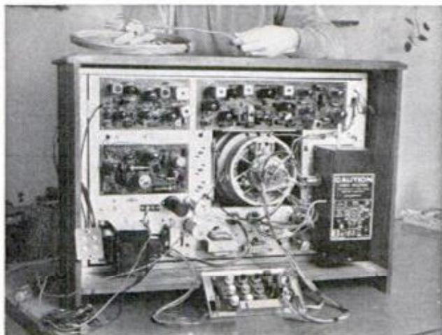
YOU DEGAUSS CHASSIS and color tube initially with coil supplied with the GR-180. Thereafter, automatic degausser does the job whenever the set's turned on
