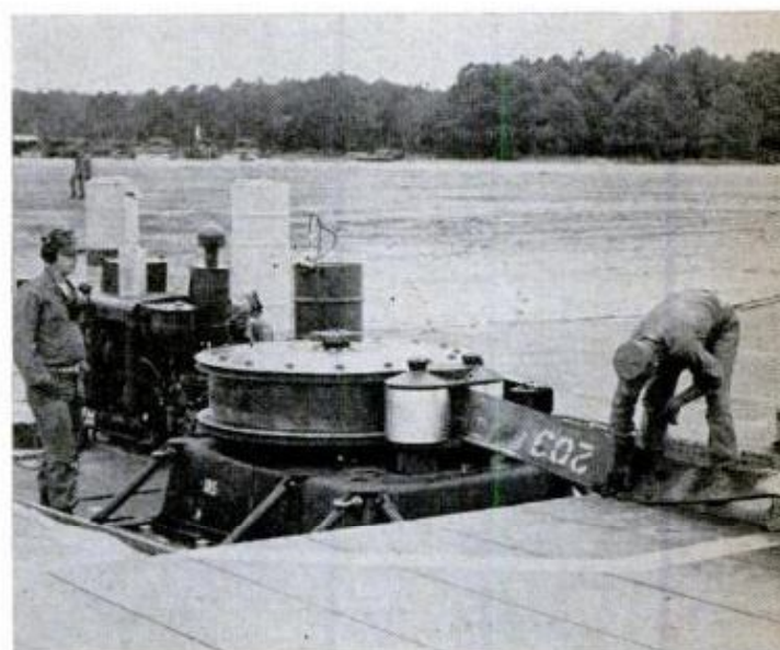
MARINE GROUND CREW wipe antiabrasive on arresting tape to prevent it from sticking. Tape is disconnected from arresting cable during takeoff sequences
