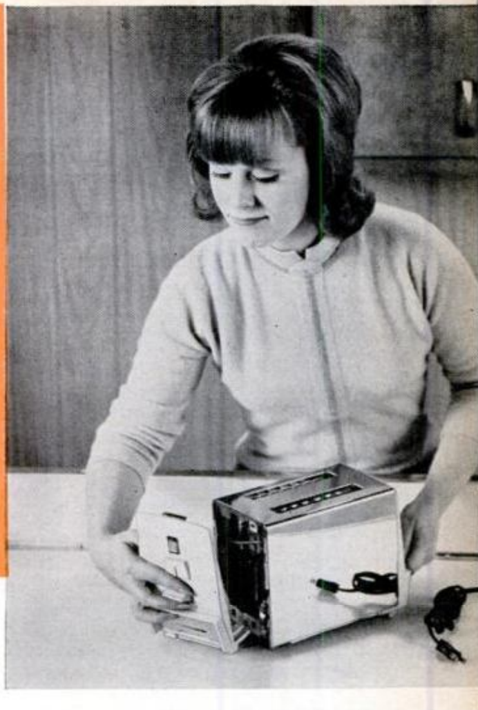
TOASTER CHASSIS , shown at center above, contains heating coils and controls. It slips out of its housing like the insides of a TV set. Entire unit can be replaced for $4.95, giving you a like-new toaster for less than half the original cost
