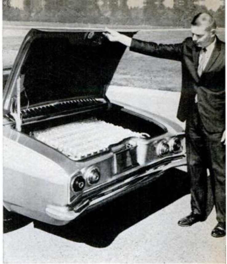
BANKS OF SILVER-ZINC BATTERIES fill front and rear compartments in the Electrovoir (top and right). Even rear seat (lower left) is stuffed with maze of switches and wiring, leaving no room for Grandma
