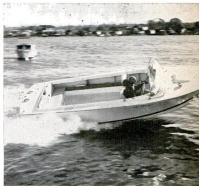
RC POWER for this 20-ft. Bertram is tucked away behind the full-width stern seat leaving cockpit completely clear. Its 185 hp pushes boat to 35 mph
