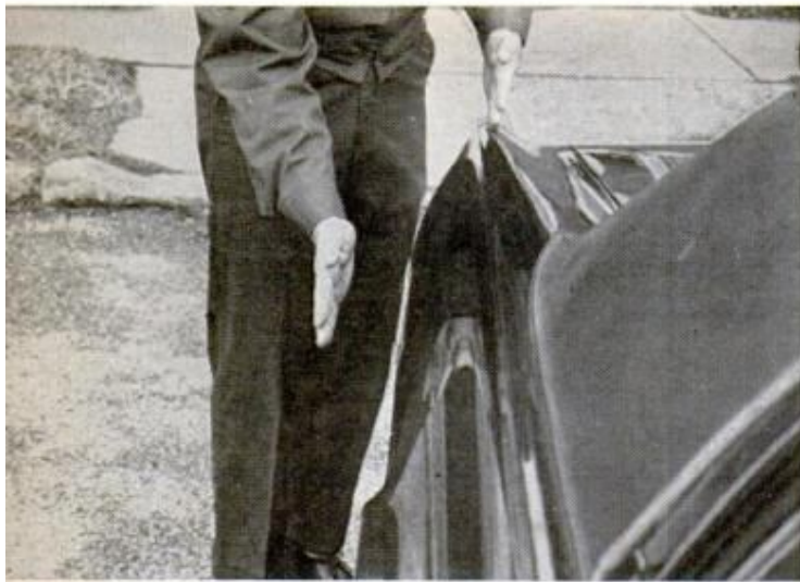
REAR FENDERS, WHEEL WELLS bulge out a good six inches beyond visual reference point when backing up, yet few owners mentioned poor rear visibility
