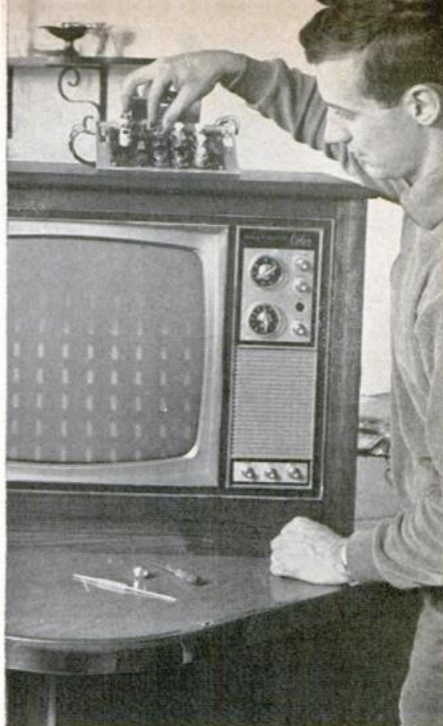
YOU USE BUILT-IN DOT GENERATOR and convergence board to align red, green and blue dots one over the other, giving a resultant white dot for perfect color
