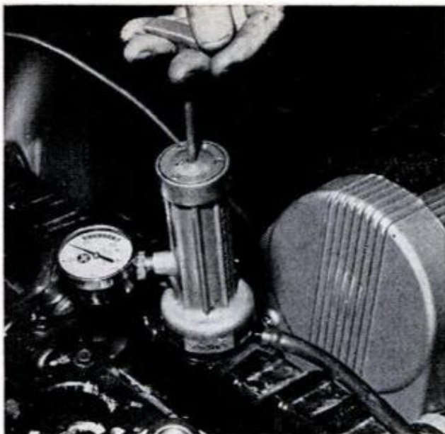
PRESSURE TESTER checks integrity of cooling system and radiator cap to contain the increased pressure necessary to increase boiling point of the coolant
