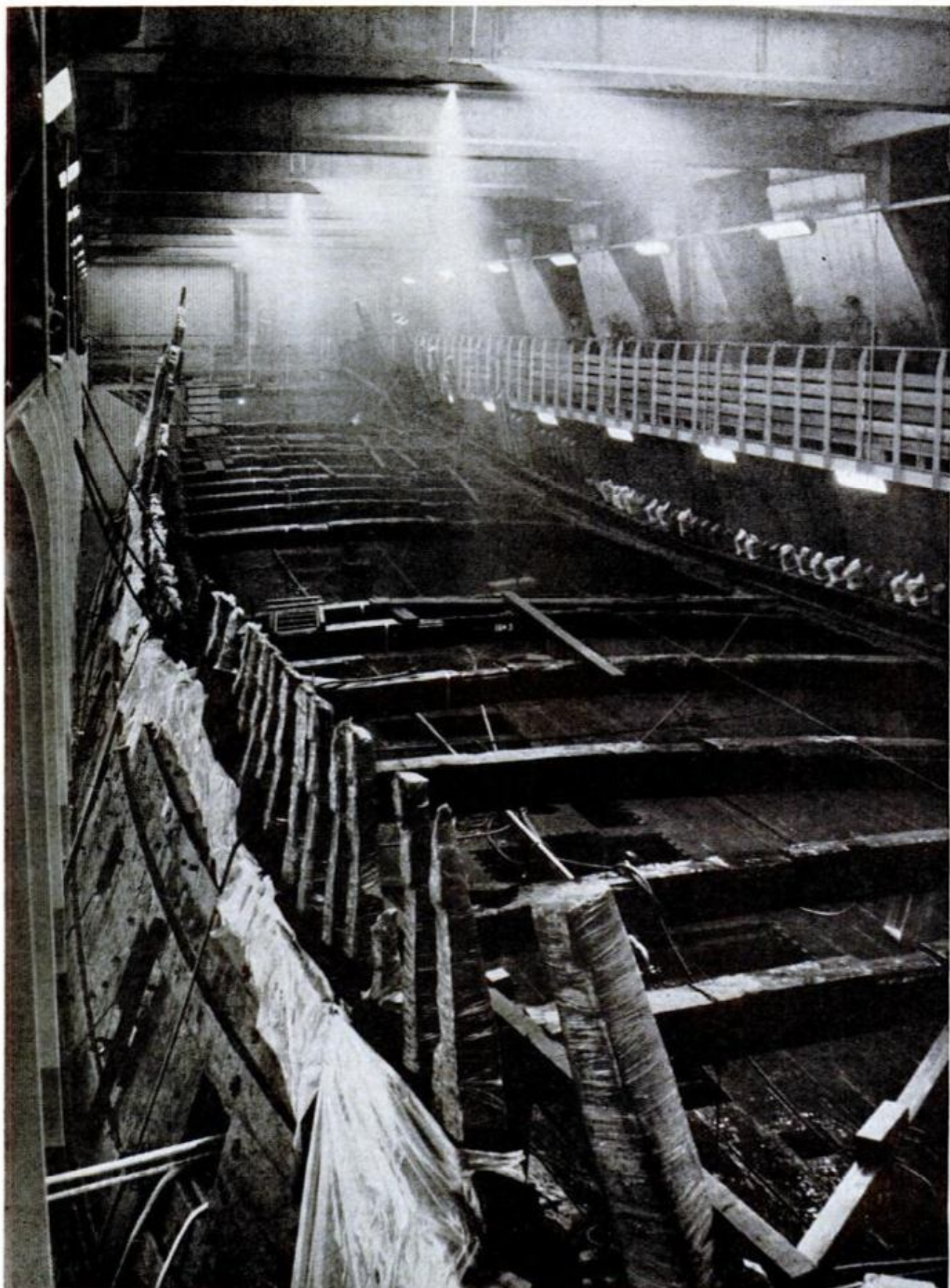
INSIDE THE HUGE SHED built around the recovered Wasa , spray jets keep the hull saturated day and night. A waxy chemical mixed with the water is gradually soaking into the wood to reinforce aging timbers
