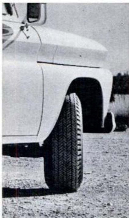
Duplex tires — Extra-wide tire replaces dual tire assemblies, cuts down cost and extra weight. Trucks carry more payload.
