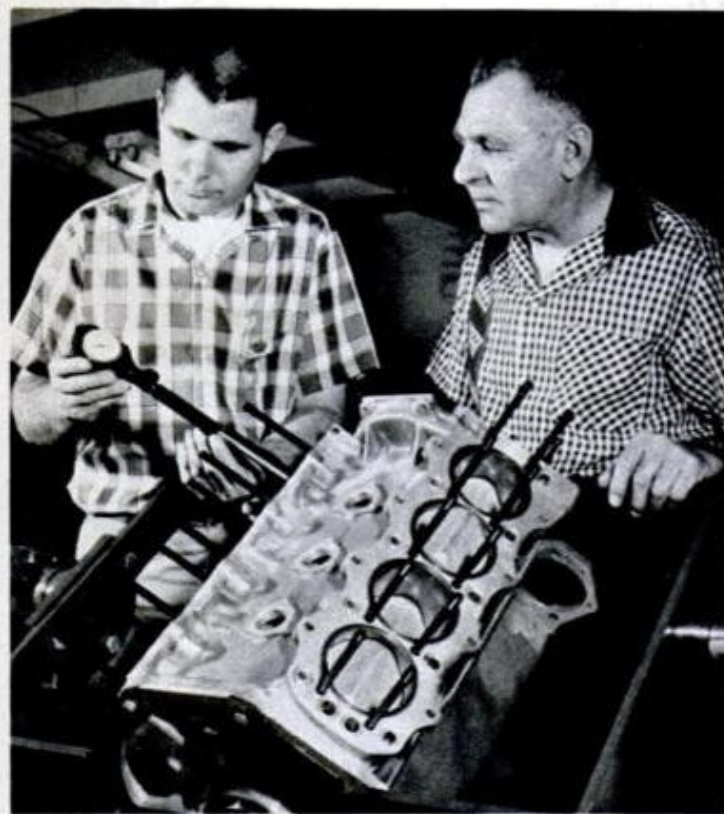
ENGINE PRECISION , reliability are keys to Indy victory. Three-time winner Lou Meyer, now a builder of Ford racing engines, and son check a DOHC block
