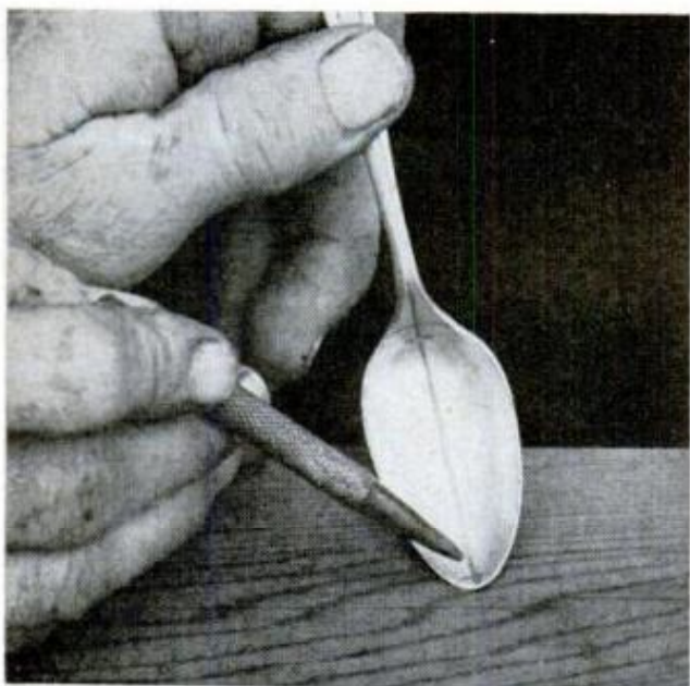
STEP 1. Mark center line and hole locations with a dark pencil or crayon on spoons. Dent hole location with a center punch so the drilling will be accurate
