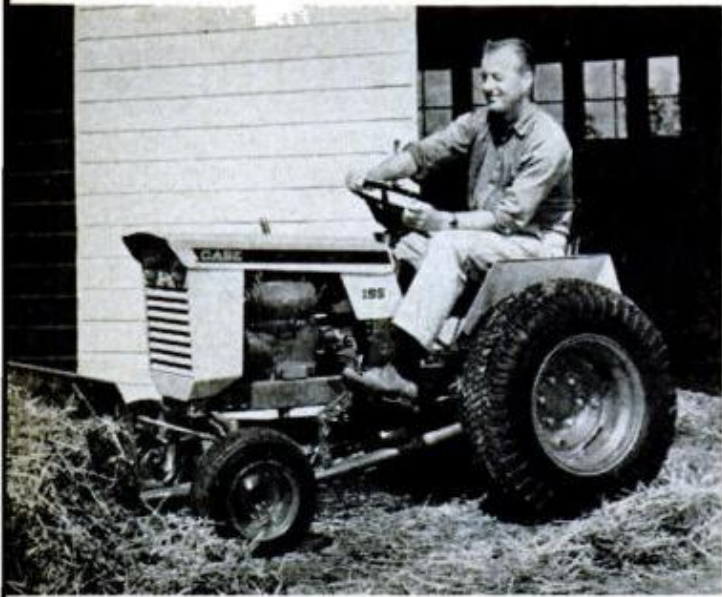
J. I. CASE'S top-of-the-line model is the 195, a 12-hp (Kohler) hydrostatic "complete" at $1175
