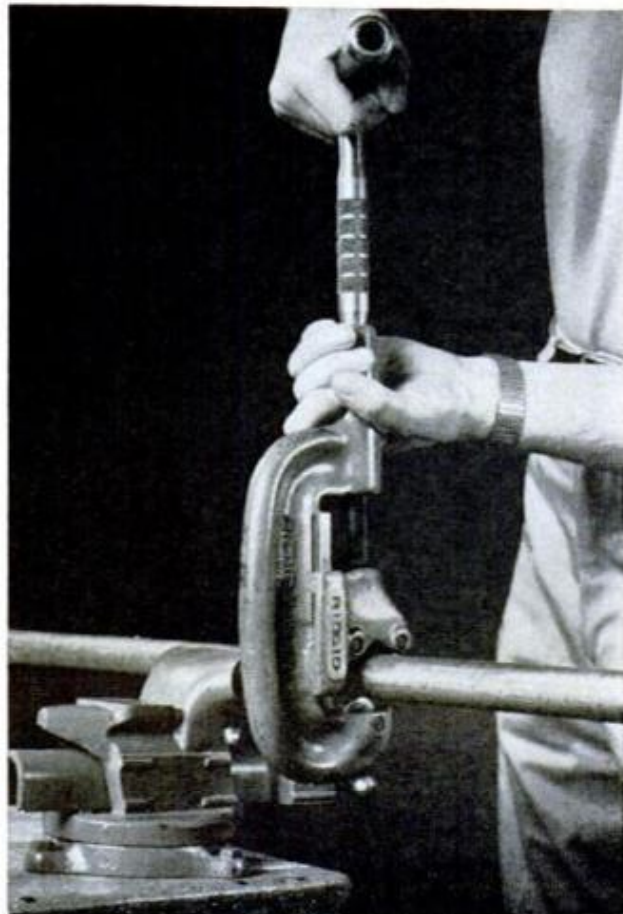
REGULAR PIPE CUTTER is the handiest way to chop pipe to length. As tool is rolled around the pipe, handle is screwed down forcing cutter against wall
