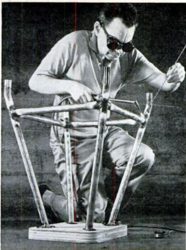
TORCH WELDING is slower than arc welding but leaves smoother fillets. However, either may be used provided proper care is taken in smoothing joint
