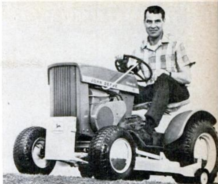
JOHN DEERE 10-hp has variable-speed drive that slows ground speed without rpm loss or shifting
