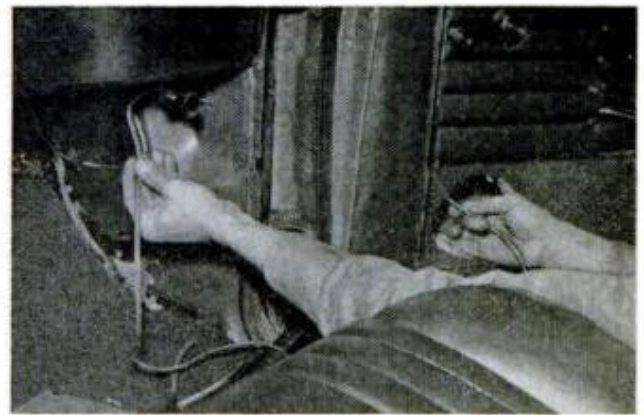
STEP 4 is snaking speaker lead through car body into the door near speaker. Be sure to use grommets
