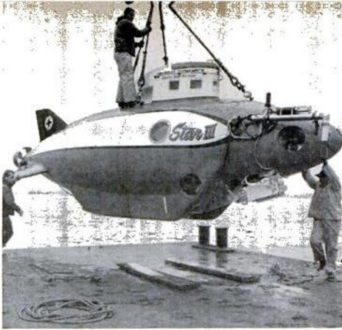
SWINGING FROM A CRANE , Star III is lifted from her support barge and swung overboard. Her pilot stands on the mini-sub during launch operations.
