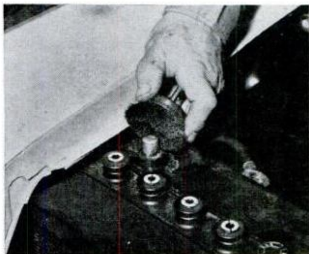
BATTERY POSTS are most easily cleaned using wire brushes specially designed for the purpose
