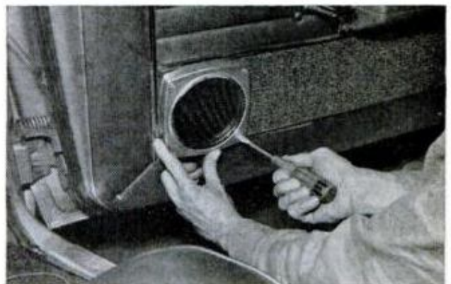
STEP 6 is securing speaker. Quick dealer installation shown in these photos, often beats doing it yourself
