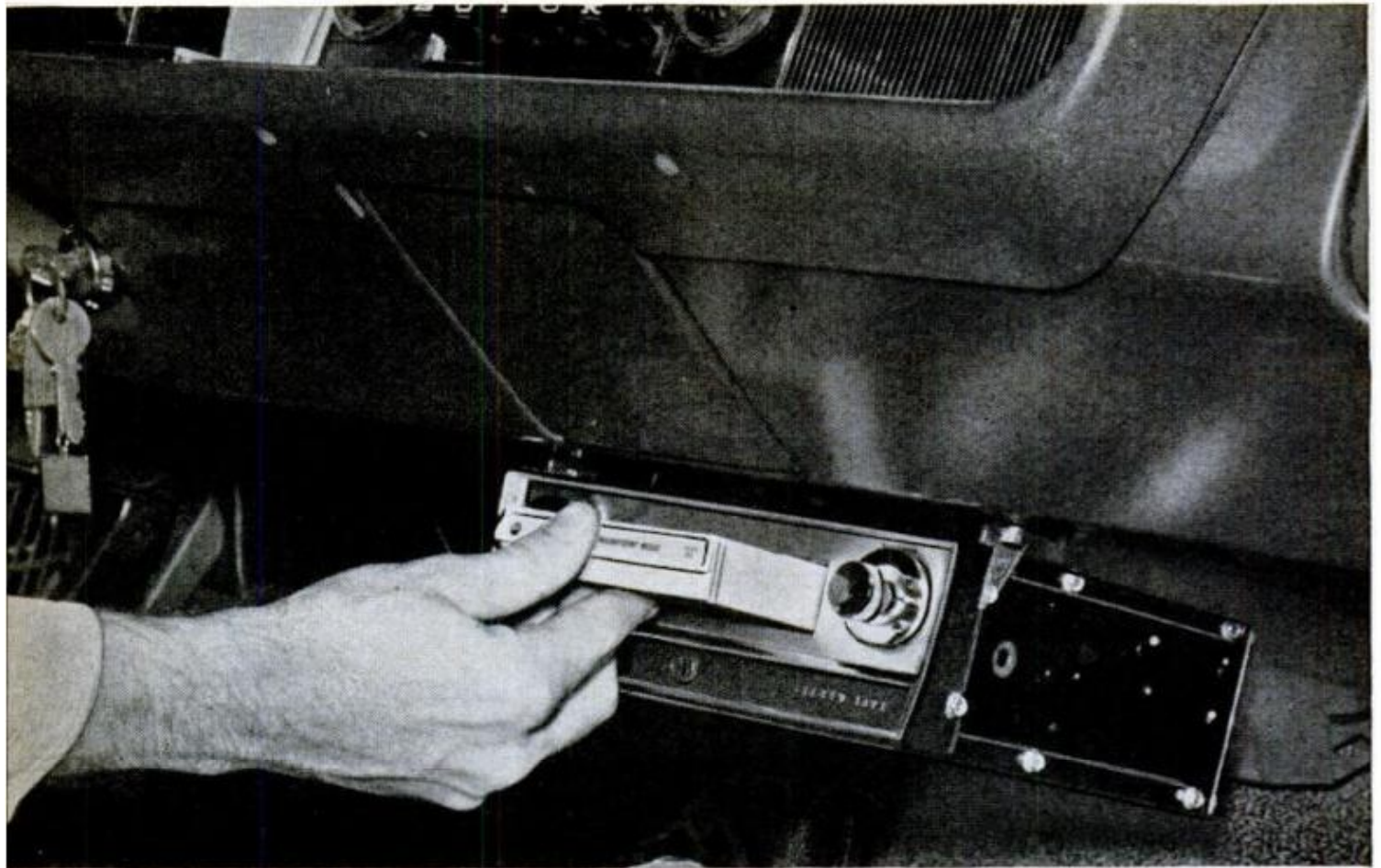
TYPICAL TAPE-PLAYER INSTALLATION shows Motorola 8-track unit under the dashboard of a Buick Skylark
