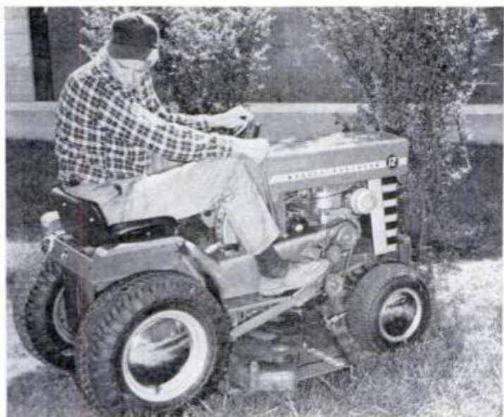
MASSEY-FERGUSON 12-hp hydrostatic offers wide range of speed variations without clutching
