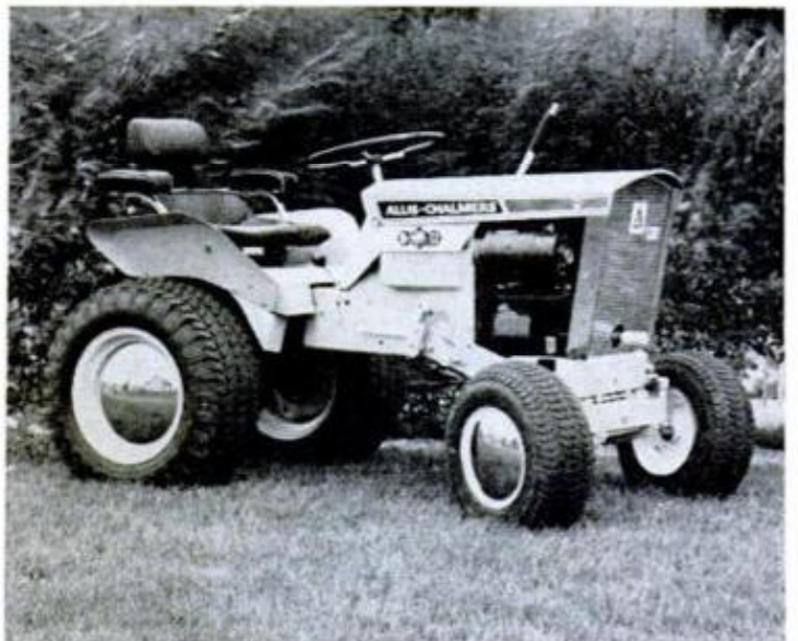
ALLIS-CHALMERS: 12-hp B&S "balanced" engine, gear drive, 3 PTO outlets, controlled differential. $885
