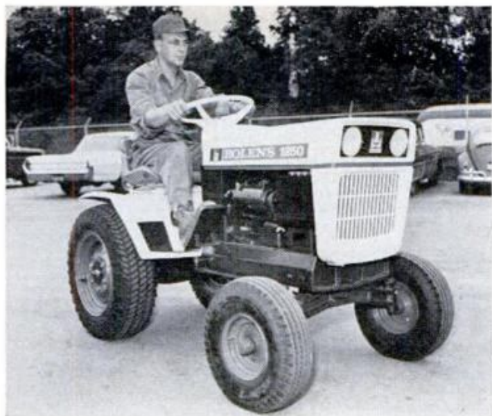
BOLENS Husky 12½-hp (Wisconsin) hydrostatic moves forward with toe pressure, reverses with heel
