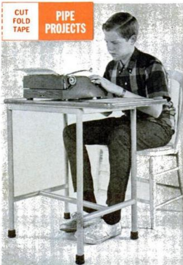
TYPEWRITER TABLE has an offset top which overhangs the frame at one end, providing extra space to hold books, papers or other materials to be copied
