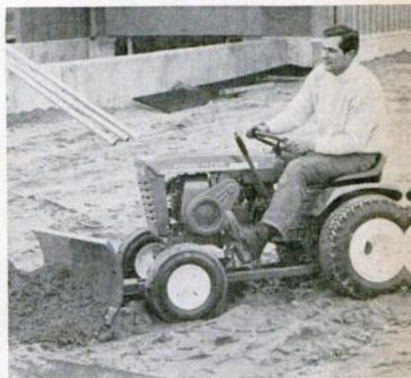
INTERNATIONAL-HARVESTER Model 123 shows few sheet-metal changes, but under the hood a 12-hp engine and I-H's exclusive "all-piston" hydrostatic transmission revamps performance
