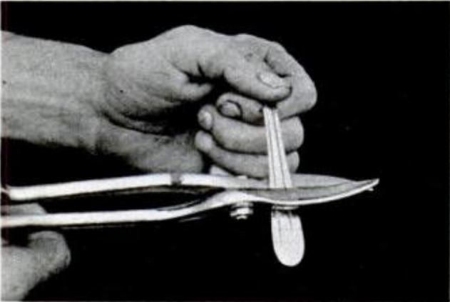
STEP 5. Cut handle to any length. Using 10-inch snips, round off the ends. Then file edges smooth. Mark and dent spots for holes. Use \frac{1}{4} -inch drill bit
