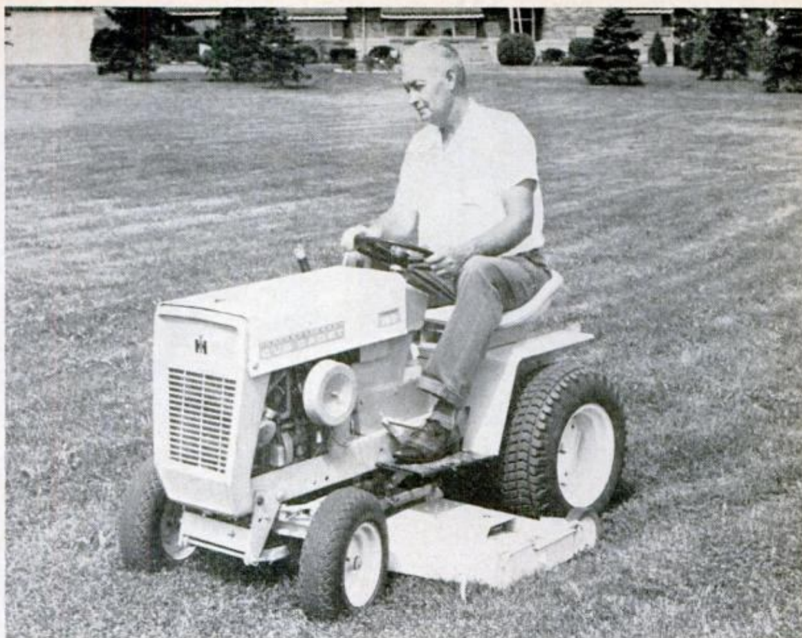
INTERNATIONAL-HARVESTER Model 123 shows few sheet-metal changes, but under the hood a 12-hp engine and I-H's exclusive "all-piston" hydrostatic transmission revamps performance
