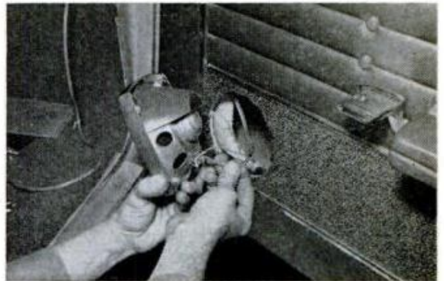
STEP 5 is connecting lead to speaker terminals. Rain shield over cone deflects water from window slot
