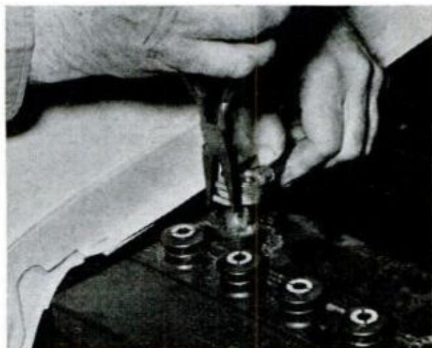
BATTERY CABLES can be tricky. Tighten securely, but take care not to overtighten or twist the post
