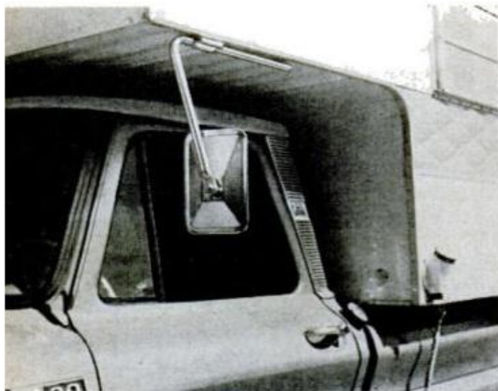
NEW REAR-VIEW MIRROR stays with your camper, not your truck. It gives a full rear view instead of a partial view from the truck-mounted mirror
