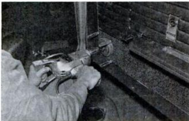
STEP 3 is cutting speaker hole with toothless cutting mandrel for clean hole without snagging carpet
