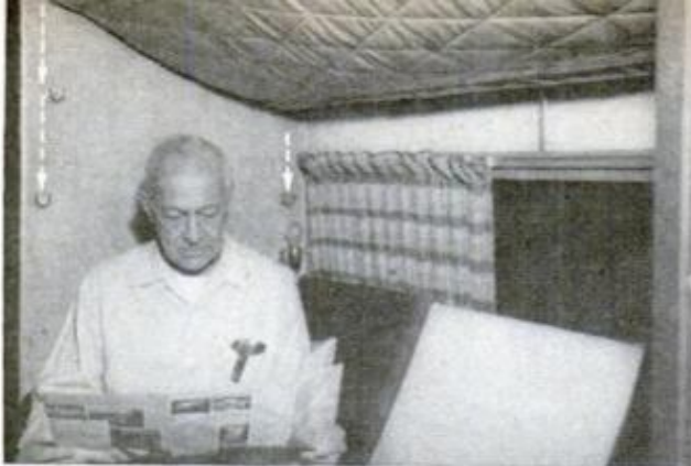
AN ADDITIONAL BED is always handy. During the day, the bed is lifted to the position shown above. At night, it's lowered to brackets shown by the arrows
