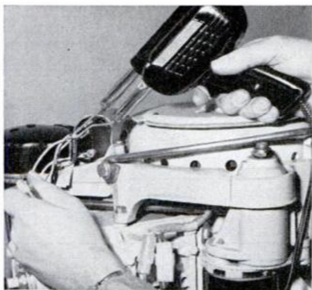
INSTALLATION instruction may not call for soldering connections, but it's a good idea to do this
