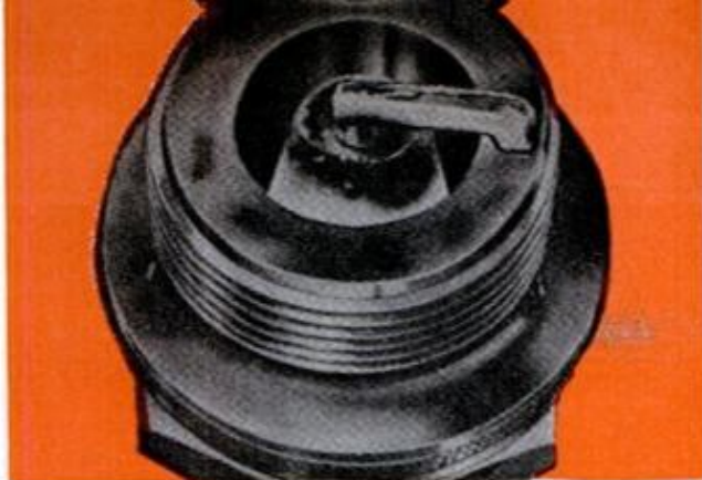
ADVANCED TIMING causes plug overheating, which breaks down porcelain insulation and greatly shortens plug life. This is only one effect of mistiming
