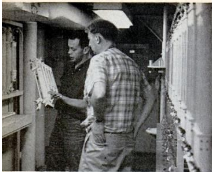
NANSEN BOTTLES are stored in "wet" lab. They are an old but still very good way to get water samples and temperature readings at assigned depths
