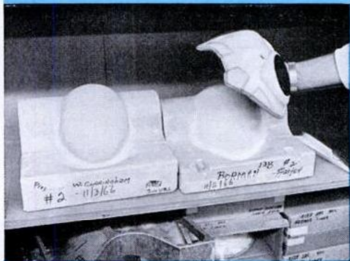
HEAD SIZES (those of Astronauts Cunningham and Borman are shown here) are taken to create each helmet to fit individual astronaut's skull contours
