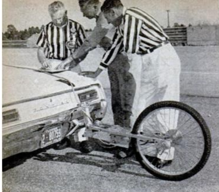
FIFTH-WHEEL-EQUIPPED OFFICIAL CAR carefully checks all distances covered by test cars. Wheels, calibrated each day, are accurate to one-tenth foot
