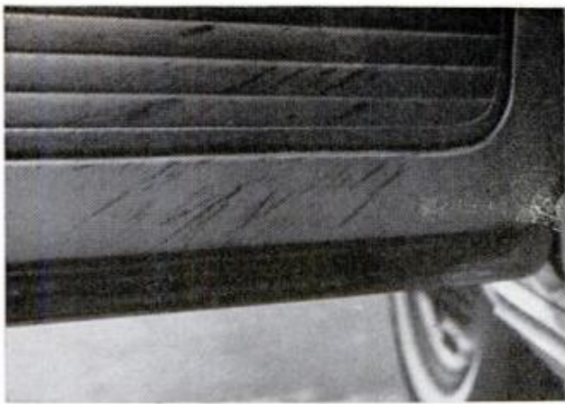
INSIDE DOOR PANELS take a rough beating at their lower edges (above). Scuff marks can be removed and the material retinted for a like-new look (below)
