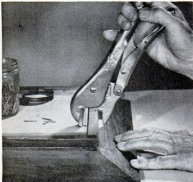
STANDARD WRENCH —here, a straight-jaw 10-incher—does better job than hammer of driving brads in critical spots. Since jaw limit is regulated by screw at end of handle, all nails will project same amount. Note how padded jaw protects the frame's finish
