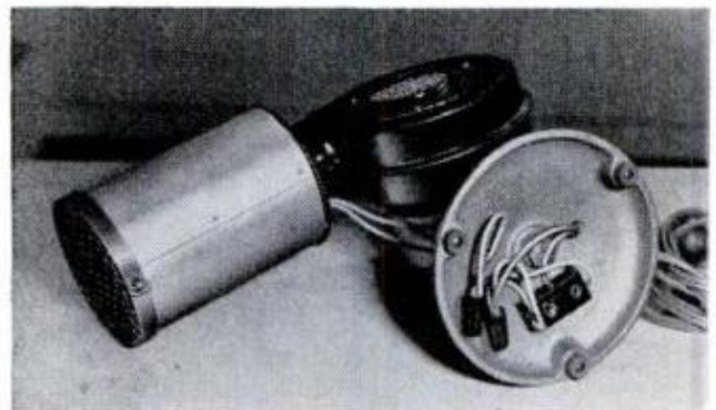
ALL WIRING CONNECTIONS are made near body of a center-off toggle switch and concealed on underside of the microphone stand that forms the base
