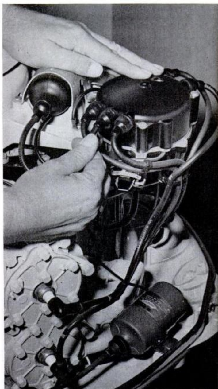
SPECIAL COIL fits under the shroud easily. A high-tension lead included in kit is used to connect it
