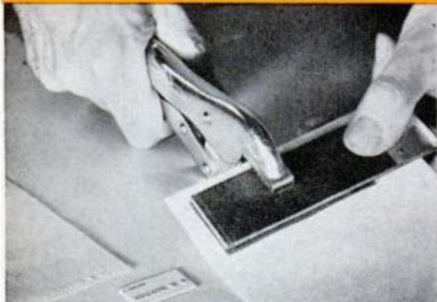
EMBOSSED PRESS —for personalized stationery—is easily made. Die is nameplate snipped from plastic credit card. Adjust jaws for enough pressure to emboss the raised letters, but not the die outline, then squeeze the nameplate in two places for uniformity
