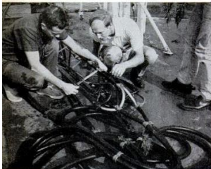
MEMBERS OF SCIENTIFIC PARTY check the sparker and clear it of seaweed after pulling it in by hand. The insulated cable transmits electric pulses
