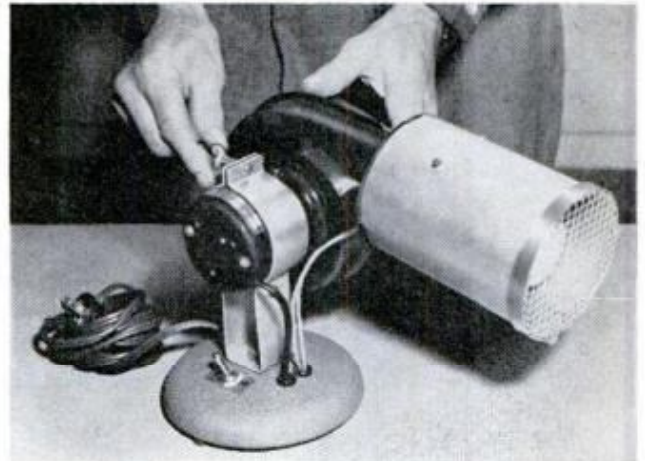
DIRECT THE AIR SUPPLY up, down or where you want it by loosening a wingnut on the motor clamp, turning blower unit to position and retightening nut
