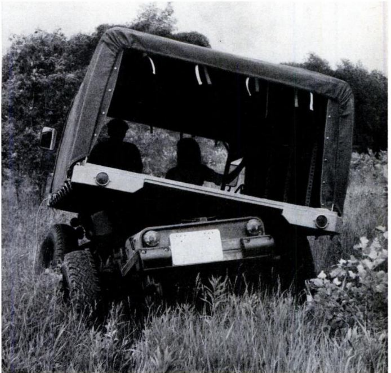
WITH BACK CURTAIN ROLLED UP , there's no blind spot to rear. Note, too, how chassis twists with terrain
