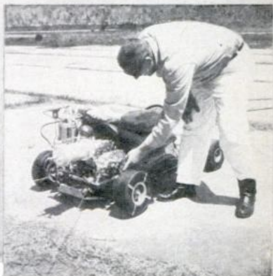
WHEEL-DRIVEN VERSION of kart is tied down and weighted for static test. Turbonique engine puts 45 hp to wheels
