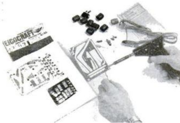
CIRCUIT BOARD mounts components of relaxation oscillator that comprises Eicocraft "Mystifier Kit"
