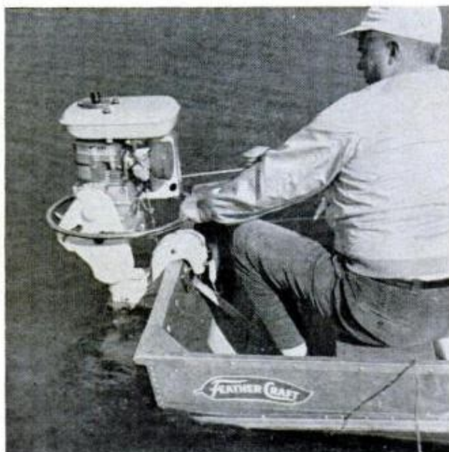
STARTER ON SIDE makes locking catch necessary to prevent motor from spinning when cord is pulled
