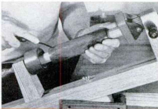
CRADLING STOCK of old side-by-side double shotgun requires this mounting, while matching forearm needs special holder shown below
