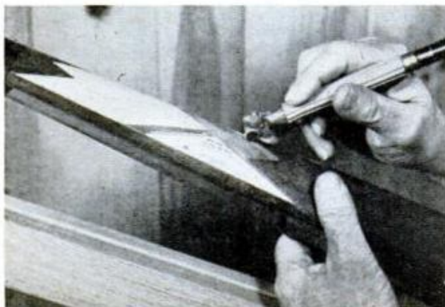
DECAL PATTERN is cut away with wheel (above) controlled by foot switch. Cheekpiece (partly scored, below) has full skip-line-pattern decal
