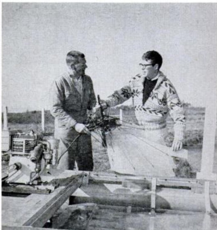
THINKING BEHIND invention shown in these three photos is that better way to propel boats is by side-to-side fishtail action than by the usual rotary prop
