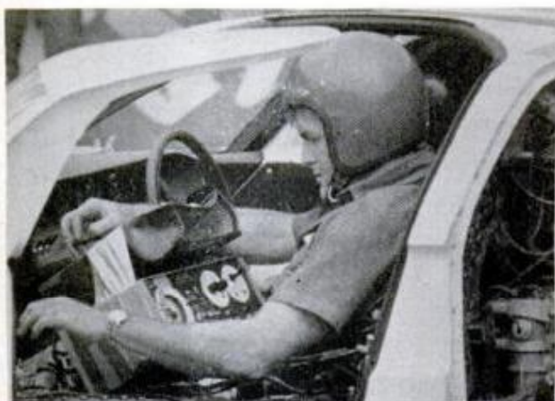
BRISTLING FORD GT CAMERA CAR boasted five radio-controlled camera mounts, TV remote monitor plus three-way radio. Below, Johnny Stephens loads forward side mount; above left, he mans cockpit. Above right, his rig chases Garner and Bedford as they dice for lead. Forward camera will pan broadside as he moves up
