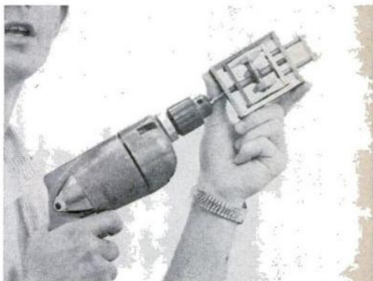
DEVICE ATTACHED TO DRILL converts rotary to linear motion by means of rotating weights. Linear motion can be stopped without stalling rotary motion
