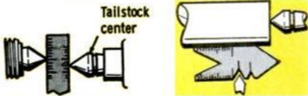
Setting threading tool with center gauge
