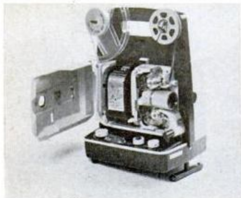
HONEYWELL'S ELMO , the only sprocket machine in the group, hides its format selector under the lamphouse cover. It's available with or without slow motion
