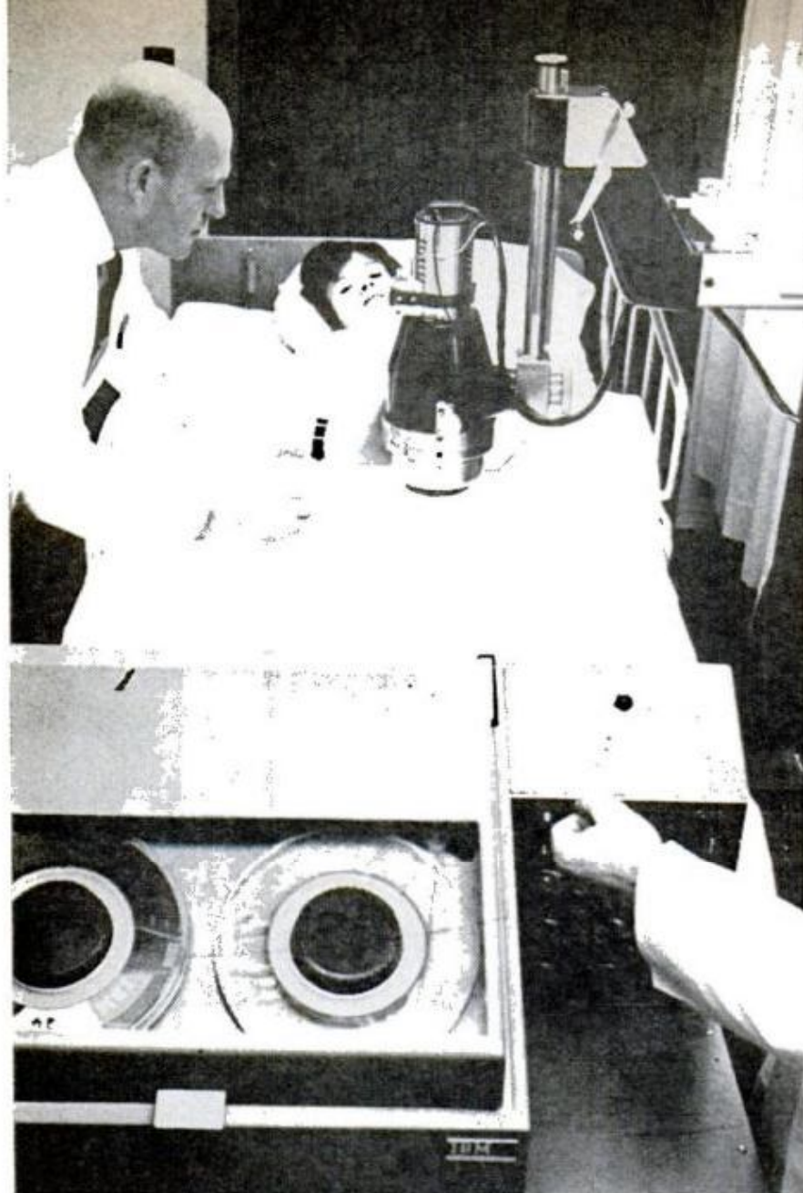
RADIATION SCANNER , placed over patient by doctor, records all radioisotope data on magnetic tape for computer processing in Mayo-IBM system
