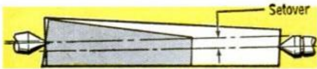
At same amount of setover, taper varies with length of workpiece
