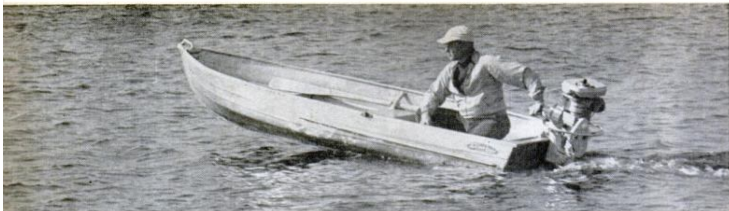
TRIM MAY NOT BE IDEAL here, but it was the best I could achieve without a tiller extension. The Honda isn't really designed for use on a light planing hull. It belongs on heavier, displacement-type work boats
