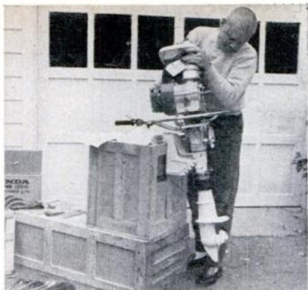
ENGINE BOLTS on lower unit, can easily be removed and used separately as power source for machinery
