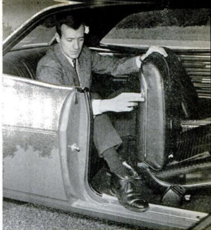
FRONT SEAT BACKREST RELEASE is safety feature that owners find easy to use when it becomes habit
