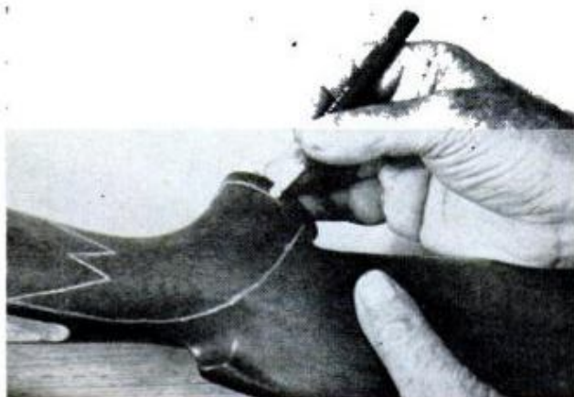
FREEHAND OUTLINE of grip pattern is easy to pencil. To hold front of pump-gun stock, use fitting below; screw other end to metal butt pad
