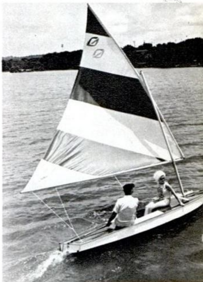
GLASTRON ALPHA is billed as a "super-sailboard." The lateen rig has 98 sq. ft. of sail, and in case you get too enthusiastic, the cockpit is self-draining after a knockdown. Rudder and centerboard are mahogany. You have a choice of blue or red deck
