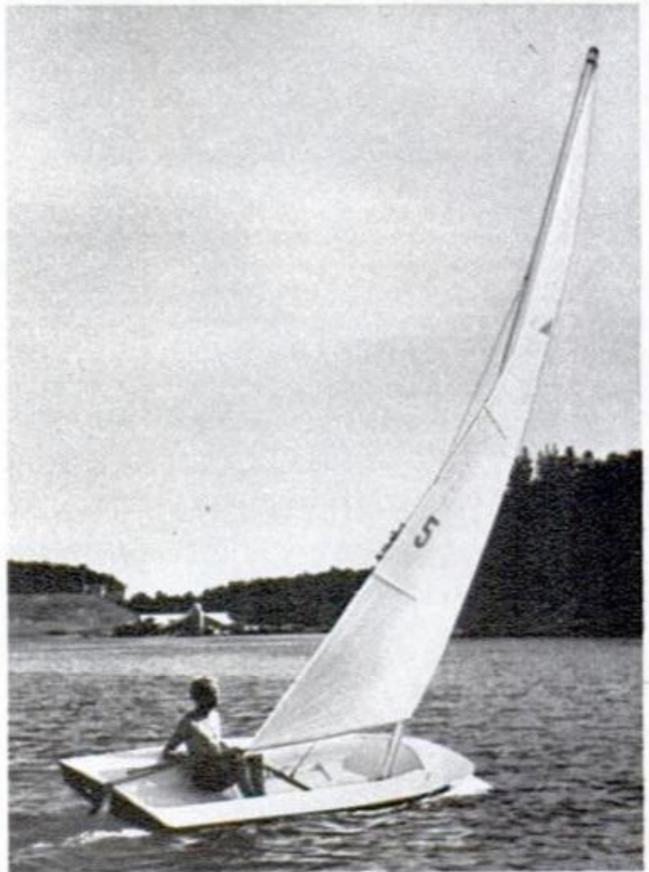
LARSON-REGATTA 132 is 13 ft. long, has a beam of 55-in. and carries 85 sq. ft. of Dacron sail. Completely cartoppable, it still offers a cockpit that is large enough for more than just your feet. The mast, boom, rudder and centerboard are aluminum
