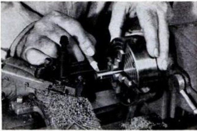
CHALK OR PENCIL MARK method for centering in four-jaw chuck. Here line is not continuous, shows work is off center. Not acceptable for close work
