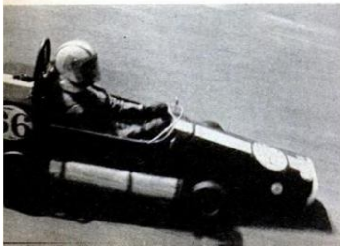
UNUSUAL ENTRY is this wedge-shaped kart with saddle gas tanks installed on each side. Tanks and front panel are made of aluminum. Two Chrysler engines power this machine. The big tires are 8x16s
