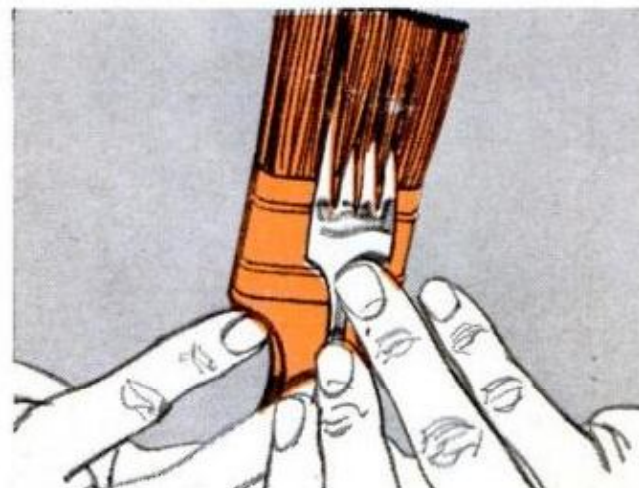
OLD KITCHEN FORK helps clean paint from a brush. Comb bristles with the fork while you rinse brush in water or paint solvent (depending on the paint)
