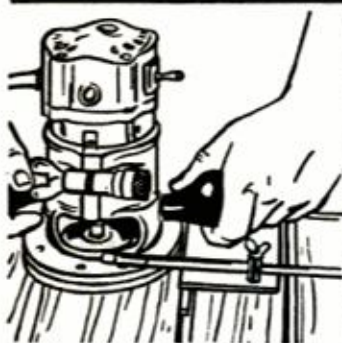
Use guide bar with pivot pin removed, or simple T-square made of scrap, to cut decorative grooves and slots.
