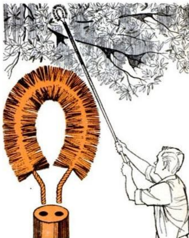
SWEEP CATERPILLAR NESTS off trees with fiber kitchen brush on a pole. Discard brush handle, drill holes in one end of long pole, insert brush prongs in holes
