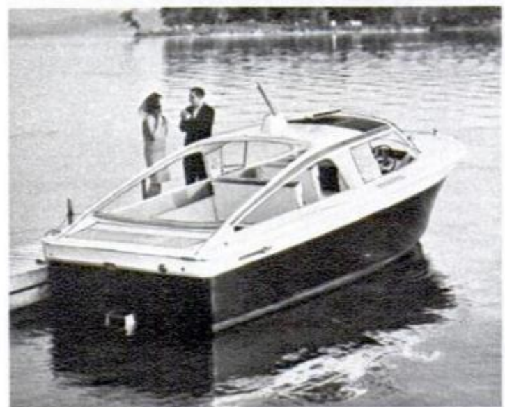
BUEHLER BAR HARBOR , 24 ft. of V-bottom jet "day cruiser," features streamlined styling by Virgil Exner. This jet-set dreamboat is propelled by a three-stage Turbopower unit with engine options of 290 to 325 hp, carries 60 gal. of fuel and has foam flotation
