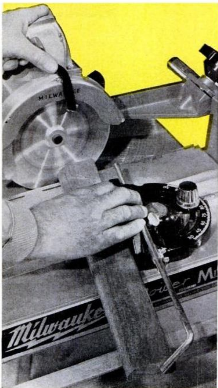
ODD ANGLES , other than 45 and 90°, are cut with work held against an adjustable protractor unit
