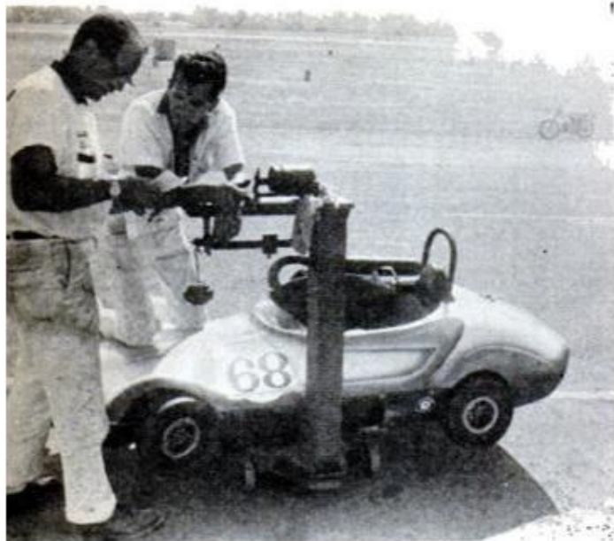
WEIGH-IN FOR KART AND DRIVER after winning a fast, tough race at Riverside, Calif. This Bultaco-powered kart goes onto scales to make sure that total weight conforms with the track's regulations
