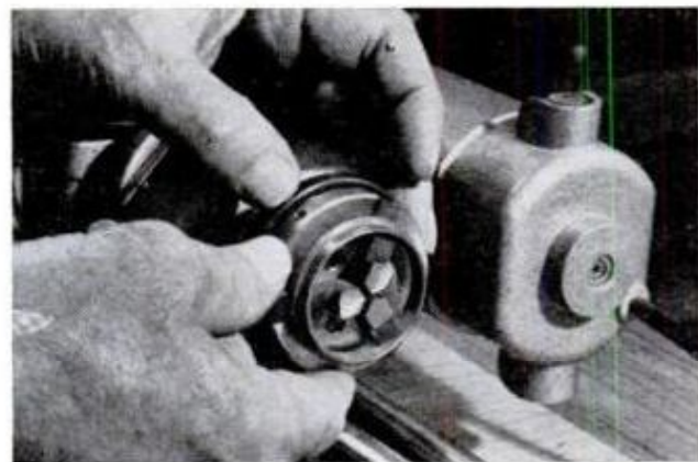
GRIP INSIDE OF WORKPIECE with jaws of universal chuck by backing them out, rather than running in. This permits both facing and edging of the workpiece
