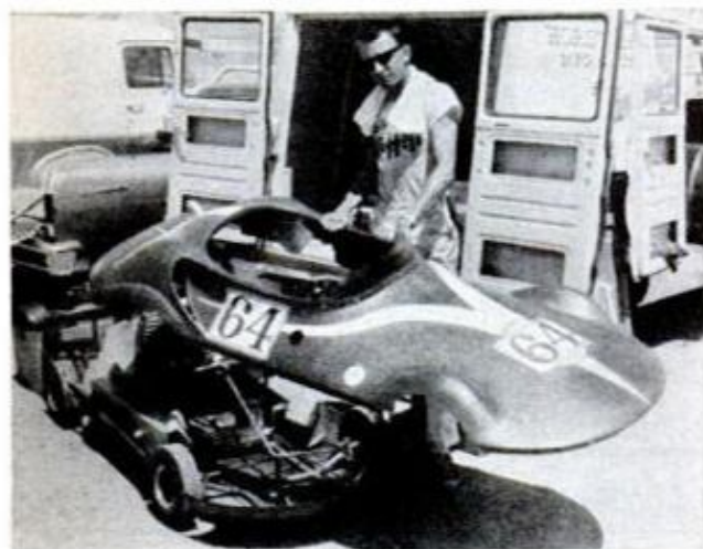
VITAL PARTS ARE EASY TO GET AT; simply lift the one-piece body with fingertips. Lightweight fiberglass makes streamlining a snap. A McCulloch 75 engine powers this baby. Bodies are custom-made
