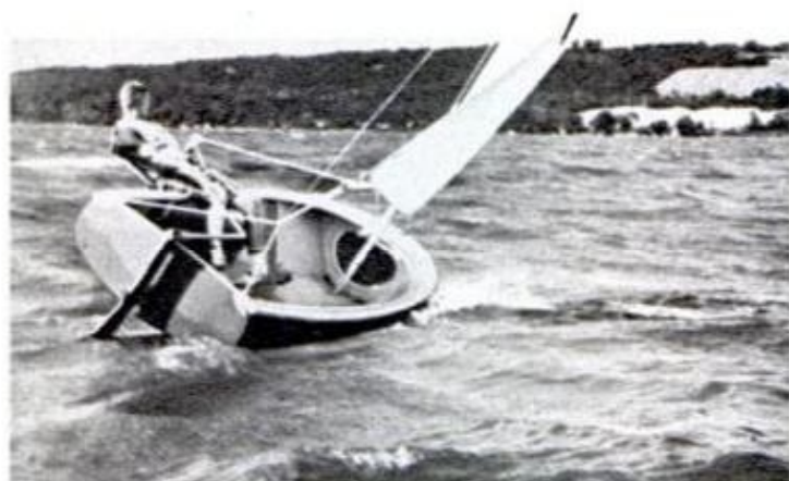
GRUMANN BALLERINA is one of several all-aluminum sail models in the company's 1967 line. The 12-ft. hull features foam-in-place flotation between the cockpit sole (floor, to all you non-salts) and the hull. All in all, a lot of sport crammed into 12 ft.
