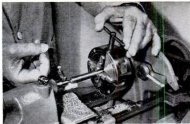
TAILSTOCK CENTER used as indicator for centering in four-jaw chuck. Workpiece is center-punched or center-drilled. Method not acceptable for close work
