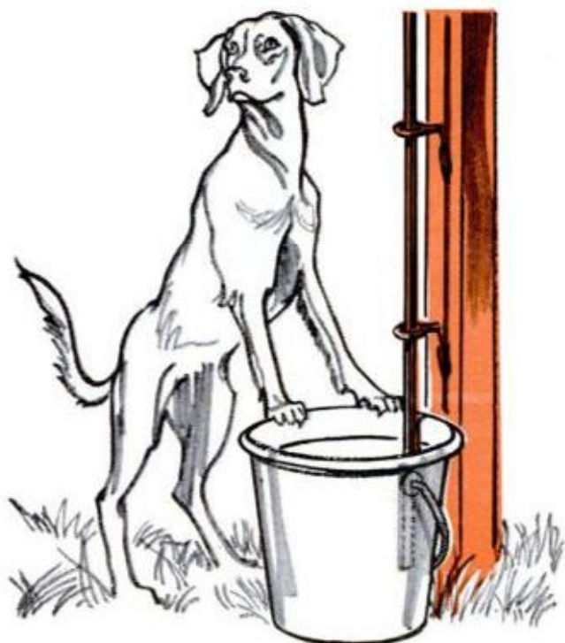
IF YOUR DOG delights in upsetting his water bucket, you can put an end to constant refilling by locating it under a sliding pipe that hooks inside pail
