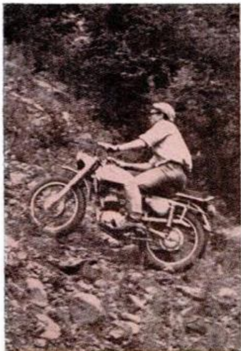
RUNNING A DIAGONAL COURSE up a steep rock-strewn slope off the side of a road, the Benelli Cobra 125 gets off to a fast start, but when geared down, lunges into the rocks and throws rider
