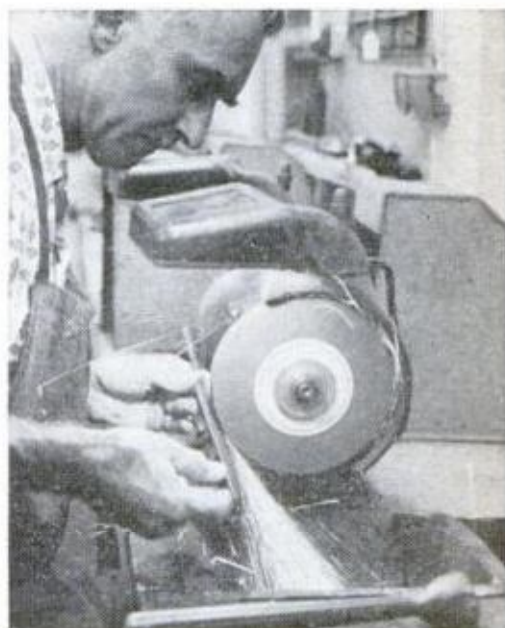
FORGED BLADE is now ground to size and contour wanted. It is then hardened by reheating it and immersing it in oil
