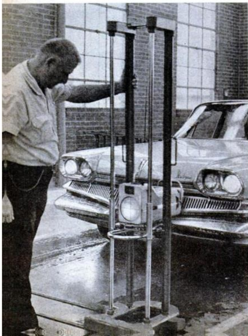
IN NO UNCERTAIN TERMS , stickers above call out condition of cars checked. Gauging headlights, below, quickly reveals any misalignment
