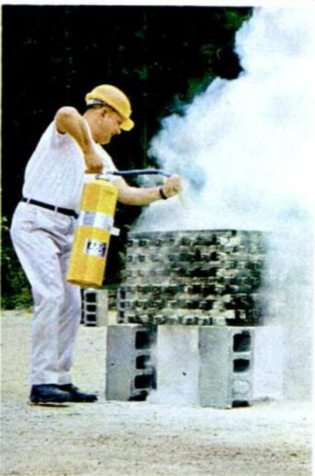
ROARING FIRE IN TEST CRIB had seven-minute pre-burn before a technician hit it with a dry-chemical all-purpose extinguisher. Blaze was killed in 65 seconds in the test timed by Popular Mechanics editor
