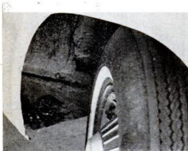
WHEEL TURNED in Corvair front-wheel well reveals how front panel forms ledge to collect dirt and salt. Lip around fender edge is another spot to watch
