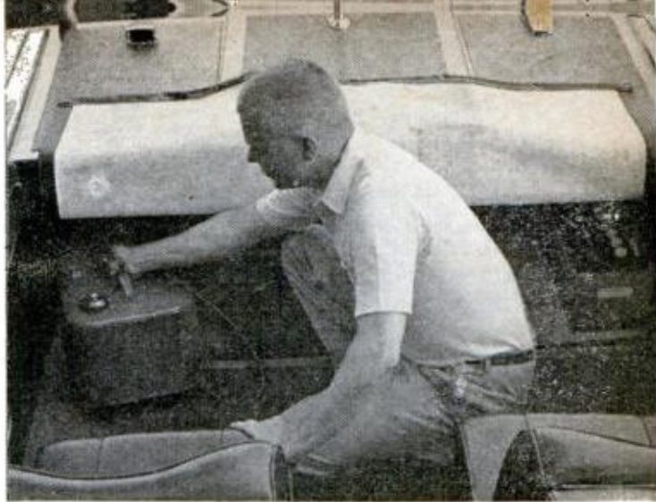
ROOMY ENGINE COMPARTMENT has plenty of space for battery box and extra tank of fuel to supplement 12-gallon bow tank. Vinyl curtain snaps to floor bar.
