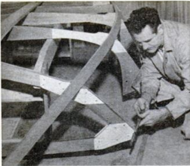
BEVEL NOTCHES for both sheer clamp and chine log so they will fit flat when bent over the framing
