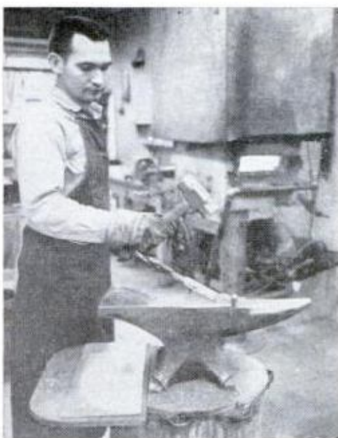
CHERRY RED , rough blade is hammered to general shape. Original blank of carbon-tool steel stock is used for knives
