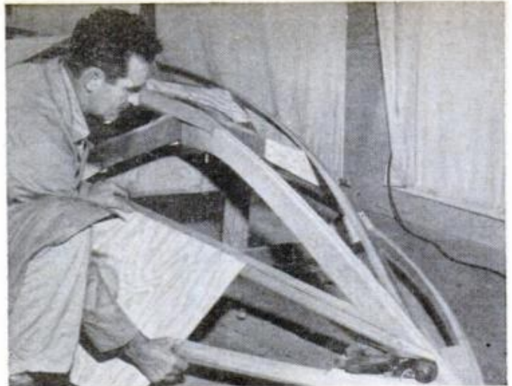
FAIR CHINE along line from Frame No. 5 to center of chine at stem so bow portion of planking will fit
