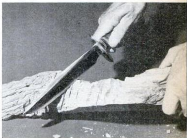
RANDALL TESTS knives on hard Florida heart pine before shipping them to customers. His knives are noted for holding cutting edge through long service
