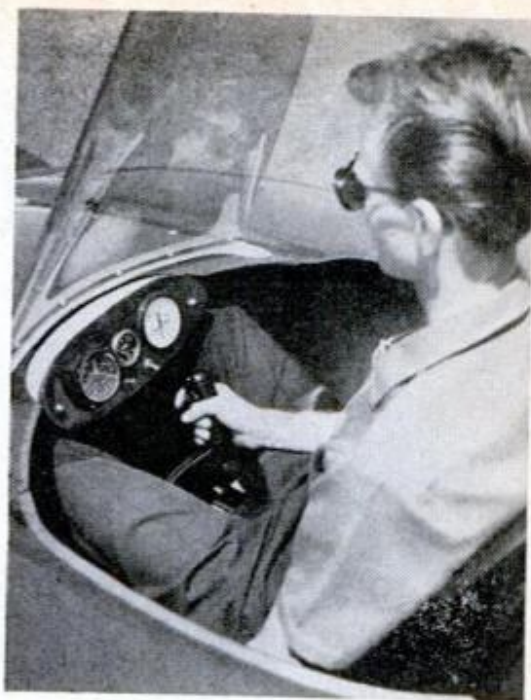
ONE-MAN COCKPIT has standard basic instruments and controls, including a cyclic-control stick and collective pitch throttle
