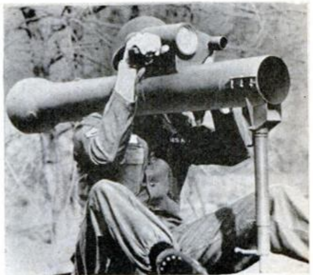
Shoulder-fired tank killer that launches a guided missile and can be carried by a soldier is being developed for the Army by McDonnell Aircraft Corp. The missile has rocket motors around its body. As commands are sent electronically, these thrusters correct the missile's flight and guide it to the target.
