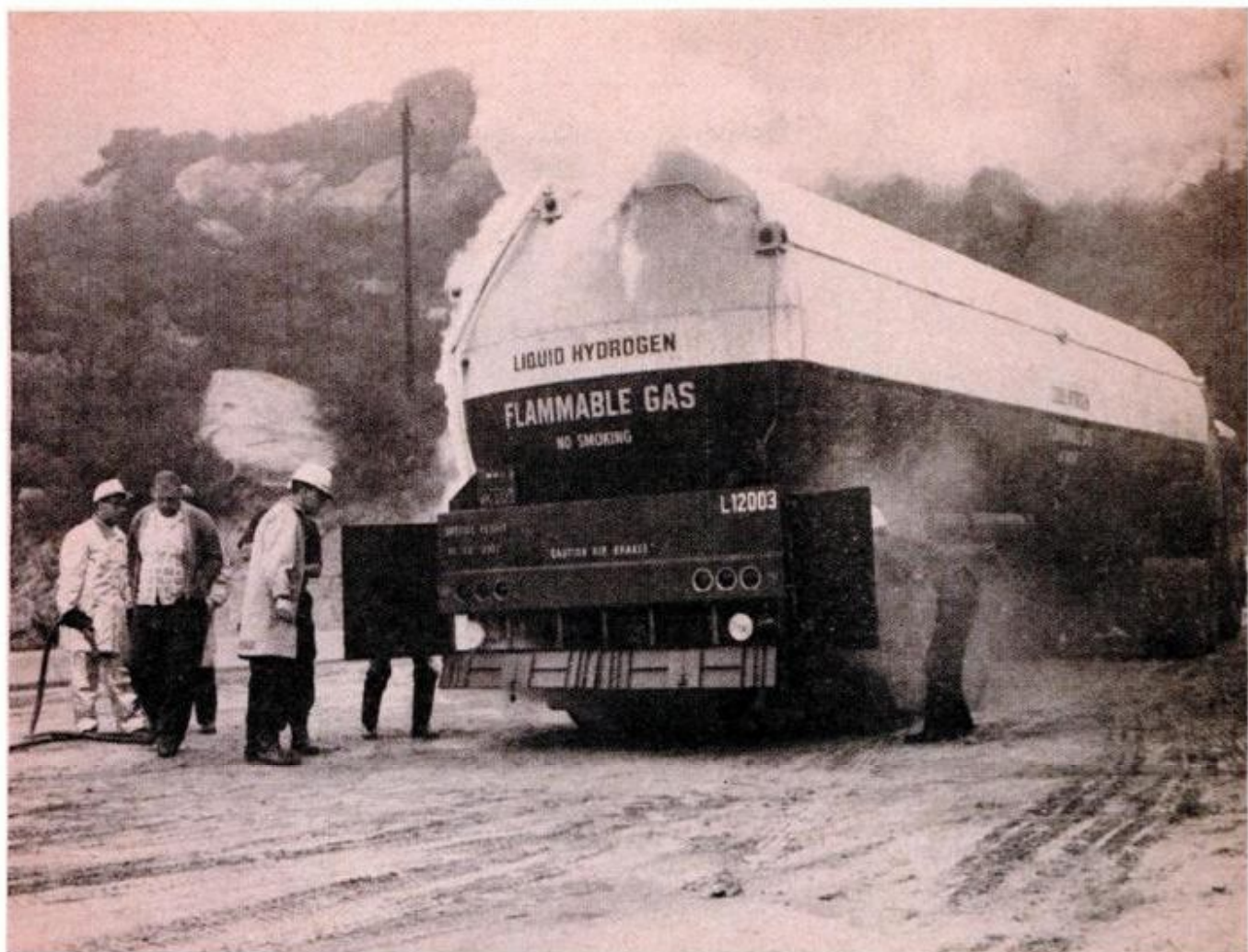
WRECKED TRUCK WITH FLAMMABLE GASES is a threat to firemen (left) who must use special methods to bring it under control. Leaking hydrogen (above) is allowed to dissipate into the atmosphere
