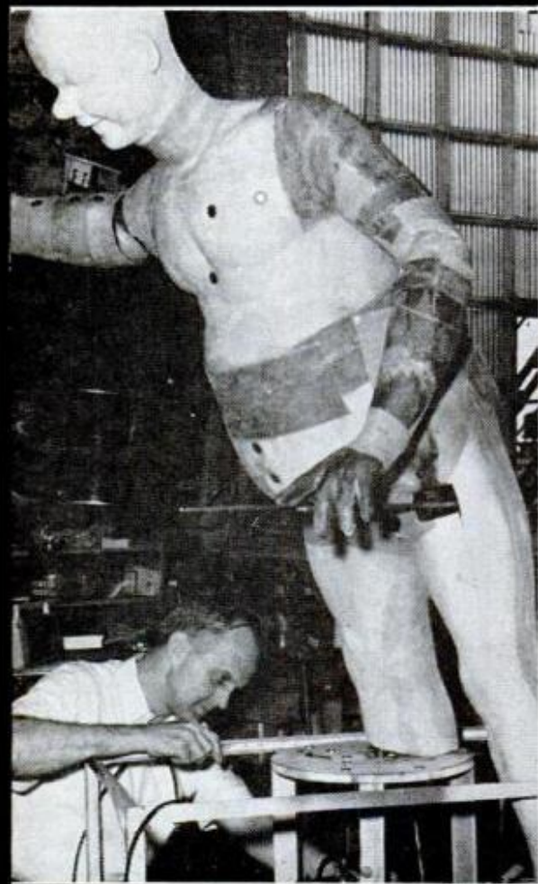
SANTA MINUS RED SUIT gets work done on his motor, which activates shafts running up leg. They, in turn, make his right arm wave
