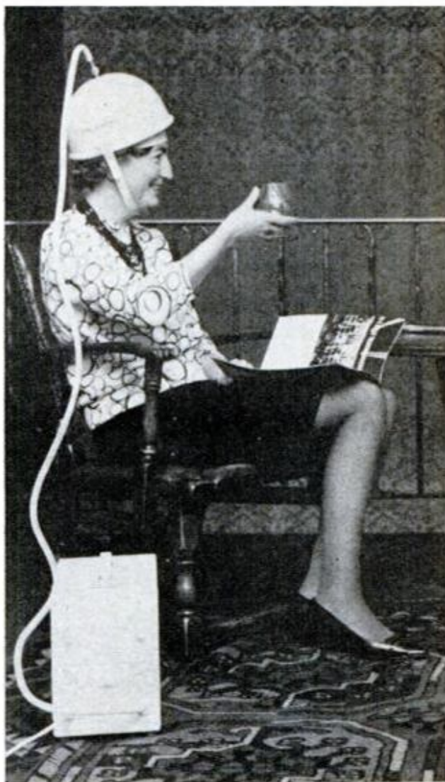
She's enjoying an air massage at home without interruption of her other activities. The plastic helmet is alternately filled with air under pressure, then exhausted of air. That action gives the user of the new German machine a brisk scalp massage.
