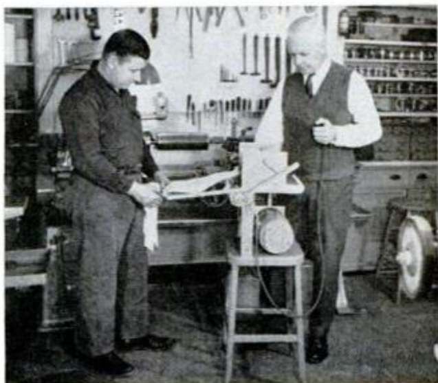
CLOTH-LIFTING MACHINE is now used in a laundry for folding towels; other versions are being developed to handle cloth during garment manufacture
