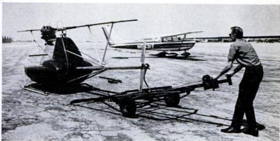
SCHRAMM HELICOPTER weighs 500 pounds empty and can easily be handled by one man. Engine is 100 hp and can power it to 100 mph up to a ceiling of about 12,000 feet
