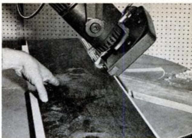
TOP-GRAIN MOLDING is best done in outboard position with molding head centered on rip trough. Feather board clamped to table holds work against fence
