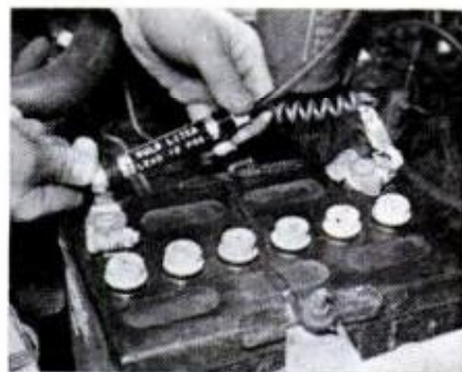
CHECK THE POLARITY of the battery with the tester. With the clip to the positive terminal and the case to negative, the bulb will light
