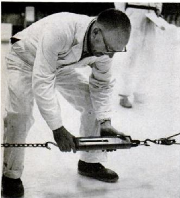
SCALE WITH 500-LB. CAPACITY hooked between test vehicles indicated tires equipped with ceramic studs would out-pull plain snow tires on ice
