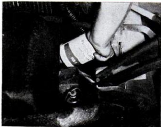
HAND TIGHTENING is the slogan for oil filters. Wrenches can crush the canister or ruin the gasket
