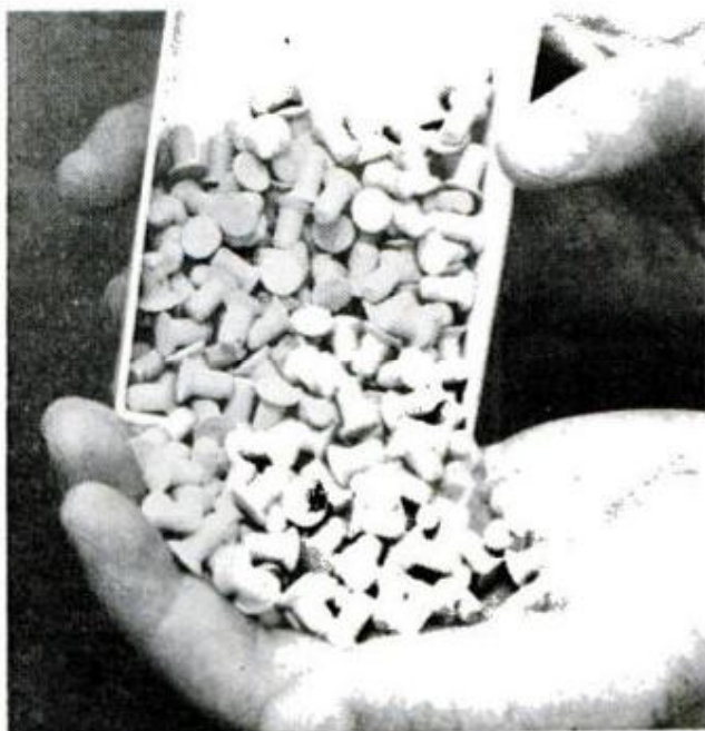
COATING ON RIVETS holds millions of capsules containing a rust preventive. When rivet is hammered into place, capsules break to release primer
