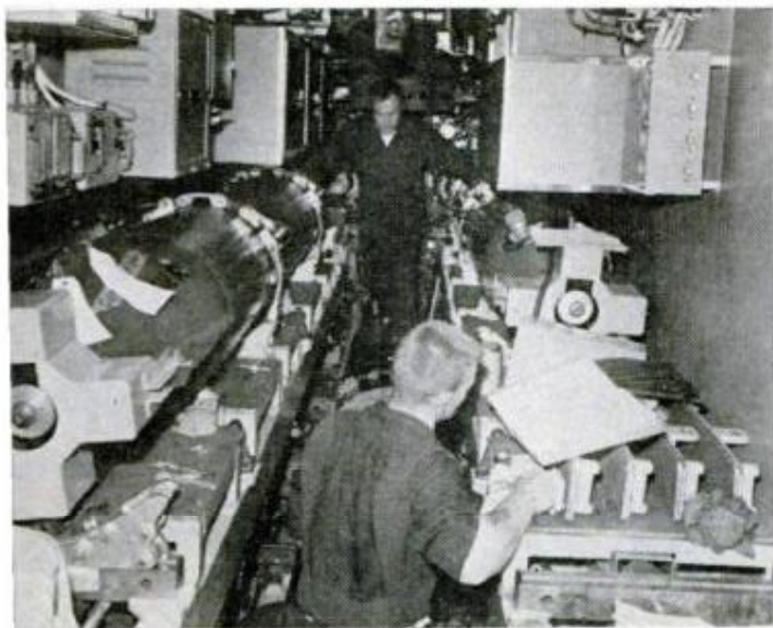
TORPEDO CREW readies "fish" for mock attack on enemy. High-pressure water ram pushes torpedo from tube, catapulting it out for run on target NOVEMBER 1966
