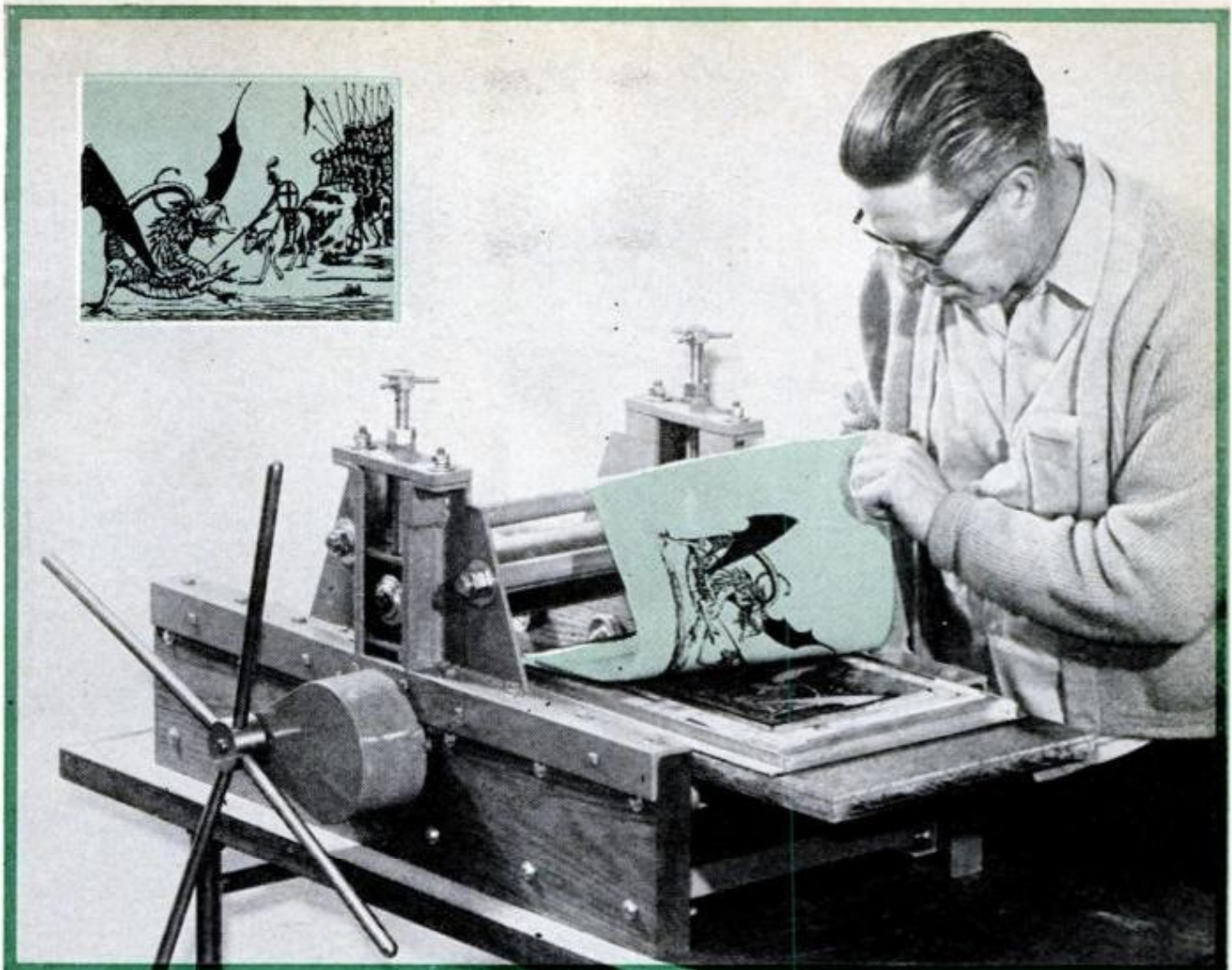
FIRST IMPRESSION of woodcut (see inset) is a quality check to determine final adjustments for the press
