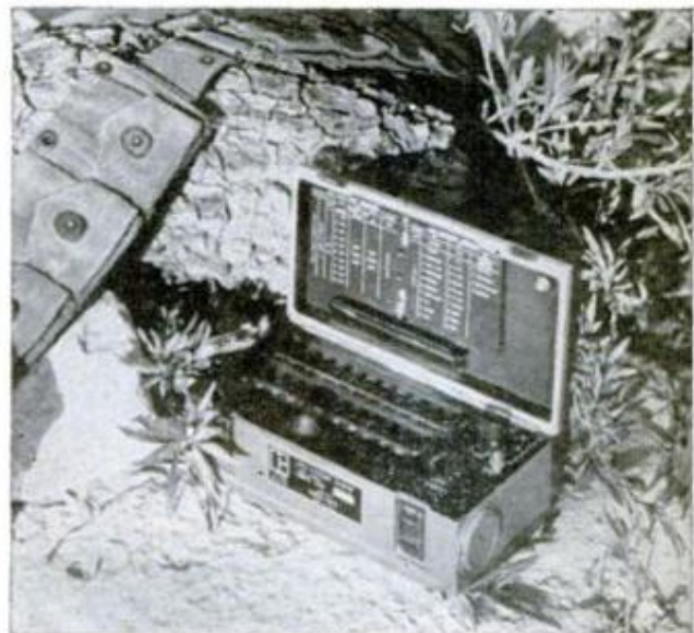
Canteen-sized transmitter is triggered to transmit any of 22 coded messages with the flick of a switch. The Litton Industries unit is called the Digital Message Entry Device, although the programmed transmissions can be switched out in favor of voice communications when necessary. Messages are received and unscrambled on field receivers which send an audible tone acknowledging receipt of the message.
