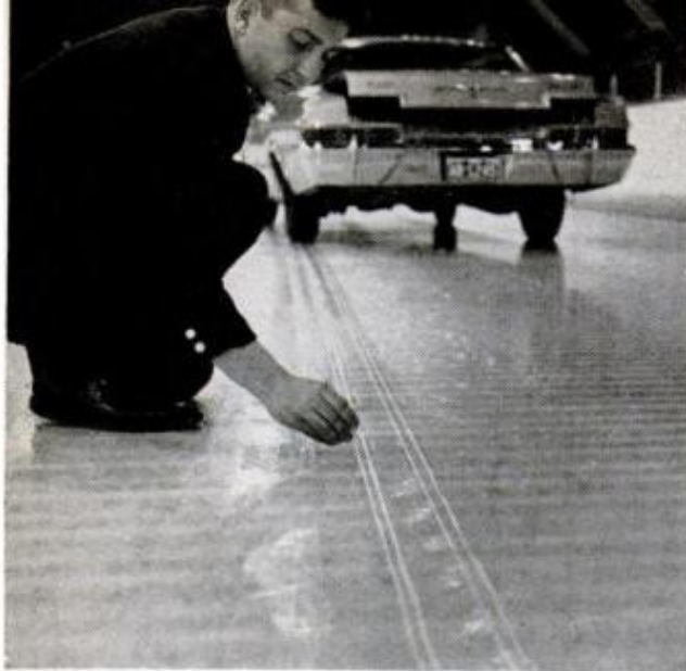
STUD SCRATCHES were easy to identify on smooth ice following braking tests. Studless snow tires tracked noticeable smears, made possible exact measurements
