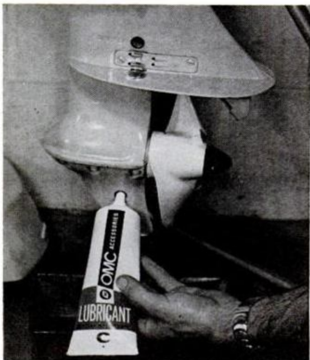
LUBRICATE GEAR CASE in the usual way, squeezing grease through the lower hole until case is filled
