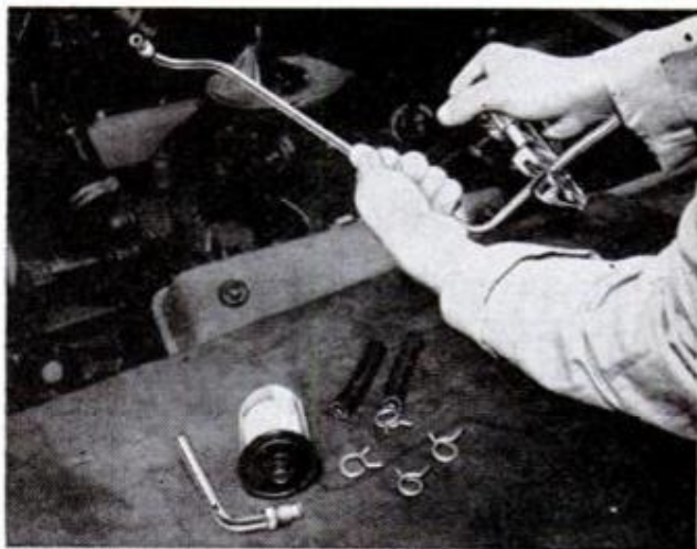
DETACH THE FUEL LINE and cut it at a relatively straight section, removing about 3½ in. of tubing
