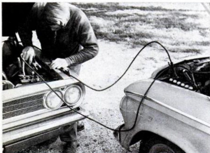
JUMPER CABLES GIVE QUICK STARTS with a weakened battery, but be sure of proper hookup to protect the rectifiers in the alternator
