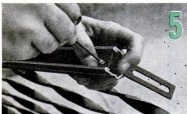
NO DRILLING IN IRON IS NEEDED. Slip the L-bars into the ends of the railings and tighten the socket setscrews on the tension plates. Bend each L-bar to the angle of the cut end. Before mounting on wall, check distances from bottom rail to stair nosings
