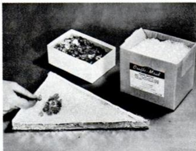
SPREAD LAYER OF CRYSTALS 3/8-in. deep in tray and add pattern of color chips. After pane is baked, glue it in rabbets by means of assembly jig shown below
