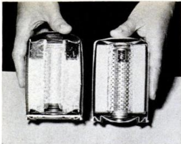
POPULAR OIL FILTERS are the waste-pack with viscose type (left) and those using micronic paper
