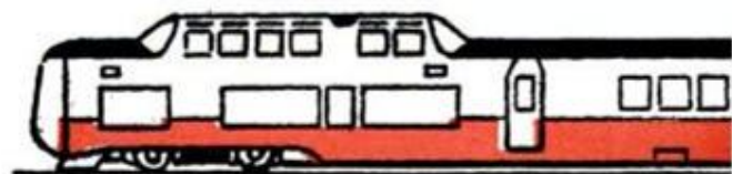
SUPPORTED AT THE TOP , "pendulum car" bodies respond to centrifugal force by banking inward on curves. Air springs produce a soft, stable ride
