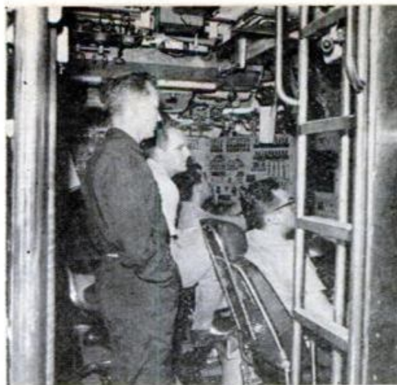
CONTROL AREA is enlarged cockpit, holding 12 men or more. Underwater maneuvers are controlled from here as airliner's maneuvers are in air
