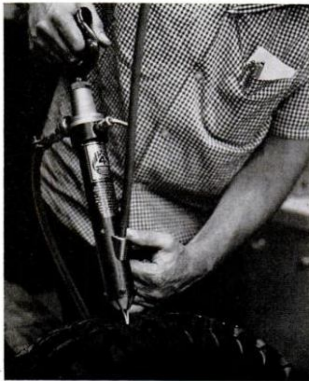
GUIDING "FINGERS" of air gun spread open hole in rubber tread, fire ceramic stud headfirst into tire
