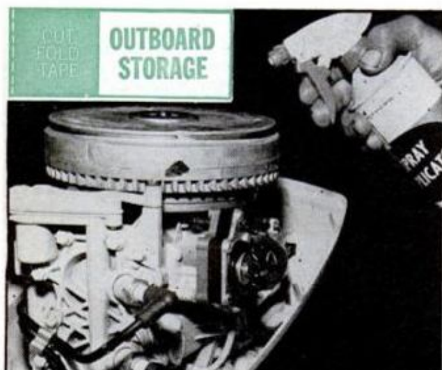
SPRAY POWERHEAD with a corrosion preventive to protect external parts during long storage period
