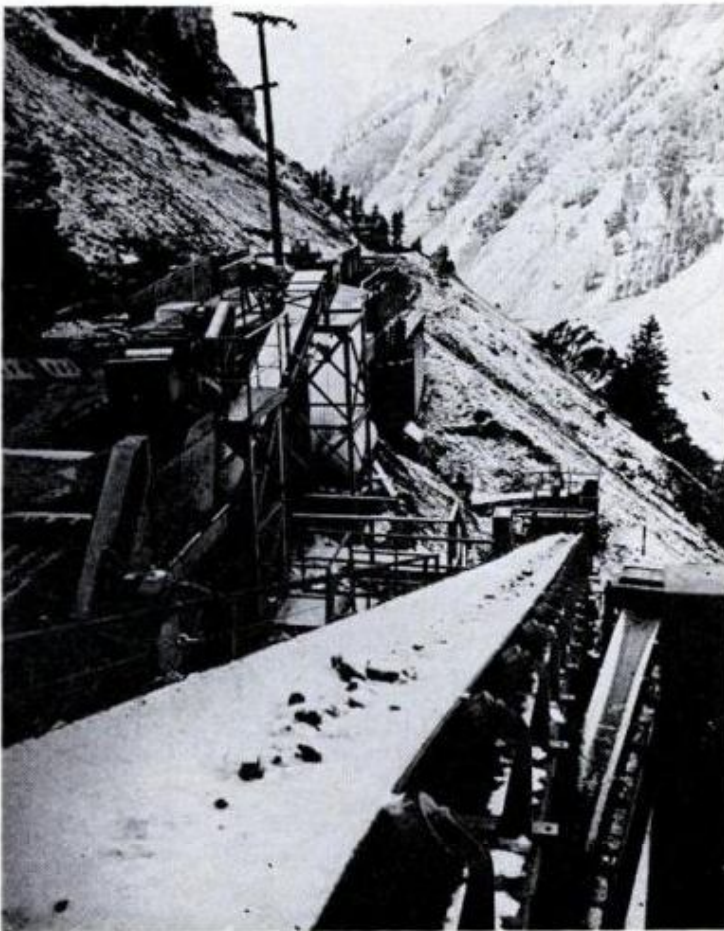
AFTER MINING , shale is crushed and carried by conveyor to processing tower. Heating produces a substance called kerogen, from which oil is refined
