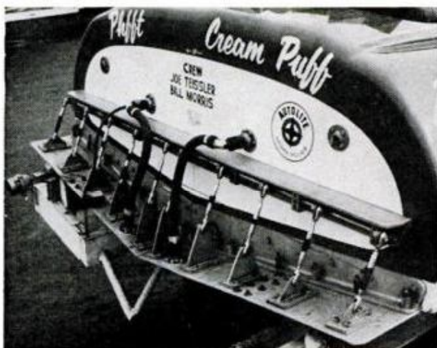
PLANING PLATE serves as extension of boat bottom, can be adjusted up and down during race by driver. Cranking plate down tends to raise stern, lower bow
