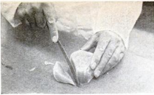
CHUNK OF GASOLINE slices like cheese. Squeezed in wringer, plastic cell walls will burst to release gasoline, which makes up 95 percent of brick
