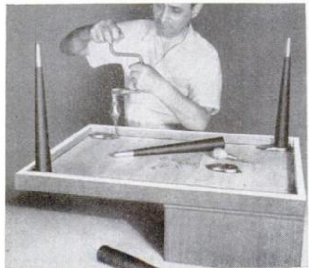
CONVERSION TO TABLE is simple matter of attaching socket plates at four corners and screwing in ready-made legs—removable if you change your mind later
