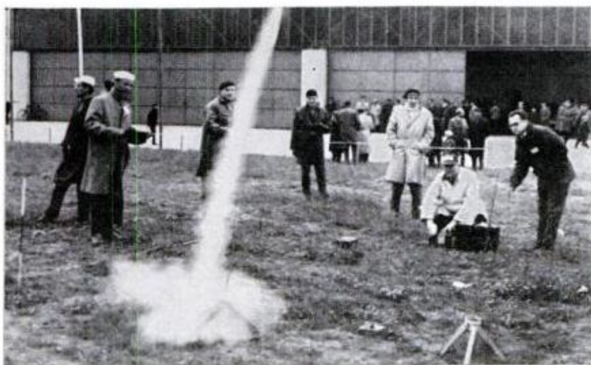
BLASTING OFF , a U.S. rocket is operated from an electric starter by A. W. Guill. When the rocket reaches its ceiling, the specially designed engine fires a forward charge that releases the nose cone and ejects a parachute for safe landing
