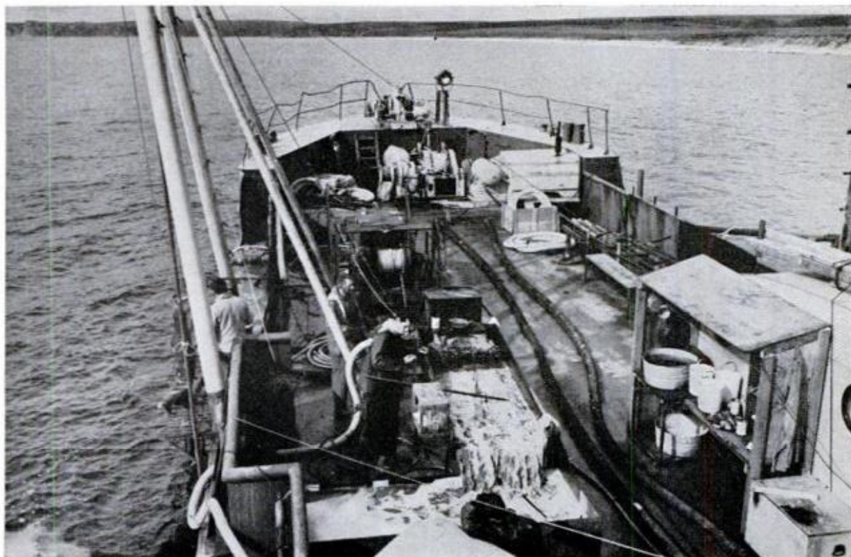
GRAVEL AND SEA WATER pumped from bottom is run through sluice box on deck of prospecting ship
