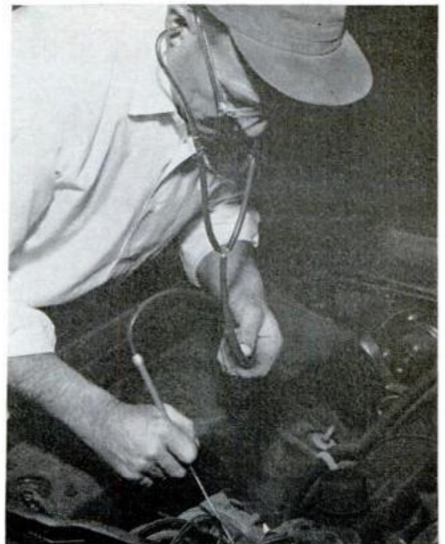
AN AUTOMOTIVE STETHOSCOPE is an excellent aid in diagnosing engine noises. Tool sells for about $7
