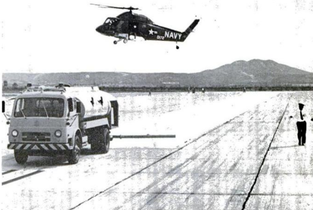
Planes coming in with disabled landing gear can in five minutes be given a 3000-foot-long blanket of foam to slide on. The Navy's new runway-foaming tanker can lay down that blanket, 24 feet wide, to lessen the danger of fire. This method cuts in half the time required by the old method of spraying foam from a hand-held nozzle.
