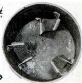
MIXING BUCKET is equipped with stationary blades that are bent by hand and bolted or riveted inside
