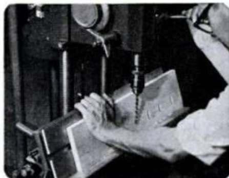
16 1/2" DRILL PRESS —Shopsmith swings instantly into vertical position to drill, mortise, rout.
