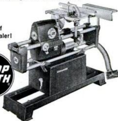
EXCLUSIVE SPEED DIAL —Infinitely variable speed dial insures correct speed for every job (range: 700 to 5200 rpm).
