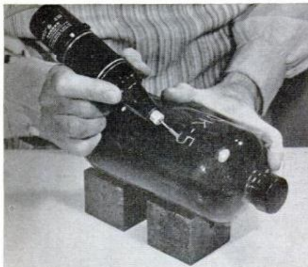
TO WRITE ON GLASS , use tiny abrasive wheel. Larger wheels are better for rounding sharp glass edges
