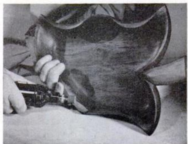
ROUTER ATTACHMENT on Dremel Moto-Tool is being used here to cut straight half-round grooves in wood
