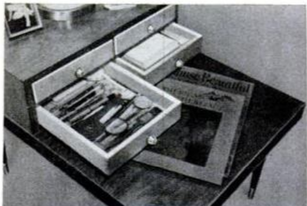
DRAWERS FLOAT over magazines on table because they ride on thick cleats shown in center photo. Drawers store all those small items that can stray
