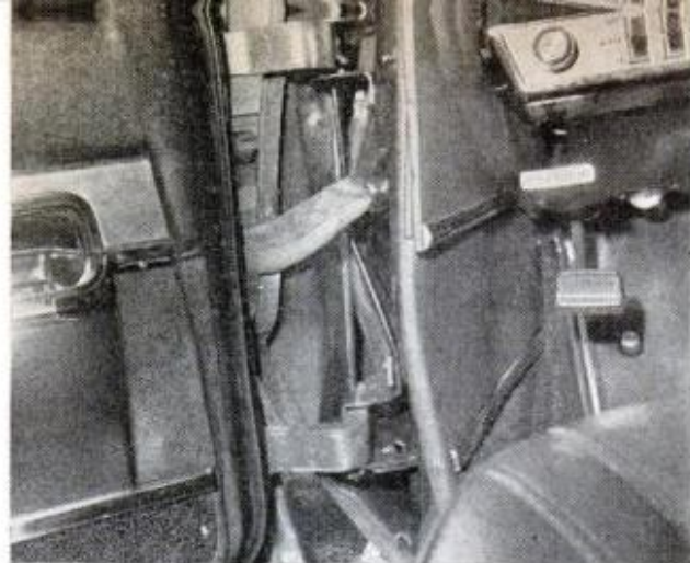
TORONADO doors—big and heavy—open much easier in new models. Required effort is cut in half thanks to new standard spring-operated assistors
