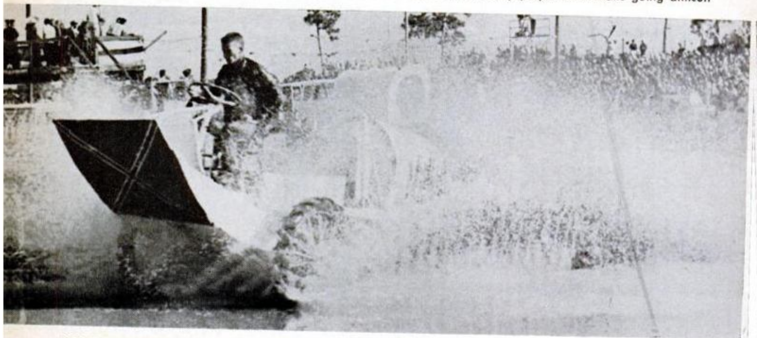
UPSWEPT PROW on this special racing model allows the buggy to hit the potholes and slide on through
