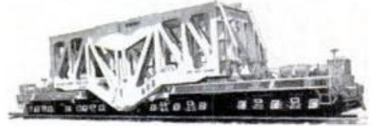
UNIQUE "SCHNABEL" CAR built for Westinghouse separates at center to support the ends of 250-ton transformers. Load-bearing frames with retractable derricks are rigidly latched to the transformer. The big car is shown closed at right
