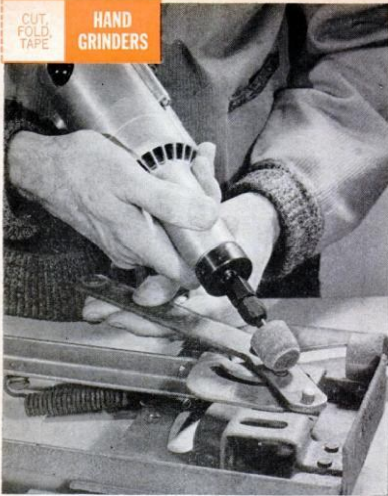
GRINDING OFF RIVET heads is a shop job that goes fast when it's done with hand grinder such as Sears Craftsman model
