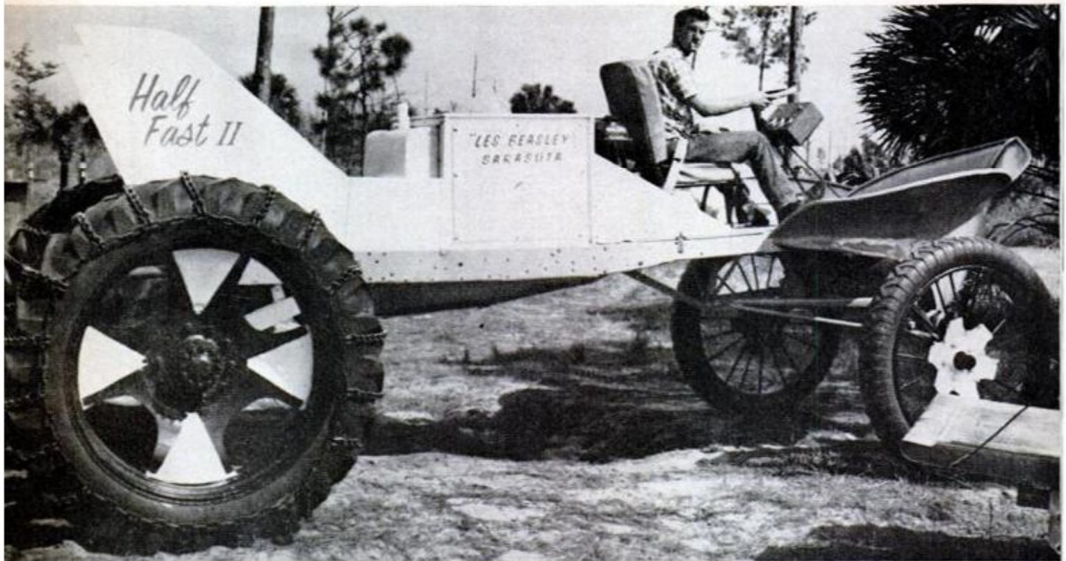
HUGE REAR WHEELS with tractor tires take the full load on this racing model, and the smaller front wheels barely touch the ground when it is under way. Without a seat belt the driver would be thrown at full tilt
