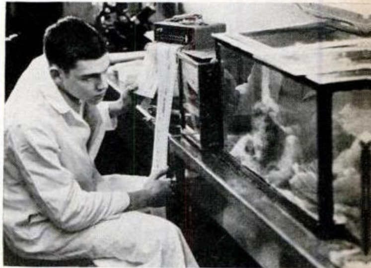
ACTIVITY IN TANK is automatically recorded when fish swims across it and interrupts light beam. Activity records are then checked with phases of moon
