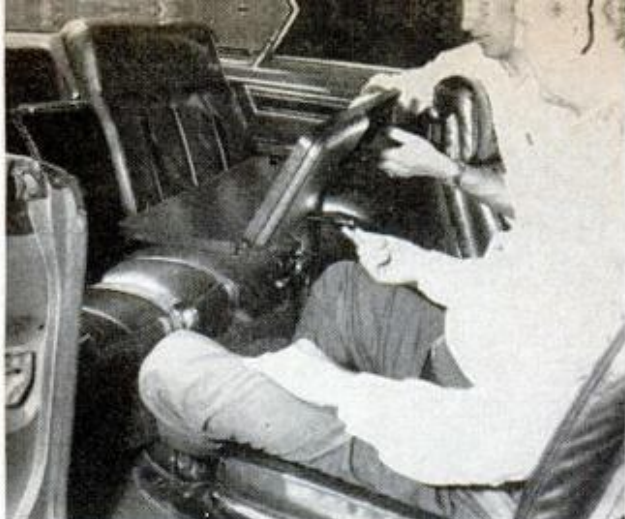
IMPERIAL offers "mobile director" option in Crown Coupe. Front passenger seat can be turned around, the arm rest reversed and unfolded to form a table
