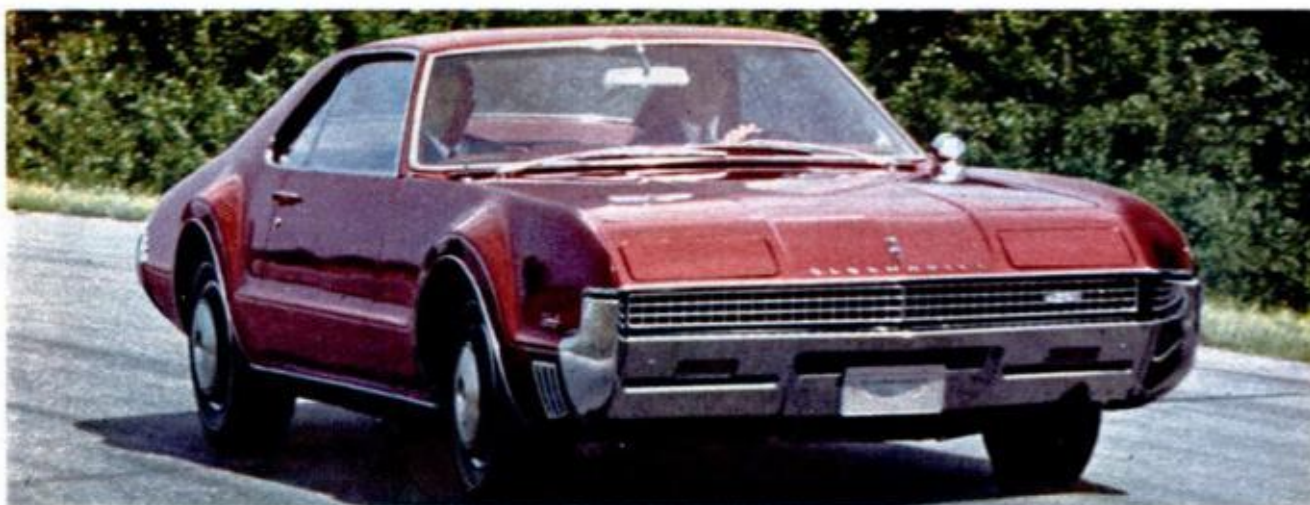
TORONADO headlight covers are flush with hood this year. Olds claims car has a smoother, quieter ride
