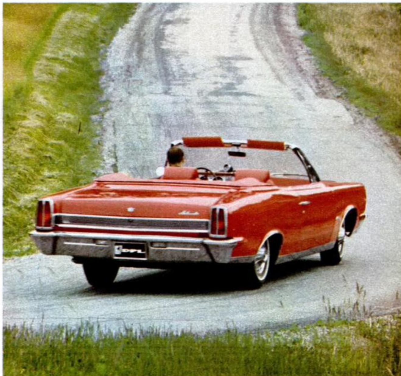
AMBASSADOR is bigger, more luxurious for 1967. Wheelbase is upped to 118 inches, overall length to 202.5
