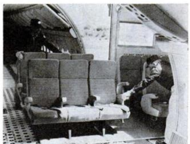
Quick-change artist: A plush passenger-carrying airliner by day, the Boeing 727QC (for quick-change) becomes a cargo carrier by night, doing double duty on United Air Lines. Seats, mounted on carpeted pallets, are unlocked and moved over floor-mounted rollers to a storage van (above) and replaced by pre-packed cargo pallets in a few minutes (left).
