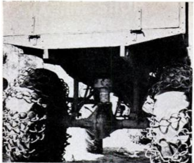
CHAINS ARE LIMITED to seven-inch links of half-inch stock, and many are welded from reinforcing rod
