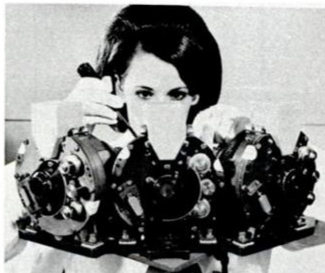
Three eyes for a space observer. This three-camera television system was designed for "Nimbus," NASA's experimental weather satellite. Built by the Astro-Electronics Division of RCA, the cameras will cover a path 2000 miles wide, taking 12,000 pictures of the earth's surface and cloud formations each day from an altitude of 600 miles.
