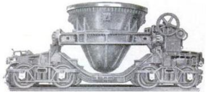
SELDOM SEEN , because most are outlawed on the high iron, are fleets of industrial cars. Basically, designs don't change, but capacities do. For example: single-pot slag haulers (right) are now losing out to larger multibucket jobs
