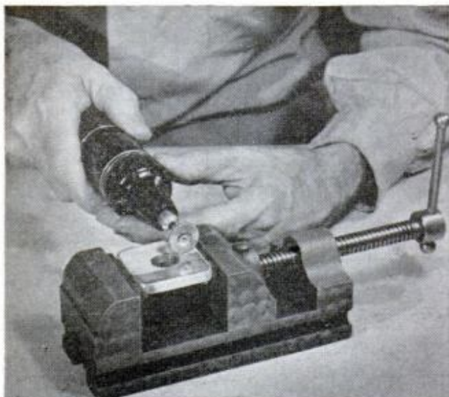
BRUSHED EFFECT on brass can be produced with wire brush chucked in grinder. Movement controls pattern
