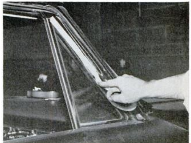
WORN OR LOOSE WINDOW seals are another source of wind noise. Road test car after taping each window
