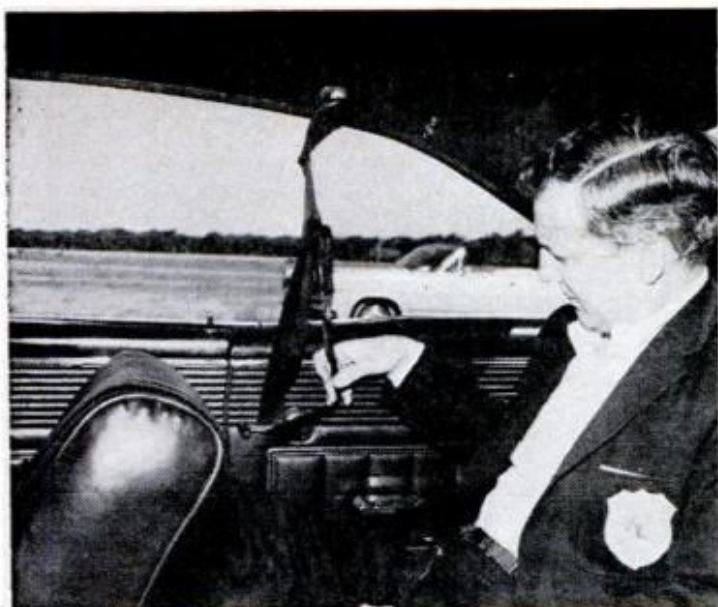
MERCURY still hasn't figured out how to stow the optional shoulder harness. This arrangement is bad
