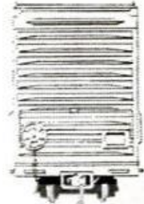
"SIDE-DOOR PULLMANS" have been given a two-way stretch—to 91-foot length and 15-foot height. But platform clearances still hold width to 10 feet
