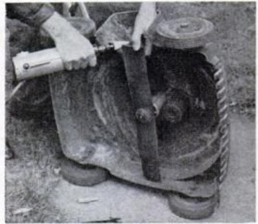
MOWER BLADE can be sharpened right on the mower with a conical abrasive wheel
