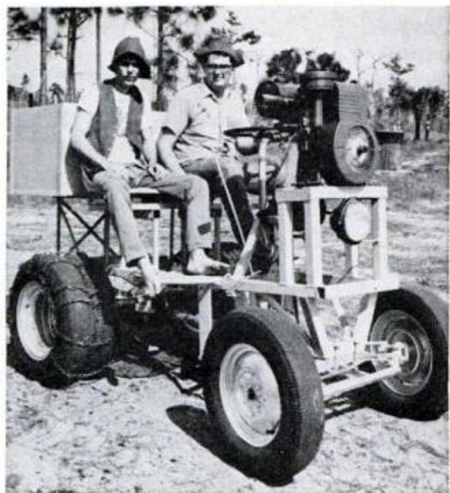
COMPLETELY HANDMADE , this welded frame putt-putt has air-cooled engine mounted high to keep it dry
