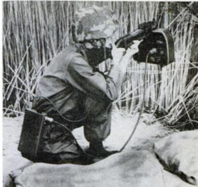
Two-pound battlefield radar mounts on grenade launchers, bazookas and machine guns to spot targets and indicate distance. It also has an FM radio for use between men using the device. Radar and radio are controlled by just three knobs.
