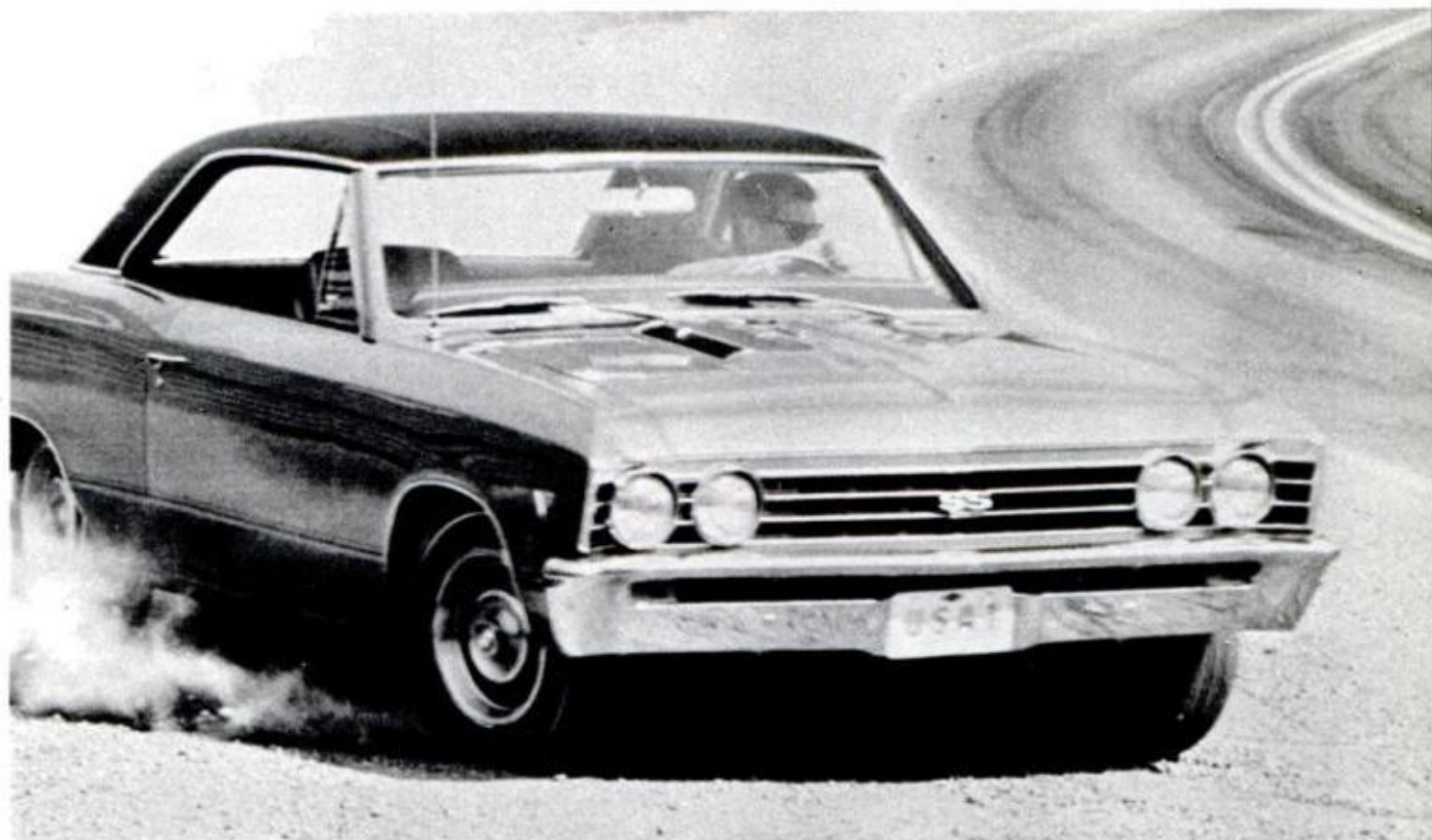
CHEVELLE SUPER SPORT 396 is available as a two-door hardtop coupe and convertible. Car's standard engine delivers brisk 325 hp while optional high-performance version cranks out 350. Car weighs 3600 pounds
