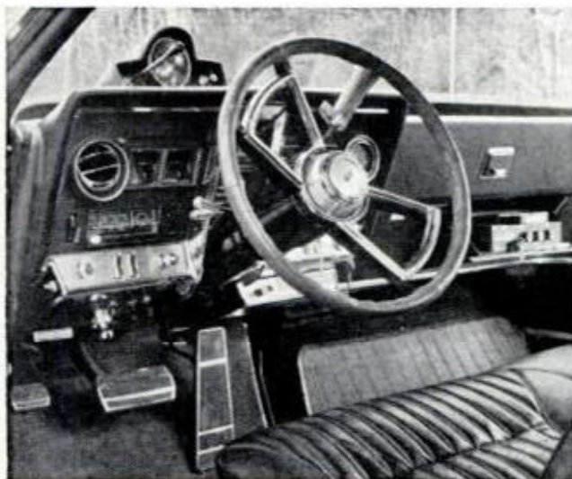
EXTRA DASH PANEL houses tach, fog-light switch and driving light flasher. Wheel has laced leather cover
