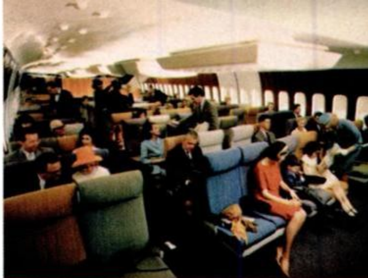
SEATING CONFIGURATION for Boeing 747 calls for 9 or 10 abreast, but individual seats will be 10 percent wider than those currently used in the "economy" class
