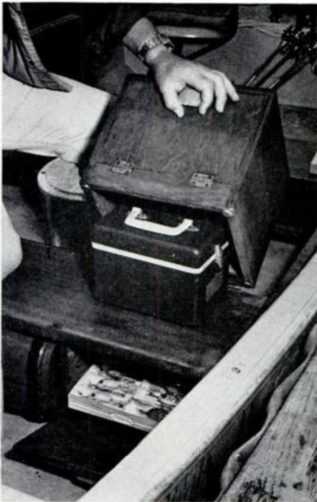
BOW SEAT , a box hinged to the boat's front seat, is also a storage compartment for Dick's electronic fish finder. Using the foot control, right, he can regulate the operation of the electric trolling motor
