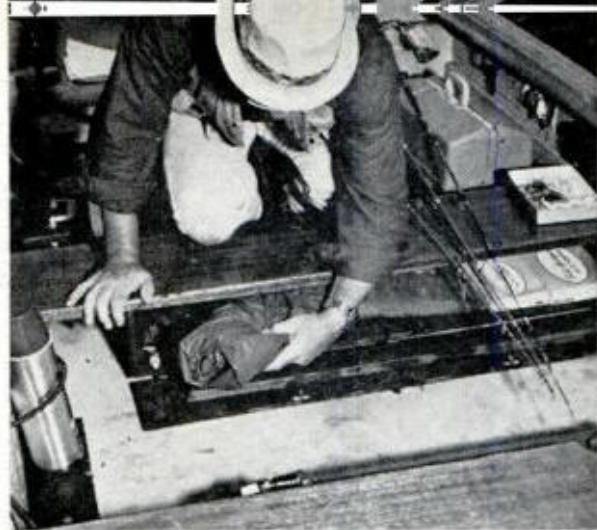
STORAGE CHEST made by enclosing space beneath a seat provides a dry place to put rain gear, tools, lunches and other necessities. It keeps the boat free of clutter, ready for fishing
