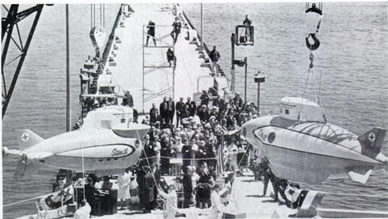
Midget two-man subs, Star II and Star III, to be used principally for deep-sea research, get their first taste of salt water as they are launched by crane by General Dynamics Corp. With tail fins and "rudders" they look like chubby aircraft. The larger can operate at a depth of 2000 feet, has a range of 15 miles and a speed of five knots. The Navy foresees use of such subs in surveillance.
