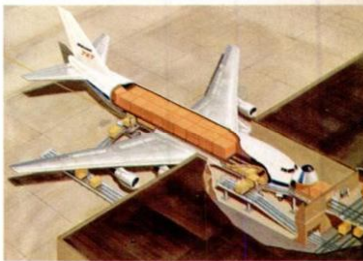
CONTAINERIZED CARGO in 10-foot-long boxes will roll on at rate of 100 tons—plane's capacity—in under 10 minutes. There will be both nose and side loading
