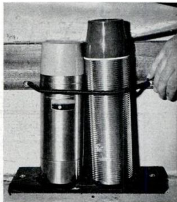
HOT AND COLD DRINKS are always carried in the same place—seated in a recessed base and secured to the side of the boat with a screen-door spring. They're easy to remove, but can't fall over
