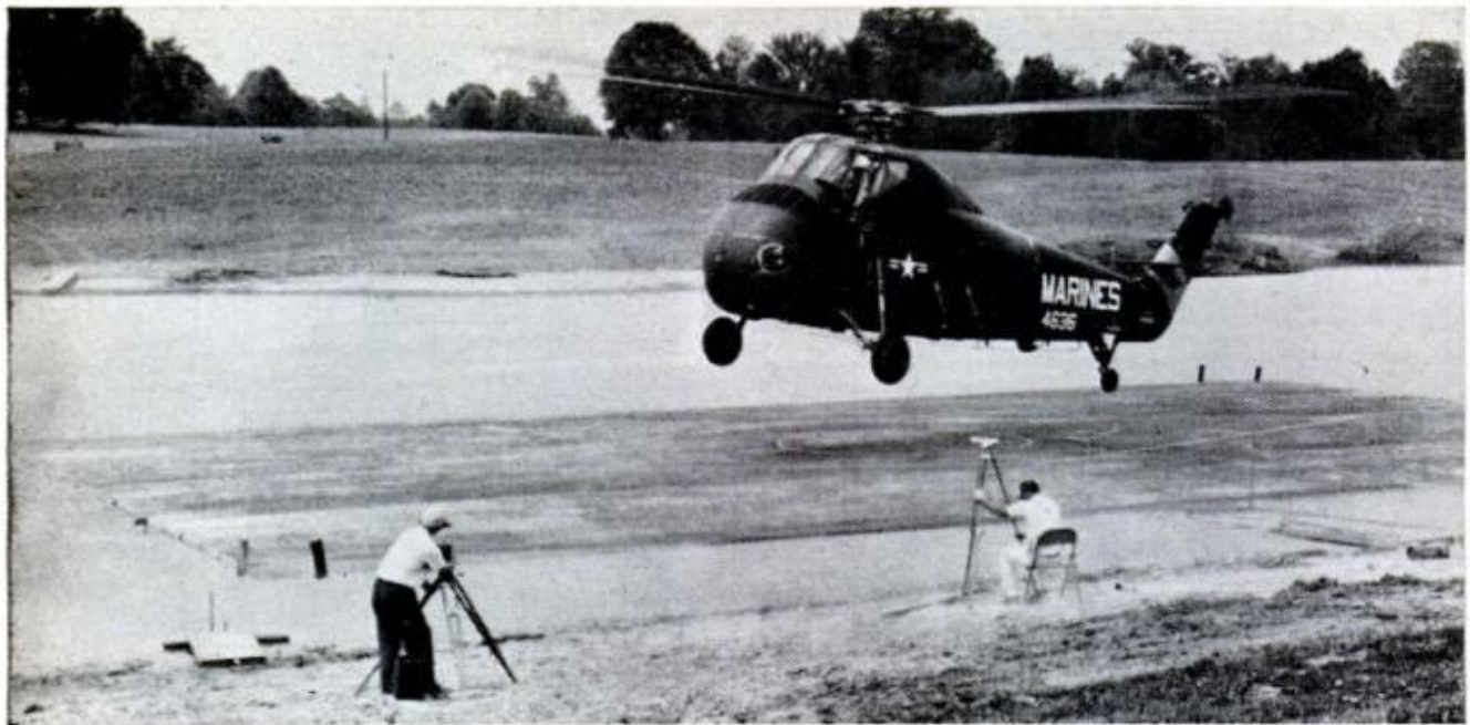
Floating landing mat , made of bonded aluminum sections with polyurethane cores, can be set up in marshes and rice paddies converting them into airfields for helicopters. The mats, which can support impact weights up to 26,000 pounds, have a two-year life expectancy.
