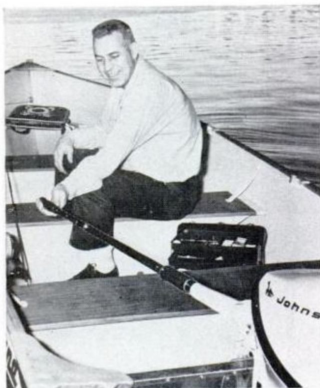
Extension handle for outboards permits midships control of throttle and steering. The handle can be snapped on or off in seconds, and extends from 28 to 37 inches, with locking positions at three-inch intervals. It's made by Waukegan Outdoor Products, 1534 Washington St., Waukegan, Ill.
