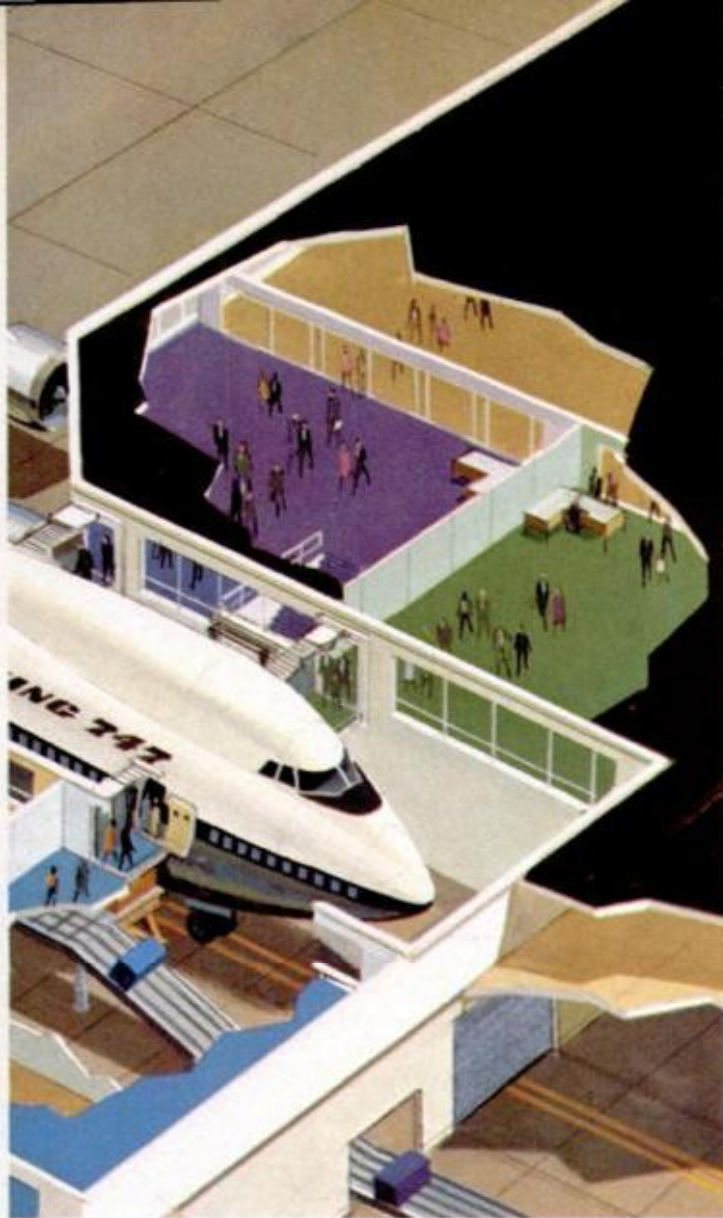
TO SPEED BOARDING , 490-passenger Boeing will require four waiting rooms, each with entrance to airliner. Speedy conveyors will carry aboard all baggage
