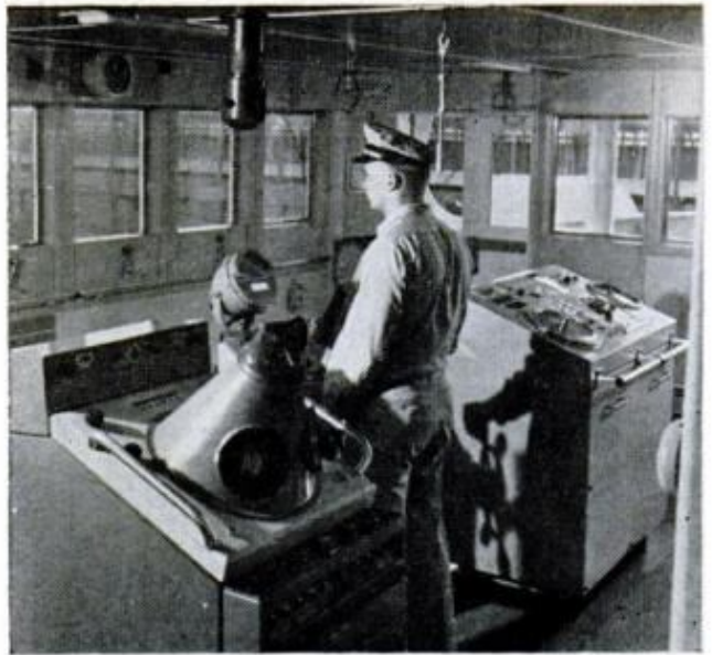
SLIGHT TURN OF WHEEL on bridge console (at helmsman's right) instantly slows or speeds up the ship
