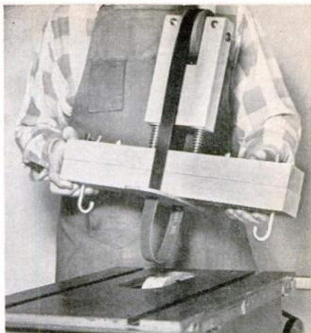
ON AND OFF in minutes, attachment won't interfere with saw's usual function. Just put drive pulley on arbor and tighten two hook bolts to anchor base
