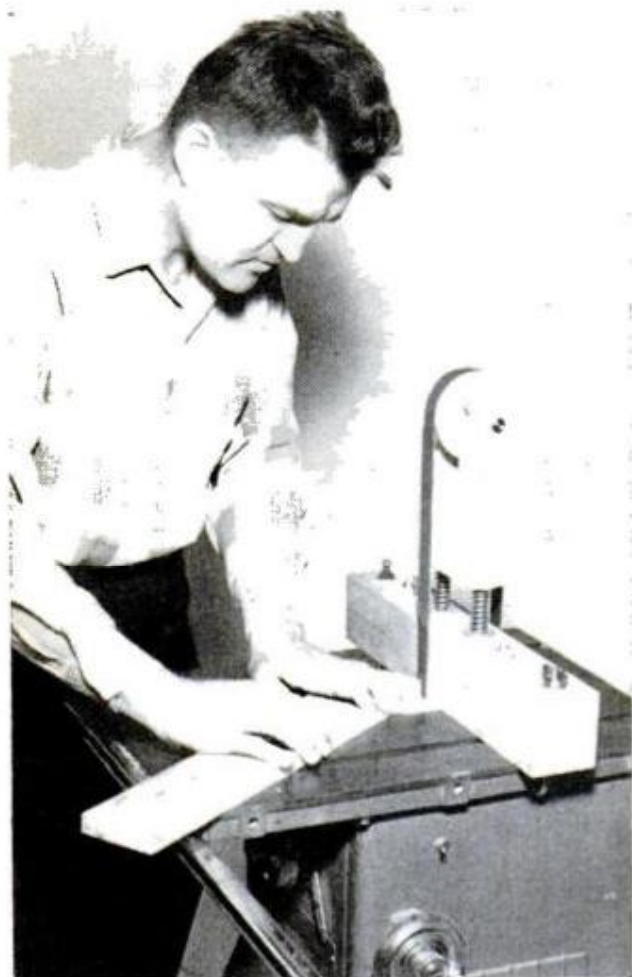
CLAMPED TO SAW , attachment makes use of tool's table as well as its motor. Note how doubled 2x4 base serves as backup plate for square sanding
