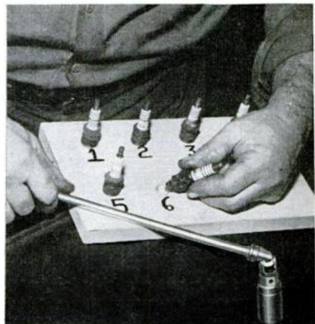
POSITIVE SPARKPLUG ANALYSIS can be achieved with board drilled and numbered as shown (see text)
