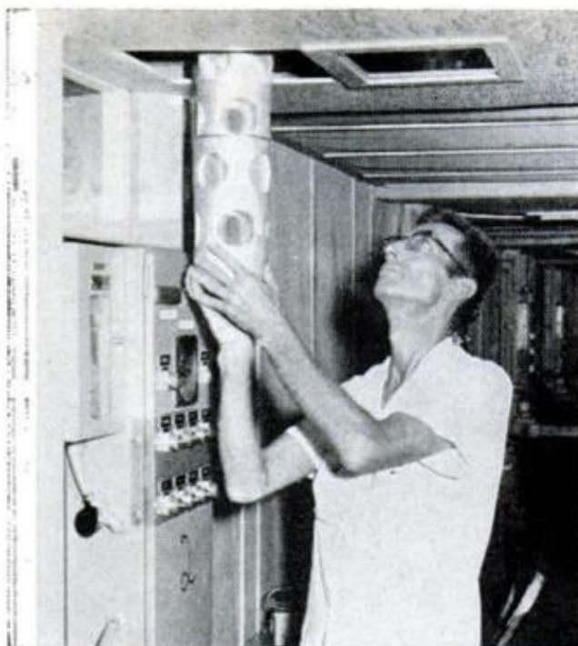
CANISTER FILLED WITH BUGS in pupa stage is pushed up into cobalt-60 chamber for sterilizing blast
