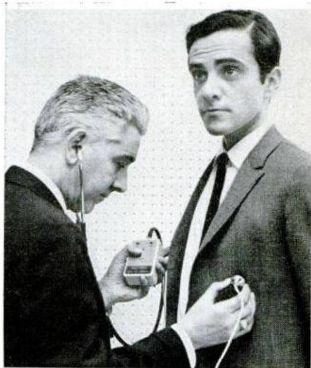
Hi-fi for the heart. Far more sensitive than conventional instruments is this new stethoscope that uses a microphone and six-transistor amplifier. The unit can easily pick up heart and chest sounds through several layers of clothing.
