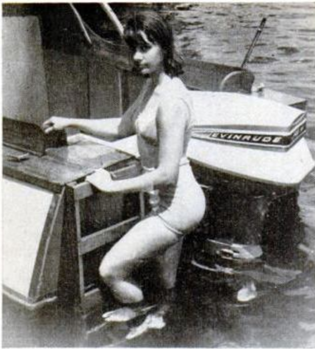
1/2" No. 8 BRASS SCREWS AND GLUE SECURE 1x1 CLEATS TO LADDER
