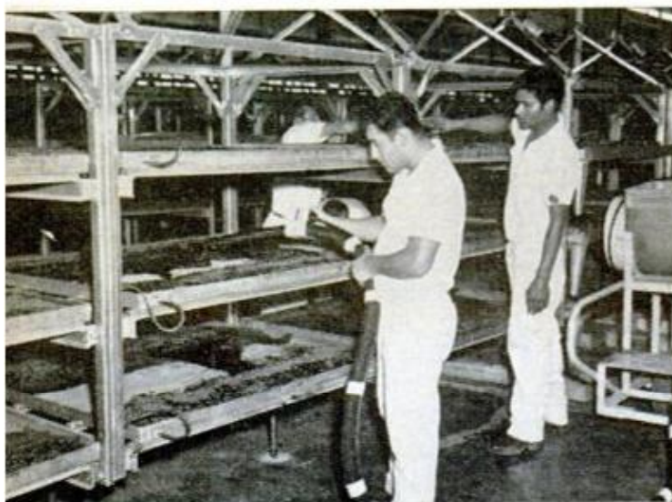
START OF PRODUCTION LINE: Newly hatched larvae are beefed up with special food mixture and are kept a comfortable 99°F. in traylike heated vats
