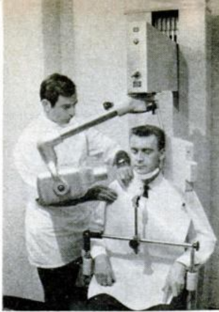
NEW PANORAMIC MACHINE (left) takes picture of whole mouth in one exposure as X-ray tube swings around patient's face. Thick feature in center of film is spinal column. Camera angle is chosen to make patient's front teeth appear on either side of spine
