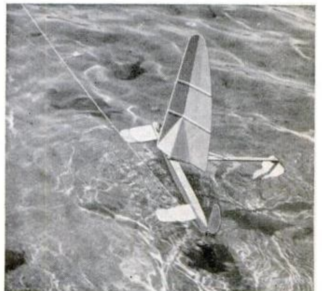
LINE ON STERN runs to a spinning rod, simplifying retrieval. Model can also run free, if you choose
