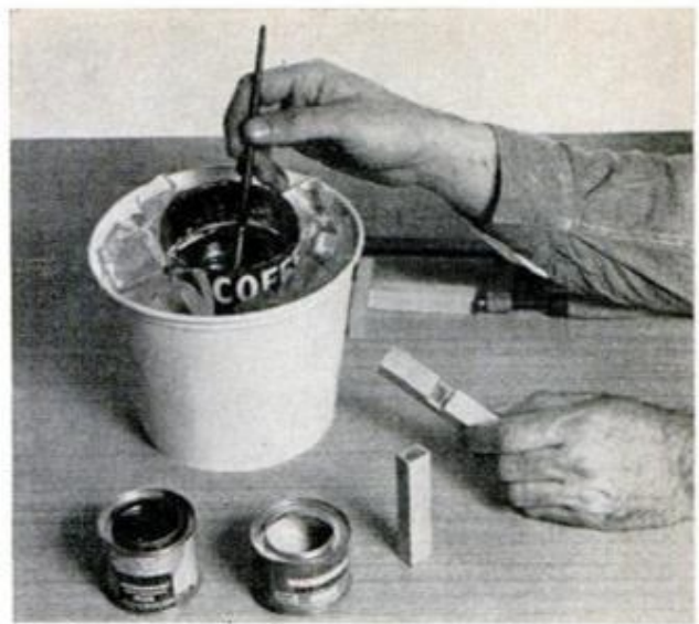
RESORCINOL GLUE CURES FAST in hot weather. You'll prolong its pot life by packing ice around glue pot
