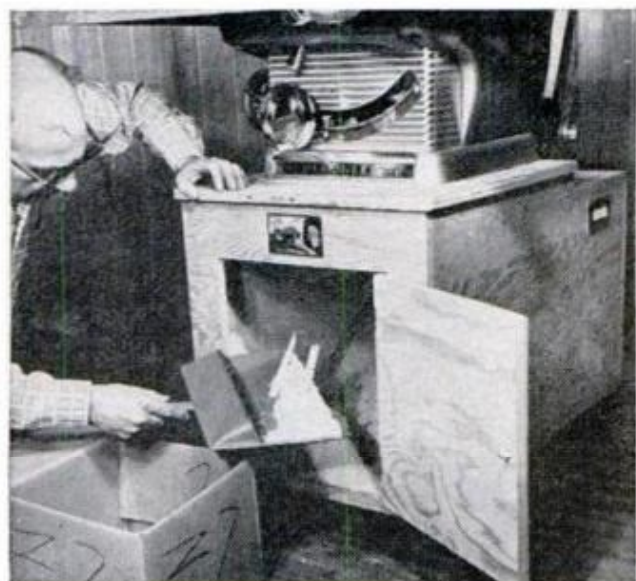
SAWDUST BIN at front of the base keeps the shop clean. Weatherstrip the door all around to seal it
