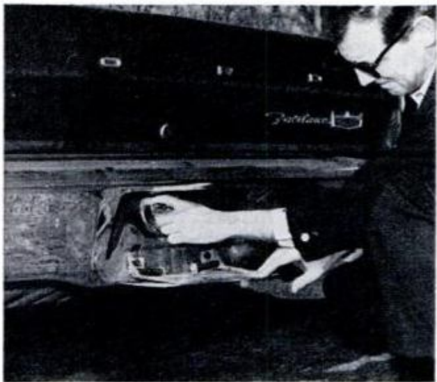
A FLYTRAP and no Venus is the spring-loaded (and how!) license plate covering the gas-fill location. Owners say access is difficult, tank hard to fill
