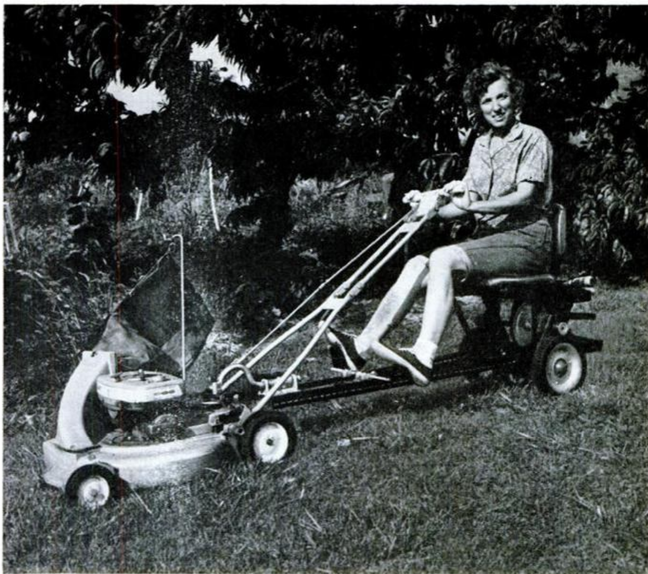
JUST STEER —that's all there is to mowing lawn with this rear-engine driven sulky. Pedals alone, like in Model T Ford, control forward, stop and reverse. Arched hook swivels on body of mower itself for steering
