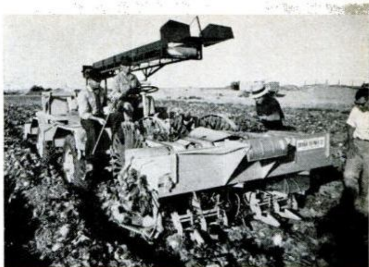
LETTUCE PICKER patrols four rows at once, selecting heads ripe for harvest and leaving young ones behind. Feeler device tests hardness and swishing blade severs head from stalk
