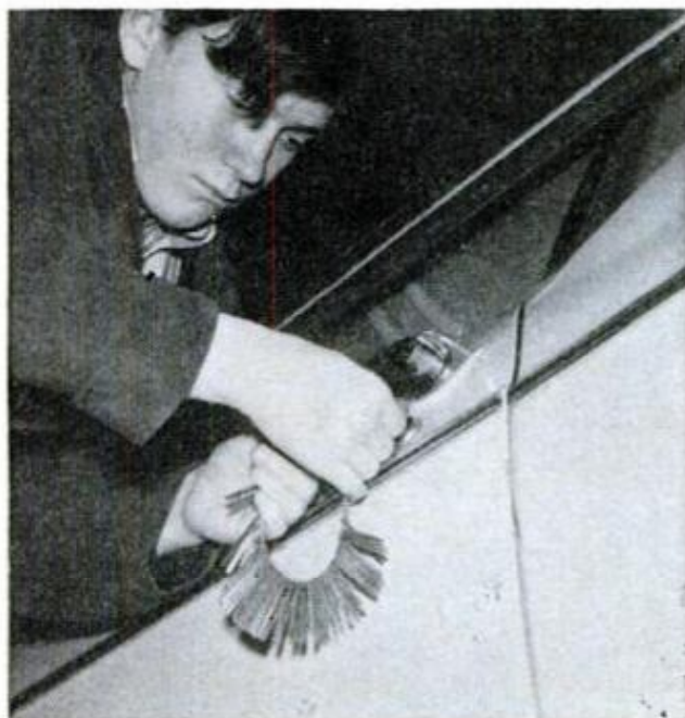
MASTER KEYS are tried on locked car until thief finds one that fits. The key is marked, and the thief returns at his convenience to drive it away
