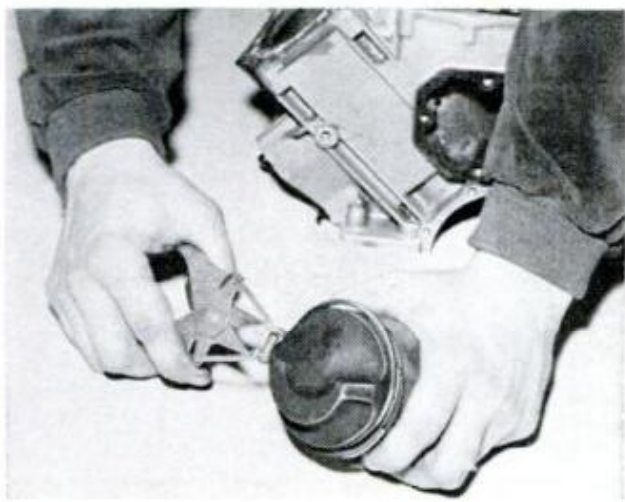
REPLACE RINGS and hone cylinder walls. The few extra dollars involved will add years to engine's life
