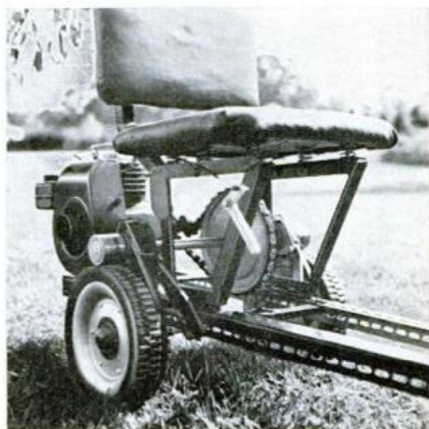
UNDER VIEW of driver's seat from right side, showing L-shaped throttle handle, sectional V-belt from engine to jackshaft and right roller on wheel. Exhaust is behind driver; doesn't bother him on hot day
