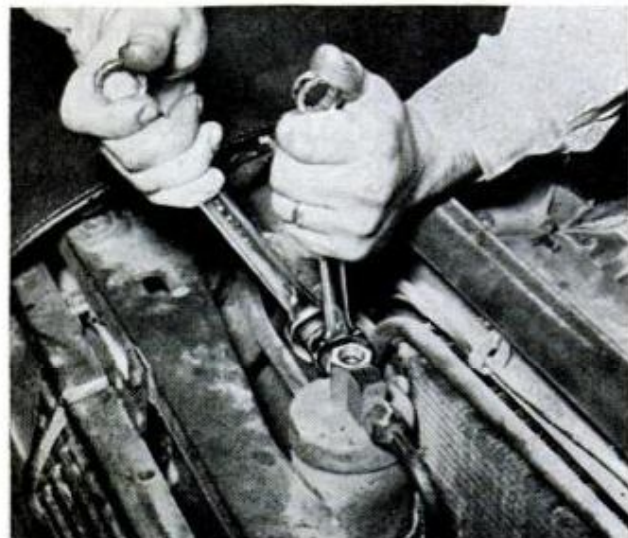
RECEIVER-DRYER UNIT is pulled for a replacement. A clogged filter may require this after a few years
