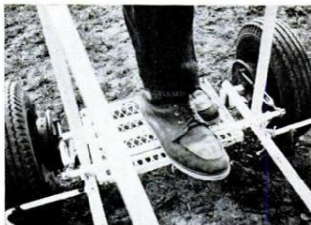
WHEELED SLEDS have not replaced the snow sled, and snow racing is still popular, but the three-wheel carts, which are little more than a steel frame with a steel mesh step for the driver, have enabled snow mushers to give added dimension to the sport
