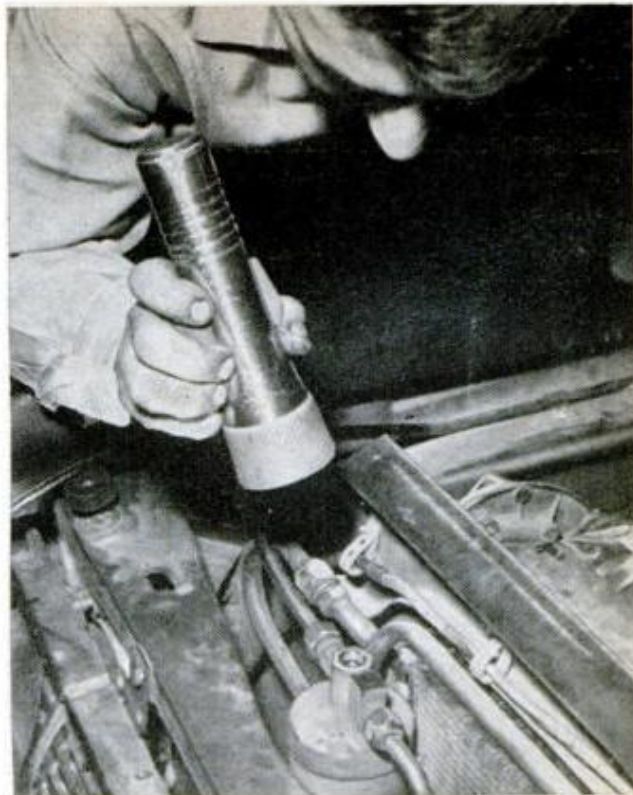
AMOUNT AND CONDITION of refrigerant can be seen through sight glass located on the receiver-dryer
