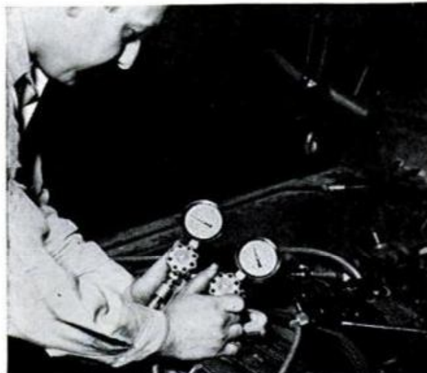
MANIFOLD GAUGE SET , a must for most a/c troubleshooting jobs, tests suction and output in system
