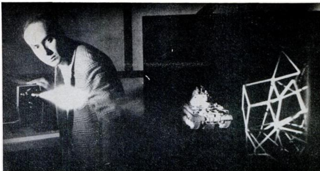
HOLOGRAM DISPLAY: Laser at left illuminates hologram; reconstructed images at right are tank and frame
