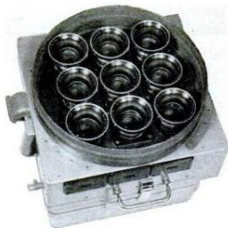
NINE-LENS CAMERA photographs target through nine different filters simultaneously. Two frames above of identical site show remarkable difference. Stream, barely visible in top photo, shows up vividly through another filter
