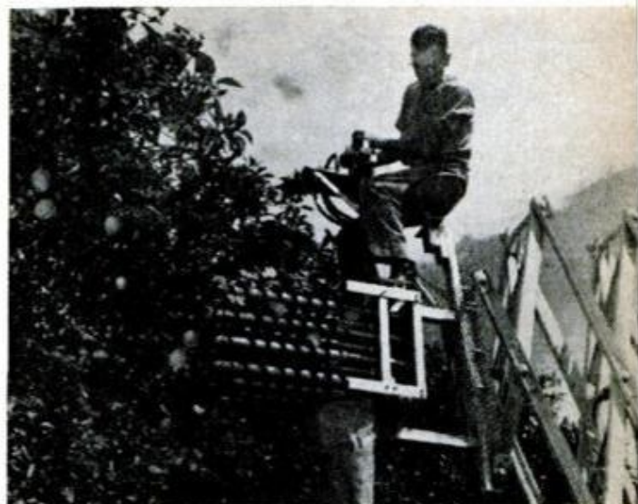
FRUIT PICKER uses group of auger-shaped spindles on end of scissorslike support to spin fruit off trees and drop them uncrushed into long canvas bag
