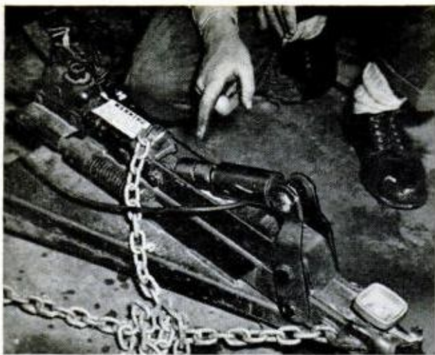
FRONT END of inertia brake system on trailer tongue consists of master cylinder, shock absorber, springs
