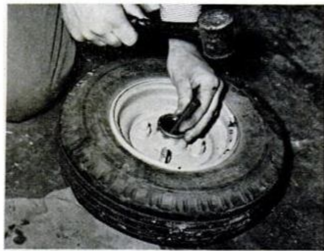
USE A DRIFT to knock out inner bearing. Races of bad bearings should be knocked out and replaced too
