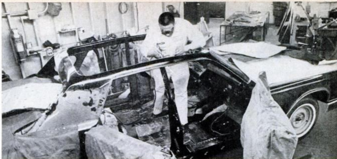
ROUGH EDGES are carefully removed, all gaps filled to assure flawless fit of finished limo's vinyl top
