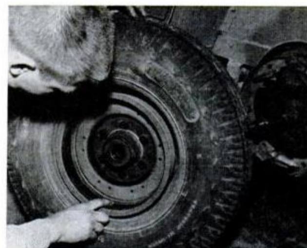
HOW ARE BRAKE DRUMS? If only slightly damaged they can be turned, but replace badly scored drums
