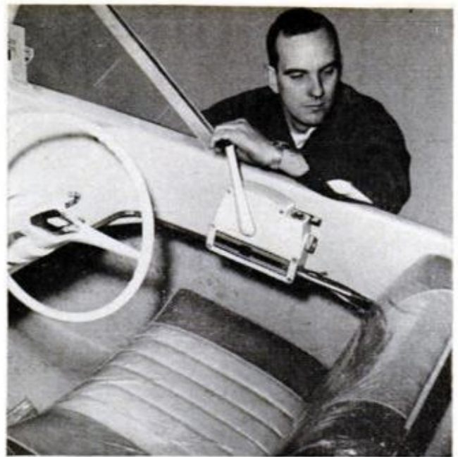
MOVE THE LEVER (or levers, with dual controls) while keeping your eye on cable ends. They should move
