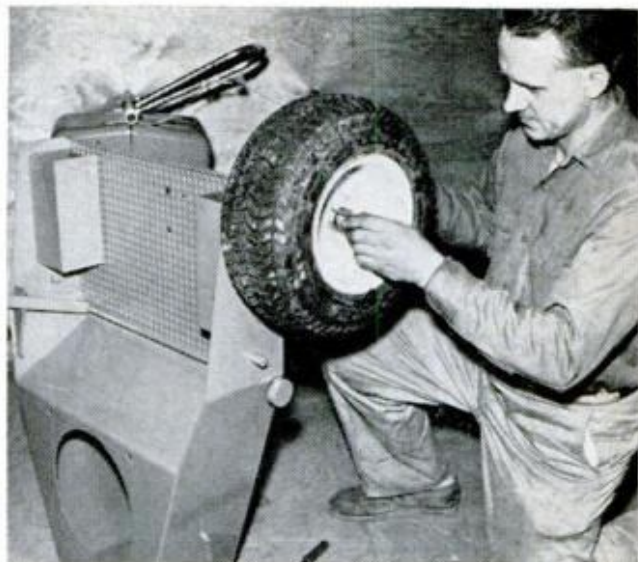
8. REAR WHEELS are secured with castellated nuts and cotter pins, taking care that they turn freely
