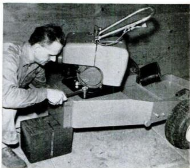
10. FOUR BOLTS hold the Power Wheel in the body. Be sure these are tight before you continue assembly
