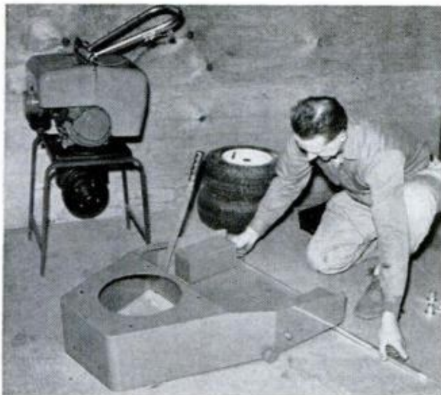
7. REAR AXLE fits into holes in body, is held by bolt through hole in body into tapped hole in axle
