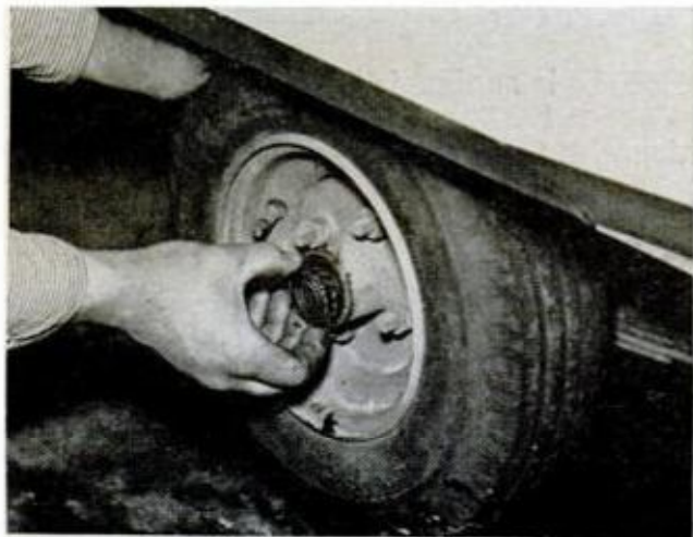
TO SERVICE BEARINGS: remove dust cap, cotter pin, adjusting nut, then wheel; pull bearing from spindle
