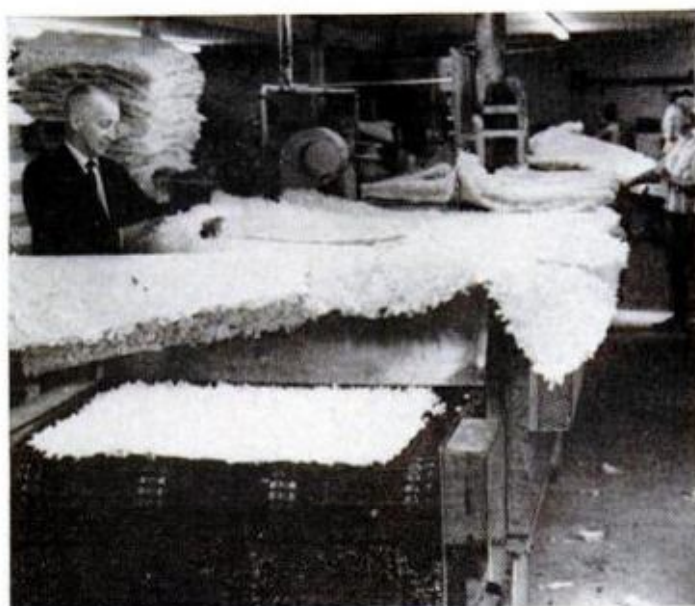
MILES OF COLORFUL PAPER are used to cover the floats; Vaughn's factory has ovens where the tissue is dried to backing before being pinned into place
