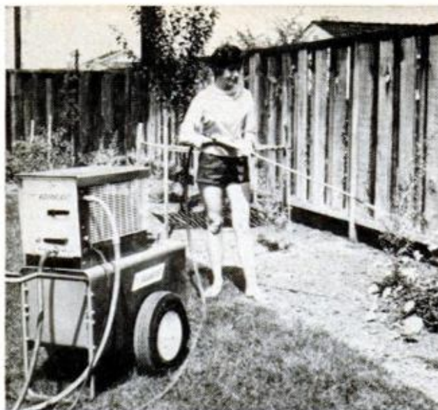
BLAST OF PLANT-TREATING CHEMICALS is applied with Aquablast. It has 30-gallon tank and a 1-hp electric motor to provide the power. Cost is $595
