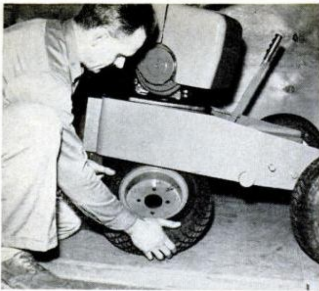
11. FRONT WHEEL slips over studs in the hub of the Power Wheel. Tighten nuts so there's no play left
