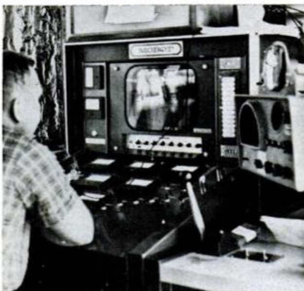
REMOTE-CONTROL MOBOT is sent to bottom by itself and operated from control panel aboard mother ship
