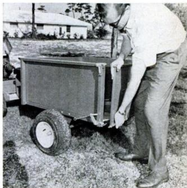
TO TAKE OFF the tailgate entirely, just release two catches on each side. This often simplifies loading
