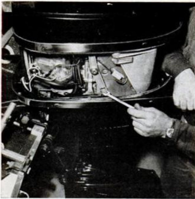
TO CHECK CABLE functioning, disconnect the cables from the engine. This involves only two connections
