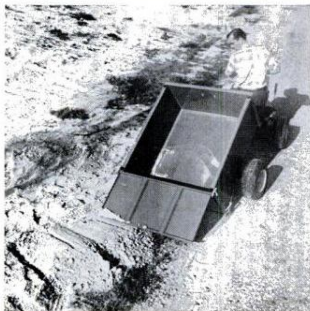
DUMPING LEVER is located on the trailer tongue, can be operated from driver's seat. Tailgate swings out
