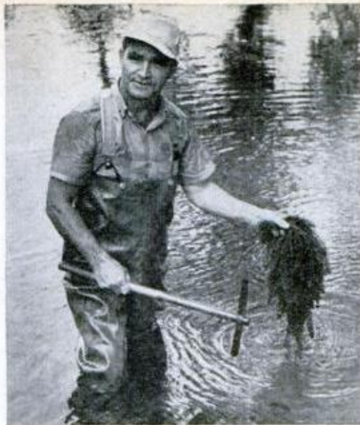
SPECIAL TOOL , butcher knife attached to long wooden handle, gathers moss between blades, then flips the plants over and cuts
