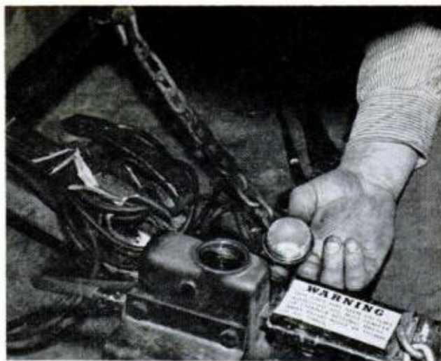
TAKE A PEEK into the master cylinder to check the fluid level. Keep an eye peeled for leaks here too
