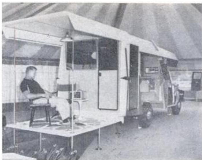
PATIO with slide-out canopy is a feature of the "dream camper" designed for Chevrolet truck chassis
