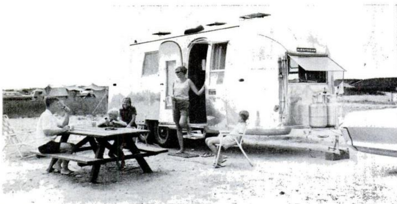
ROUNDED BODY of this 24-foot Airstream is designed to cut down wind resistance. The aluminum reflects the sun, keeping the interior relatively cool even in an open area such as this one at Cape Hatteras, N.C.
