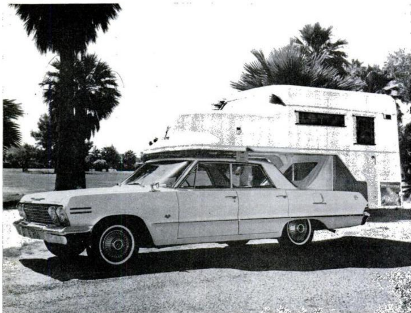
TOTEMOTEL is a fibreglass camper that weighs only 375 pounds and mounts on any station wagon or sedan. It will sleep 11 persons, and is equipped with a butane stove, a sink, an ice chest and a chemical toilet
