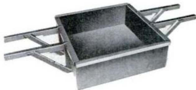
COMPLETE SUMP ASSEMBLY will take exposure to the elements. It is joined with waterproof glue and countersunk screws, waterproofed and painted with gloss enamel before being mounted on the chassis
