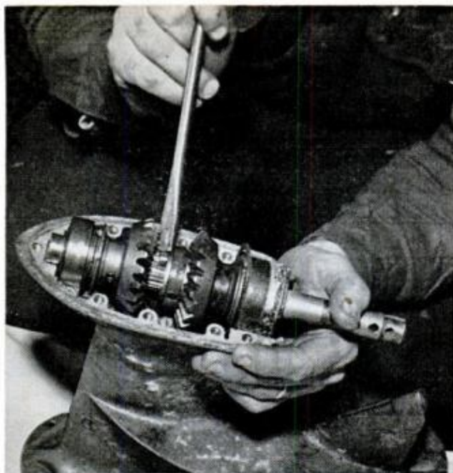
MERCURY-TYPE MOTORS have this spring-loaded ratchet shift dog arrangement. Gears are designed for quick meshing, wear better is snap-shifted to full limit
