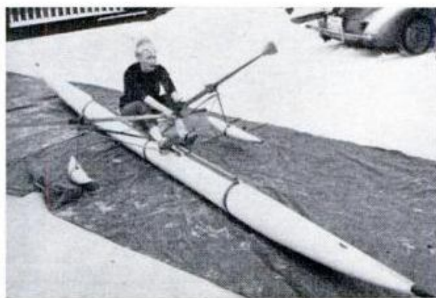
Hot-dog scull introduced by a German firm at the Hamburg Boat Show is basically just an inflated plastic tube which folds into a compact package for carrying. The six-meter boat is said to cost only a third as much as traditional wood models.
