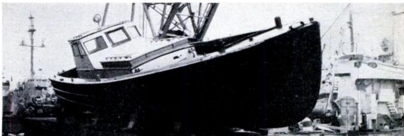
SURPLUS COAST GUARD BUOY BOAT , on delivery to the U. S. Naval Supply Depot, Seattle, was stripped, recaulked and then rehabilitated as a carrier and fitted with a new diesel engine
