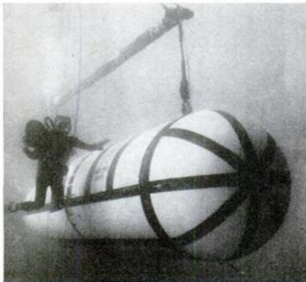
NAVY'S MORAY , another underseas vehicle, has dived to 2000 feet, may eventually go to 6000. Military and scientific groups are both interested in shelf
