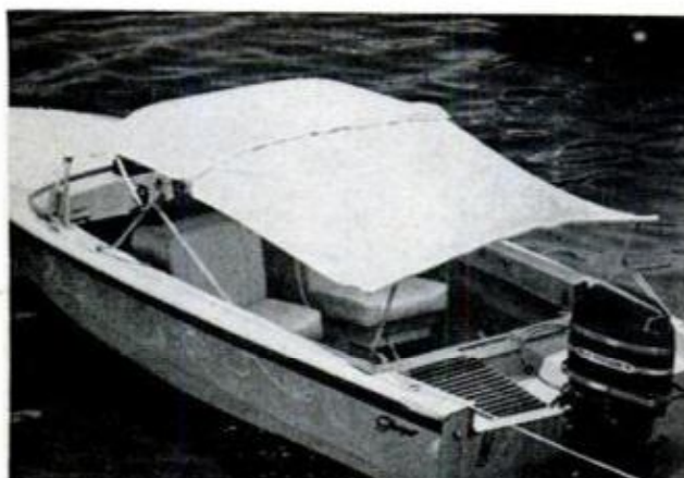
LET IT RAIN. With the homemade Dacron covering over the rear of the cockpit, the boat's occupants are well protected from rain or nighttime dew
