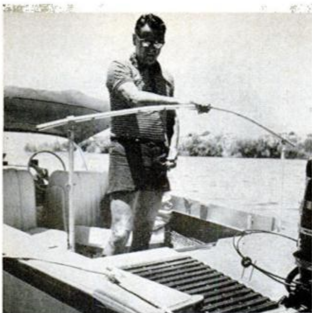
HOMEMADE SUPPORT for a Dacron covering that fits over the rear of the boat's cockpit is made of aluminum tubing and held in place with shock cord
