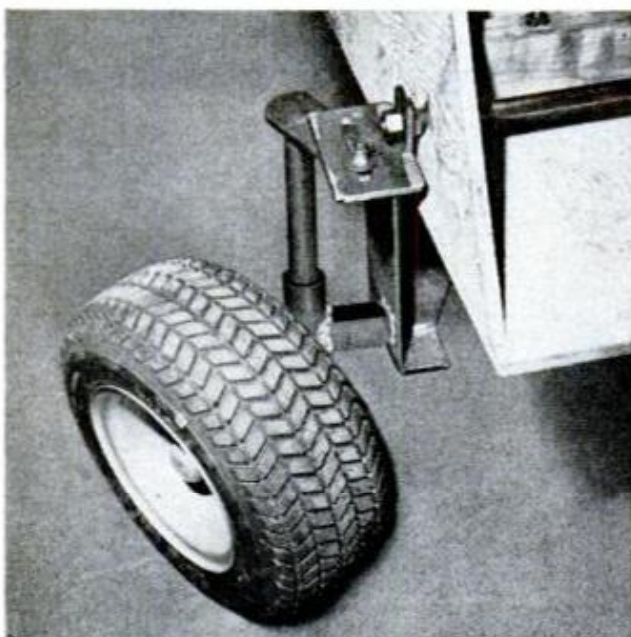
WHEEL BRACKET , a part of the kit, is mounted on the plywood platform and notched into the pontoon
