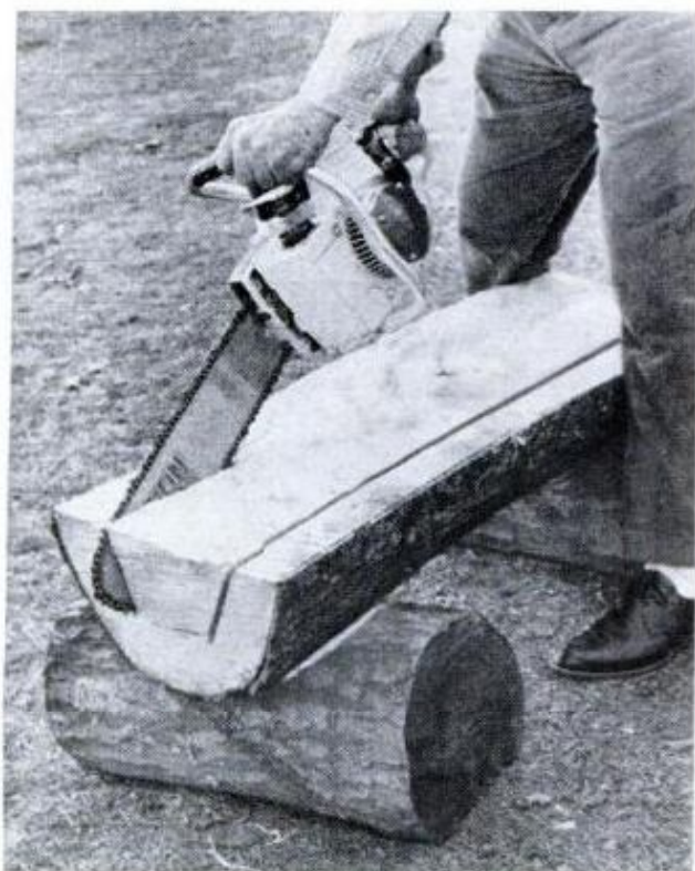
FULL-LENGTH CUTS , running parallel but canted inward, are made to consistent depth in halved log
