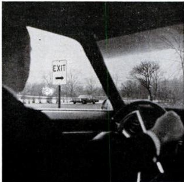
SINGLE FRONT WINDOW is boost to visibility, but ventilation system no match for old vent windows
