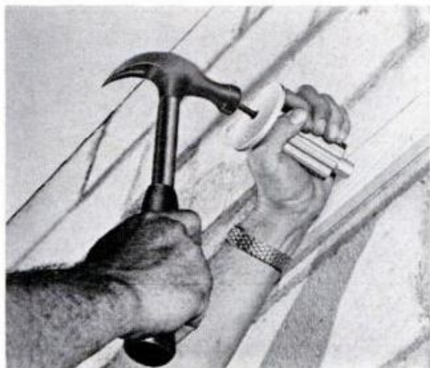
HANDY, FAST FASTENING TOOL will nail furring strips—or almost anything—to hard masonry surfaces nearly as easily as you'd drive a nail into wood
