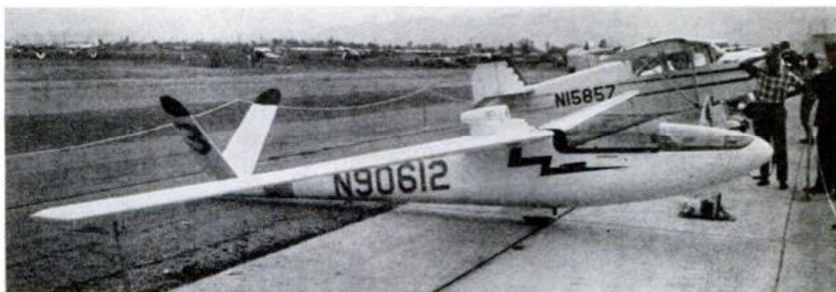
JET ENGINE is mounted piggyback on sailplane for initial test flights, boosting it to 1000 feet
