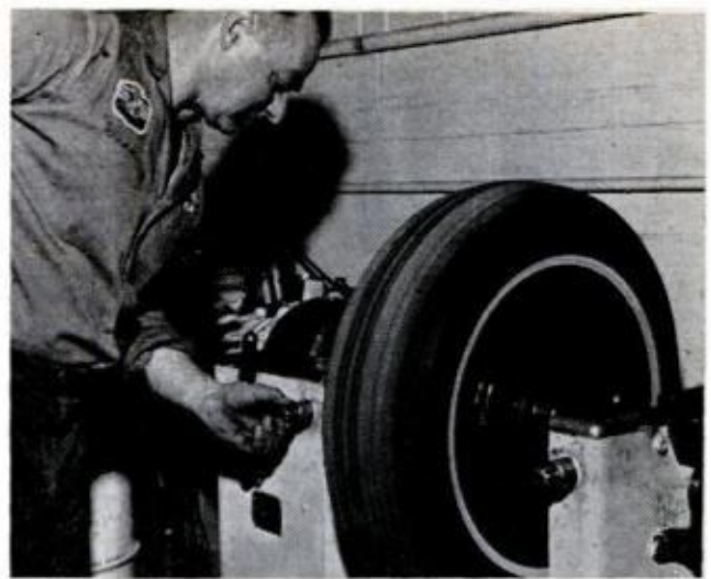
WHEEL IS THEN TURNED on balancing machine to show if it's unbalanced statically or dynamically
