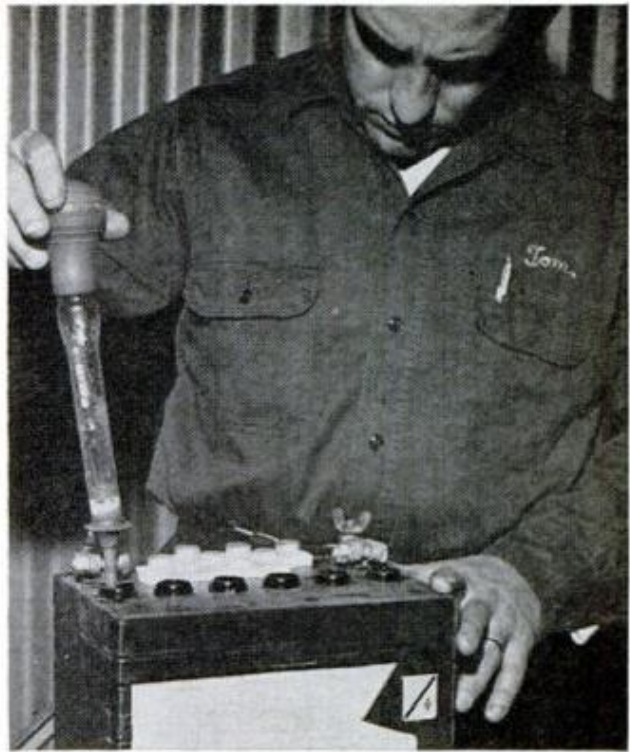
HYDROMETER TEST checks the overall condition of your battery plus the health of each individual cell. It's a troubleshooting must with all starters
