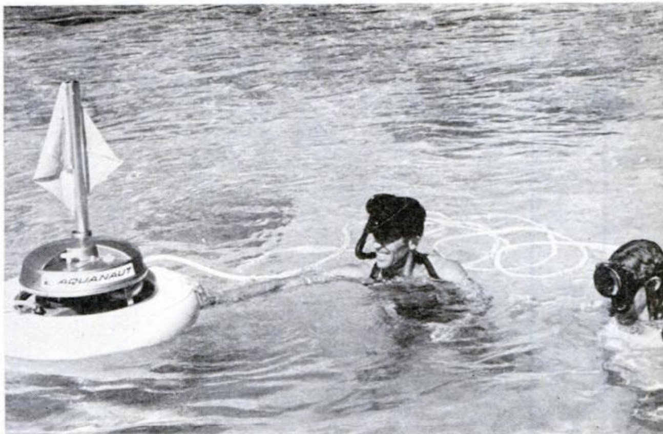
Breath of fresh air. By eliminating compressed-air tanks strapped to the backs of divers, a new power-driven compressor, which floats on the surface and delivers air at the rate of 2.35 cu. ft. per minute or more to 25-foot depth, allows more freedom of action in underwater exploration. Made by Evinrude Motors, Milwaukee, Wis.
