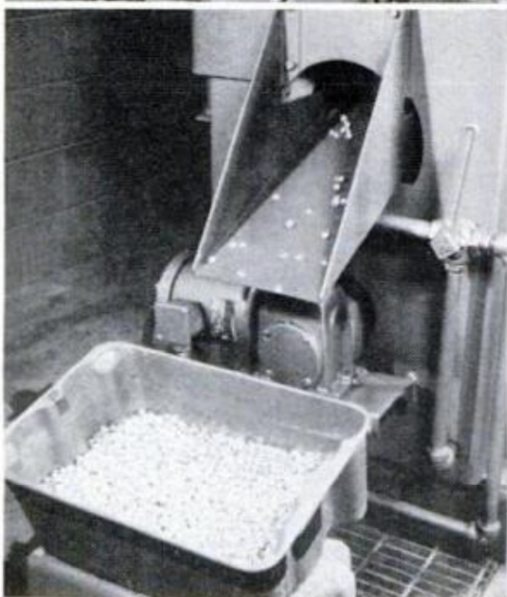
INSIDE BARREL small metal parts are "hammered" by bouncing glass beads until they have a burrished finish. Process is called peen plating
