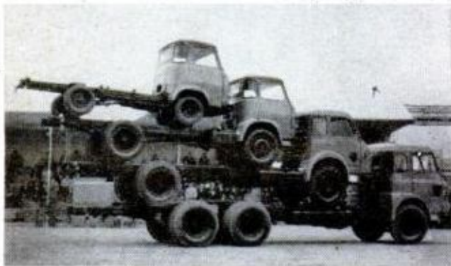
Illegal load. New model Saviem trucks from France stacked four-high make an unusual display at their debut showing. Low truck on the pyramid is a 235-hp diesel rated to carry almost 20 tons, the limit for this vehicle on French roads. Each unit has a useful payload of almost twice its own weight. Loaded, the smallest truck weighs 3.85 tons.
