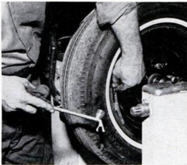
WHEEL BALANCING consists of adding or removing weights to wheel. Weights range from \frac{1}{4} to 16 oz.
