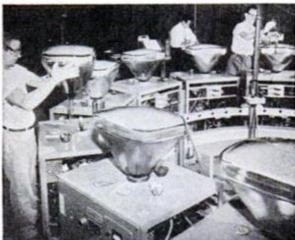
MOVING CARTS create a vacuum inside TV tubes, allowing aluminum vapor to become bonded to the glass. The operation is completely automatic
