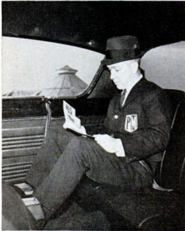
FASTBACK STYLING leaves rear-seat headroom, but rear window fogs up, is hard to keep clean
