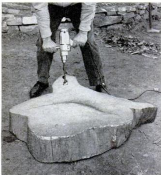
GIANT AUGER BIT — 1\frac{3}{4} -in. dia.—bores 3-to-4-in. deep sockets in bottom face for driving in three legs
