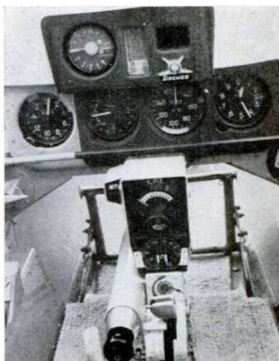
THROTTLE CONTROL and engine gauge is mounted in cockpit between pilot's knees in test sailplane. Other instruments are standard gauges
