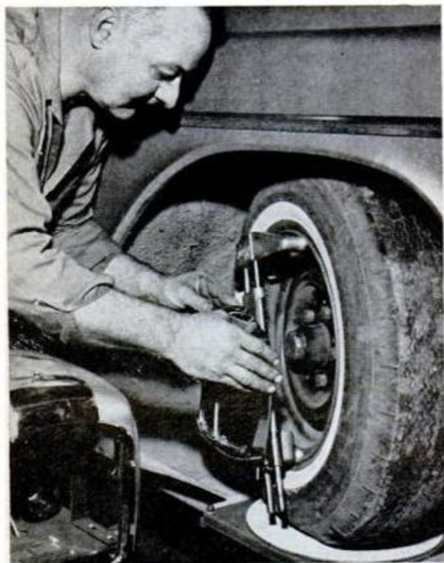
SPECIAL WHEEL GAUGE measures steering axis inclination. Projector (left) throws readings on a screen
