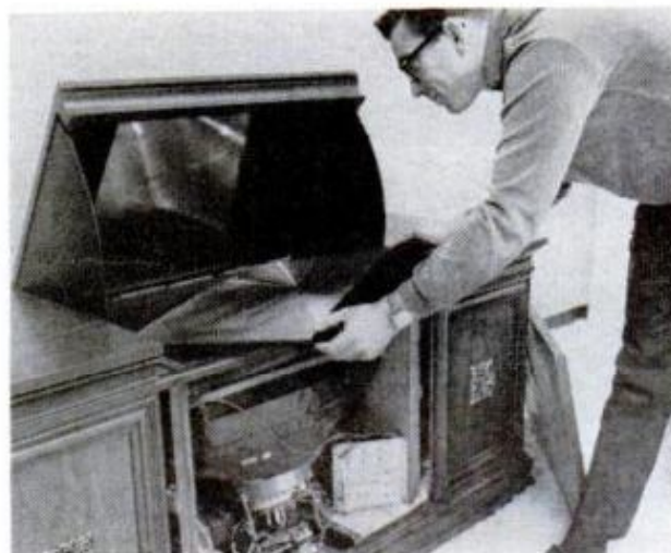
OPTICAL SYSTEM is uncovered by removing front cabinet panel. Plastic lens is above the color tube
