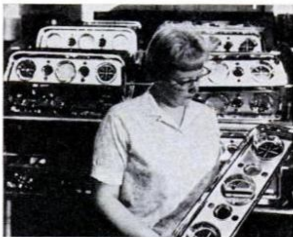
PLASTIC IS BONDED to metal before dashboard sections are stamped out, giving them built-in finish and eliminating need for final spraying
