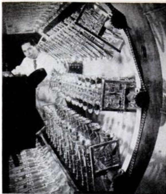
METALIZING OF TOY TRUMPETS is done in vacuum chamber. Coating material is heated to gas and is deposited, atom by atom, on surfaces of toys
