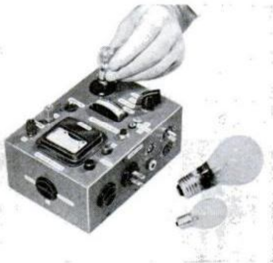
WITH ROTARY SWITCH SET at "lamps", all types of bulbs can be tested, both flash and incandescent
