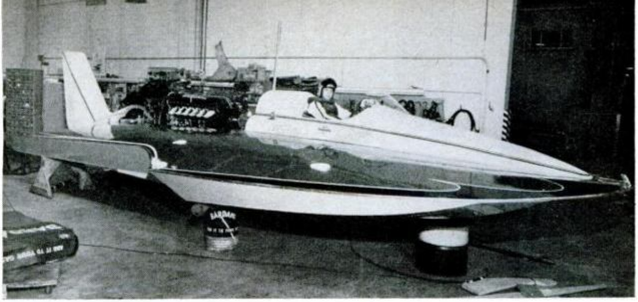
BIG ROLLS engine is swung into place for installation. It'll be covered with a streamlined canopy
