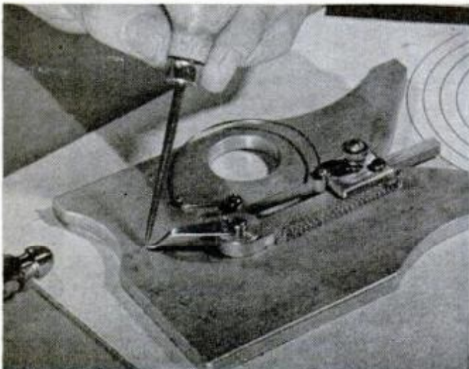
TEMPORARY PUNCH MARKS and penciled scale of calibrating operation will be engraved and stamped
