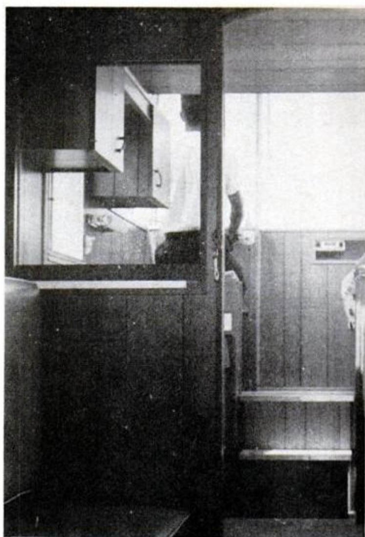
LIVING QUARTERS , below cockpit, included small galley and dinette and four bunks. Two-burner alcohol stove, sink and icebox provided for meals
