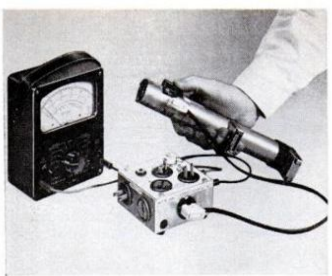
SUPPLEMENTARY TEST BOX , plugged into the VOM, is being used to check B. C. or D-size flash cells
