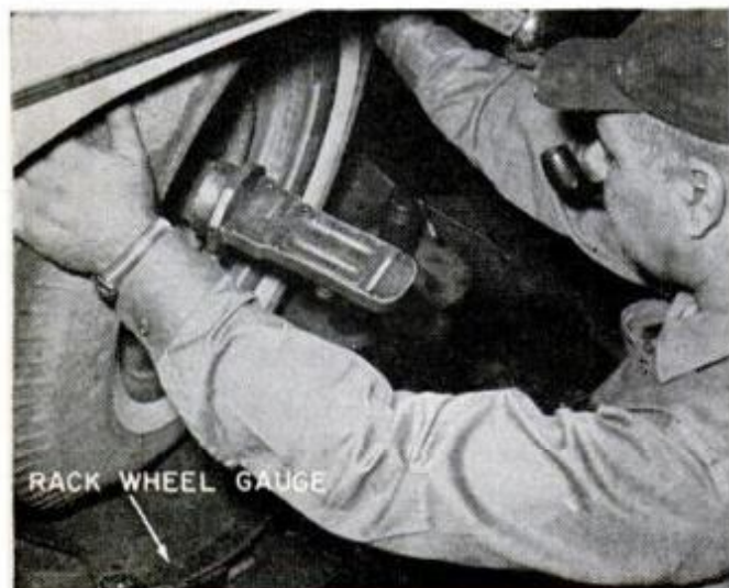
CASTER CHECK: Wheel is turned out 20^\circ , then in 20^\circ . The gauge reading should match manufacturer's specs
