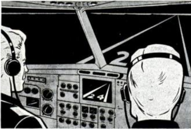
PILOT'S EYE VIEW of laser "radar" in use might be something like this. The painted runway limits stand out clearly against the ground on radar screen
