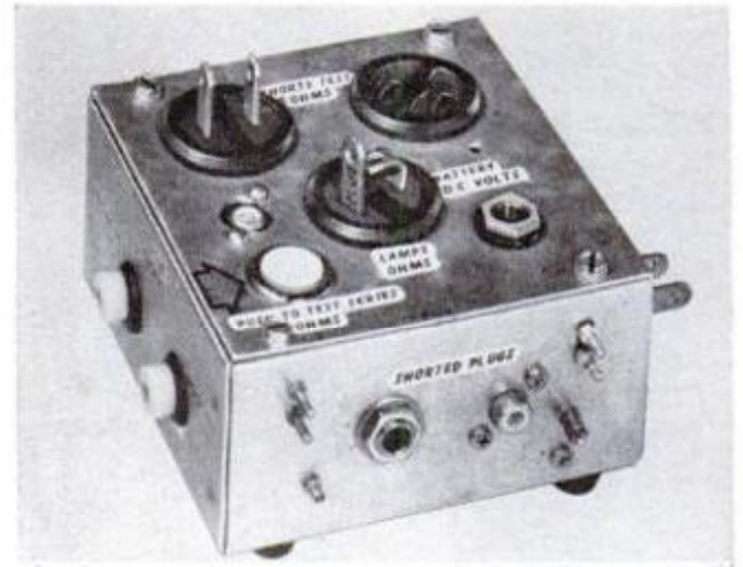
HERE IS THE COMPLETED supplementary test box showing location of all components properly identified
