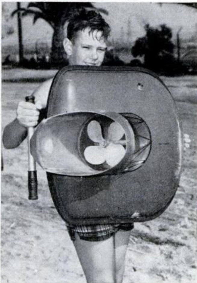
Joyriding swimmers and lifeguards may be towed at up to 5 mph by this motorized float called the "Polliwog." A small instrument panel contains recoil starter, throttle and choke. Steering is accomplished by leaning on handlebars into the desired direction. Priced at $229, it is manufactured by La Habra Plastics Engineering Co., La Habra, Calif. 90631.
