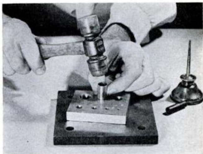
TO SHRINK THE END of a tube, place the shrink plate on a solid surface, apply a little oil to the hole to be used and strike the tube with a mallet. End will be neatly tapered when tube is removed from hole
