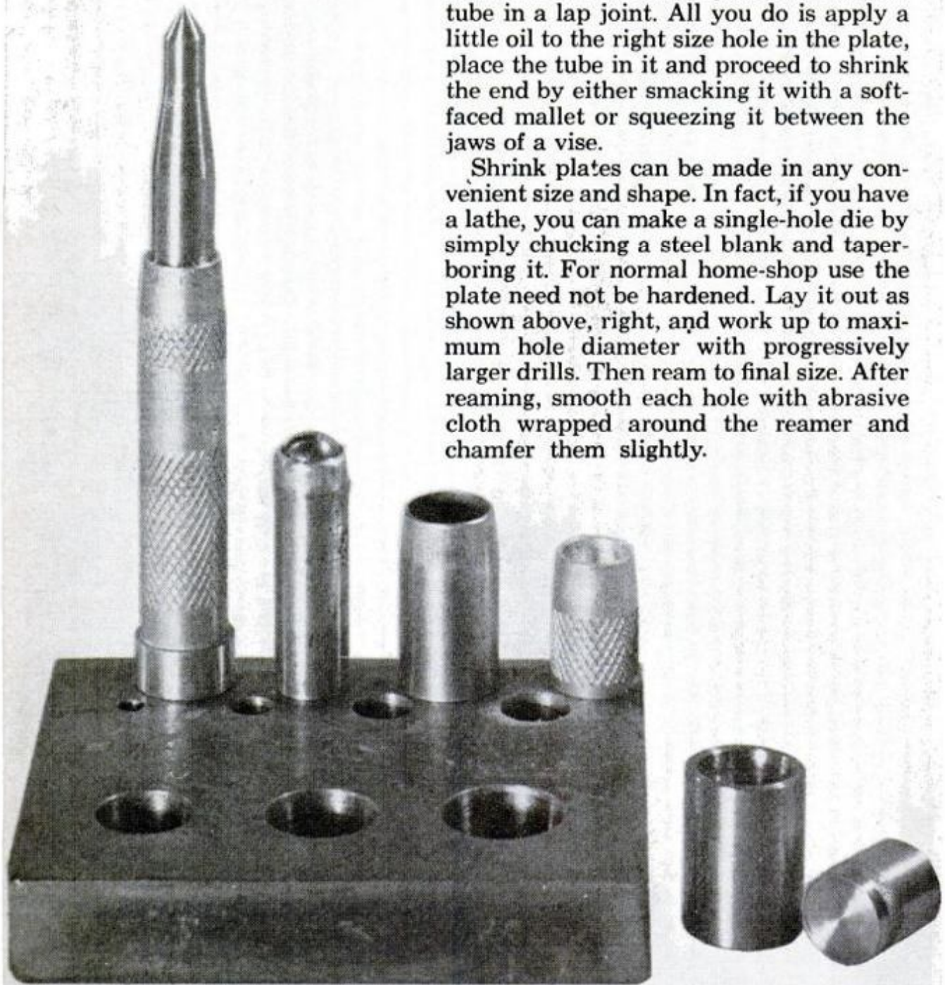
EXAMPLES OF WORK include (left to right) aluminum body of center punch shrunk around hardened shank, copper tube of embossing tool shrunk around steel ball, and two types of ferrule. At far right is the single-hole die used to shrink a disk into the end of the tube lying next to it
