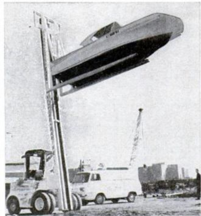
Boating's on the upswing, at least when it comes to launching and dry-docking at the Brooklyn Marina. A forklift designed for the marina lifts boats out of the water (top photo) and deposits them on racks up to three stories high—and returns them to the water just as easily. The lift can handle up to four tons. It takes one operator just five minutes to launch or retrieve a boat.
