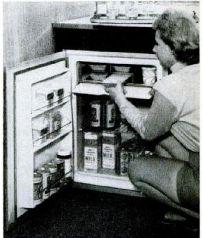
Weekend refrigerator. Designed for boats, a refrigerator keeps ice cubes and frozen food for 48 hours without power. It uses the eutectic principle of storing a "charge of cold" that is released when it is disconnected from outside power. General Thermetics, Farmingdale, New York.
