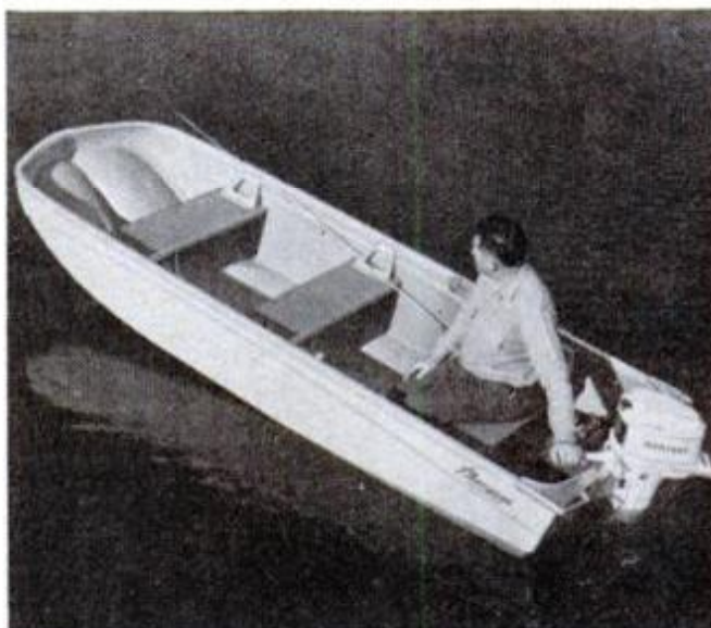
THOMPSON'S 11-foot Take-A-Long fishing boat looks like a streamlined john-boat, weighs 110 pounds. It's molded from Royalex (foam encased in hard rubber)
