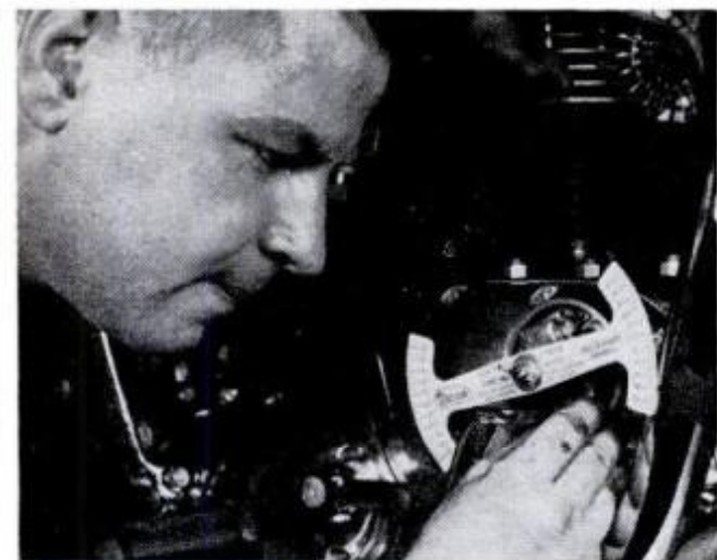
DO YOUR OWN TIMING. It's easy enough using a $3 timer obtainable from your cycle shop. You'll save money too; cycle shops charge up to $10 for this job
