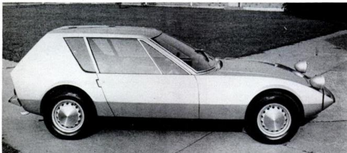
OOPS! FORGOT THE HEADLIGHTS. Special-bodied coupe uses German NSU Prinz 1000 TT chassis, does 105 mph
