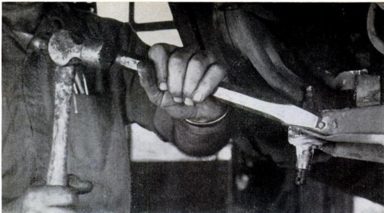
THIS CHEVY HAD RIVETED BALL JOINTS as original equipment. After removing the spindle from the joint, the rivet head had to be chiseled off as shown so that the joint could be taken from the car.
