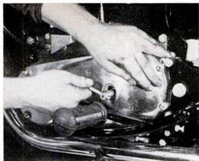
CHECK CLUTCH WEAR by removing access plate on primary case, backing off locking nut of outer clutch plate, adjusting pressure plate as described in text
