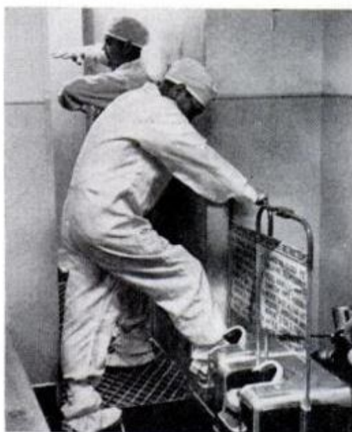
BEFORE ENTERING clean rooms, technicians in lint-free coveralls pass through two filtered air showers that "wash off" dust
