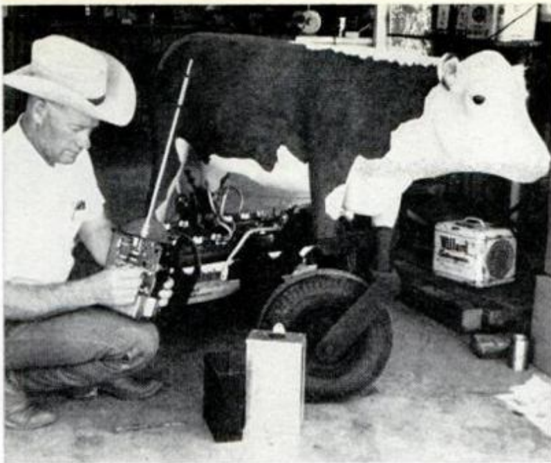
LEE ROY HARRIS, INVENTOR of mechanical maverick, poses with his friend (left) and demonstrates remote transmitter (right). Front wheel is free-swinging and rear wheels are controlled independently so calf can make sharp turns within its own radius. Some models have dual rear wheels for better traction in sand
