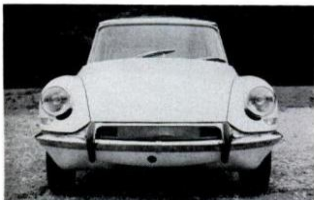
FLOATING HEADLIGHTS in the French Citroen DS 21 seem to be firmly set in fenders, but are counterbalanced to focus on road despite car's pitching
