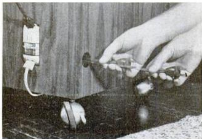
DOUBLE EXPOSURE dramatizes how cord retracts till plug nests inside hole. White cord goes to hot tray
