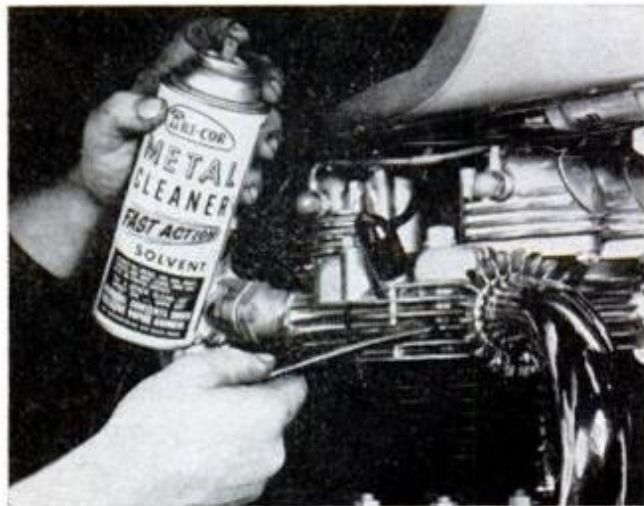
CAKED-ON MUD AND DIRT between the cooling fins will cause engine to run hot. Use a metal-cleaning solvent to loosen dirt so it can be scraped away
