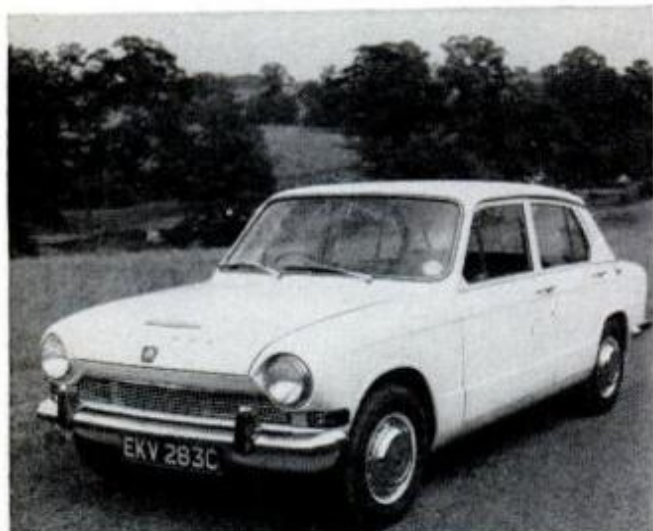
STEERING ADJUSTS for rake and height in front-wheel-drive Triumph 1300 to accommodate any size driver. The $2200 English car has disc brakes
