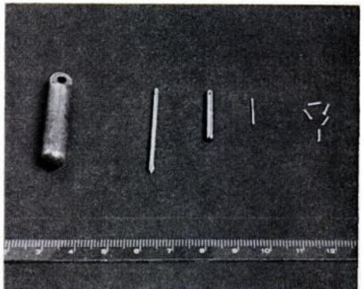
RADIUM SOURCES used in medicine include (left to right) capsule, needle, tube, cell and a gold radon seed for permanent implantation in tissue
