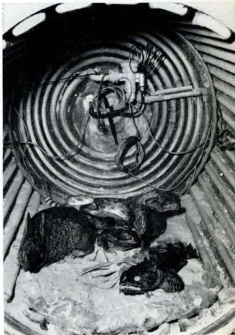
FREEZE-DRY CHAMBER used at Smithsonian can hold several small animals, but largest single one handled was a fox. Unit is exceptionally well insulated
