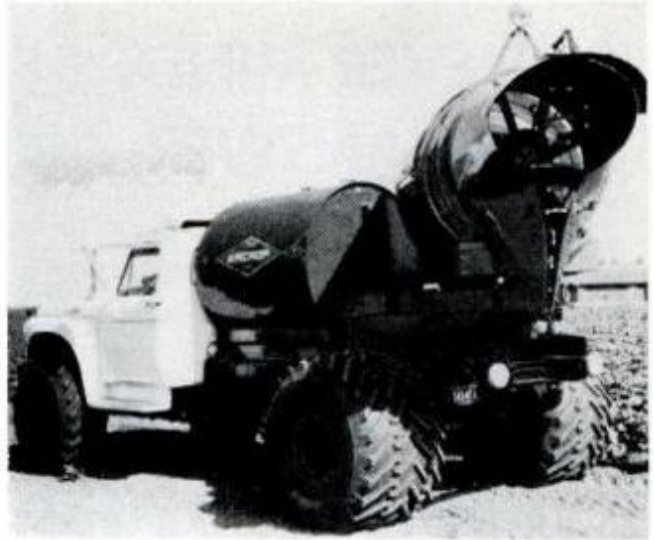
Floating truck. Old boll weevil has always flourished during the irrigation season when spray trucks would bog down in the fields, but a new rig is numbering his days. With the help of Shell Development Co. of Houston, Tex., a California farmer, Gordon Thomas, has equipped a spray truck with Goodyear Terra-Tires. They spread the 15,500 pound weight of the truck so that the force against the ground is only 12 pounds per square inch, allowing the rig to literally float across the soggy fields.
