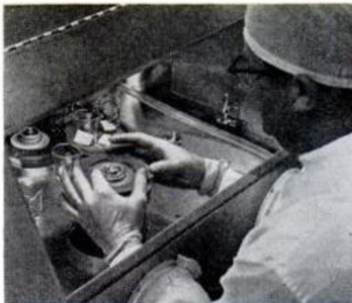
ADJUSTING the memory disc of an inertial guidance system inside a sterile glass shield free of dust and static electricity
