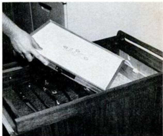
TRAY STAYS LOOSE for easy removal, is kept from shifting by press fit against tiny cleats. Sliding top is removed, here, exposing utensil drawer (left)
