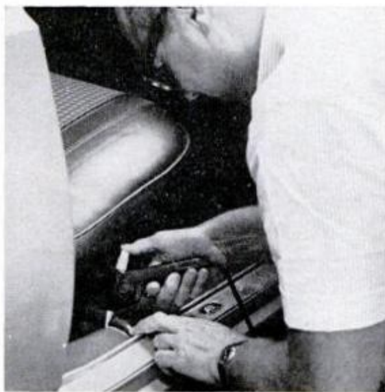
GLUING DOWN a loose auto carpet is a cinch with this new electrically heated glue gun.
