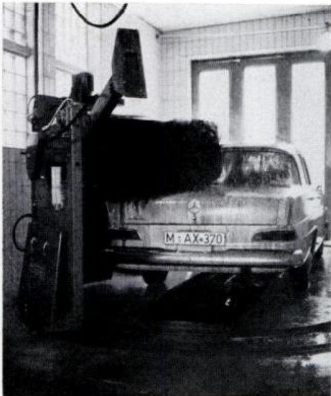
Car washer made in West Germany takes but a minute—30 seconds per side—to do a full-sized car. The fully automatic unit rolls on tracks and moves around the car, which remains stationary. Vertical and horizontal brushes scrub as two nozzles spray the car with water. A chemical in the rinse water is said to speed drying and prevent spotting. Made by Messerschmitt, the washer is distributed here by the Gilbert & Barker Manufacturing Co. of West Springfield, Mass.
