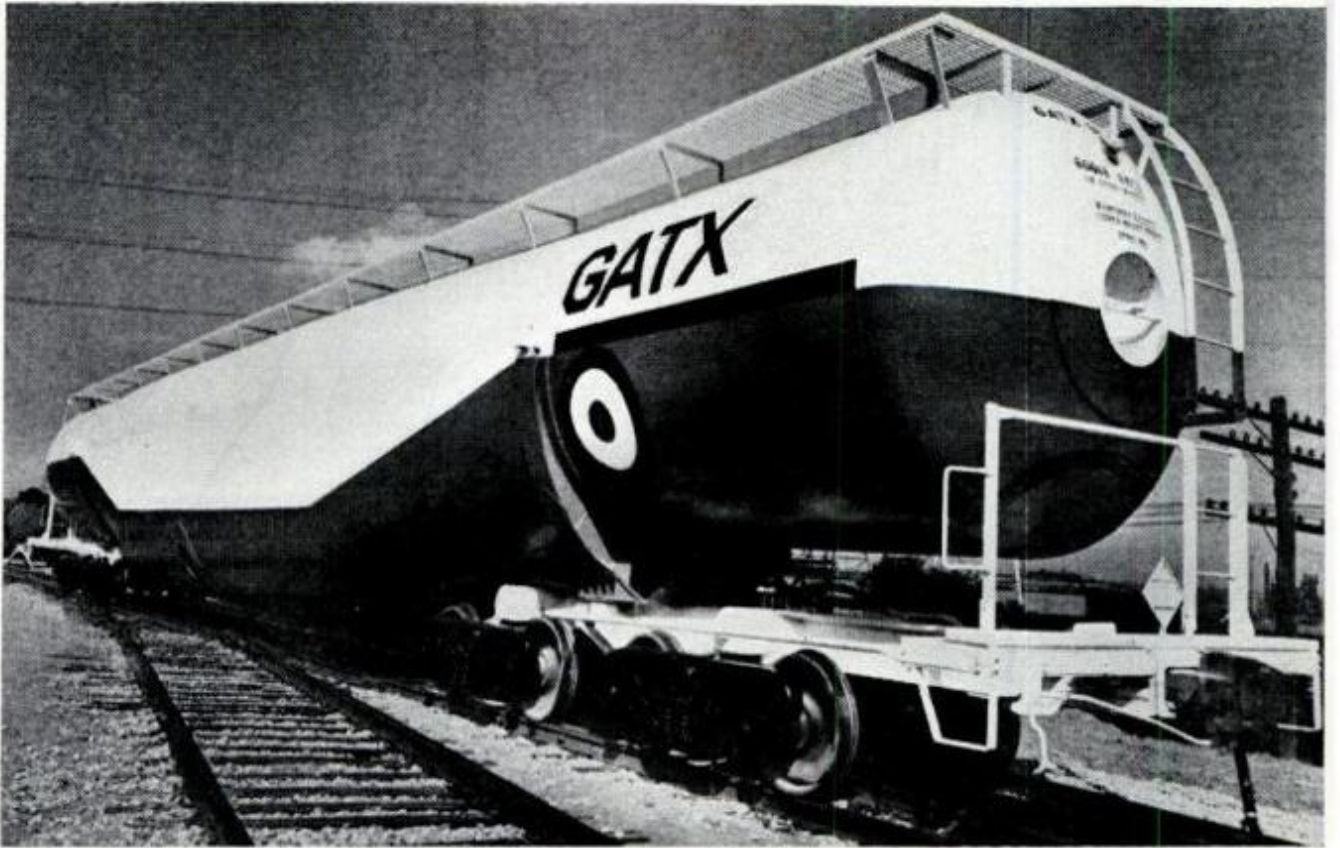
World's largest tank car , with a capacity of 60,000 gallons, is almost three times as long and seven times the volume of the typical tank car in use at the end of World War II. The 96-foot-long car rides on four four-wheel rail car trucks. Introduced as a "rolling laboratory" by General American Transportation Corp., the giant tank will develop working data to indicate its marketing demand.
